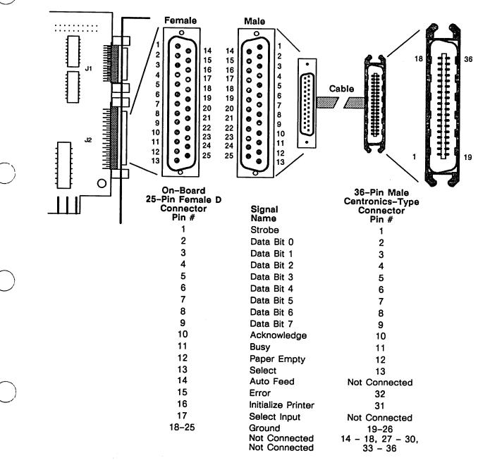
Figure 15-4 shows the parallel port on the IDEAssociates serial/parallel board.
