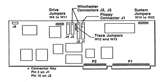
Figure 5–3. 8621 Disk Controller Board Component Locations
