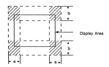
Using the pincushion test signal, the edge of the display image must be within the area indicated by the oblique line in the following illustration.
