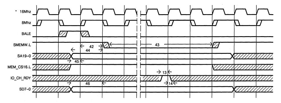
Figure B-6. Bus 8-Bit Memory Write Cycle
