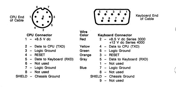
Figure 12-3. Keyboard Cable Connectors
