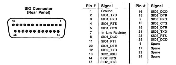
Figure 3-5. DS4000 P2 SIO 3-Port Connector
