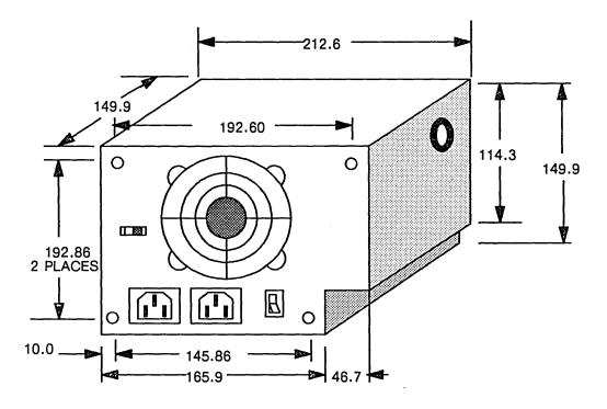
Figure 4–7. Power Supply Physical Dimensions (Centimeters)
