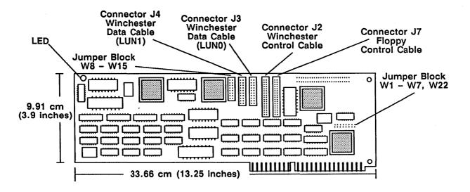
Figure 5–2. 8610 Disk Controller Board Component Locations
