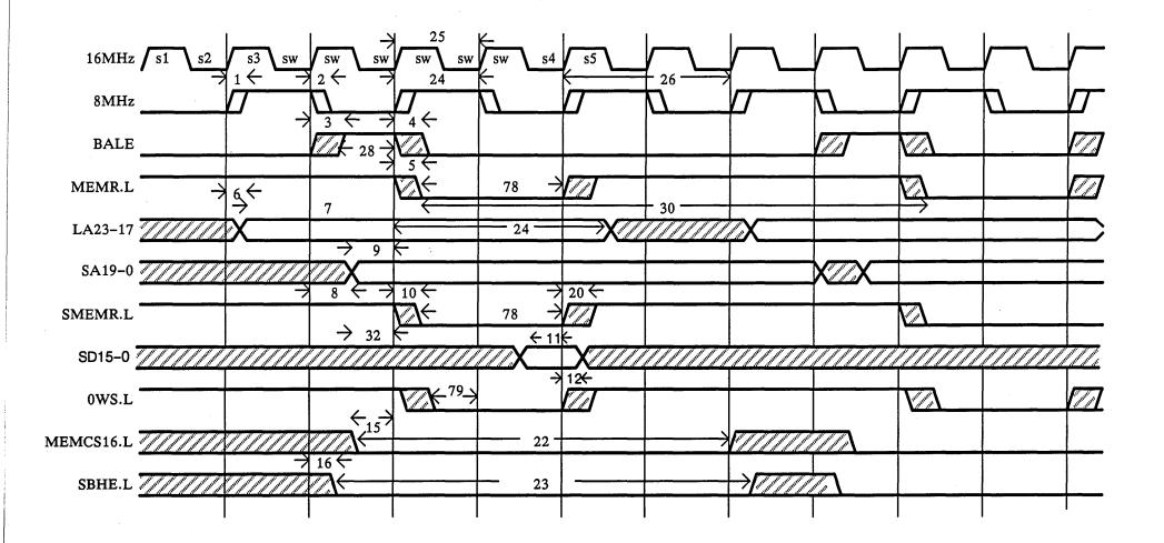
Figure B-14. Bus 16-Bit Memory Read Cycle (Zero Wait State)
