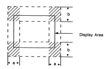
Using the pincushion test signal, the edge of the display image must be within the area indicated by the oblique line in the following illustration.
