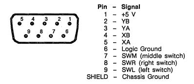
Figure 12-4. Pointing Device Connector (at Keyboard)
