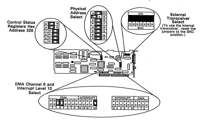
Figure 14–3. Standard 802.3 Network Controller–AT Jumper Configuration (AT–Compatible Slot)
