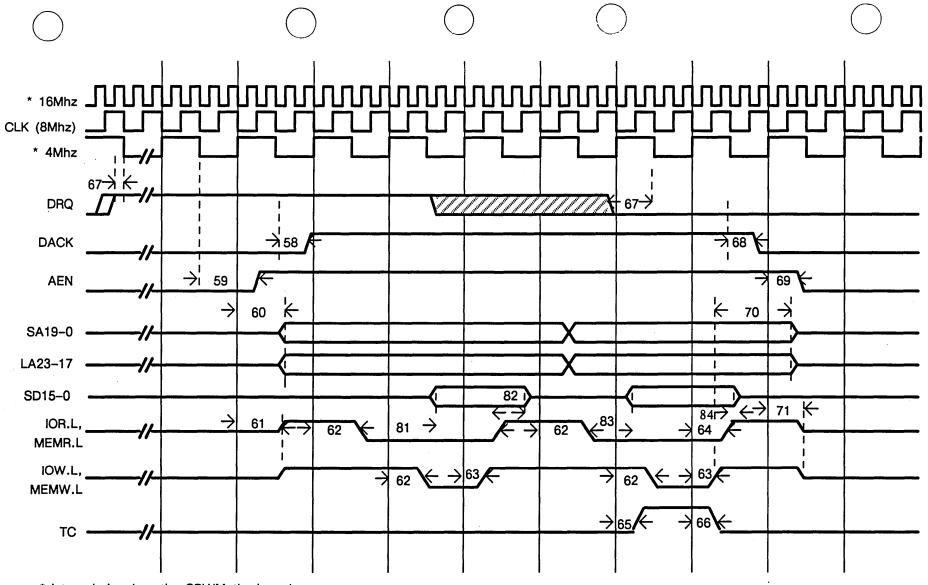
Figure B-9. Bus DMA Cycles
