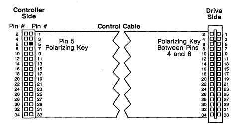
Figure 7–4. Floppy Disk Drive Ribbon Cable Connectors
