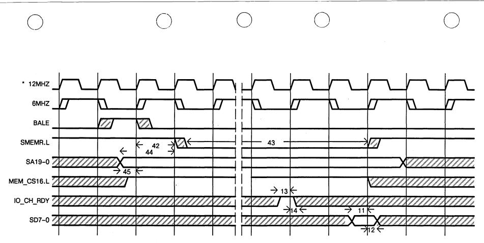
Figure A-5. Bus 8-Bit Memory Read Cycle
