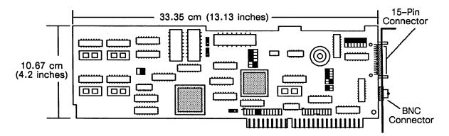
Figure 14–1. 802.3 Network Controller-AT PCB
