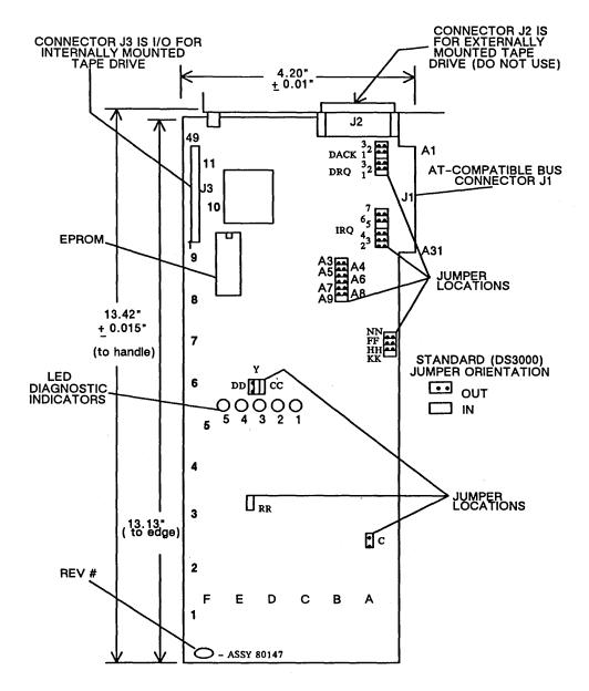
Figure 8–2. Cartridge Tape Controller Physical Layout
