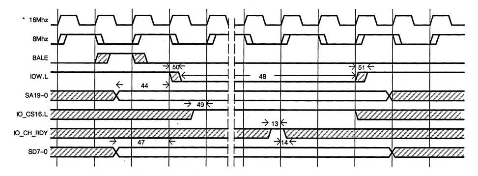
Figure B-8. Bus 8-Bit I/O Write Cycle
