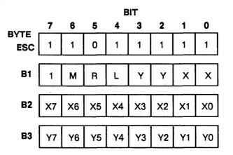
L, M, R = Left, Middle, Right Switch Data; 0 = switch depressed X0 - X7 = X coordinate in signed Two's complement representation Y0 - Y7 = Y coordinate in signed Two's complement representation
