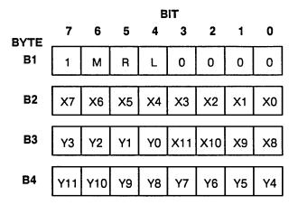
The bits are labelled such that the higher numbers are the more significant bits.
