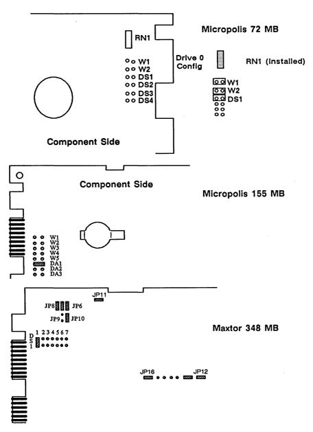
Figure 6–6. Winchester Disk Drive Jumper Configurations
