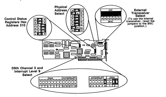
Figure 14-4. Alternate 802.3 Network Controller-AT Jumper Configuration (XT-Compatible Slot)
