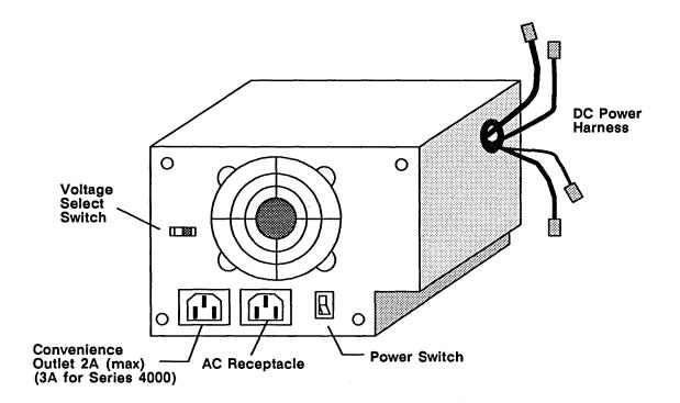
Figure 4-1. Domain System Power Supply
