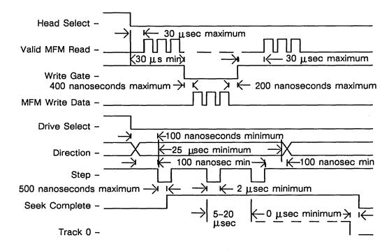
Figure 6-4. Winchester Interface Timing Diagrams
