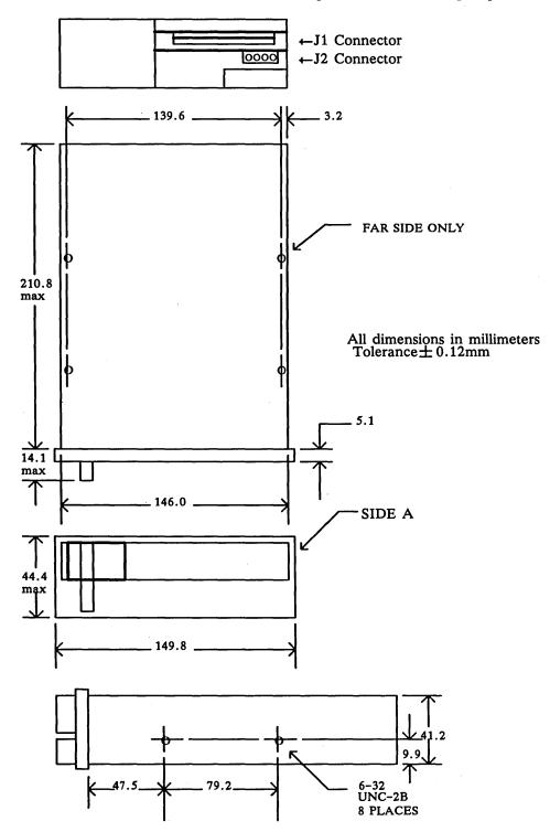
Figure 9-2. Tape Drive Exterior Dimensions and Mounting Holes
