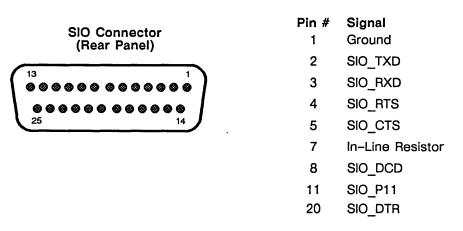
Figure 3–4. DS3000 P2 SIO Single–Port Connector
