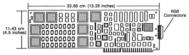
Figure 10-5. 8-Plane Color Graphics Controller PCB
