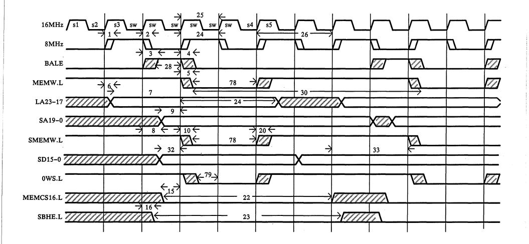
Figure B-12. Bus 16-Bit Memory Write Cycle (Zero Wait State)
