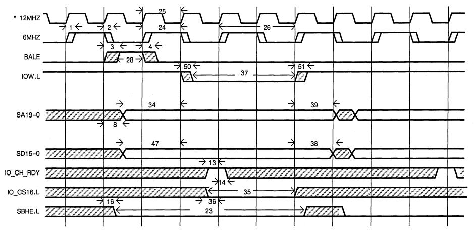
Figure A-4. Bus 16-Bit I/O Write Cycle
