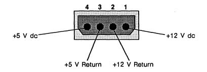
Figure 9–3. Tape Drive Power Supply Input Connector
