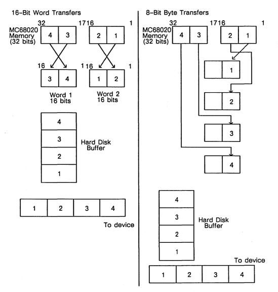
Figure 5-4. Data Transfer Byte Alignments
