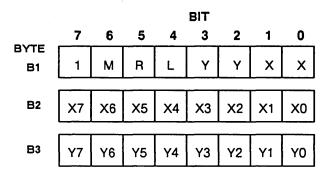
L, M, R = Left, Middle, Right Switch Data; 0 = switch depressed X0 to X7 = Y coordinate in signed Two's complement representation Y0 to Y7 = Y coordinate in signed Two's complement representation
