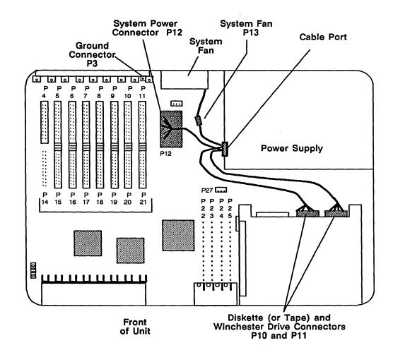
Figure 4-4 shows the destination for the dc connectors in the Series 4000.
