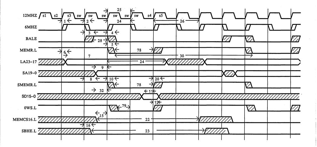
Figure A-14. Bus 16-Bit Memory Read Cycle (Zero Wait State)
