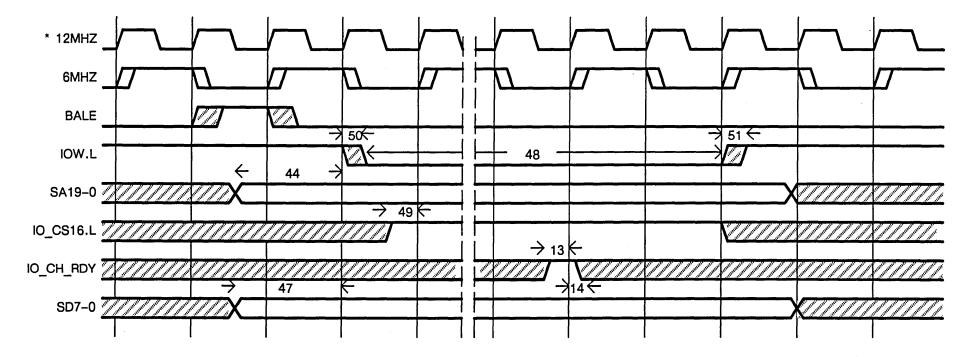
Figure A-8. Bus 8-Bit I/O Write Cycle
