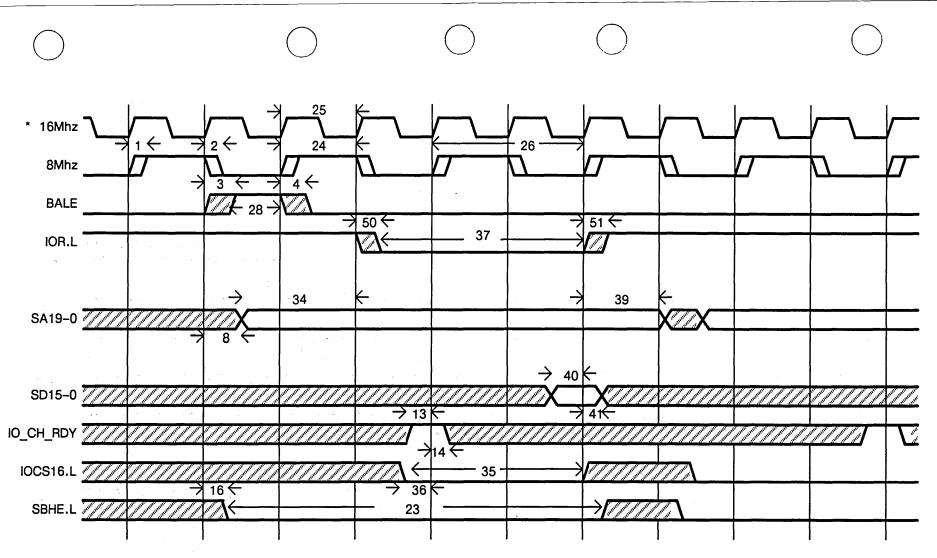
Figure B-3. Bus 16-Bit I/O Read Cycle
