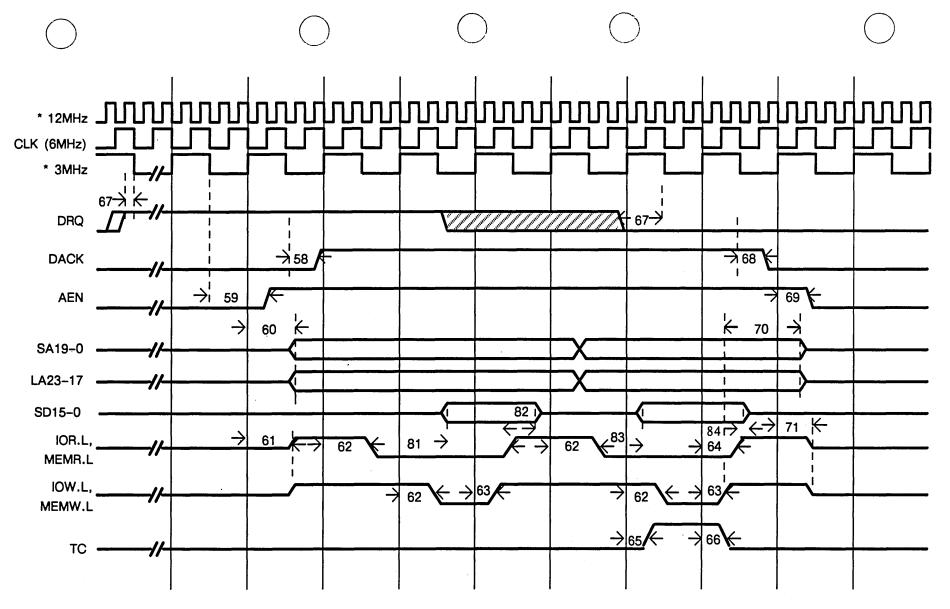
Figure A-9 Bus DMA Cycles
