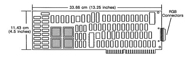
Figure 10–1. 4–Plane Color Graphics Controller PCB
