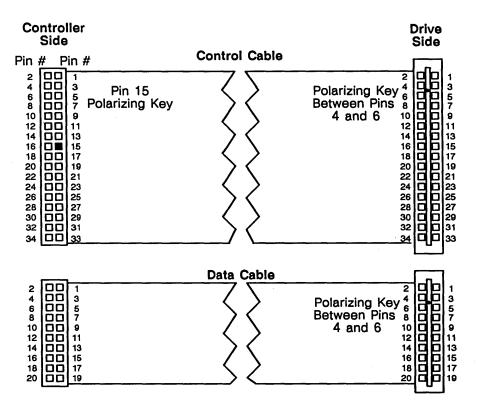
Figure 6-2 shows the ribbon cable connections to the Winchester disk drive and disk controller.
