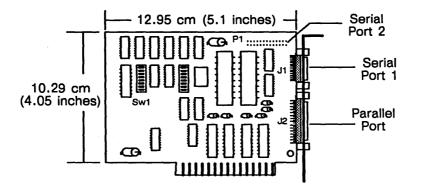
Figure 15–1. IDEAssociates Serial/Parallel Controller PCB
