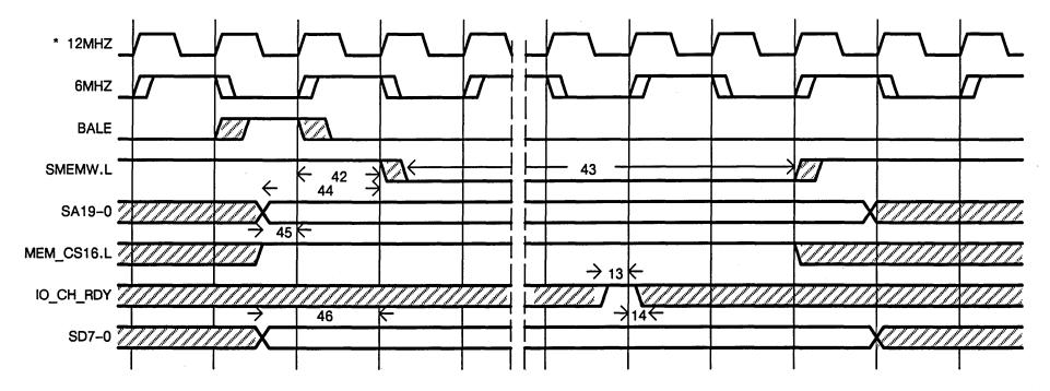
Figure A-6. Bus 8-Bit Memory Write Cycle
