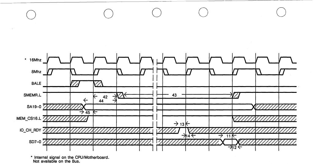
Figure B-5. Bus 8-Bit Memory Read Cycle
