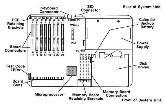
Figure 3-1. Top View of the DS3000 System Unit (With Cover Off)
