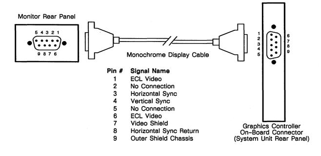
Figure 10-4. Monochrome Display Cable
