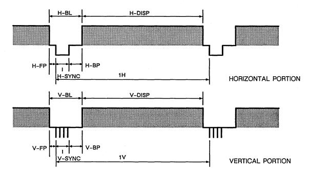
Figure 11-4. Signal Waveforms
