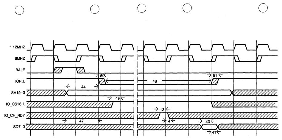
Figure A-7. Bus 8-Bit I/O Read Cycle
