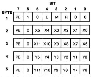
L, M, R = Left, Middle, Right Switch Data; 1 = switch depressed X0 to X11 = X coordinate in unsigned representation (0 to 4095) Y0 to Y11 = Y coordinate in unsigned representation (0 to 4095) PE = Even Parity
