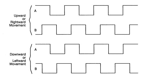
Figure 13–1. Quadrature Clock Signals
