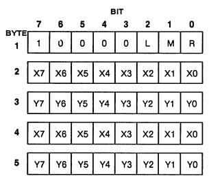
L, M, R = Left, Middle, Right Switch Data; 0 = switch depressed X0 - X7 = X coordinate in signed Two's complement representation Y0 - Y7 = Y coordinate in signed Two's complement representation
