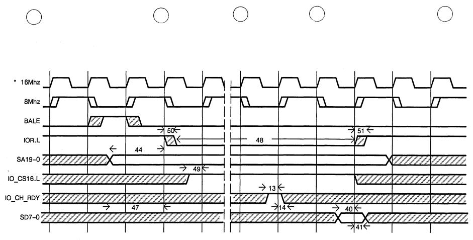
Figure B-7. Bus 8-Bit I/O Read Cycle
