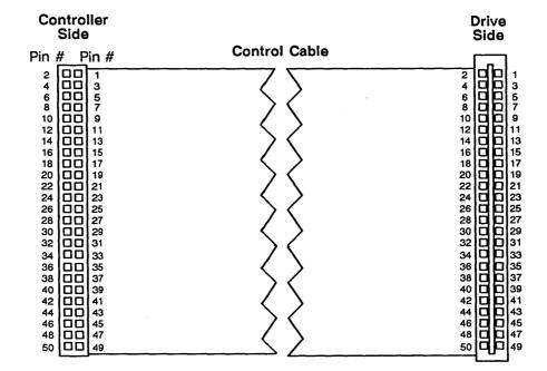
Figure 9-4. Tape Cartridge Drive Ribbon Cable Connectors
