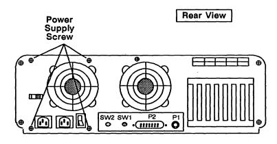
Figure 4-8. Power Supply Mounting
