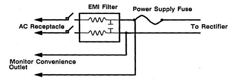
Figure 4–5. Series 3000 AC Lines Protection
