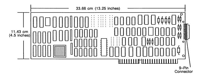
Figure 10–3. 1280 x 1024 Monochrome Graphics Controller PCB
