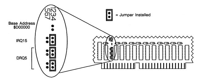
Figure 16-3 shows the alternate jumper configurations for the PC Coprocessor PCB.
