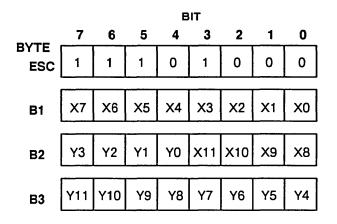
The bits are labelled such that the higher numbers are the more significant bits.
