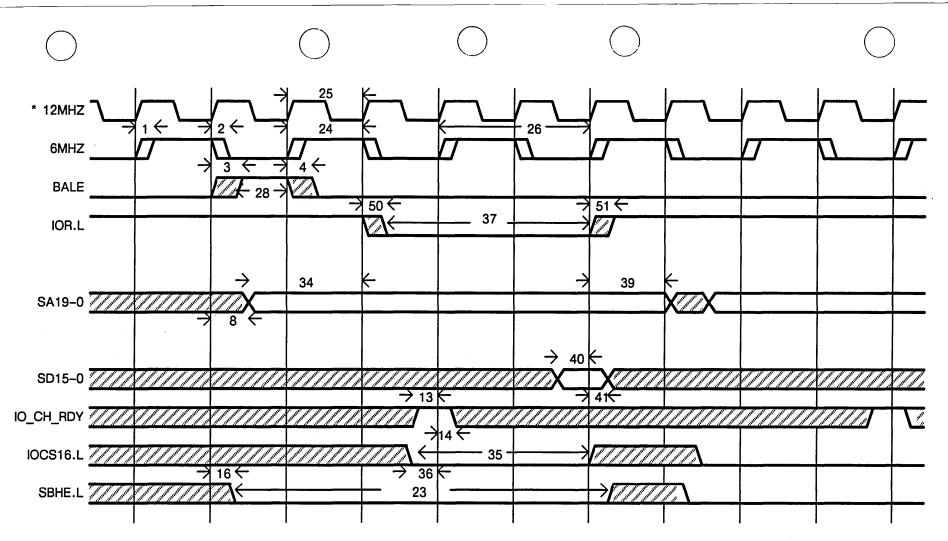
Figure A-3. Bus 16-Bit I/O Read Cycle
