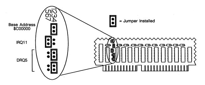
Figure 16–2. PC Coprocessor Standard Jumper Configuration
