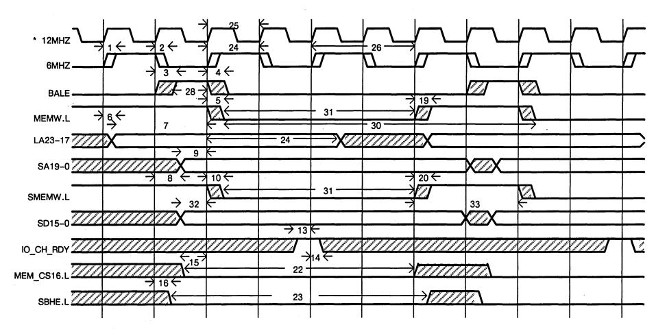
Figure A-2. Bus 16-Bit Memory Write Cycle
