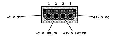
Figure 6–3. P10 Winchester Drive Power Supply Input Connector
