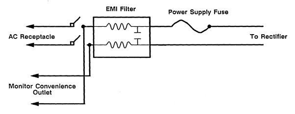
Figure 4-6. Series 4000 AC Lines Protection
