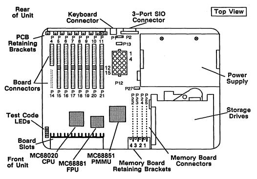
Figure 3-2. Top View of the DS4000 System Unit (With Cover Off)
