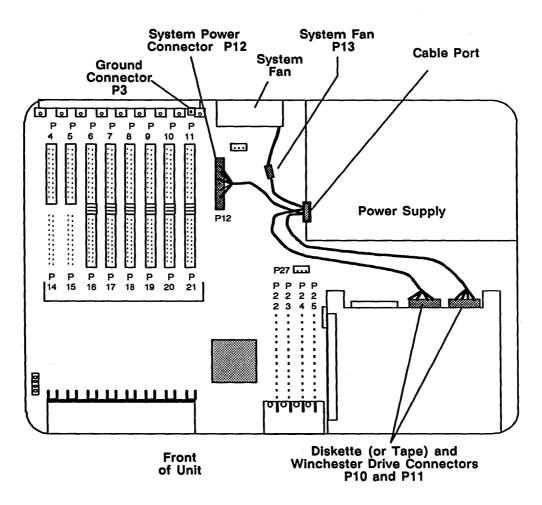
Figure 4–3. Series 3000 DC Connectors Destination
