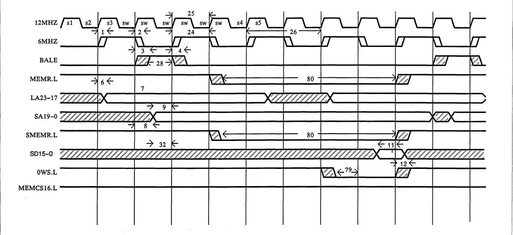
Figure A-15. Bus 8-Bit Memory Read Cycle (Zero Wait State)
