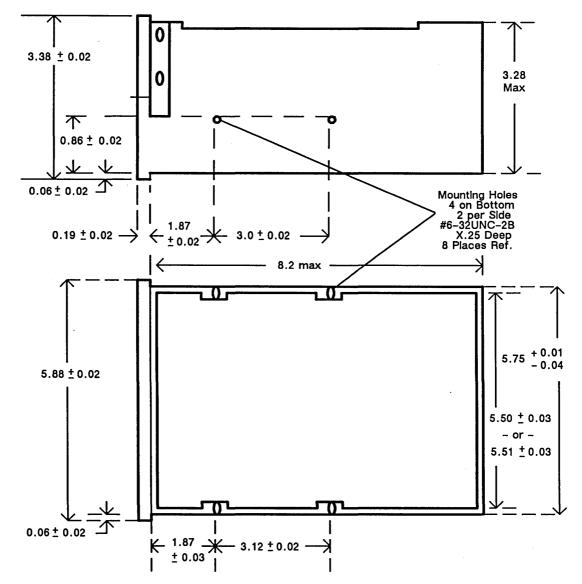
Figure 6-5. Winchester Disk Drive Dimensions
