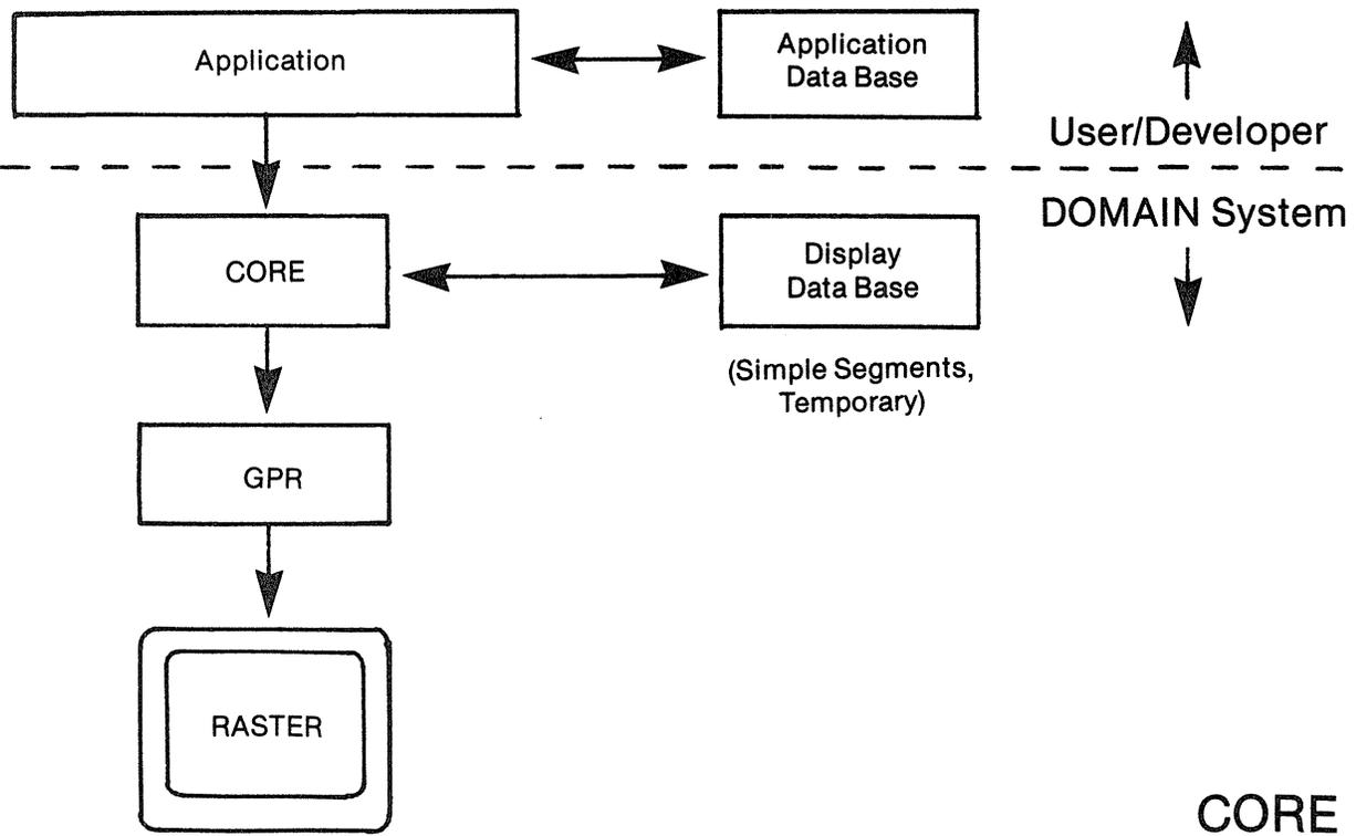
Figure 1-2. Relationship of DOMAIN Graphics: GPR and Core
