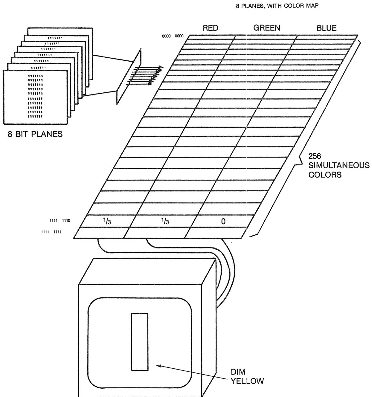
Figure 14-1. The Pixel Value Used as an Index into the Color Map
