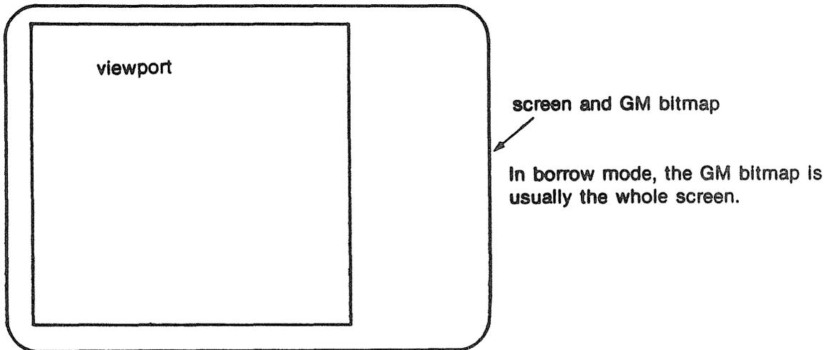
**Figure 2-2. Borrow Mode: Screen and GM Bitmap**
