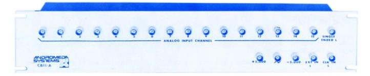
An optional termination box, the CB11-A, provides BNC connectors for all 16 channel inputs as well as 2 external conversion command inputs. The calibration outputs are also brought to BNC connectors. The CB11-A is a 3.5" high rack mountable or free-standing unit. It connects to the ADC11 40 pin external connector with an optional cable.
