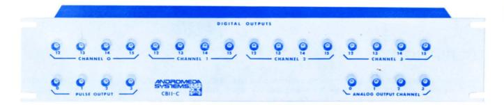
An optional termination box, the CB11-C, provides BNC connectors for the four analog outputs, the 16 digital control outputs and the four pulse outputs. The connector box is 3.5" H and may be rack mounted or free-stand. The CB11-C plugs into the I/O connector on the DAC11 with an optional cable.
