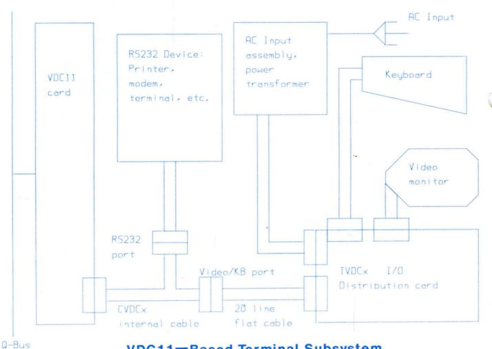
VDC11—Based Terminal Subsystem
