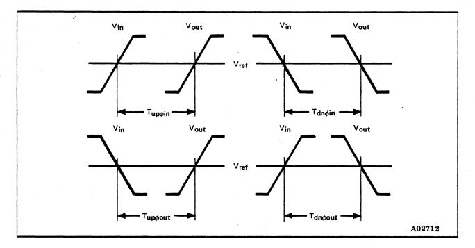
Figure 5-2. Definition of Switching Types
