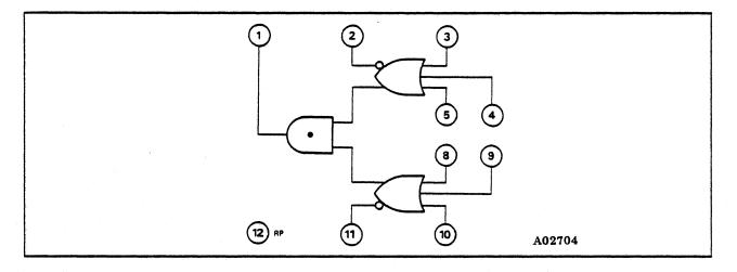
Figure 5-9. Two Wide, 3-Input OR-AND/Dual, 3-Input NOR Macro 11
