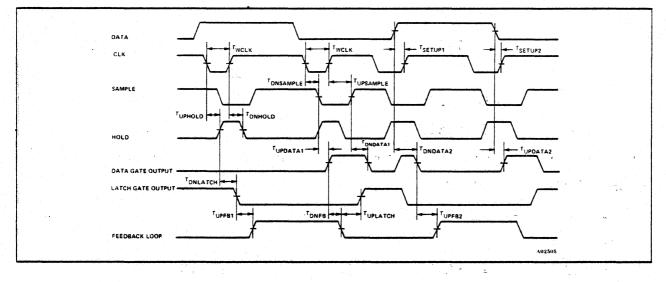
Figure 7-11. Out-of-Phase Latch Timing Diagram
