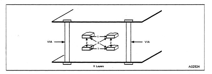
Figure 2-10. Three Types of Parallelism
