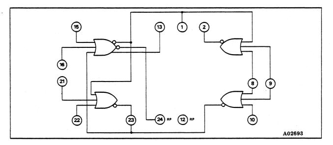
Figure 5-21. Out-of-Phase Latch with Scan-In/Scan-Out Macro 3199
