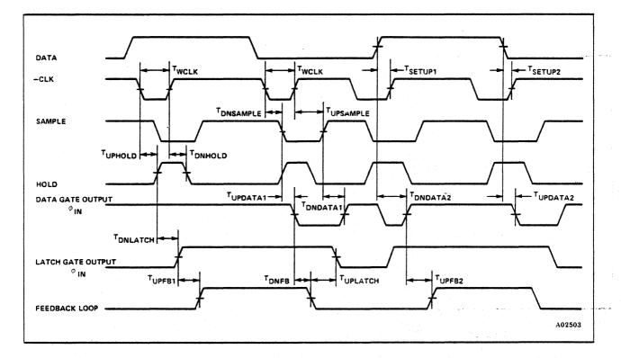
Figure 7-9. In-Phase Latch Timing Diagrams
