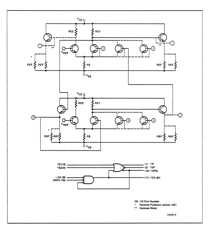
Figure 7-2. Macro 32 Out-of-Phase Latch
