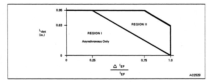
Figure 2-5. Maximum Distance Between Dots for Different Chip Outputs
