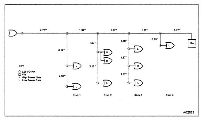
Figure 2-9. Example of Type 2 Non-Critical Net
