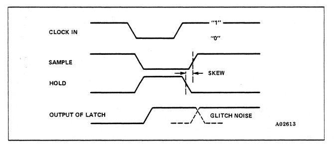
Figure 7-7. Skewed Driver (SD) Signal Waveform
