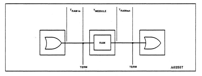
Figure 5-27. Basic RAM Module Delay Definitions
