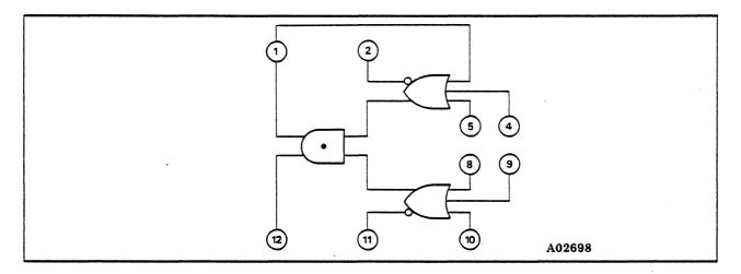
Figure 5-14. In-Phase Latch without Scan-In/Scan-Out Macro 31
