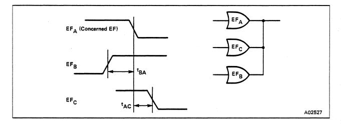
Figure 2-3. Definitions of  $t_{BA}$  and  $t_{BC}$
