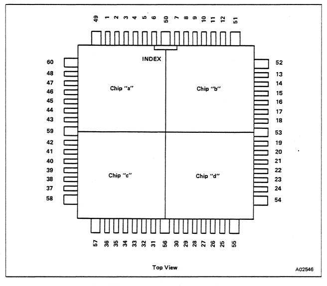
Figure 4-5. RAM Module I/O Assignments
