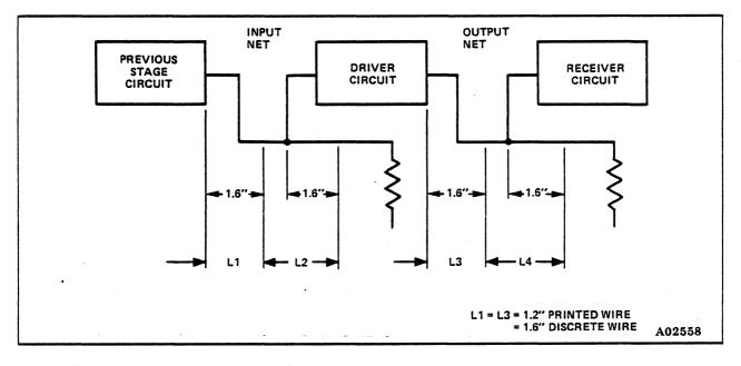
Figure 5-26. Off-Chip Loading Parameters
