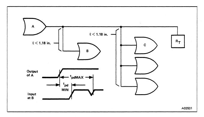
Figure 2-7. Type 1 Delay Equation
