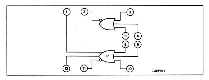
Figure 5-12. 3-Input NOR/3 Input 2 Sample Skewed Driver Macro 21
