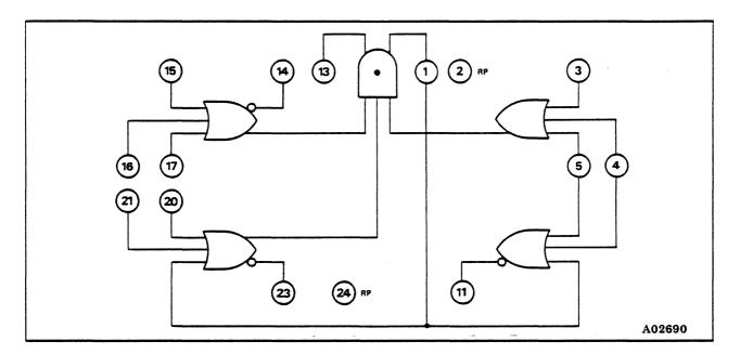
Figure 5-22. In-Phase Latch with Scan-In/Scan-Out Macro 3299
