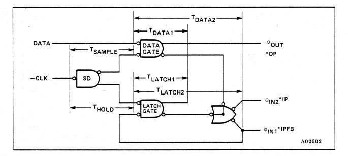
Figure 7-8. In-Phase Latch Path Definitions
