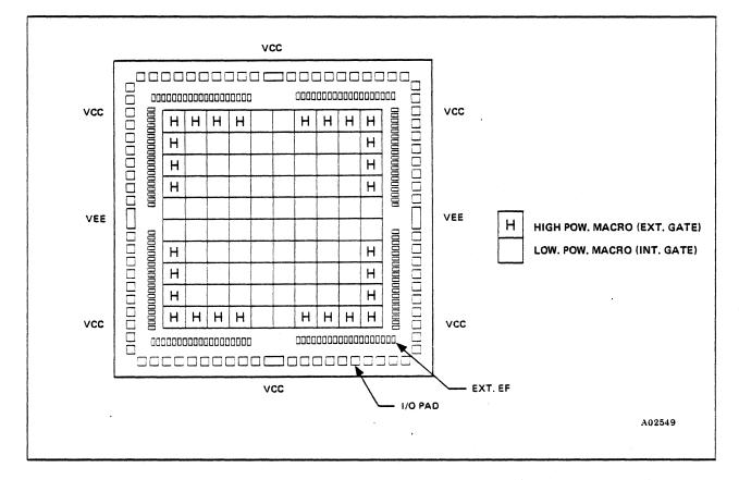
Figure 6-2. High/Low Power Cell Placement
