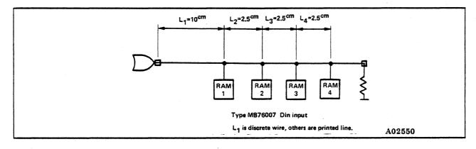
Figure 5-32. Driver Fan-out with Four Input Pins
