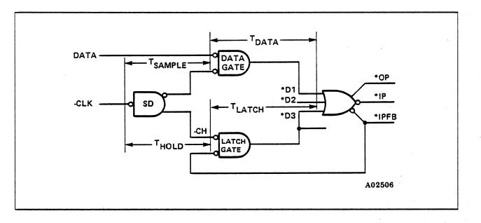
Figure 7-10. Out-of-Phase Latch Path Definitions
