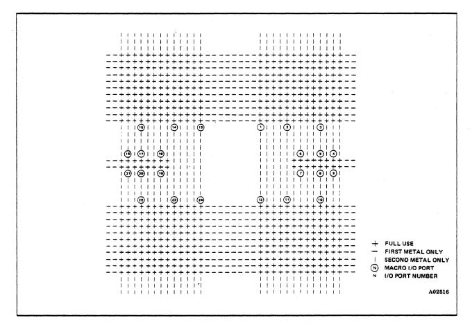
Figure 6-3. Interconnect Grid and I/O Hit Ports (Full Macro)
