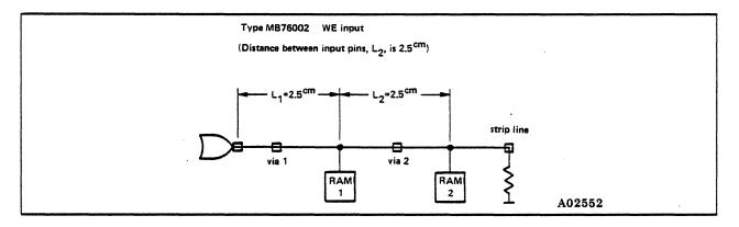
Figure 5-30. Driver Fan-out with Two Input Pins (Up-Min)
