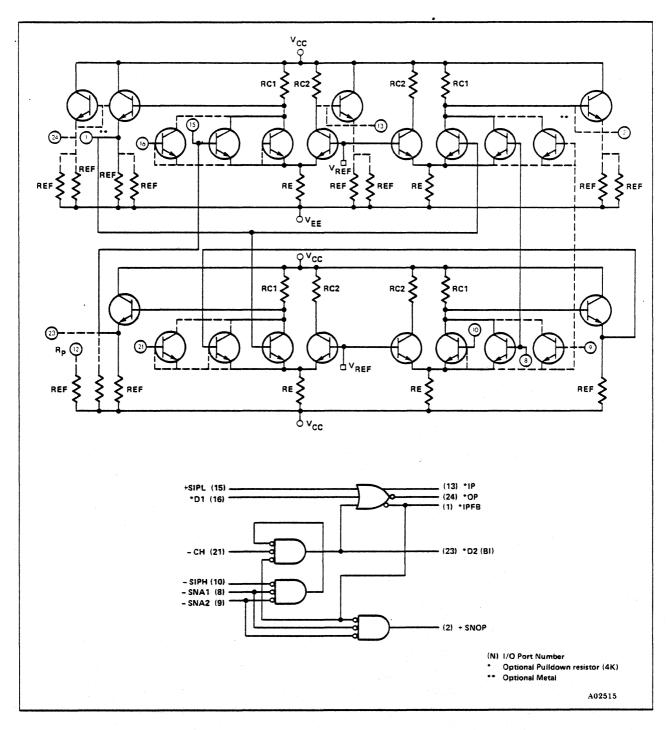
Figure 7-5. Macro 3399 Out-of-Phase Latch
