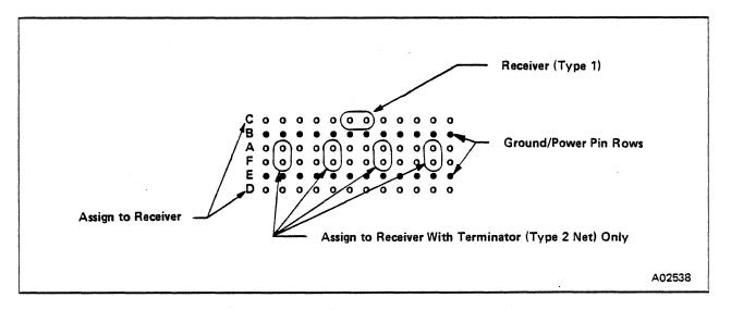
Figure 2-14. Simplified I/O Assignment
