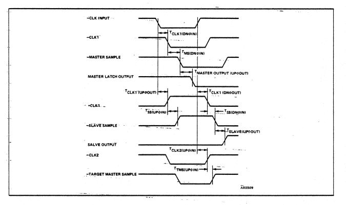
Figure 7-15. In-Phase Latch Timing Diagram
