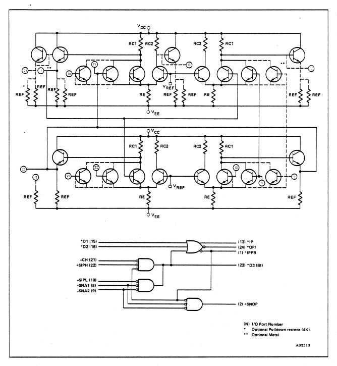
Figure 7-3. Macro 3199 Out-of-Phase Latch
