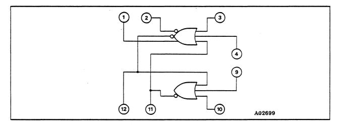
Figure 5-15. Out-of-Phase Latch without Scan-In/Scan-Out Macro 32
