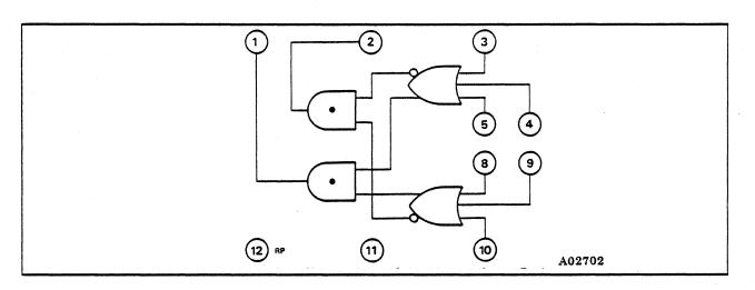
Figure 5-10. Two Wide, 3-Input NOR-AND/2-WIDE, 3-Input OR-AND Macro 12
