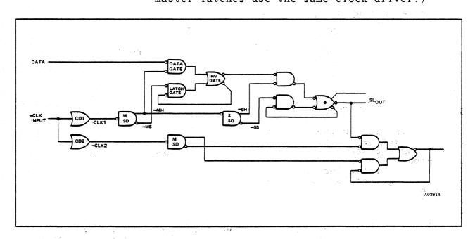
Figure 7-12. Out-of-Phase Master/Slave Latch
