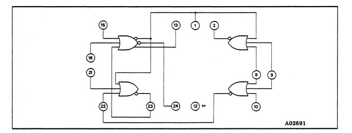
Figure 5-23. Out-of-Phase Latch with Scan-In/Scan-Out Macro 3399
