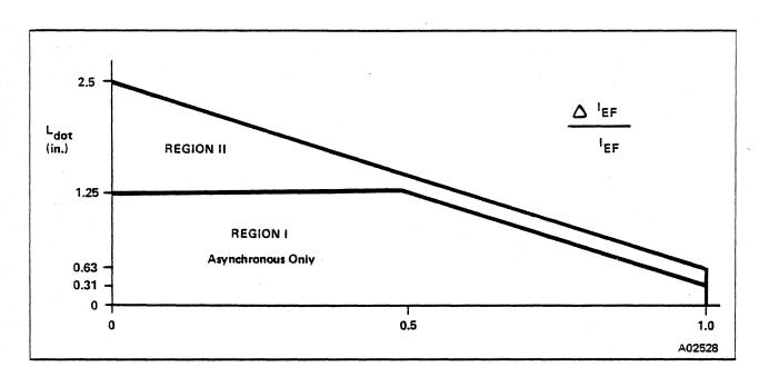
Figure 2-4. Maximum Distance Between Dots for Same Chip Outputs
