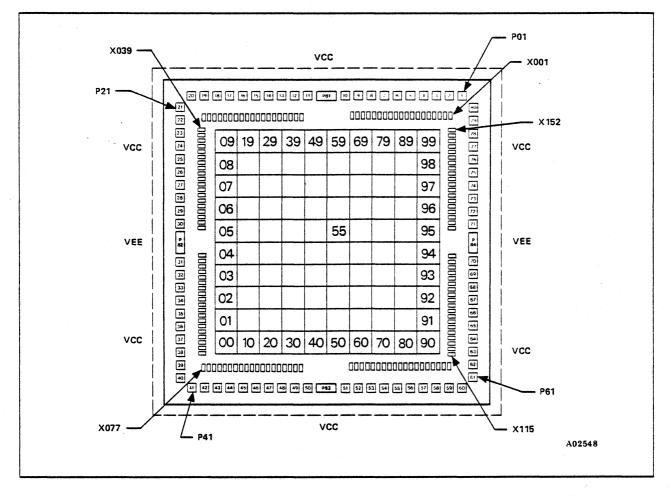
Figure 6-1. LSI Cell Numbering (Chip Top View, Cooling STUD Down)
