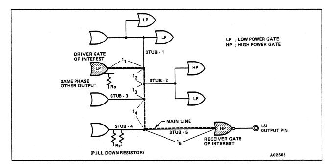
Figure 6-4. Limitations of Internal Net
