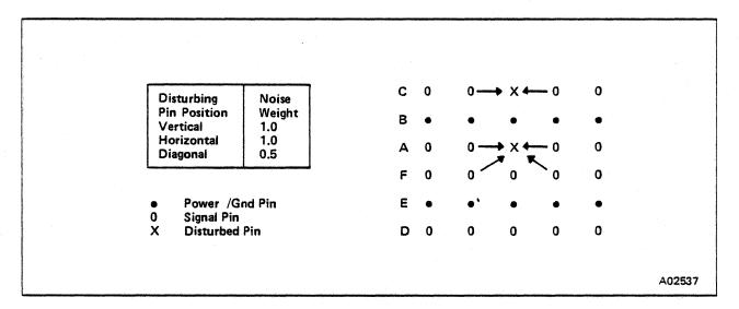
Figure 2-13. Noise Coupling Weight
