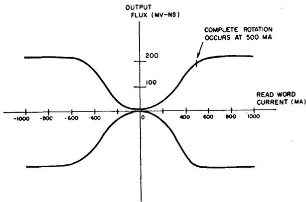
Figure 4—Output flux vs. read word current
