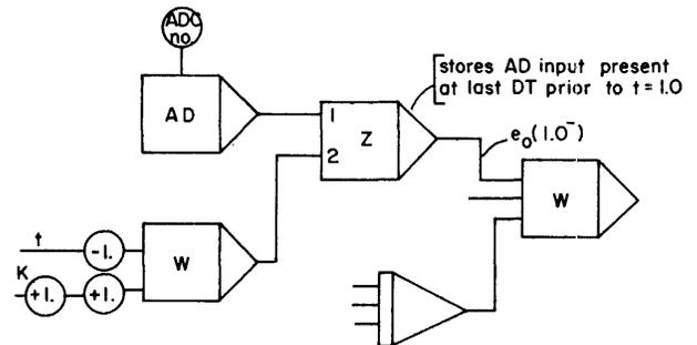
Figure 12—AD block used to modify a parameter at the beginning of a run
