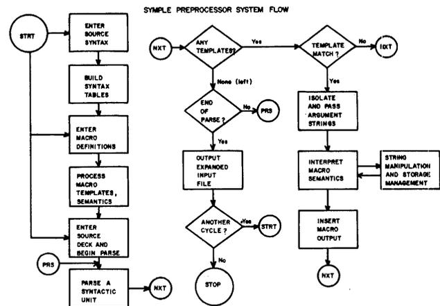
Figure 1—A general flow of the SYMPLE macro preprocessor system
