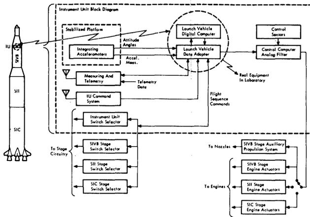
Figure 1—Real and simulated flight equipment
