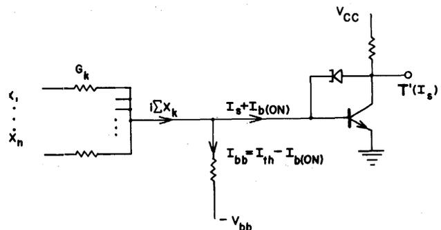
Figure 1—Modified RTL gate with tunnel diode feedback
