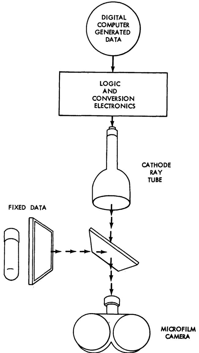
Figure 5—CRT microfilm recording
