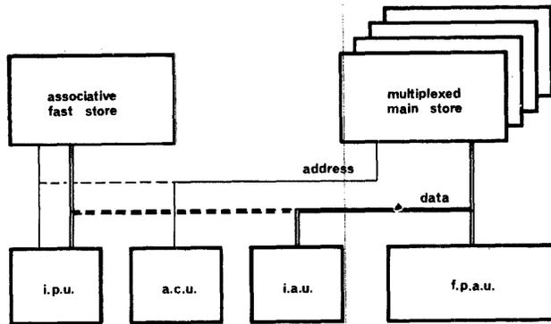
Figure 6—Typical hardware for a future large scale computer
