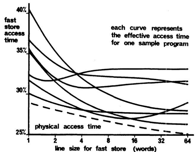
Figure 3—The physical access time of a fast store (broken line) and the effective access times (continuous lines) for several sample programs. Access time is a percentage of main store access time, line size is in words, and store size is 1024 words
