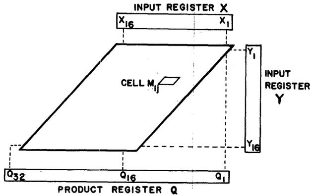
Figure 5—16 × 16 bit functional multiplier.
