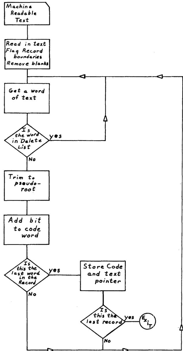
Figure 1—Coding procedure
