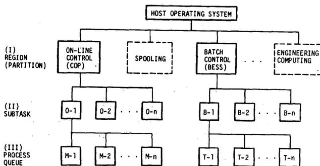
Figure 1—Hierarchical control on three levels of multi-programming
