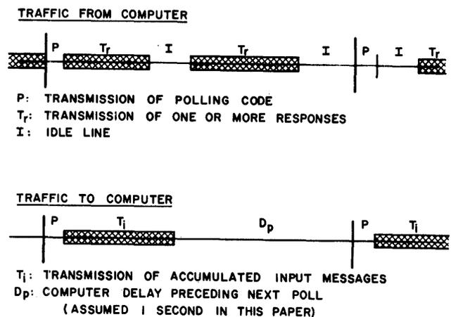
Figure 2B—Typical cycle of operation (Full-duplex message Transmission)
