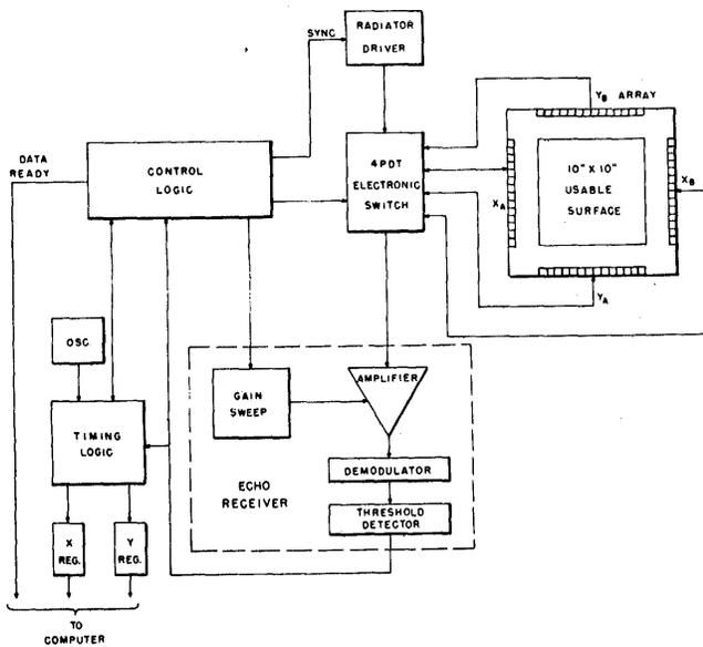
Figure 4—Position encoder block schematic
