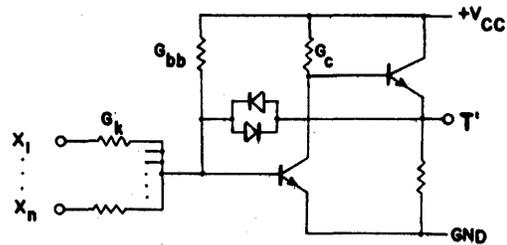
Figure 4—Collector biasing and emitter follower output.
