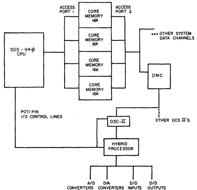
Figure 5—Connection of hybrid processor to SDS-940
