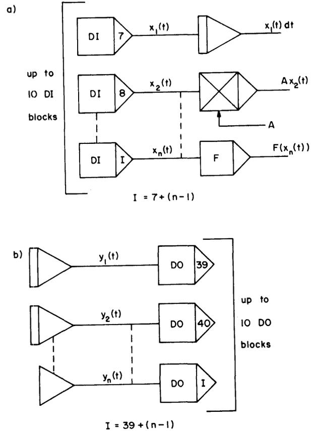
Figure 17—Disk input and disk output block configurations
