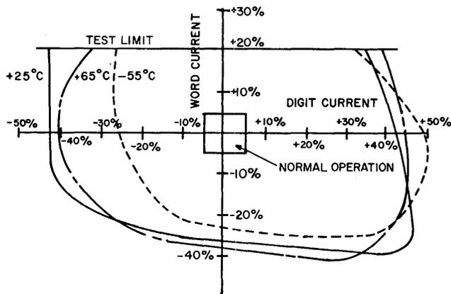
Figure 18—Memory system operating margins
