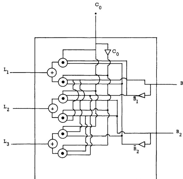
Figure 5b—Cell-K of the input control circuit
