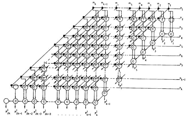
Figure 2—The "single-bit" asynchronous multiplication cellular array
