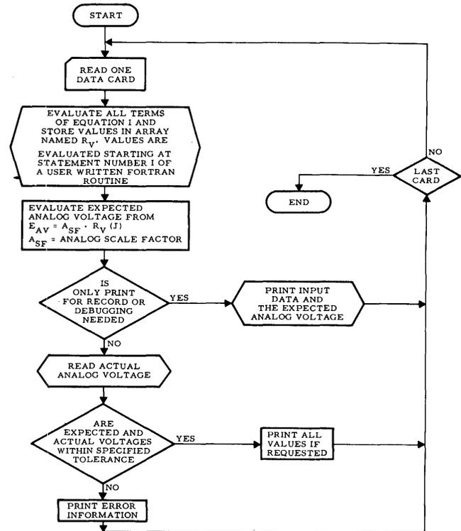
Figure 4—Static check control
