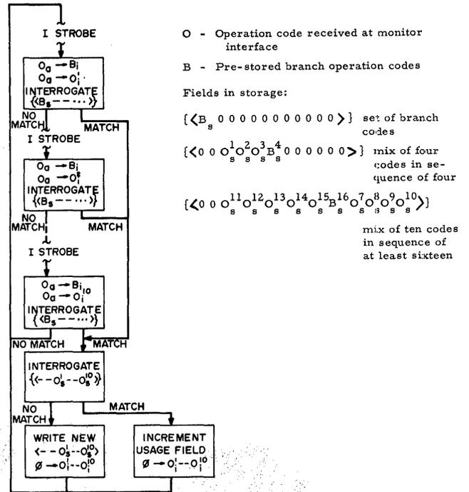
Successive operation codes are placed in successive O fields across the I/E register by means of a string of macroinstructions differing only in the routing
