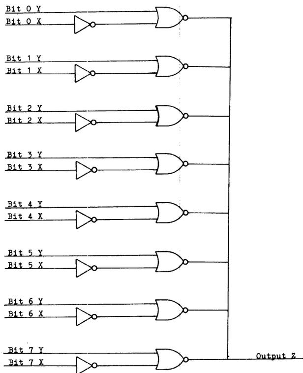
Figure 4—Hardware to test if X is a subset of Y
