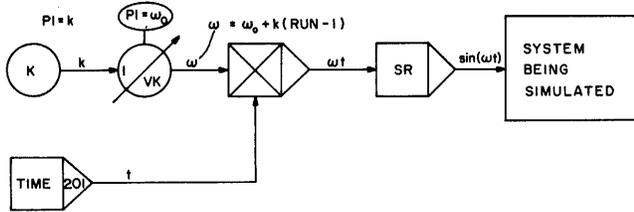
Figure 5—Frequency response implementation through use of the VK element to increment  $\omega$
