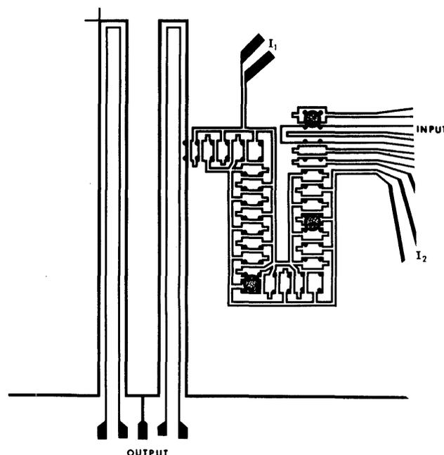
Figure 10—Photograph of the conductor pattern of a unidirectional shift register utilizing a biphasic propagating source. The circuit contains a controlled replicate input and an output circuit which detects a change in flux. Circuit is capable of propagating domains having a nominal diameter of 4 mils
