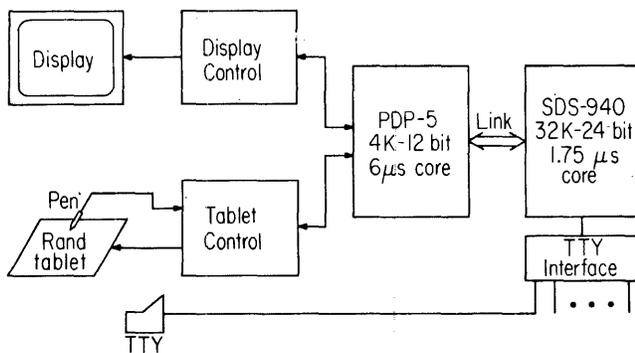
Figure 1—Hardware used in recognition research
