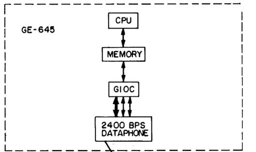
(THIN LINES REPRESENT DATA TRANSMISSION; HEAVY LINES REPRESENT TRANSMISSION OF STATUS INFORMATION AND INTERRUPTS)
