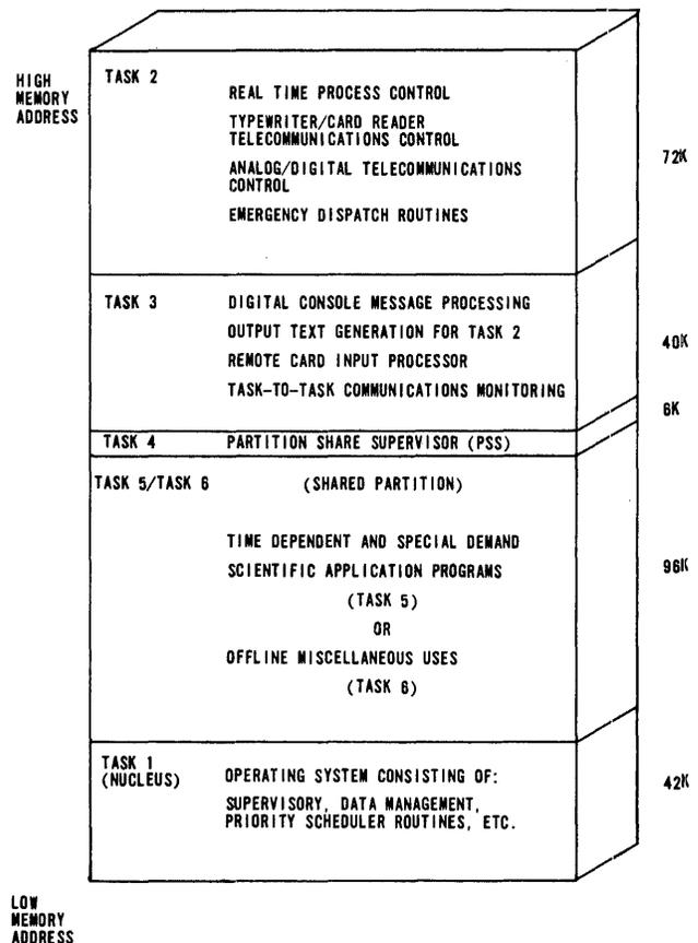
Figure 1—Initial memory configuration with task functional descriptions and relative locations shown
