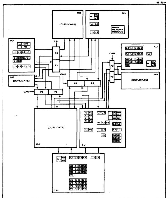
Figure 17—MCB-Modular computer breadboard block diagram
