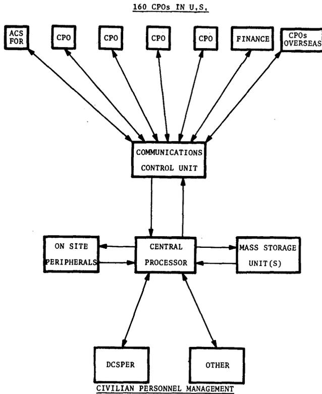
Figure 2—Single computer configuration data input and output
