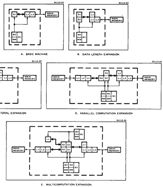
Figure 14—Four stages of expandability
