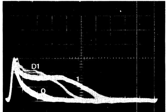
Figure 7—Superimposed outputs of 32 elements (zero, one and disturb one)
