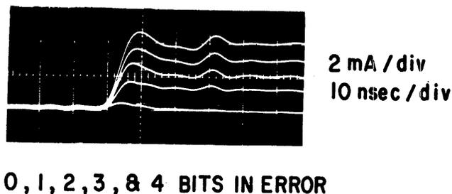
Figure 11—Analog mismatch signal
