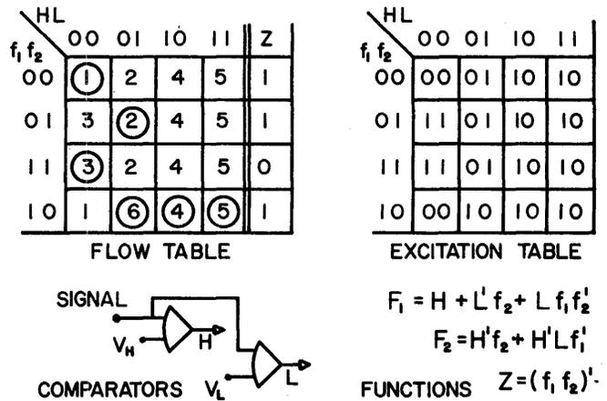
Figure 2—Pulse-height detector — Description
