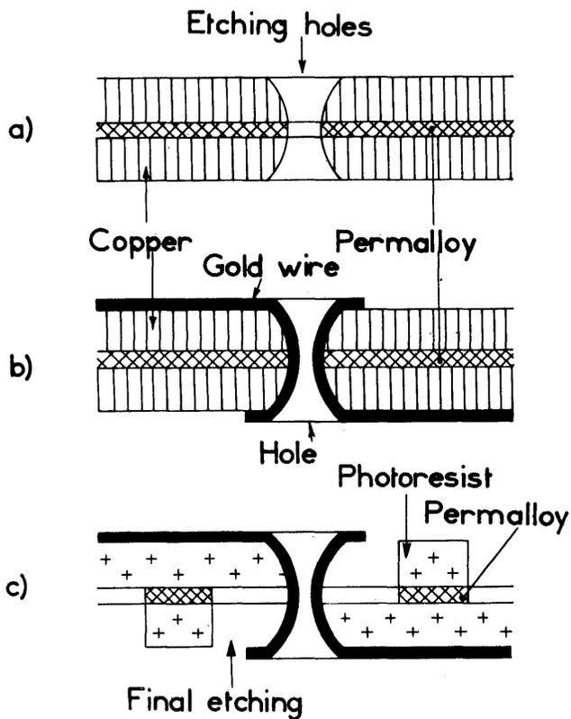
Figure 4—The new fabrication process: cross sectional view
