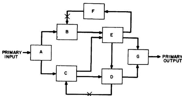
Figure 3a—Functional modules of a processor an example
