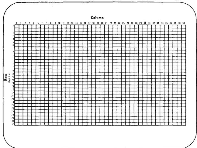
Figure 2—This shows the organization of the screen into 32 rows and 40 columns forming 1280 addressable units. The standard alphanumeric characters occupy two of these boxes, i.e., two rows by one column
