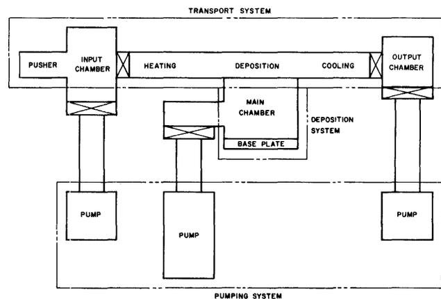
Figure 10—Continuous vacuum evaporator
