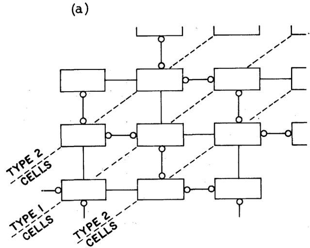
Figure 9a—Alternating type 1/type 2 cells in the multiplier matrix
