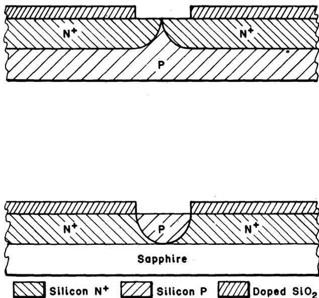
Figure 3—Diffusion failures in bulk silicon and silicon-on-sapphire
