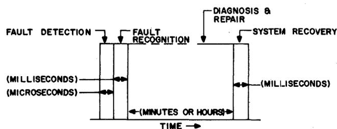
Figure 1—Fault recovery sequence (without spare)
