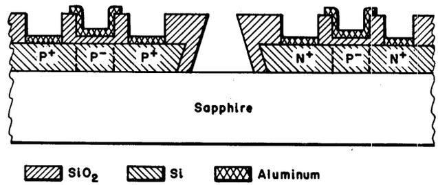
Figure 6—Final device structure
