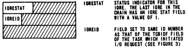
Figure 7—I/O request element (IORE)
