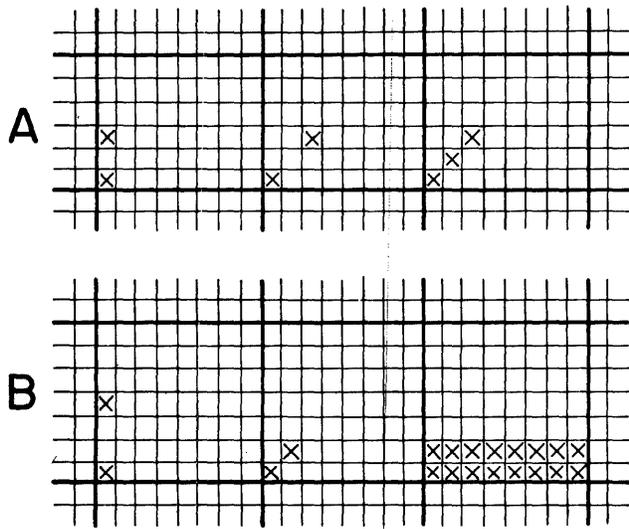
Figure 8—(A) shows three dot patterns which permit light pen detection; (B) shows three dot patterns which would not be detected by the light pen
