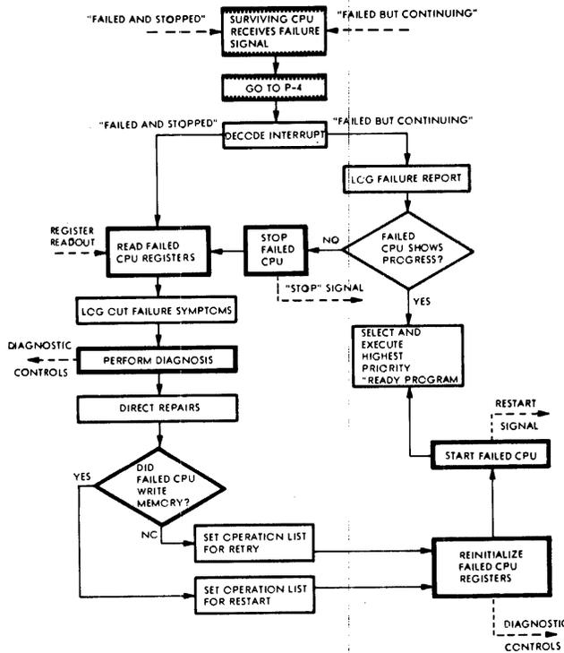
Figure 7— Central processor error: Surviving CPU
