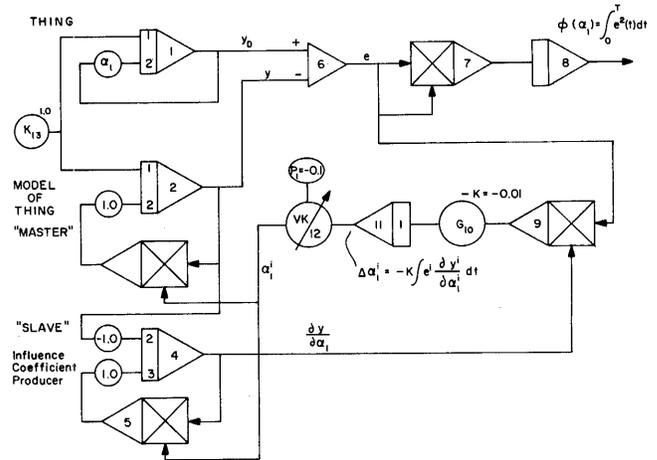
Figure 6—MOBSSL block diagram demonstrating use of VK block as iterative element in parameter search by discrete sensitivity difference equation technic
