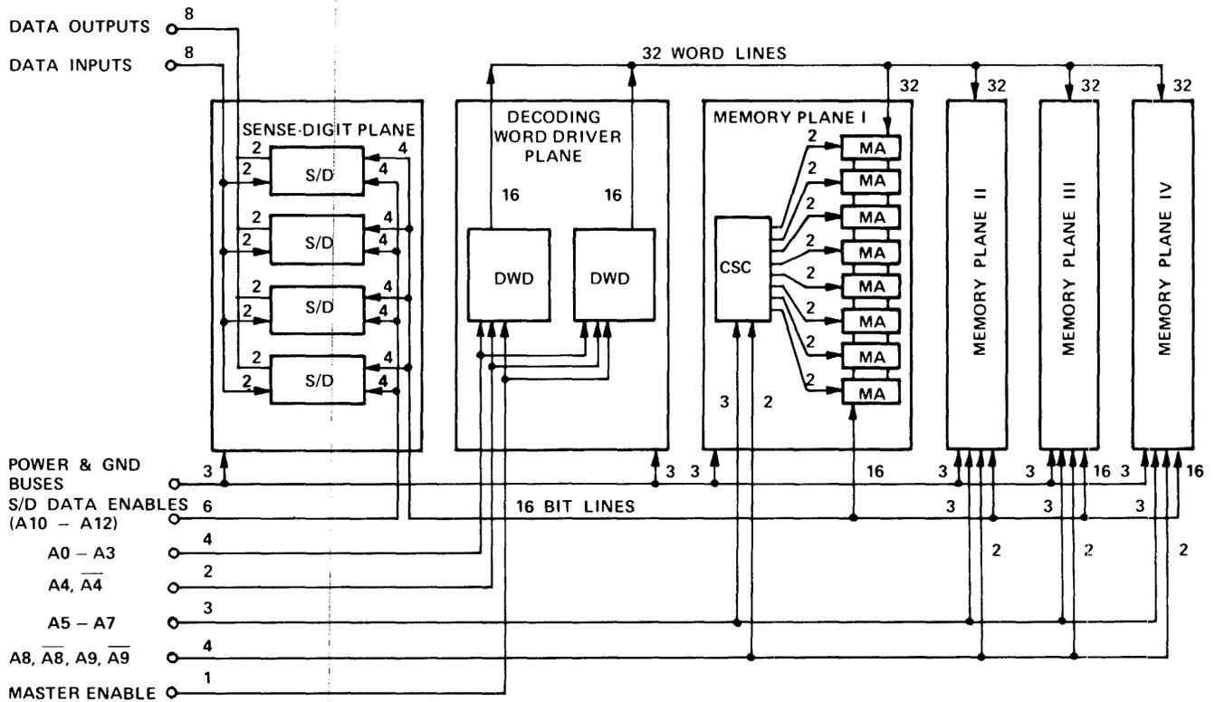
Figure 13—8192 bit memory stack-electrical organization
