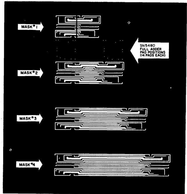
Figure 11—Four relocation patterns for SN5480's
