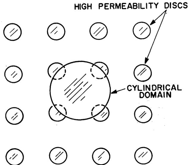
Figure 5—Interaction between a matrix of high permeability disks and a cylindrical domain
