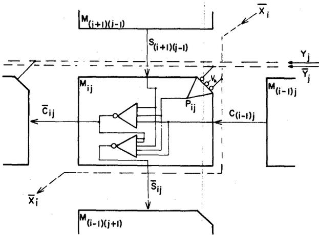
Figure 6—Functional multiplier cell
