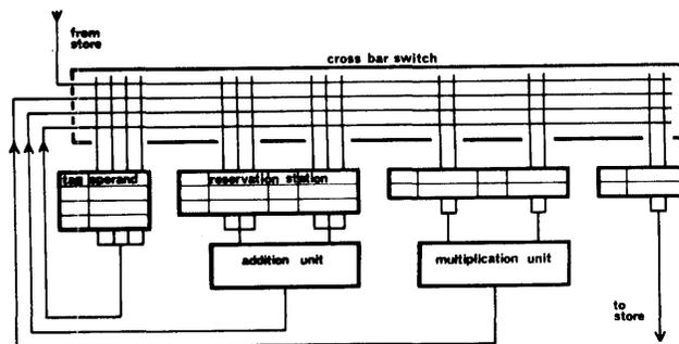
Figure 5—Typical floating point unit for use with Tomasulo's algorithm
