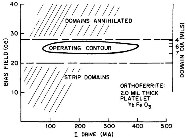
Figure 7—Quasi-static operating contour for 2.0 mil thick platelet of  $YbFeO_3$ .
