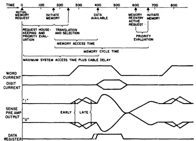
Figure 17—Timing for a typical memory cycle
