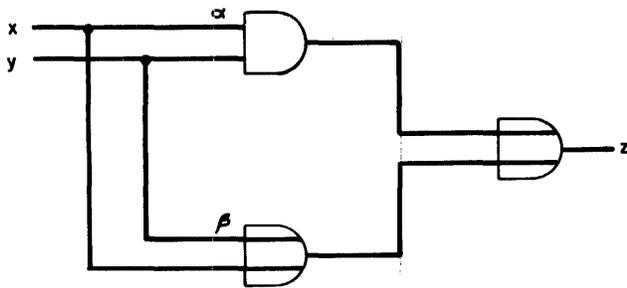
Figure 6—Example of a redundant circuit
