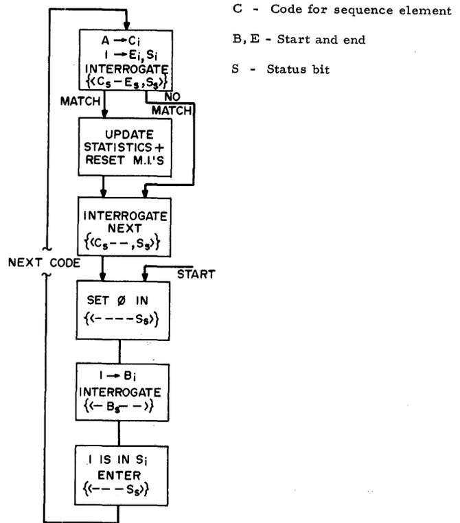
Initially, and at the end of each cycle, the status bits are set to one for all first elements.
