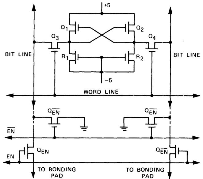
Figure 3—Storage cell circuit schematic
