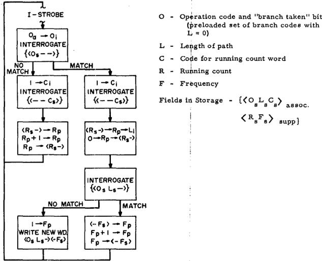
Each instruction strobe initiates a test to find if a branch was taken for one of the prespecified operation codes. These need not be the entire set of the host computer.
