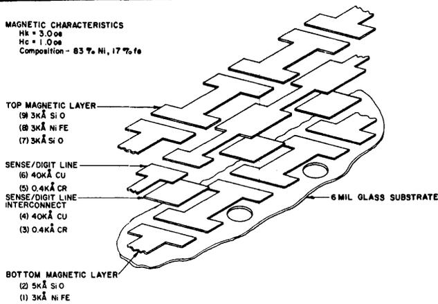
Figure 1—Storage element (exploded view)
