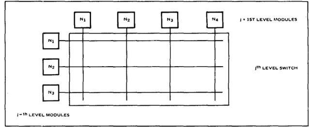
Figure 3—Module-switch-module relationships
