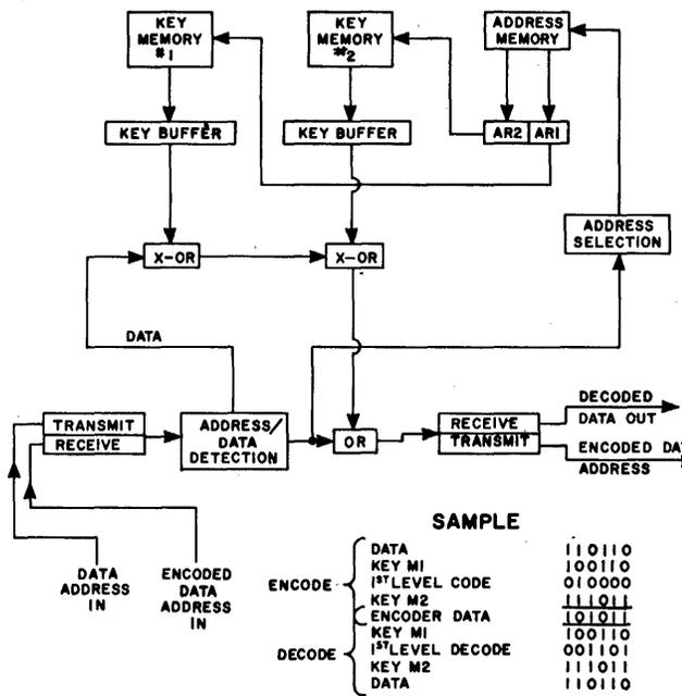
Figure 1—Digital substitution logic
