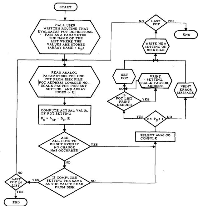
Figure 3—Potentiometer setting control
