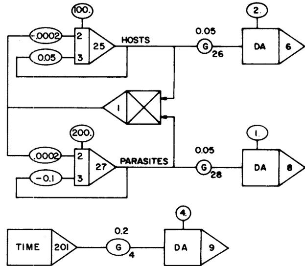
Figure 13—MOBSSL block diagram for the host-parasite problem
