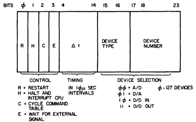
Figure 3—Hybrid processor commands
