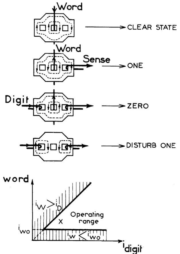
Figure 2—Operation of the three hole element
