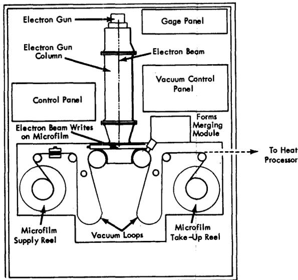
Figure 6—Electron beam recording on microfilm
