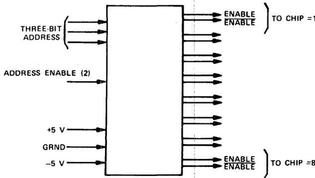
Figure 5—Chip select circuit
