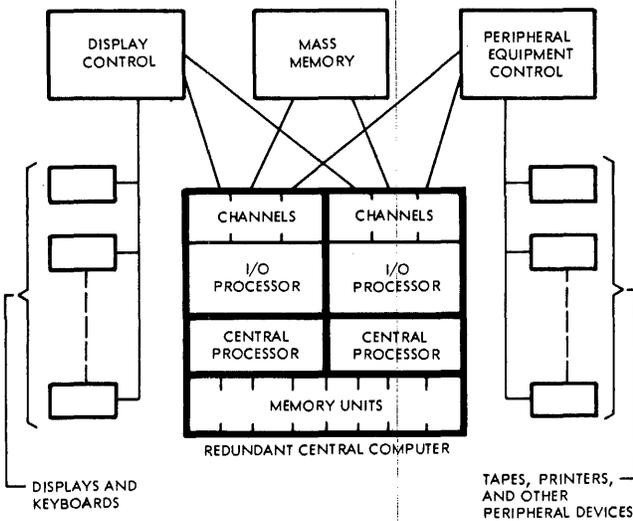
Figure 1—Typical multiprocessor application
