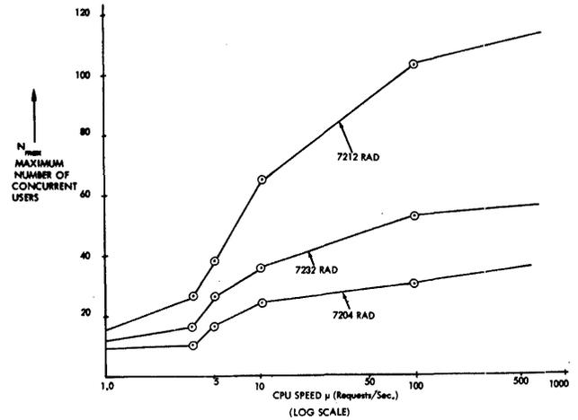
Figure 4— $N_{max}$  vs. CPU speed  $\mu$
