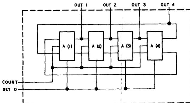
Figure 2—Four bit ring-counter
