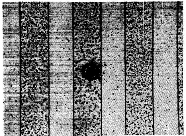
a-2. Enlargement showing self-healed pinhole
