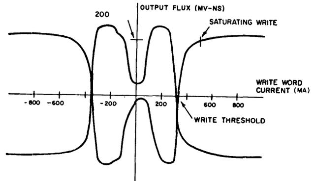
Figure 6—Output flux vs. write word current
