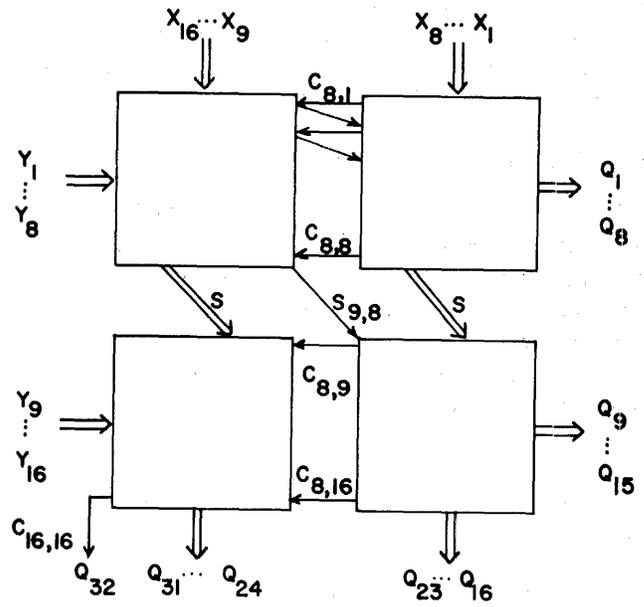
Figure 7—16 × 16 bit functional multiplier on four LSI dies
