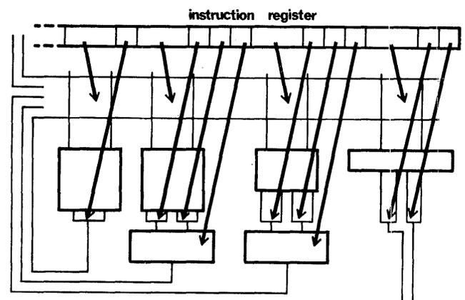
Figure 8—Control for the floating point arithmetic unit
