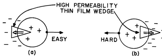
Figure 12—Domain positioned on a wedge-shaped high permeability permalloy thin film. The domain is more easily moved off the point of the wedge (a) than the blunt edge (b)
