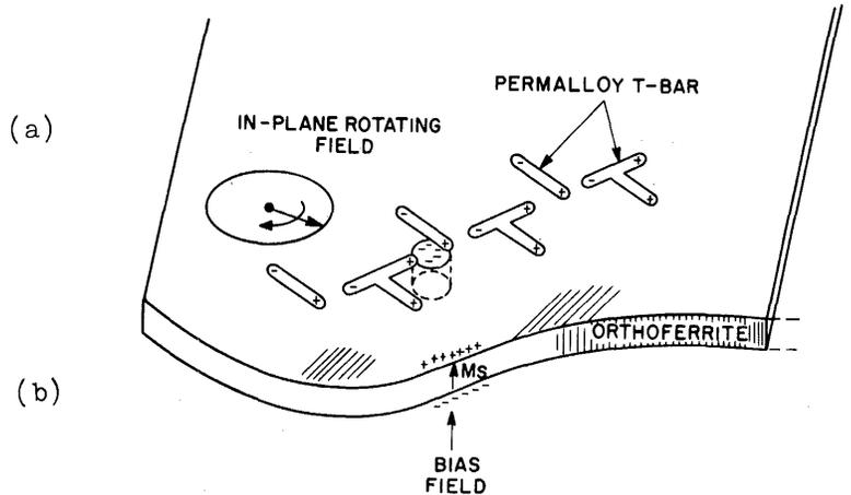
Figure 14—Isometric view of permalloy T-BAR pattern in contact with surface of orthoferrite platelet. Rotating in-plane field generates poles which cause the domain to move
