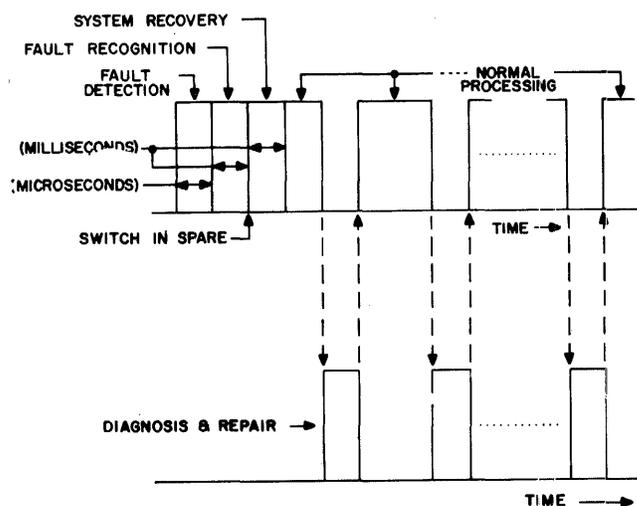
Figure 2—Fault recovery sequence (with spare)
