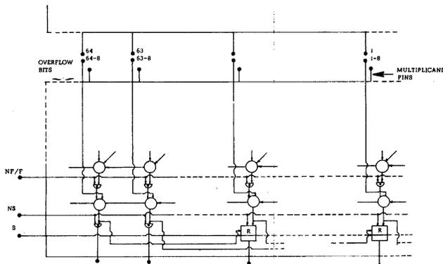
Figure 9—The combinational logic gating for reconfiguration
