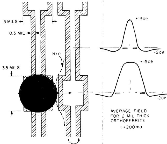
Figure 6—Conductor circuit used to propagate cylindrical domains and the resulting field profiles for 200 mA applied current
