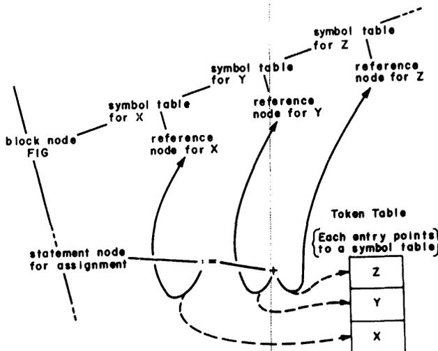
Figure 6—The internal representation of a statement before and after the execution of the search function. The broken lines show the statement's operands before the search
