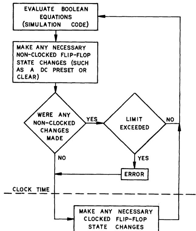
Figure 4—Simulator controller
