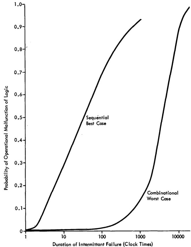
Figure 4—Sensitivity of multiply/divide logic
