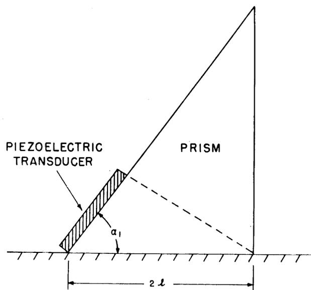
Figure 1—Surface wave radiator/sensor
