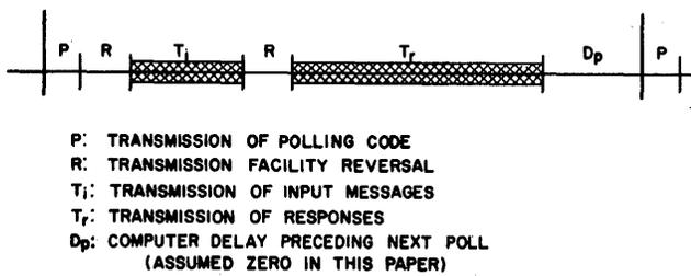
Figure 2A—Typical cycle of operation (Half-duplex message transmission)
