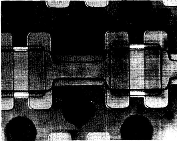
Figure 8—Enlargement of memory array
