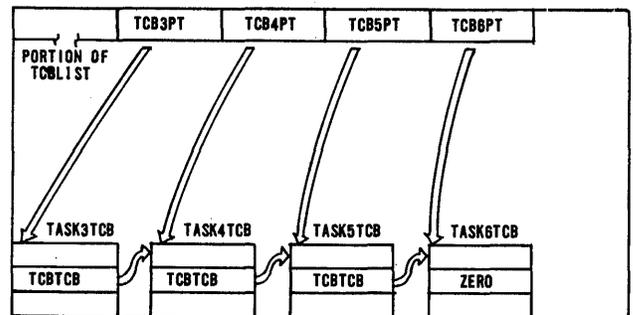
Figure 9—Portion of nucleus showing TCBLIST and TCBTCB pointer relationship prior to modification
