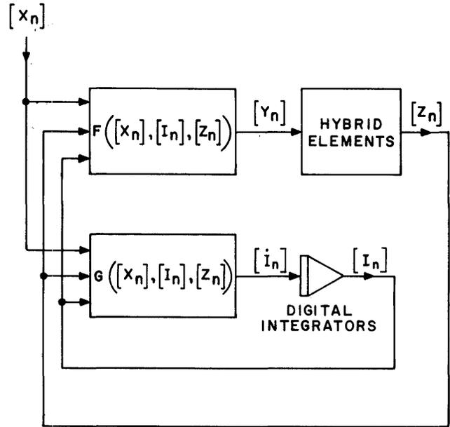
Figure 4—Principle of operation of HYPAC
