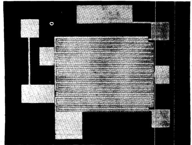
Figure 5—Breakdown strength of oxides in a multilayer test vehicle
