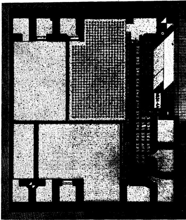
b. Oxide integrity and metallization test vehicle
