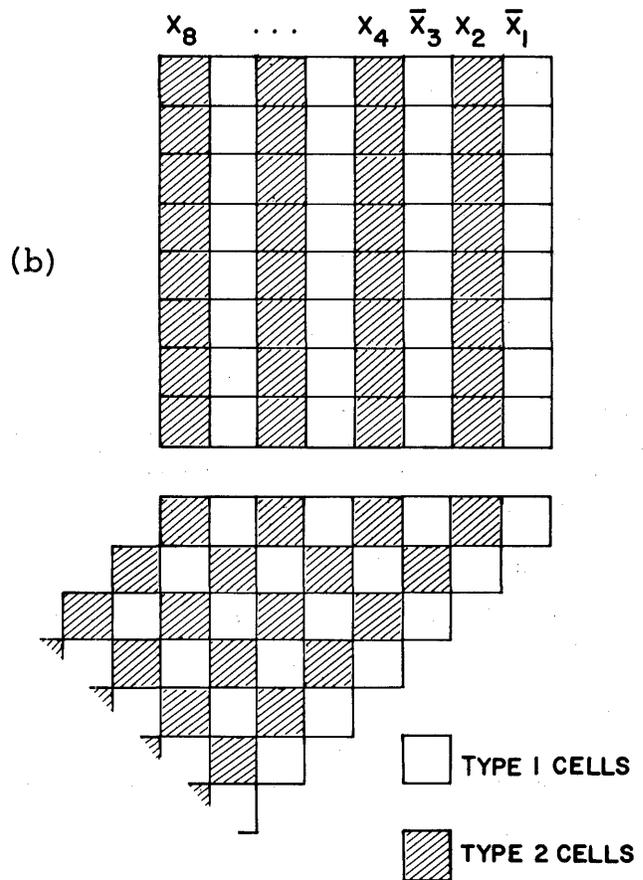
Figure 9b—Alternating columns  $X/\bar{X}$  composed of type 1/type 2 cells
