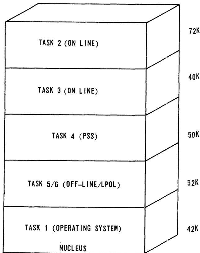
Figure 11—Initial task core allocations
