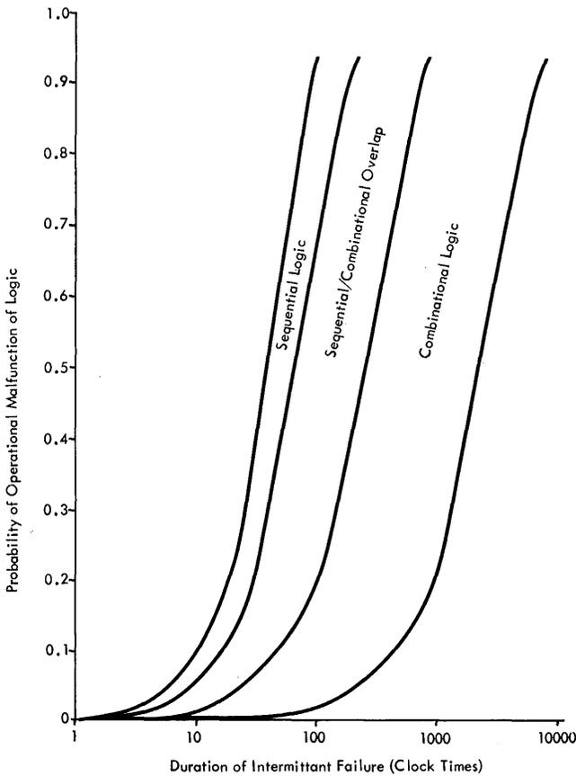
Figure 3—Sensitivity of arithmetic logic
