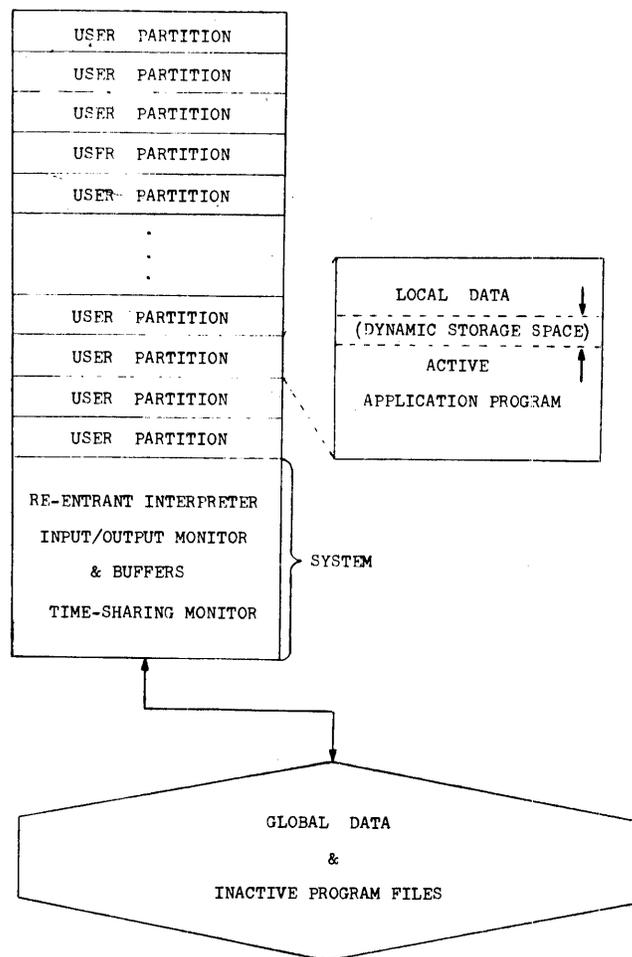
Figure 1—A schematic diagram of the core memory allocation of the MUMPS system and user partitions. A single partition is expanded to show its internal structure. The use of secondary storage (disk) for global data and inactive programs is represented.
