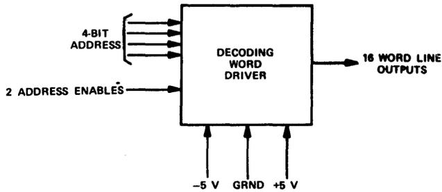
Figure 8—Decoding word driver chip
