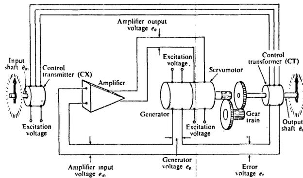
Figure 4—Schematic diagram of motor-generator instrument servomechanism
