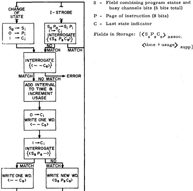
When an instruction strobe initiates a cycle, the monitored bits are routed through the A register to the I/E register for interrogation of associative memory. A match indicates no change of system state and completes the cycle.
