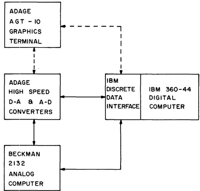
Figure 10—USC system simulation laboratory computer complement
