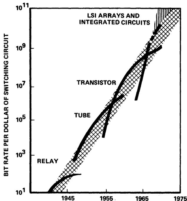
Figure 5—Switching rate per dollar for computer logic elements
