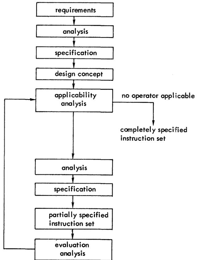
Figure 4—ISDS as a design model
