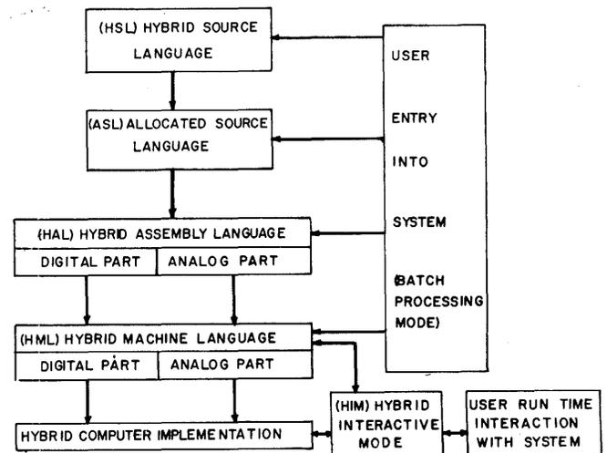
Figure 1—A hybrid computer programming system
