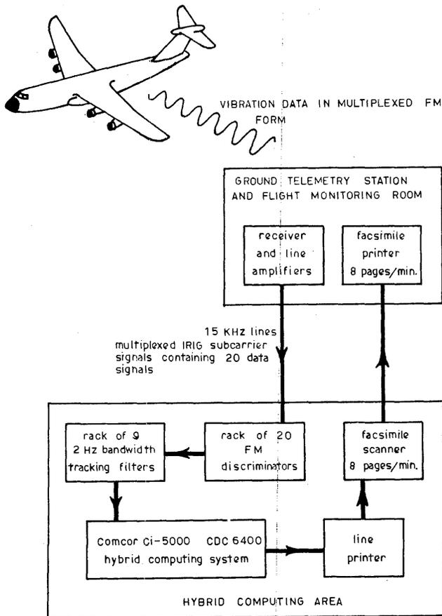
Figure 1—The data reduction system
