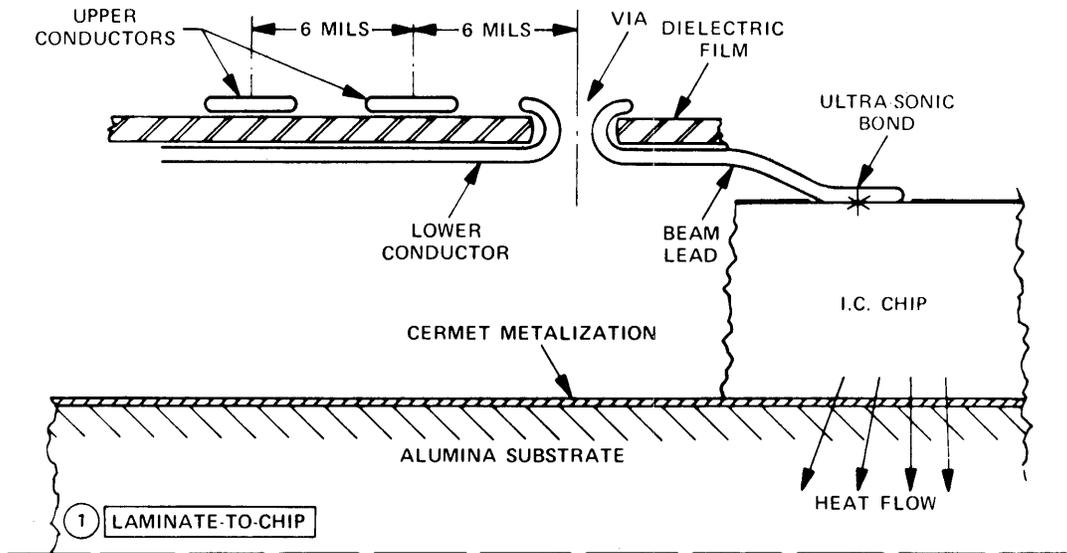
Figure 15—Interconnect cross-section
