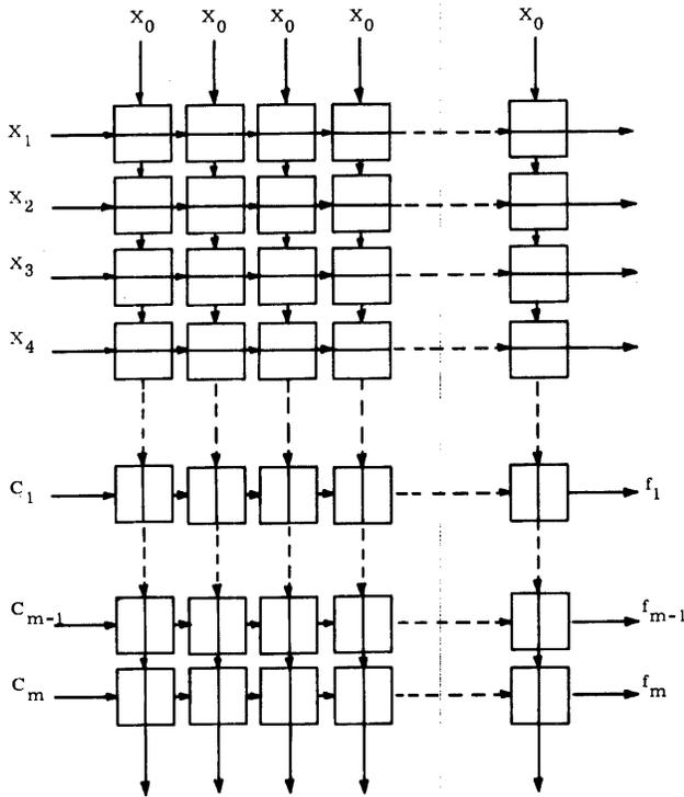
Figure 2—Construction of a testable cellular array
