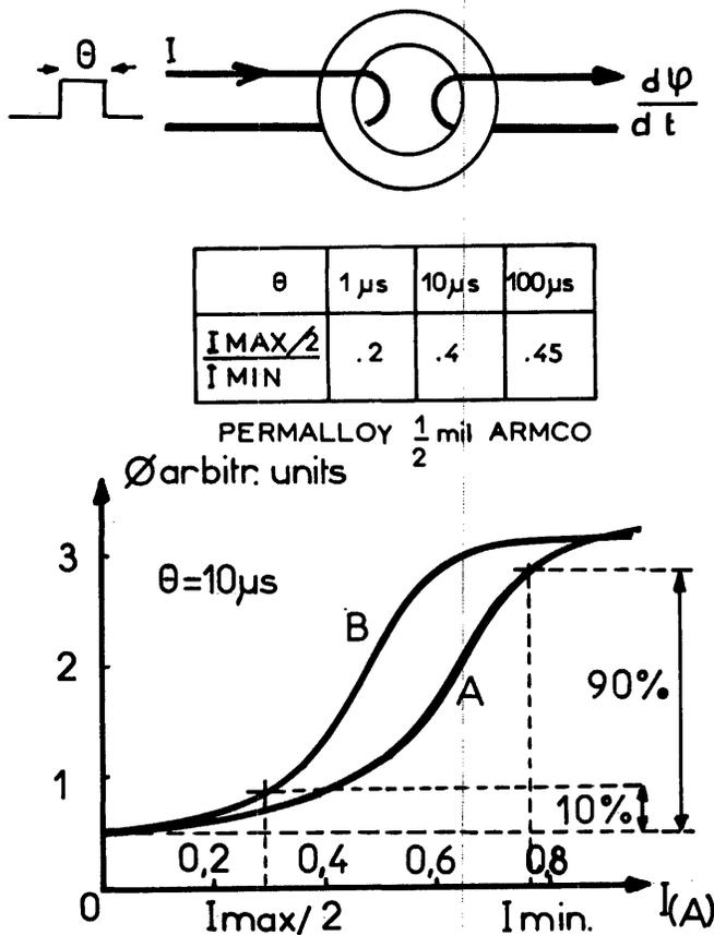
Figure 1—S-curves 1/2 mil thick etched permalloy toroids
