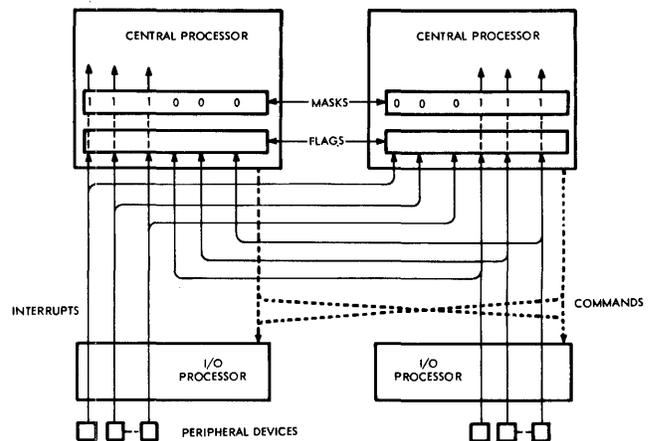
Figure 4—Input-output control block diagram
