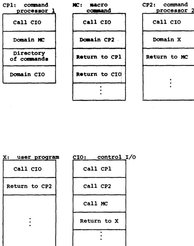
Figure 3a—Switchable control I/O—the domains
