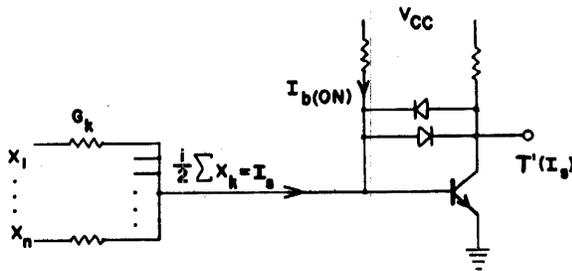
Figure 2—Threshold gate with Schottky diode feedback
