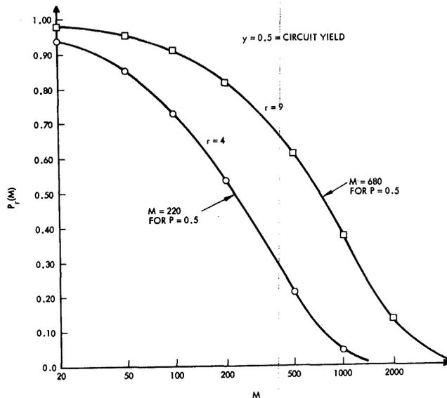
Figure 19—The probability  $P_r(M)$  of successfully fulfilling a master pattern of  $M$  circuits by relocating from one of up to  $r$  nearby circuits. Each circuit is a tested unit which may have many gates of logic complexity
