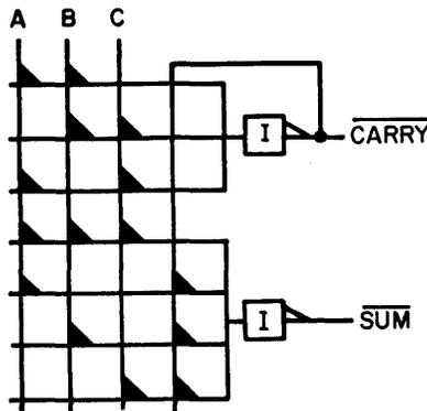
Figure 8—SLT full adder position
