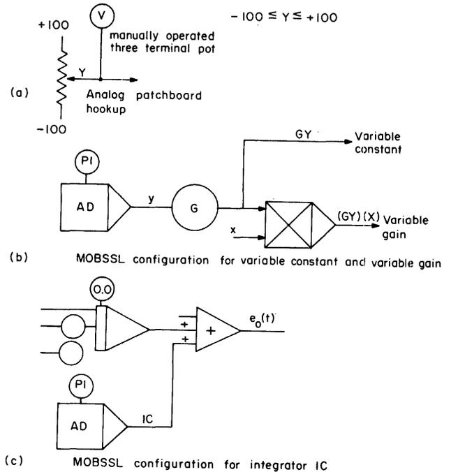
Figure 11—Use of AD element for on-line parameter changes
