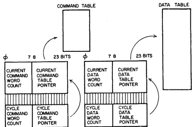
Figure 4—Command and data table structure
