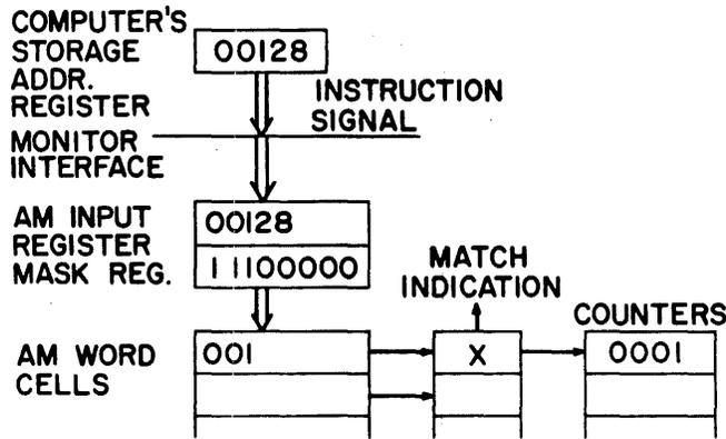
Figure 1—Assignment of counter to initial execution area
