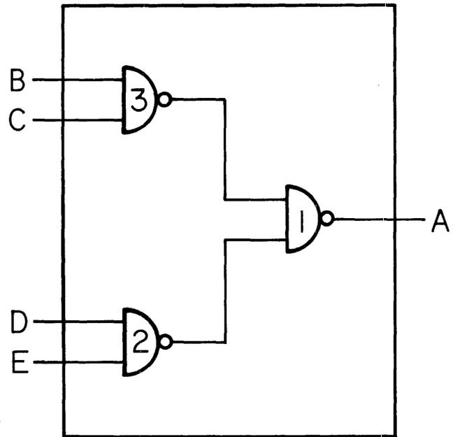
Figure 8—Logic module as defined for partitioning purposes
