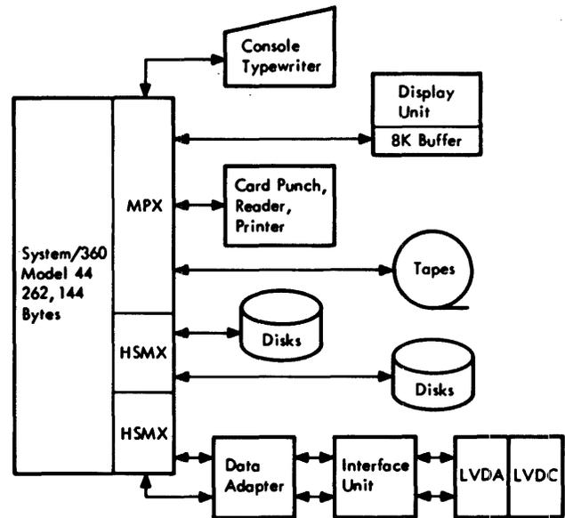
Figure 2—Flight software development laboratory—Block diagram
