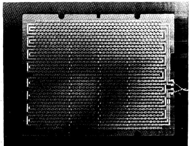
Figure 7—The mated film core array
