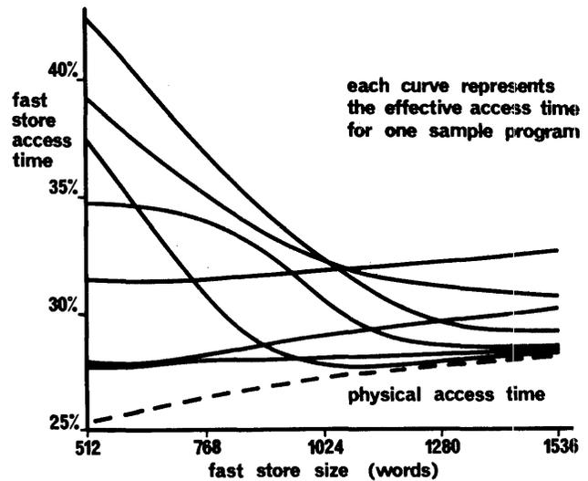
Figure 2—The physical access time of a fast store (broken line) and the effective access times (continuous lines) for sample programs. Access time is a percentage of main store access time, storage size is in words, and line size is 4 words
