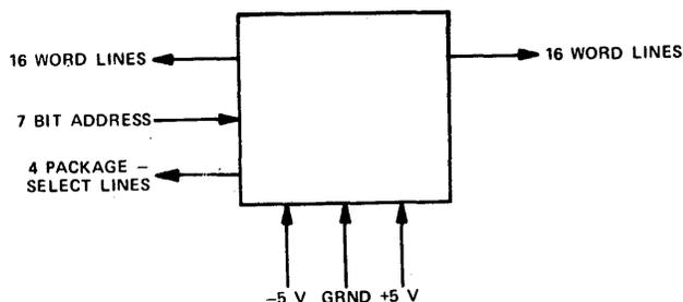
Figure 10—Decoding word driver package
