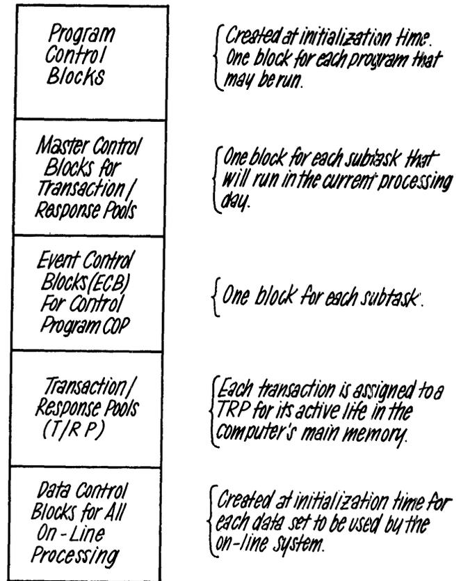
Figure 4—Control blocks for on-line processing
