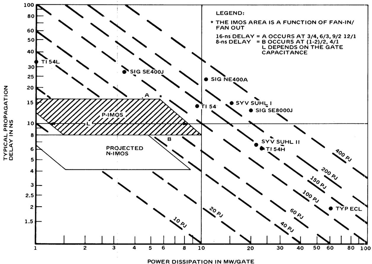
Figure 7—Speed-power products of some bipolar and MOS circuits
