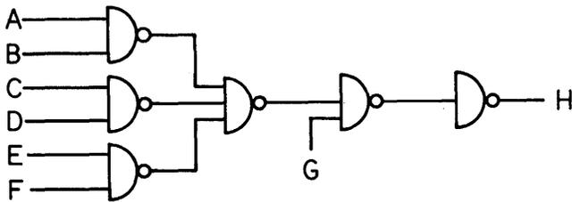
Figure 5b—NAND equivalent for H (without strapping)
