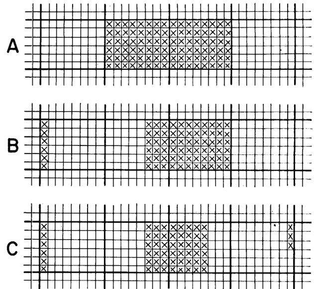
Figure 7—This shows the problem of erasure with multiple display inserts on the same row. The insertion of the single dot column in (B) causes erasure of 5 dot columns from the original pattern in (A). Insertion of the 1/2 dot column in (C) causes erasure of 3 dot column from the original pattern
