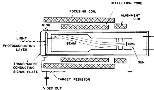
Figure 2—Schematic cross-section of the vidicon
