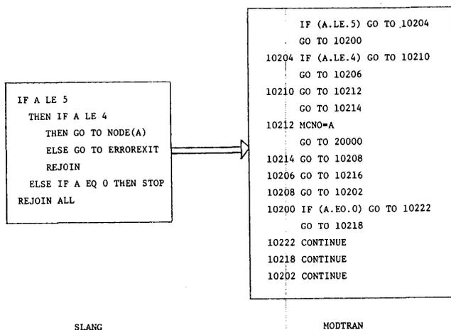
Figure 5—Example of SLANG/MODTRAN conversion
