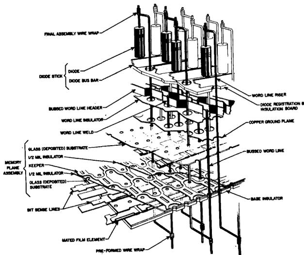
Figure 12—The substack
