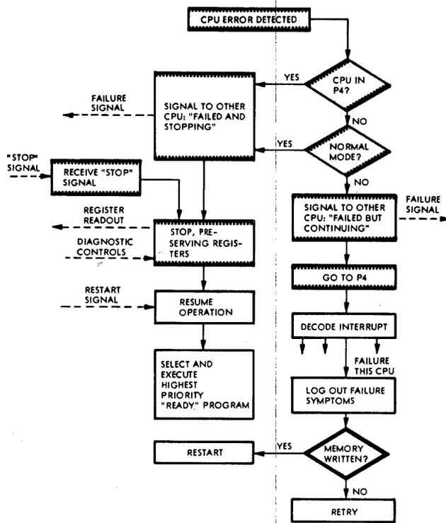
Figure 6—Central processor error: Failed CPU
