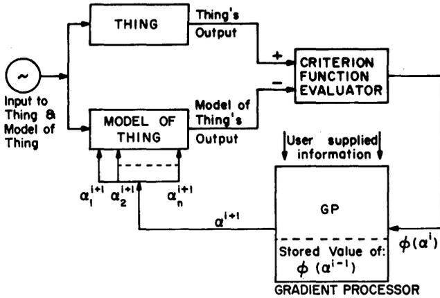
Figure 1—Application of the gradient processor element to parameter identification
