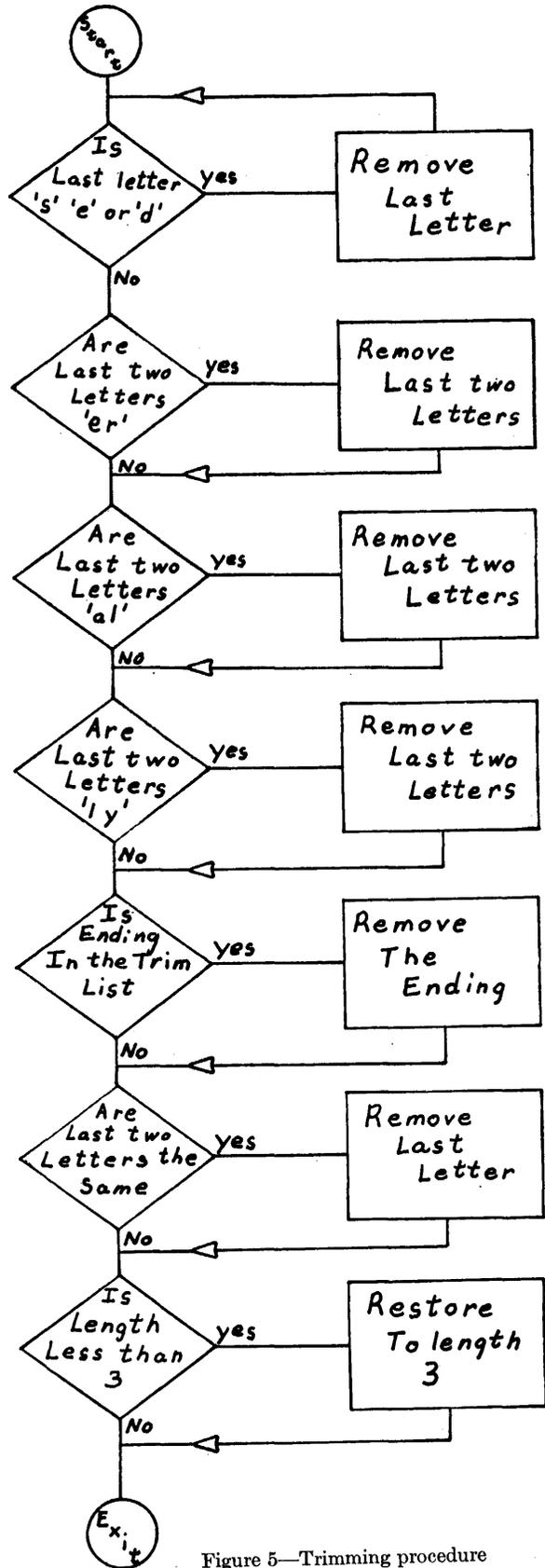
Figure 5—Trimming procedure
