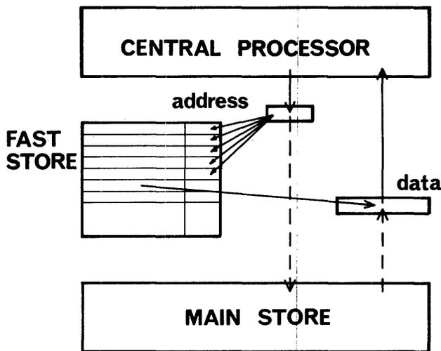
Figure 1—The use of an associative fast store to reduce the access time of the main store
