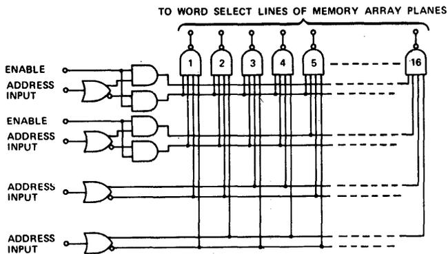
Figure 9—Decoding word driver chip logic
