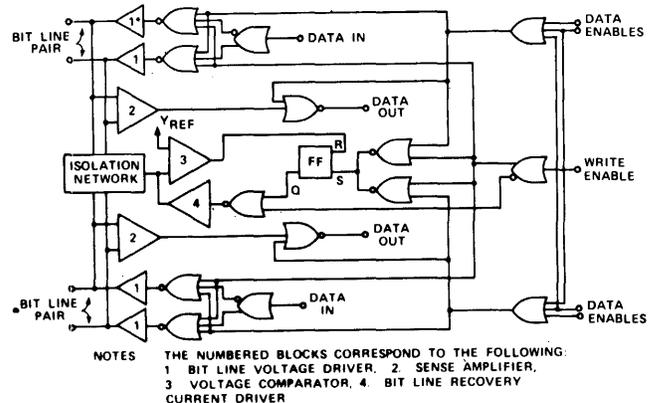
Figure 11—Sense amplifier/digit driver chip logic
