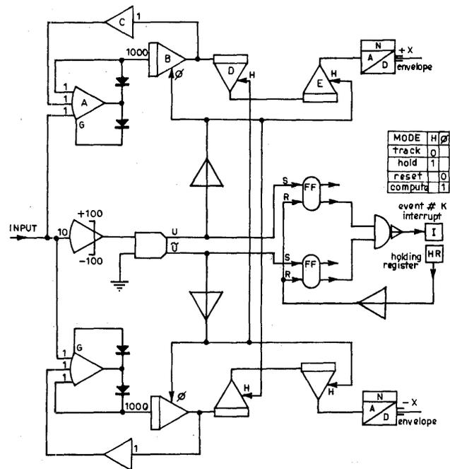
Figure 4—The envelope detection circuit
