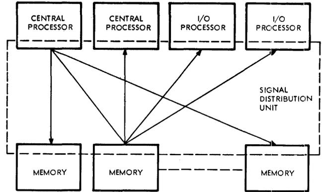
Figure 2—Fail-soft computer configuration
