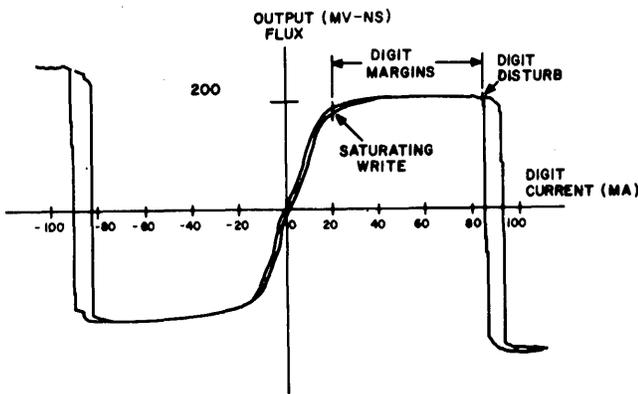
Figure 5—Output flux vs. digit current
