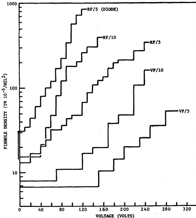
b. Pinhole density for silane-vapor-plated and R-F sputtered  $\text{SiO}_2$  on delineated aluminum 5,000 Å and 10,000 Å thick
