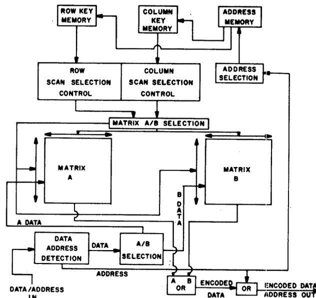
Figure 3—Digital route transposition matrix
