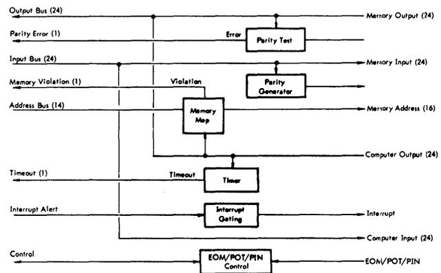
Figure 5—Interface structure
