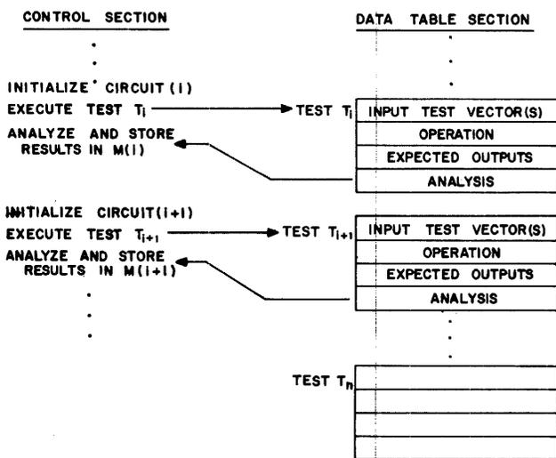
Figure 7—Layout of a diagnostic program structure
