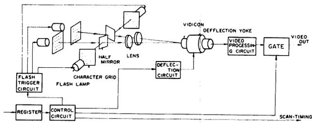
Figure 1—Schematic diagram of the character generator
