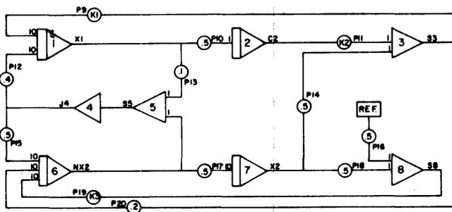
Figure 2—Simulation of an automobile suspension system
