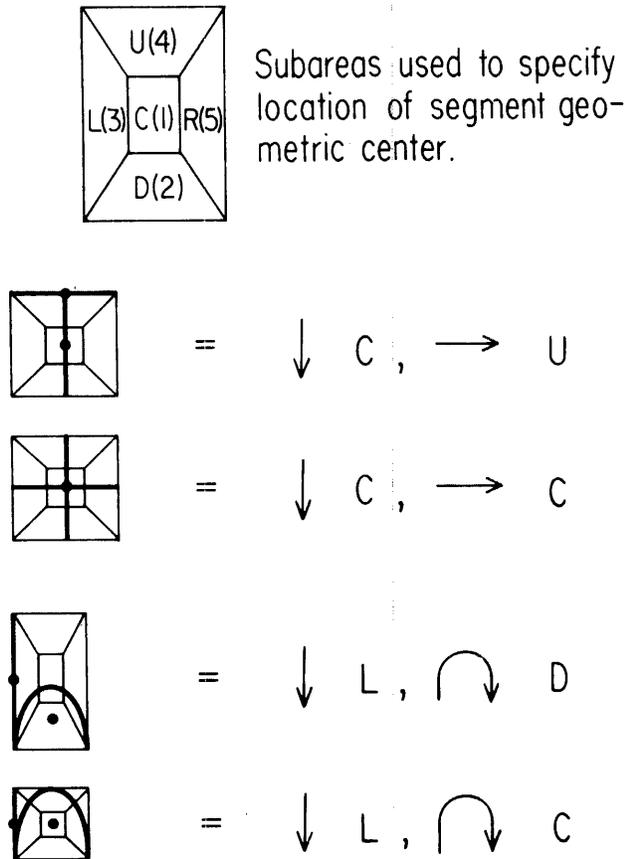
Figure 12—Geometric position of segments
