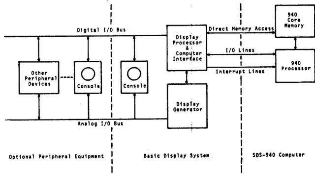
Figure 1—System configuration
