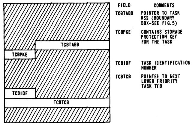
Figure 3—Task control block (TCB)
