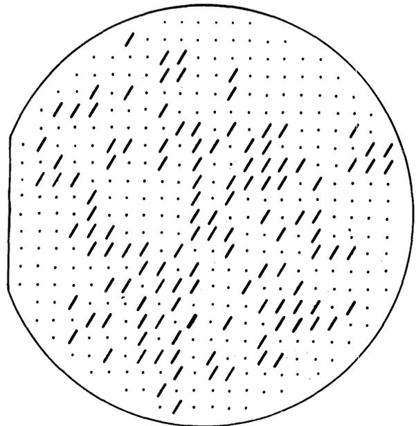
Figure 2—Wafer after test—Slashes show good circuit positions
