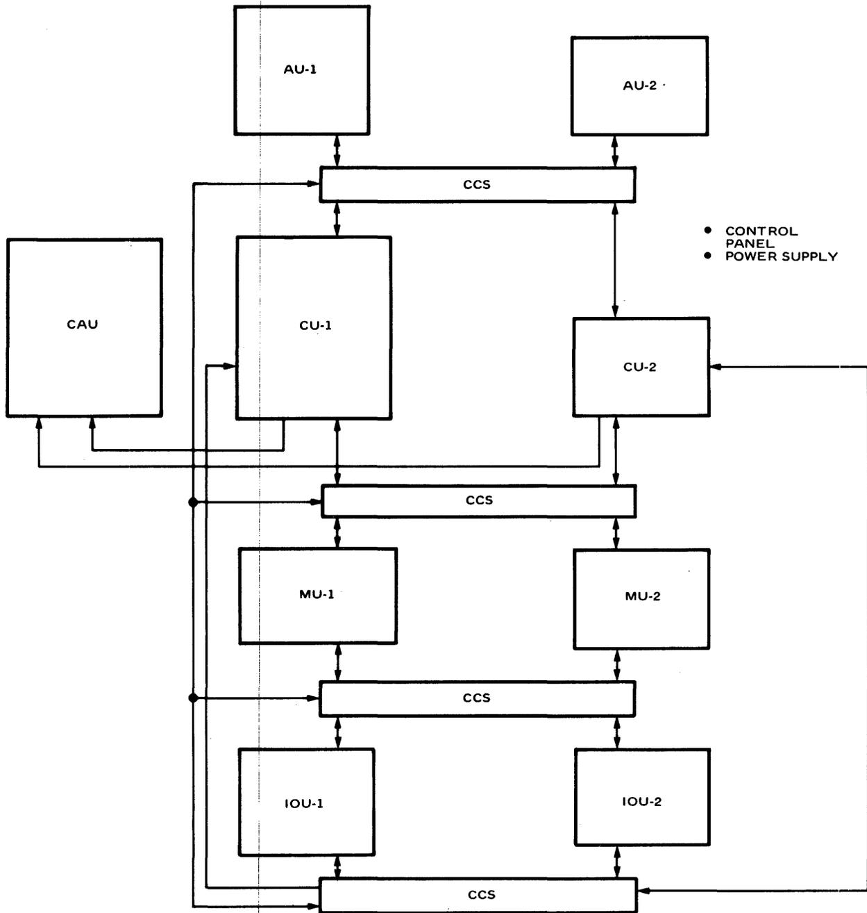
Figure 5—Block diagram of existing modular computer breadboard overlaid with the character implementation shown in Figure 6.
