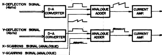
Figure 5—Block diagram of the deflection circuit
