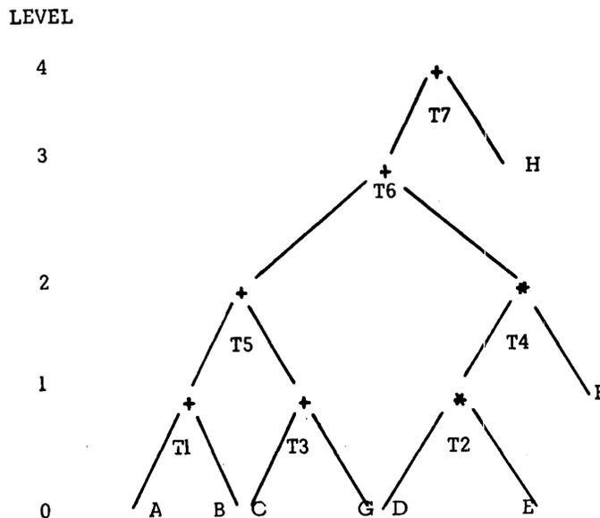
Figure 13—Parallel computation of A+B+C+D\*E\*F+G+H using Baer and Bove't's algorithm
