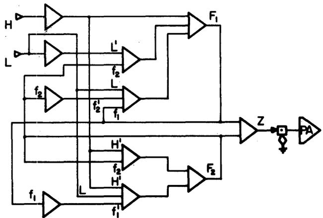
Figure 3—Pulse-height detector — Logic diagram
