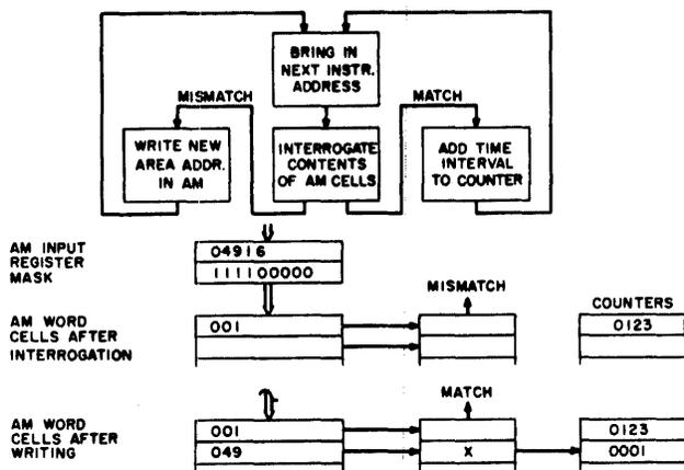
Figure 2—Assignment of next counter to next execution area
