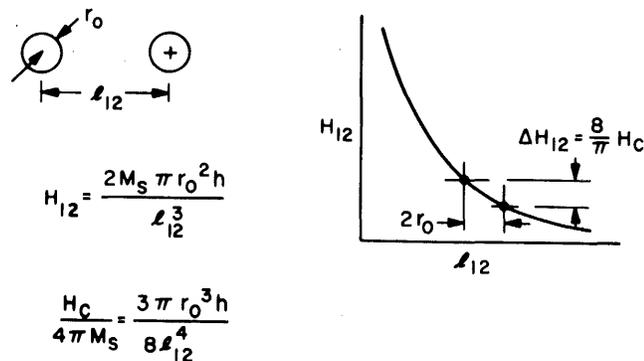
Figure 4—Two domains, mutually repelled in a material whose coercive force is  $H_c$ , reach a stable separation  $\ell_{12}$ .
