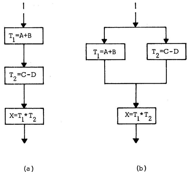
Figure 3—Illustration of parallelism within a compound task
