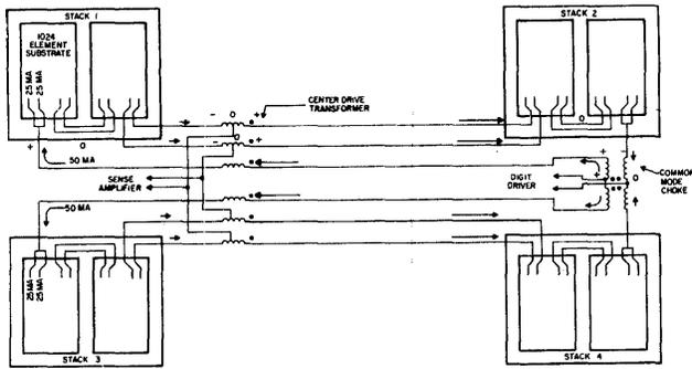
Figure 15—Sense/digit line configuration
