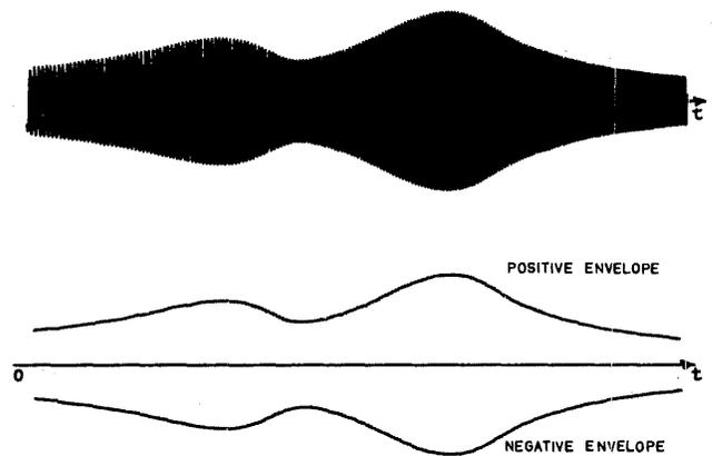
Figure 3—Typical data signal and the computer generated envelopes
