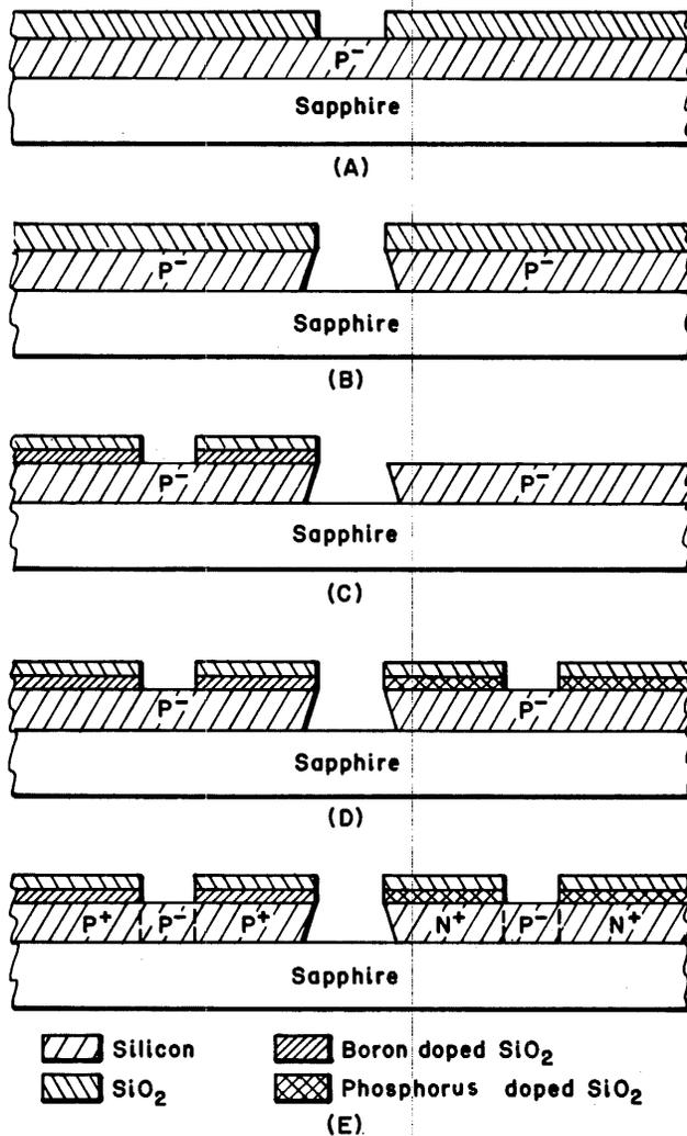
Figure 5—Low temperature CMOS Process
