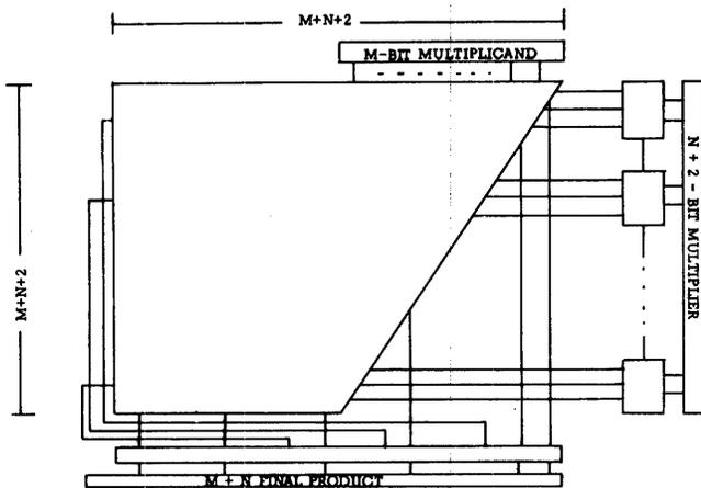
Figure 4—The modified “two bit” multiplier
