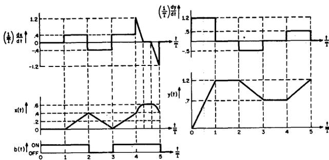
Figure 7—Composition of CRT deflection and beam waveforms
