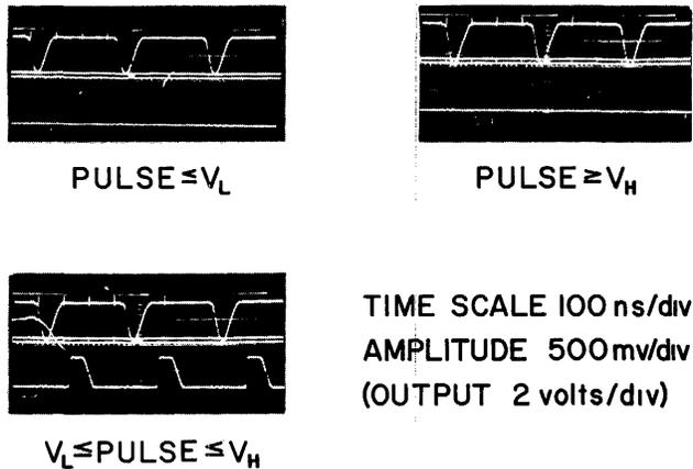
Figure 4—Pulse-height detector — Performance
