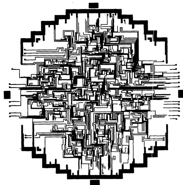
Figure 17—5-bit modular multiplier standard interconnect mask
