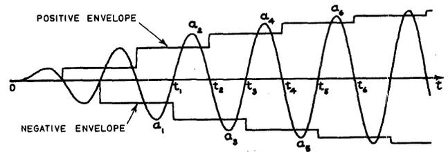
Figure 2—Data signal showing envelopes and zero crossings
