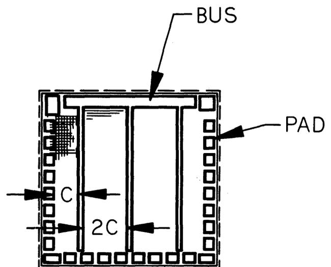
Figure 9—Typical chip layout
