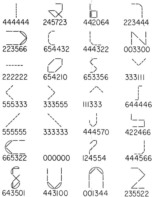
Figure 6—Segments used to print teletype symbols
