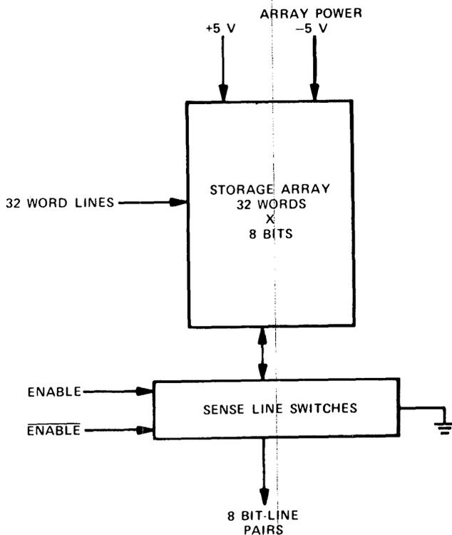
Figure 2—Block diagram MOS storage array
