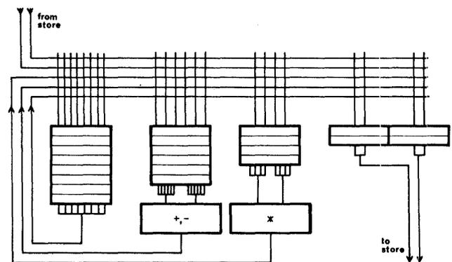
Figure 7—Detail of the floating point arithmetic unit
