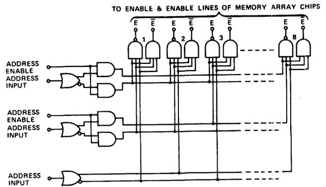
Figure 6—Chip select circuit logic
