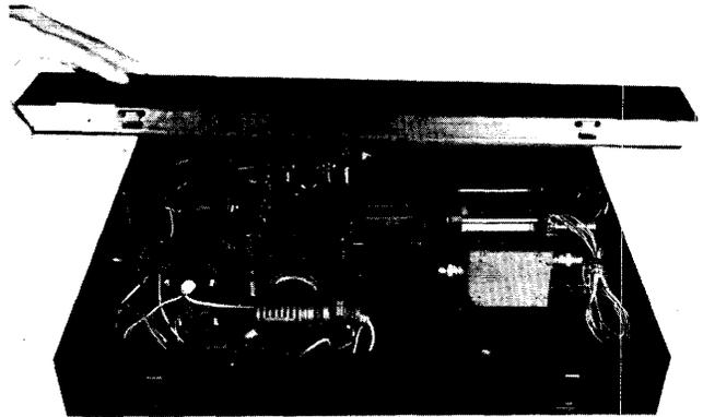
Figure 6—The optical unit of character generator
