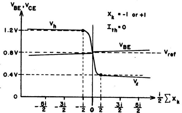
Figure 3—Transfer function of the gate shown in Figure 2
