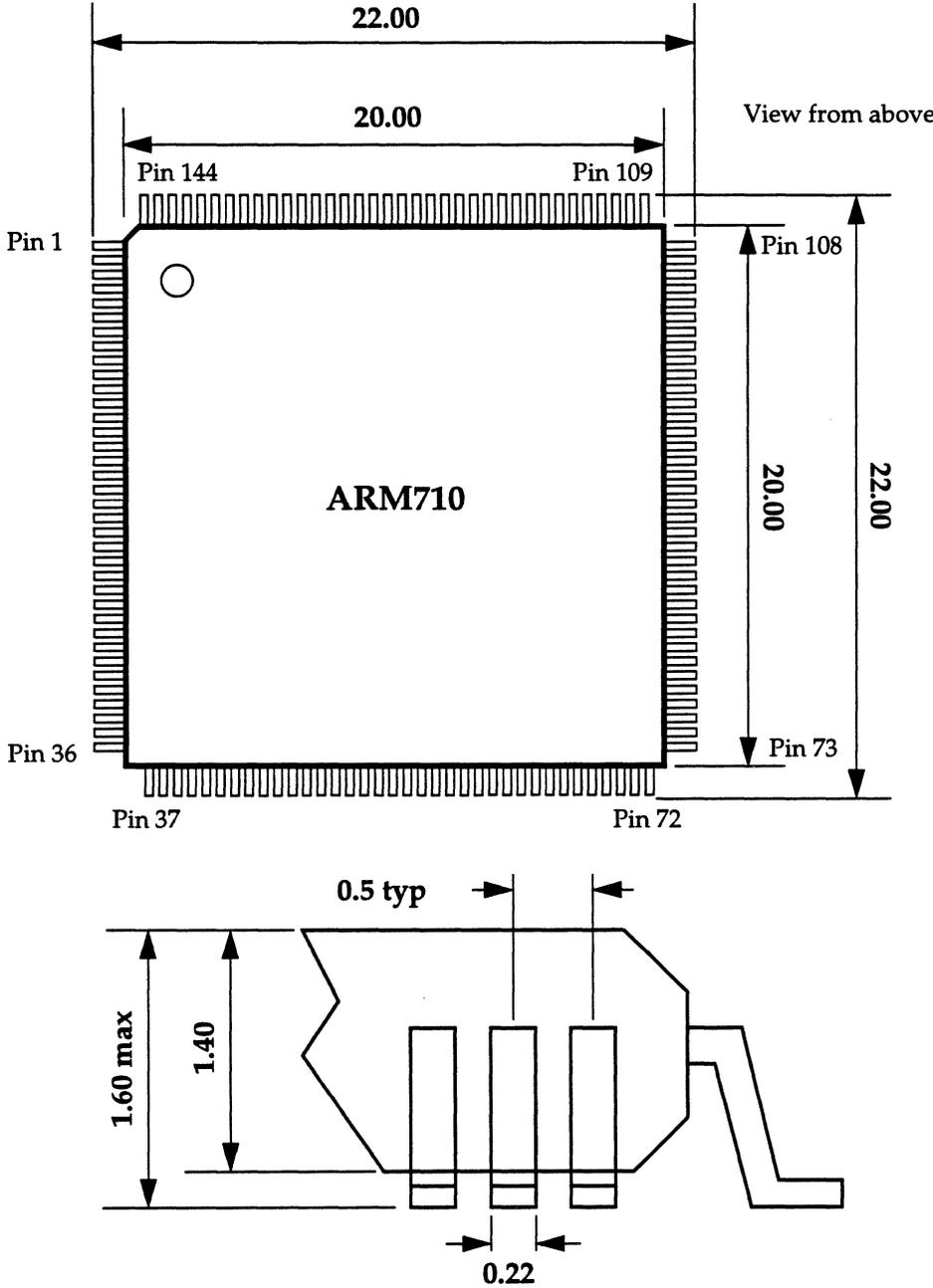
Figure 62: ARM710 144 Pin TQFP Mechanical Dimensions in mm
