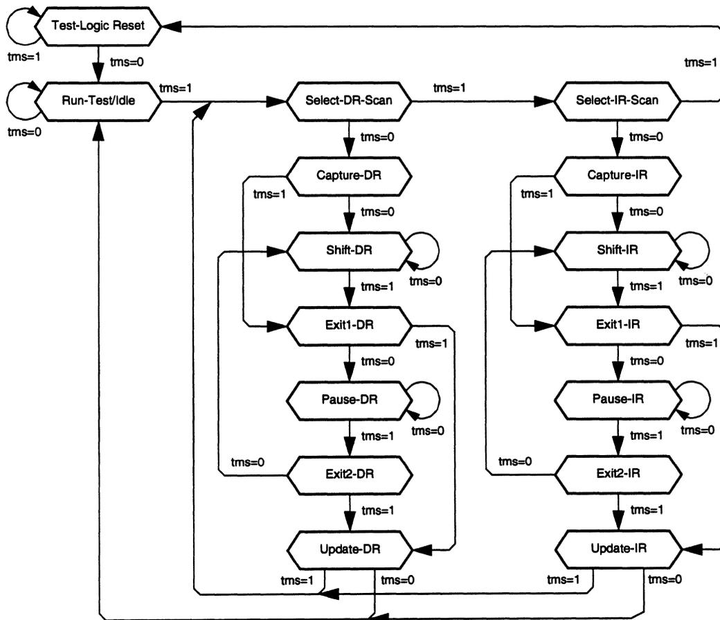
Figure 52: Test Access Port (TAP) Controller State Transitions
