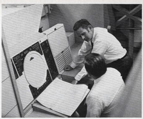
Surveillance radar shelter mock up for Air Force Electronic Systems Division tactical air control system AN/TPN-19 shows position of display console and control equipment. New system being developed by Raytheon Company's Equipment Division, Wayland, Mass., will be used by the Air Force to meet requirements of all weather landings at tactical military airfields.
