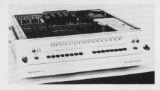
Raytheon Co. will introduce the Multiverter III® instrument, an addition to its line of multiplexed analog-to-digital converters, at the SJCC. Manufactured by the company's Computer Operation in Santa Ana, Calif., the new converter, designated Model MADC15, will operate at a throughput rate of 100 KHz with 15-bit resolution.
