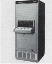
Datacraft's DC 6024/3 was designed for use in applications requiring real-time control and complex calculations.
