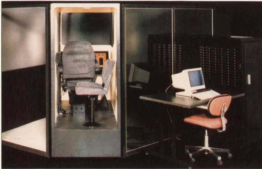
At the center of the TT150 Truck Driving Simulator is a mock-up of an actual truck cab—complete with seat, steering wheel, clutch, gear-shift lever, and all the gauges found in a typical truck. Three large graphic displays provide a 180° panoramic view of the road, along with inset images representing two rear-view mirrors. Large bass speakers inside the cab create the sound and vibration of a truck's diesel engine.
