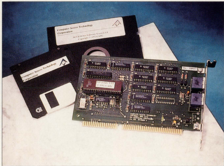
Computer Access Technology's ACCESS.bus standard AT board provides for the connection of up to 125 peripheral devices to a single communications port in a PC/AT computer. An ACCESS.bus development support kit is also available. The controller board is co-marketed with Philips.
