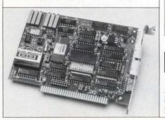
with gains of 1, 10 and 100; a sampleand-hold amplifier; and a CMOS multiplexer that scans up to 16 singleended or eight differential input signals. The board also has an internal timebase/rate generator and a general-purpose digital counter for measuring output rates of tachometers and other pulse-generating devices. Counter inputs can be at rates of up to 8 MHz. The price is \$495.
