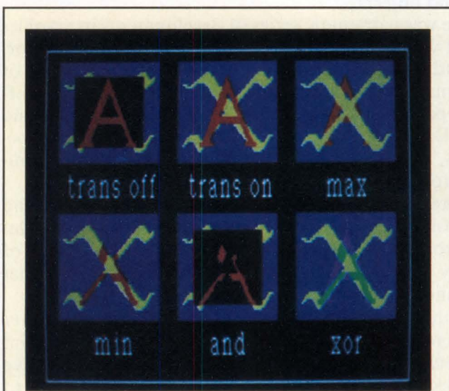
Pixblt operations allow various image combinations, including (clockwise from upper left) replacement with transparency on or off, maximum or minimum, and AND or exclusive OR.
