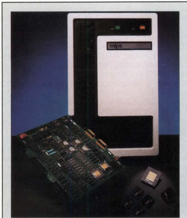
High-performance system building blocks incorporating RISC principles include component kits, CPU boards, and development systems for design and software engineers. The products are intended to establish a new price/performance standard for systems in the 3- to 10-Mips performance range.
