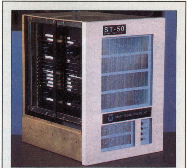
A compact CMOS-based array processor operates at 50 MFlops in compute-intensive applications such as seismic data processing, modeling and simulation and medical imaging. The ST-50 from Star Technologies uses multiple processors for I/O, storage movement, arithmetic operations and control.
