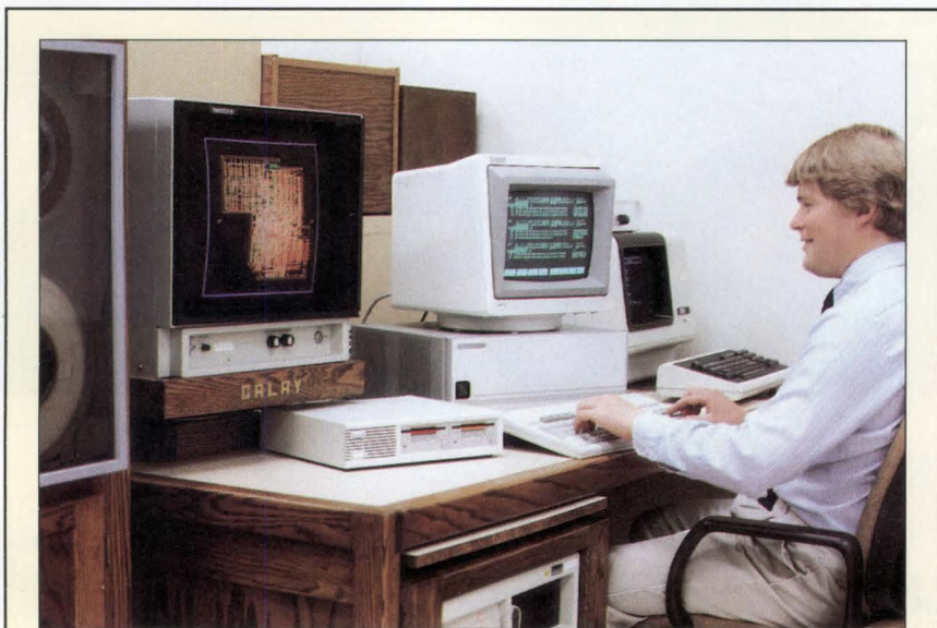
The HP 4971S troubleshoots and maintains LANs employing Ethernet IEEE 802.3 implementations. A softkey-guided programming language lets users define diagnostic tests.
