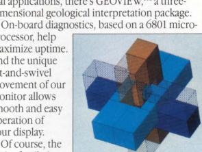
SOLIDVIEW, Lexidata's patented technology for the display of solid models, is available as an option on selected LEX 90 display processors. Its translucent shading pattern allows you to see inside vour solid model.
