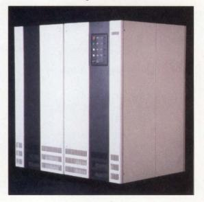
64-Kbyte cache memory increases processor throughput by providing faster access to frequently used instructions. The cache memory has a 40-ns access time and, by providing the CPU with the required instructions more than 98 percent of the time, it has a 58-ns effective main memory access time. The system provides soft error recovery, enabling the CPU to detect parity errors in the cache and reload from main memory. This recovers all soft errors and avoids halts in operation.
