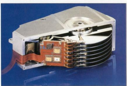
time, the design uses both a dedicated servo surface on the top platter and servo data embedded on each surface of the other disks. The rotary voice coil actuator is a statically balanced swing arm mechanism, supported on two preloaded bearings. The one-piece arm allows
