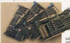
**MLZ-91A** single board CP/M<sup>TM</sup> system with on-card floppy disk drive controller, winchester interface, optional AM9511, streamer tape interface, two serial ports, one parallel port, 64K or 128K bytes RAM with parity, two EPROM sockets, and GPIB CONTROLLER.
