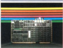
**MLZ-VDC** intelligent 640 x 480 x 4 color graphics controller based on the NEC 7220 controller chip with on-
