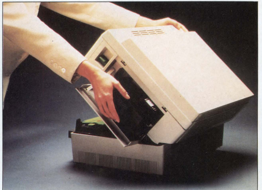
The Hewlett-Packard Laserjet printer is a desktop unit based on a marking engine by Canon. It has enough memory and intelligence to combine text and graphics with a 300-dot/in. resolution.
