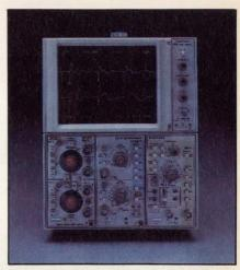
the user interface. Alphanumeric readouts are color coded by channel, while X-Y and time measurements appear in neutral. Channel 1 data are blue-green and channel 2 data are orange; voltage measurements are color coded by channel.
