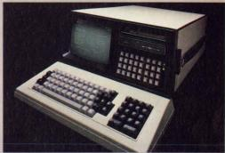
The ACT 1 is the first and only standard instrument designed specifically to test and manipulate embedded computer programs in real-time. For example, using the CRT display and full ASCII keyboard, you can identify where and when malfunctions occur and dynamically alter the programs without interrupting operations.
