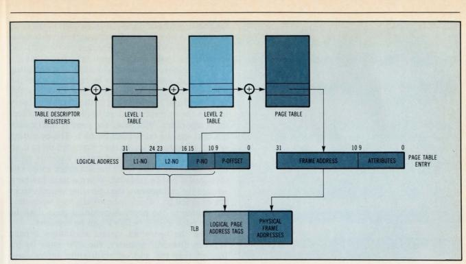
Fig 4 Using tables in memory, the CPU automatically loads the TLB. Three table levels are used to accommodate address spaces from 64K bytes to 4G bytes. System designers can eliminate either or both of the first levels to make tables smaller and to speed translation.
