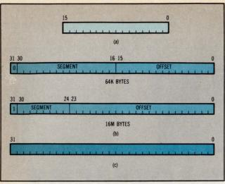
Fig 1 The Z80,000 CPU supports three address representation modes—compact address (a), segmented address (b), and linear address (c). The 16-bit, compact addresses are preferred when less than 64K bytes are addressed. Segmented mode offers two segment sizes (64K and 16M bytes). Linear mode provides uniform access to 4G bytes.
