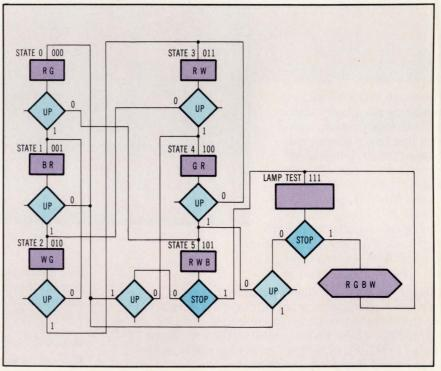
As part of Daisy Systems' hardware compiler, a simple finite state machine controls a set of four lights, noted as red (R), green (G), blue (B), and white (W). There are six distinct states, and two input signals (UP and STOP). The flow of control passes from a given state (boxes) through a decision point (diamonds) on every clock pulse. When STOP is true, the FSM cycles forever through a lamp test (state 111).
