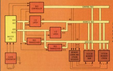
Fig 2 Simula hardware can be seen in four levels. Level 2 includes the master CPU and the shared system memory. Both RAM and ROM compose this shared memory resource, and an executive algorithm resides in EPROM.
