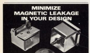
L-40 Hinge Type Flapper Solenoid Fully Enclosed To Shield Magnetic Leaks Duty: Continuous Voltage: 12 VDC Coil Resistance: 43 ohms±10% Return Spring: 1 oz. min. Insulation: Class B Leads: 24 AWG Stranded Breakdown Voltage: 700 V RMS, 60 HZ Dimensions:.780 X.780 X.750 Stroke: Adjustable
