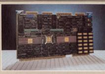
**HK68**<sup>™</sup> powerful and versatile single board UNIX<sup>™</sup> or CP/M-68K<sup>™</sup> system with MC68000 CPU, MMU, quad channel DMA, four serial ports, 128K or 256K bytes of onboard RAM with parity (expandable to 1M byte on-board!), and two iSBX<sup>™</sup> connectors for I/O expansion.
