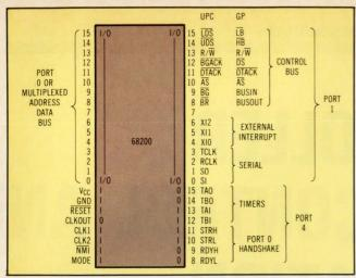
Fig 1 In the 68200 pinout, all of the pins shown on ports 0 and 1 can function as general purpose parallel 1/0s. The 1/0 pins with special functions can be programmed to serve those functions or be used as simple inputs or outputs. Strapping the mode pin selects one of the expanded bus modes, where port 0 becomes a 16-bit multiplexed address data bus and eight pins of port 1 function as associated control signals.
