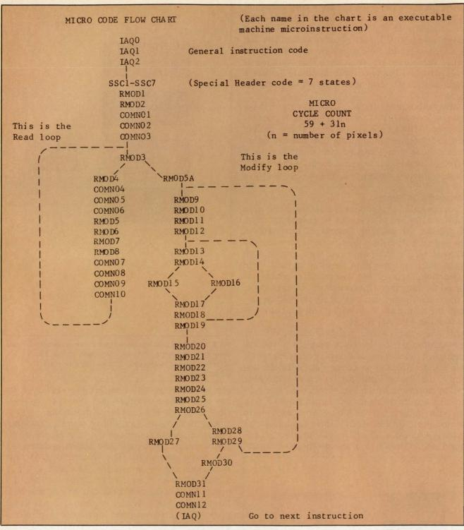
Fig 4 The RMOD instruction microcode sequence illustrates the brevity and efficiency of this approach. This code consumes only 50 control ROM locations, 19 of which are shared with other instructions.
