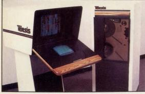
Using three microprocessors and a dualported architecture, Telesis Systems Corp's graphics processor produces picture resolutions up to 2000 x 1000 pixels. Several processor functions allow high performance processing in CAD/CAM systems.
