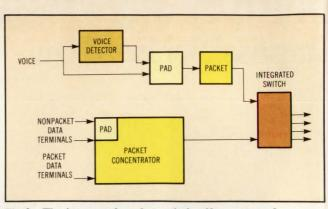
Fig 3 The integrated packet switch offers a second alternative for contending with voice and data traffic. As with the integrated hybrid switch, the unacceptable delay for the voice channels poses the biggest obstable.
