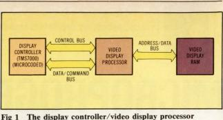
Fig 1 The display controller/video display processor interface illustrates how user written microcode helps simplify the problem of display control. Streamlined code capable of simultaneously controlling several functions optimizes the control process.
