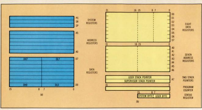
Fig 3 Both the 68200 and 68000 exhibit a regular register architecture with several general purpose data registers and address registers. The 68200 has 16-bit registers that can handle 8-bit data more efficiently (a). The 68000 has 32-bit registers to support a full 32-bit internal processor architecture (b).
