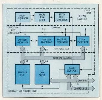
Fig 1 Control, execution, and input/output handling are the major functional breakdowns in the NS16081 FPU. Parallel execution of arithmetic computations and special hardwareimplemented algorithms are key elements in the chip's high speed capabilities.
