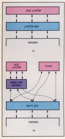
Standard microcomputer operating systems interface with computer hardware directly through an assembly language BIOS (a). Datalex has substituted a special routine in the PC-DOS bubble to interface the p-System to the normal PC-DOS (b), thereby providing both the p-System and PC-DOS the same functions.
