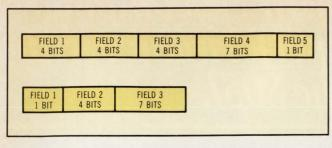
Fig 2 The arithmetic execution unit runs under the command of a dedicated microcontroller whose instruction and address fields are shown here. Each microinstruction contains a part of the address of the following microinstruction, making high speed operation possible.
