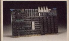
**MLZ-VDC** intelligent 640 x 480 x 4 color graphic controller based on the NEC 7220 controller chip with on-board Z-80 CPU. DMA controller, and user definable FIFO interface to Multibus<sup>™</sup> Users may display up to 16 colors from a 4K palette. Up to 1024 x 1024 x 3 interlaced also available.
