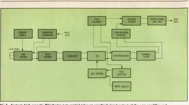
Fig 5 Vertex's high capacity Winchester R/W control takes an equalized signal output of the AGC amplifier and differentiates, filters, and digitizes it. A peak follower circuit processes this signal and, in conjunction with a zero-crossing detector, generates read data.
