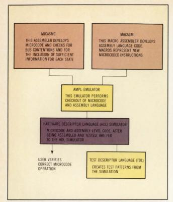
Fig 5 The user's microcode tool kit includes a microcode assembler, a macro assembly language assembler, an emulator, a simulator, and a test pattern generation utility.
