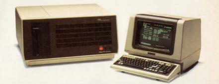
The Gould 9516S Microsystem Integration System supports **any** combination of 68000, 8086, 8088, Z8001, Z8002, 68B09E, 8085A and Z80A microprocessors. It includes a 1 megabyte thinline double-density, double-sided floppy disk drive. Its RS-232-C port lets you interface with any minicomputer for fast, effective software development.
