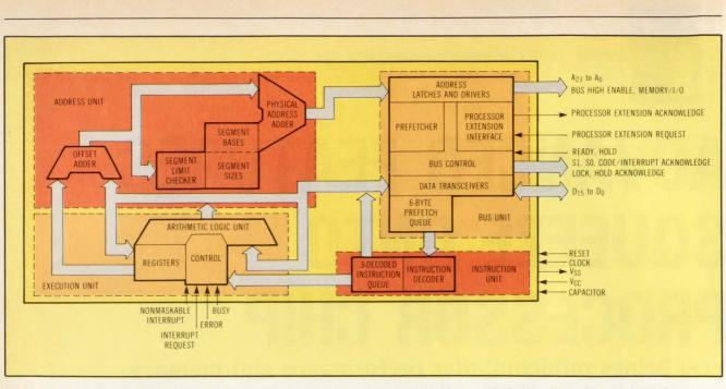
Memory management and pipelining functions, which previously separated chips or whole circuit boards, are brought onchip in the 286. Thus, multi-user and multiprocessing applications are possible, while maintaining code compatibility with the 8088 and 8086 processors.
