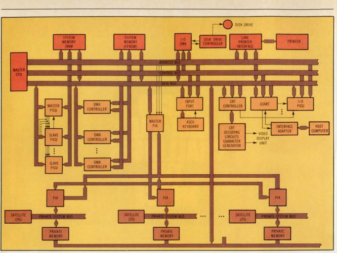
Fig 4 The parallel Simula machine is based upon tightly coupled processors operating in master/slave topology. This interrupt-driven architecture tends to improve performance by actually reducing software overhead through asynchronous service schedules.
