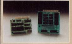
The SBX-FDIO can control up to four single or double sided, single or double density 5¼ inch or 8 inch floppy disk drives. A software toggle allows both 5¼ inch and 8 inch drives to be intermixed on the same cable!
