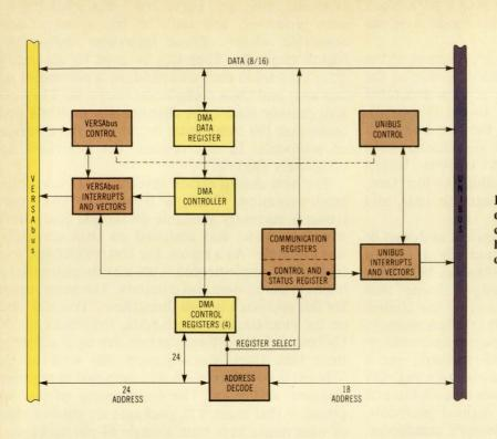
Fig 2 This UNI/VERS system block diagram centers upon the DMA controller. Two boards support all hardware functions and either bus can serve as the master.
