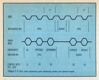
Fig 3 A slave sequencer controls transactions between the FPU and its master, the CPU. All transactions depend upon the SPC pulse, which controls information flow from the CPU to the FPU and vice versa.
