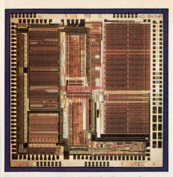
Hewlett-Packard's 32-bit CPU chip for the HP 9000 is fabricated using the company's proprietary NMOS-III process. It has a minimum feature size of  $1.5 \ \mu m$ , and a spacing of  $1 \ \mu m$ . Other chips in the set handle memory management, timing, and instruction cache functions.
