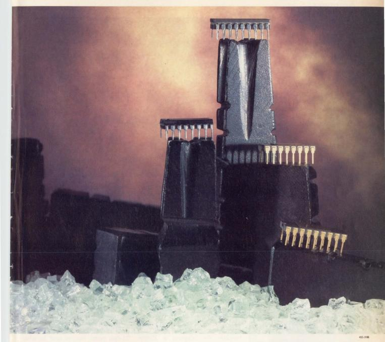
Sprague Series ULN-2000 Darlington Arrays still set the industry standard for power-interface ICs with improved ratings, hermetic packaging (cer-DIP or side-brazed), and processing to MIL-STD-883. Series ULN/ULQ/ULS-2000 (and ULN/ULQ/ULS-2800) highvoltage, high-current arrays have been driving relays, solenoids, stepper motors, LED and incandescent displays since Sprague introduced the ICs a decade ago. For Engineering
