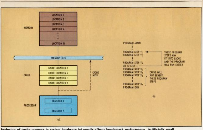
Inclusion of cache memory in system hardware (a) greatly affects benchmark performance. Artificially small benchmarks may reside totally in cache and give false indications of performance. Code segment in (b) between  $Y_1$  and  $Y_N$  should not fit entirely in cache. Segment  $X_1$  to  $X_N$  will not affect cache since it is not repeated.
