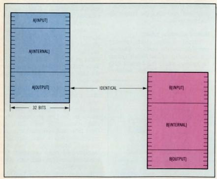
Procedure A finds its input parameters in a set of CPU registers (A[Input]), uses a block of registers for its internal operations (A[Internal]), and passes parameters to procedure B via another set of registers (A[Output]). When Procedure B begins execution, its input parameter registers (B[Input]) are identical to A[Output].
