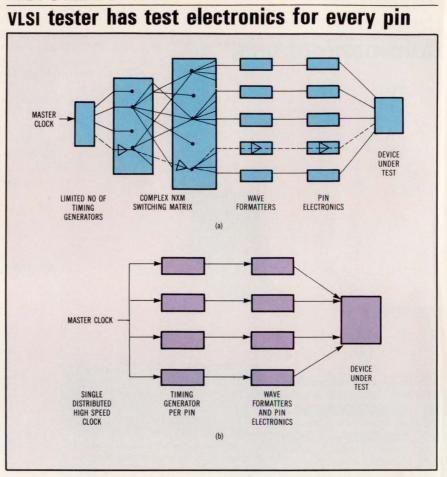
The cumbersome switching matrix of shared resource testers (a) introduces timing errors and requires programming at a low hardware level. The tester-part-pin architecture (b) allows precise calibration of all timing and can be programmed at a high level with user-defined variables and labels.
