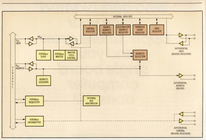
**Fig 3** The VERSAbus interface (V-board) contains the majority of hardware control circuitry. It features an internal **3**-state bus for communications, and solid-state drivers (TTL) that provide plenty of punch for longer cable runs.
