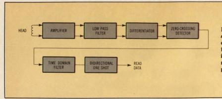
Fig 3 Low capacity Winchester read circuitry gets by with a minimum of components. After amplification, filtering, and differentiation, the signal is fed to a zero-crossing detector. The resultant output corresponds to signal peaks.
