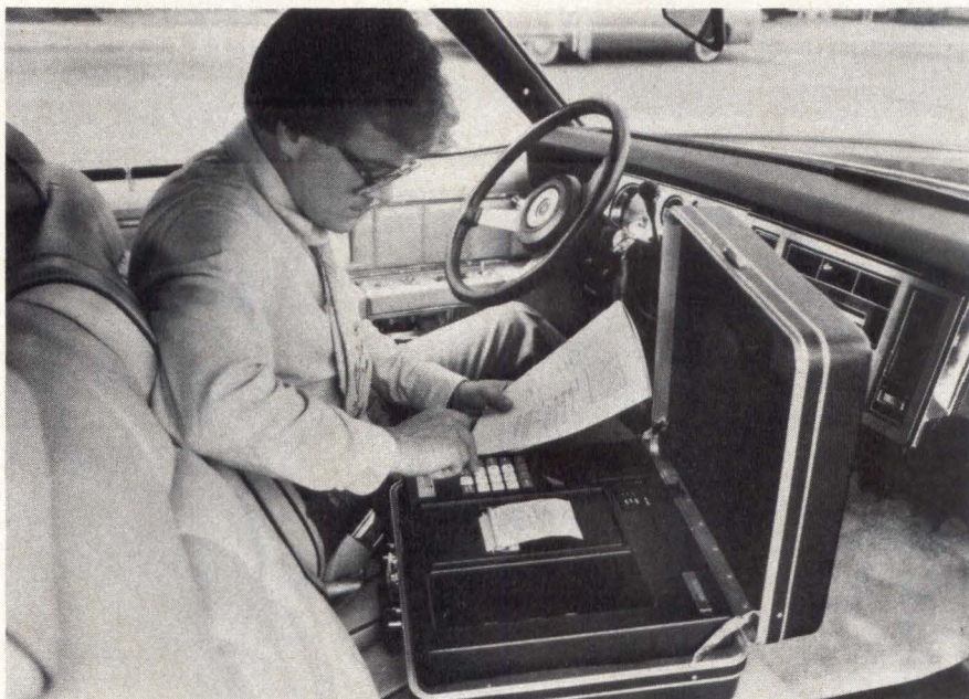
Norand's Route Commander combines data collection terminal, data storage capacity, and printer with processing and telecommunications capabilities in portable unit to extend benefits of computer data processing into distribution industry
