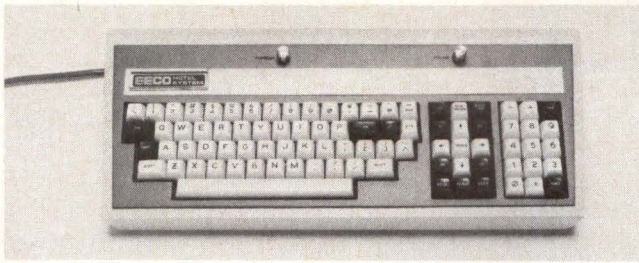
Fig 7 Keyboard variation for hotel system. Volume control adjusts level of clicks that simulate typewriter sounds. Multiple transmit keys reduce hand travel required to transmit data
