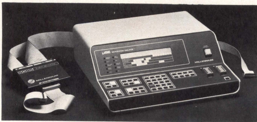
Host computer acts as multiprocessor development system with addition of Millennium Systems Series 2000 emulator that uses discrete microprocessor cards
