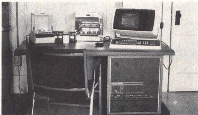
Fig 1 Micro-Coal 1 control console. MicroNova microcomputer is in cabinet at right, just above dual floppy disc drive. Interfacing circuitry and audio alarm are in upper section of cabinet. CRT displays main menu, allowing operator to choose laboratory functions. Balance at left corner of desk weighs samples of up to 30 g at accuracy to 0.0001 g. Pedal switch to left of CRT terminal strobesc microcomputer for reading balance
