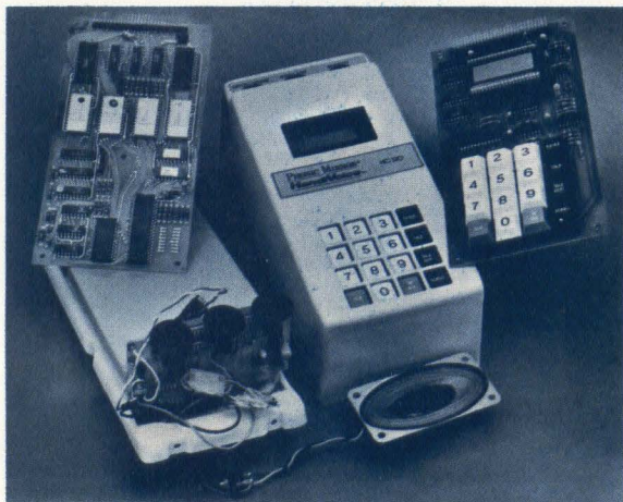
Handheld electronic device capable of producing audible human speech from keyboard inputs is based on speech synthesizer and related computer interfacing devices, developed by Votrax, that enable it to simulate human voice and articulate most English language words
