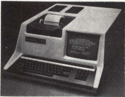
Desk-top computer from Compucorp has 65k bytes of addressable memory, 630k bytes of disc memory, 40-column alphanumeric journal printer, and full ASCII keyboard with user-definable function keys
