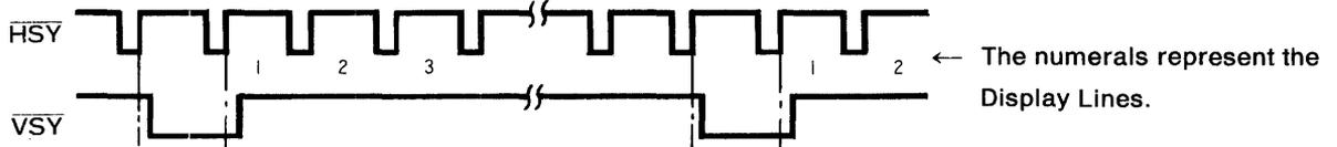
(Though the quantity of bits used for data transmission is varied, the above figure illustrates the case of 4Bit Parallel Mode.)
