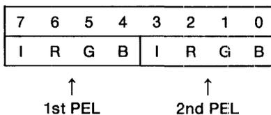
This mode is enabled when GRM<sub>1</sub>=GRM<sub>0</sub>= '1'. Since the color of each display PEL is specified in four-bit units of the data read from VRAM, up to 16 colors can be simultaneously displayed. The size of the display PELs in the horizontal direction is four times that of the 640 x 1 Bit Mode. The border will be displayed in the color selected by Bits 3-0 of the Color Register (but when BINH='1', the border will be displayed in black (IRGB="0000")).
