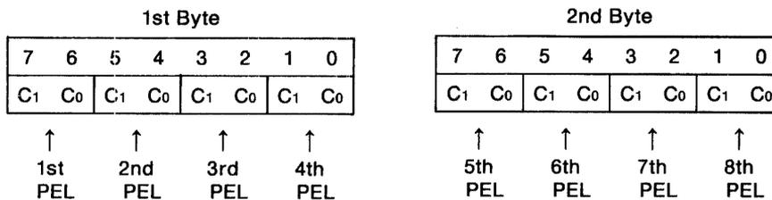
This mode is enabled when GRM1 = '0', GRM0 = '1', and Bit 4 of the Mode Register is '1'. The display colors are identical to those of the 320 x 2 Bit Mode (simultaneous display of four colors), and the size of display PELs is identical to that of the 640 x 1 Bit Mode.
