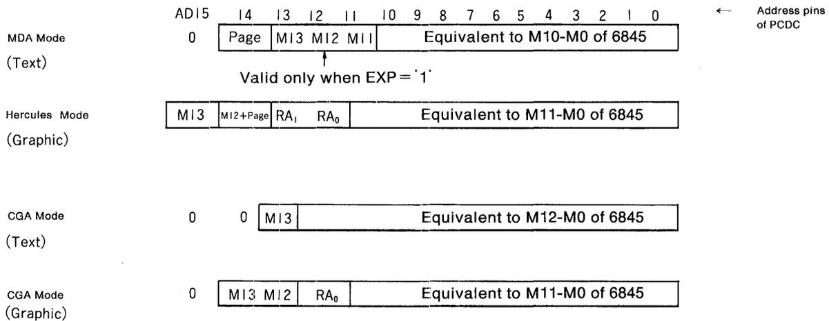
M11-M13, which are enclosed in boxes within the above figure, are valid only when EXP = '1'. Page is the output for Bit 7 of the Mode Register. (Page is valid only in Hercules Mode. Unless '1' has been written to Bit 1 of the Control/ID Register, writing to Page is impossible. In CGA Mode, Page is always '0'.)
