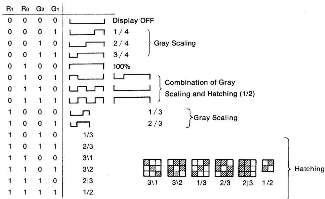
With CGA graphics software, a four-color display is adequate, so it is recommended that the user sets the gray scaling and hatching of his/her own preference. (Since a maximum 16-color display is possible in Text Mode, it is recommended that MON be set to '1' to convert to a monochrome display, then a clear display be implemented (Set Black as Display OFF and White as 100%.).)
