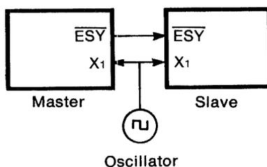
Set EXTS = '1', then set the master side to ESIO = '1' (the  $\overline{\text{ESY}}$  pin becomes an output pin) and set the slave side to ESIO = '0' (the  $\overline{\text{ESY}}$  pin becomes an input pin). Since this procedure will synchronize two chips, one chip can be assigned to Text display and the other to Graphics display for a combined superimposed display (superimposing is performed by an external circuit).
