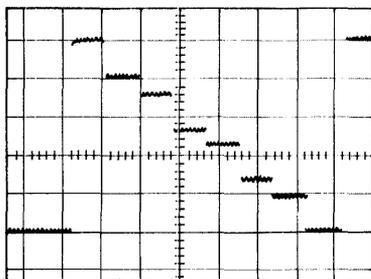
(A Waveform after Digital-to-Analog Conversion)
