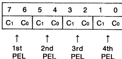
This mode is enabled when GRM1 = GRM0 = '0' and Bit 4 of the Mode Register is '0'. Since two bits of each datum read from VRAM specify the color of the display PEL, up to four colors can be simultaneously displayed.
