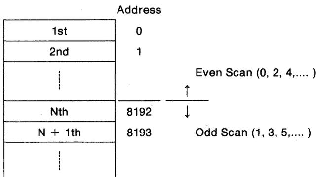
With Hercules software, the data is stored in separate banks in four-line cycles, then the banks are switched according to the Raster Address RA<sub>0</sub>, RA<sub>1</sub> (4 Bank Mode). That is, the data of Lines 0, 4, 8, ... is placed in the first 8K bytes, the data of Lines 1, 5, 9, ... is placed in the next 8K bytes, the
