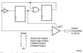
Figure 3: Additional CCLK-Pulse Generator
