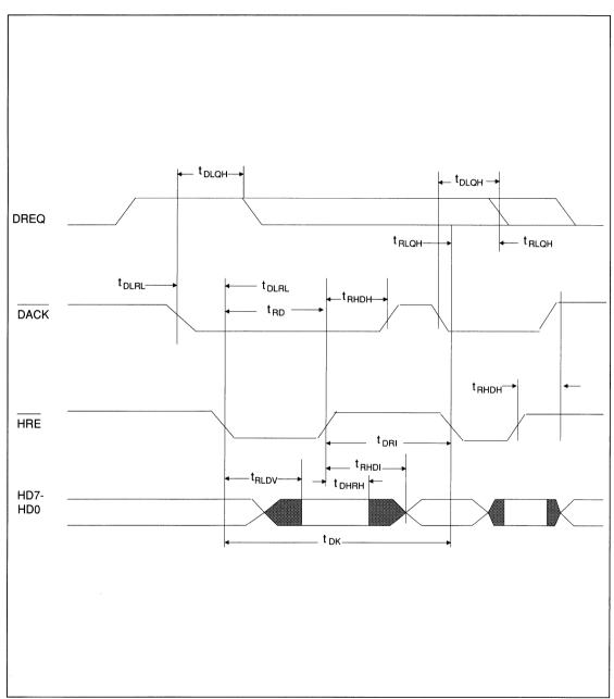
FIGURE 12. AT/XT HOST DMA READ TIMING
