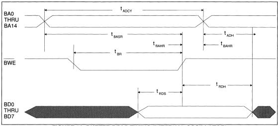
FIGURE 16. BUFFER READ TIMING (INTERNAL OSCILLATOR)
