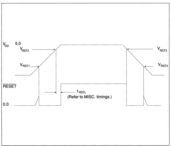
FIGURE 7. POWER QUALIFIED RESET VOLTAGE THRESHOLD
