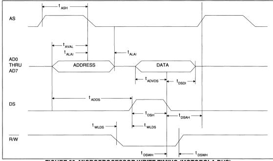
FIGURE 20. MICROPROCESSOR WRITE TIMING (MOTOROLA BUS)
