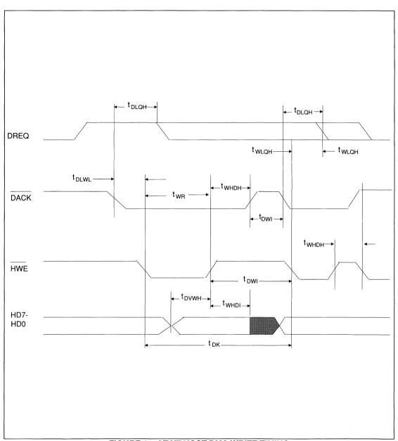
FIGURE 11. AT/XT HOST DMA WRITE TIMING
