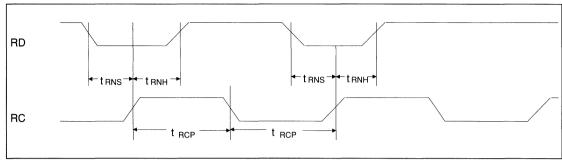
FIGURE 26. READ DATA TIMING (NRZ MODE)
