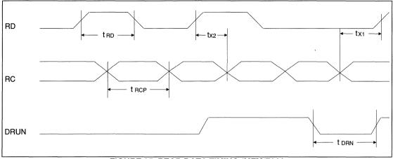
FIGURE 25. READ DATA TIMING (MFM/RLL)
