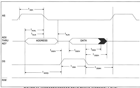
FIGURE 22. MICROPROCESSOR READ TIMING (MOTOROLA BUS)
