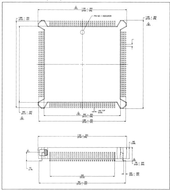
FIGURE 35. 84 LEAD PQFP
