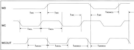
FIGURE 24. WRITE DATA TIMING (NRZ MODE)
