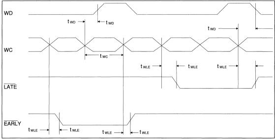
FIGURE 23. WRITE DATA TIMING (MFM/RLL MODE)
