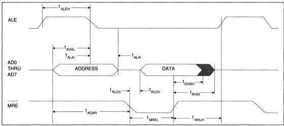
FIGURE 21. MICROPROCESSOR READ TIMING (INTEL BUS)
