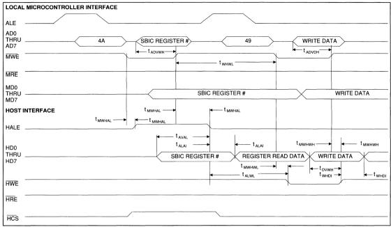
FIGURE 13. SLAVE HOST WRITE TIMING
