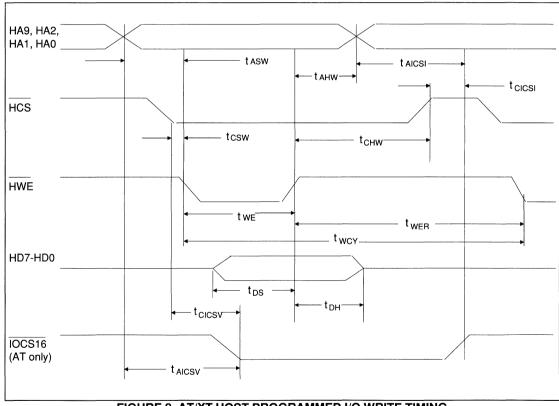
FIGURE 8. AT/XT HOST PROGRAMMED I/O WRITE TIMING
