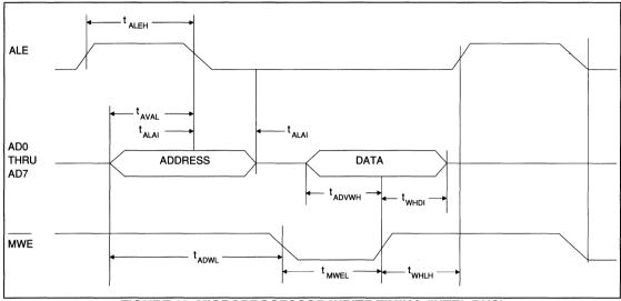
FIGURE 19. MICROPROCESSOR WRITE TIMING (INTEL BUS)
