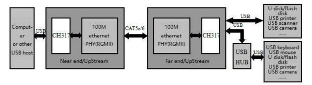
Figure 2 Block diagram of optical fiber extension scheme
