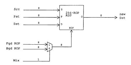
Figure 2.12-1 ET4000/W32p Graphics Accelerator Data Path
