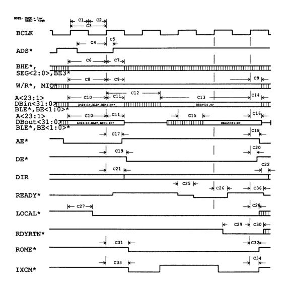
Figure 4.11-1 Local Bus Read/Write Timing
