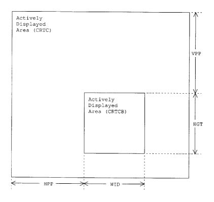
HPP: Horizontal Pixel Position WID: Width
