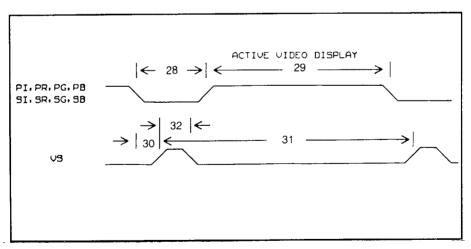
Figure 6.6.3-6 Display Vertical Sync Timing, 768 Lines
