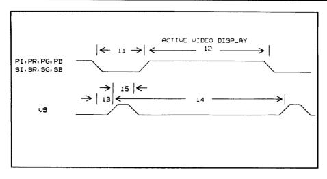
Figure 6.6.3-3 Display Vertical Sync, 480 lines
