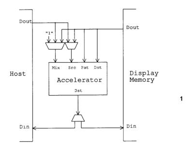
Figure 2.12-3 ET4000/W32p Accelerator Data Path Routing
