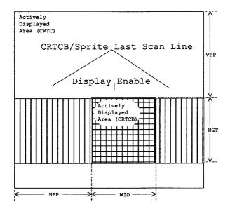
HPP: Horizontal Pixel Position WID: Width
