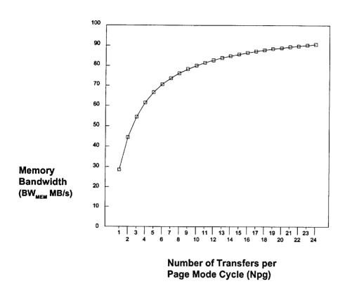
Depending on the system requirements at any given time, the ET4000/W32p will operate at a certain point on the curve. The operation point on the curve indicates how much bandwidth the ET4000/W32p can supply, not how much it is using; so if the CRT Controller requires 20 MB/s and the ET4000/W32p can supply 60 MB/s, then there is 40 MB/s (60-20=40) remaining that can be supplied to another requester.
