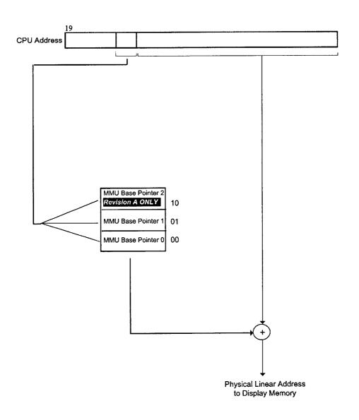
Figure 2.11.1-1 Three MMU Aperture Mapping
