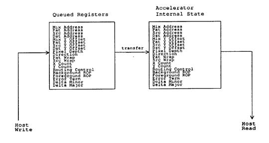
Figure 2.12-2 ET4000/W32p Queued Registers and ACL Internal State
