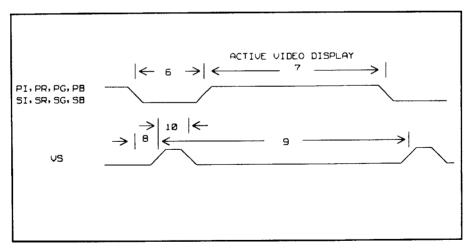
Figure 6.6.3-2 Display Vertical Sync, 400 lines
