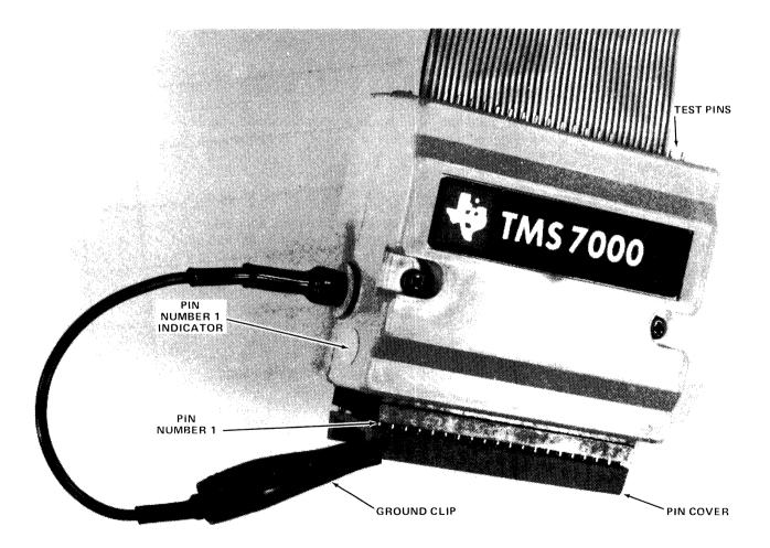
Figure 2-1 Target Connector With Pin Cover in Place
