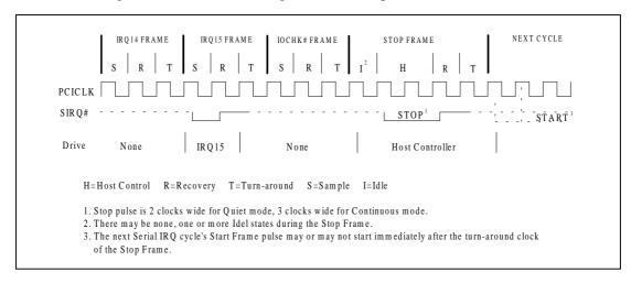
Figure 3.1-3 Stop Frame Timing with Host using 17 SIRQ# Sampling Period
