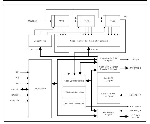
Figure 3.5-3 Block Diagram of RTC
