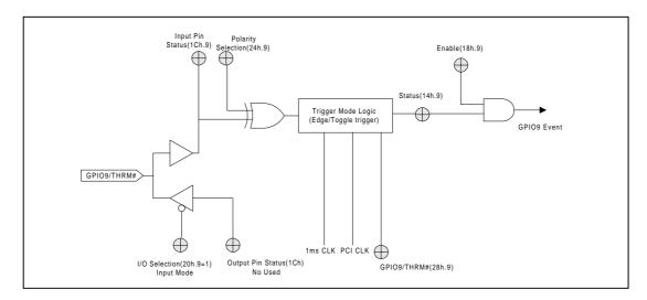
Figure 3.2-6 Thermal Detection Logic
