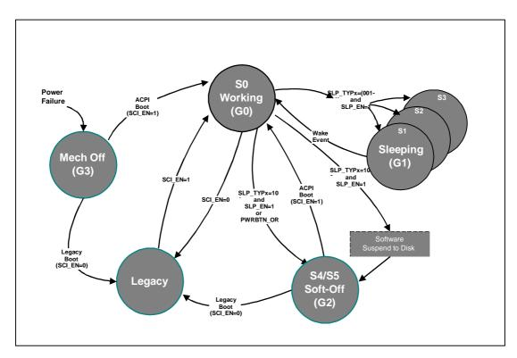
Figure 3.2-1 Global System State Diagram
