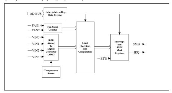
Figure 3.4-1 Data Acquisition Module Block Diagram
