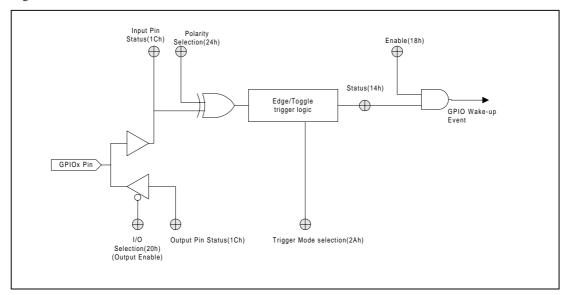
Figure 3.2-9 GPIO Logic
