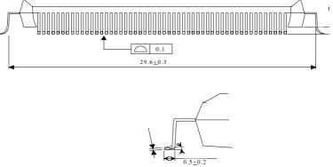
Figure 9.2-1 SiS5595 Package Specification
