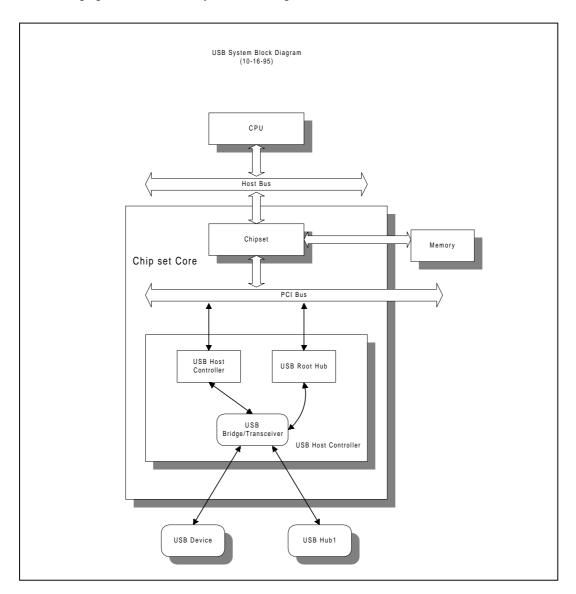
Figure 3.3-1 USB System Block Diagram
