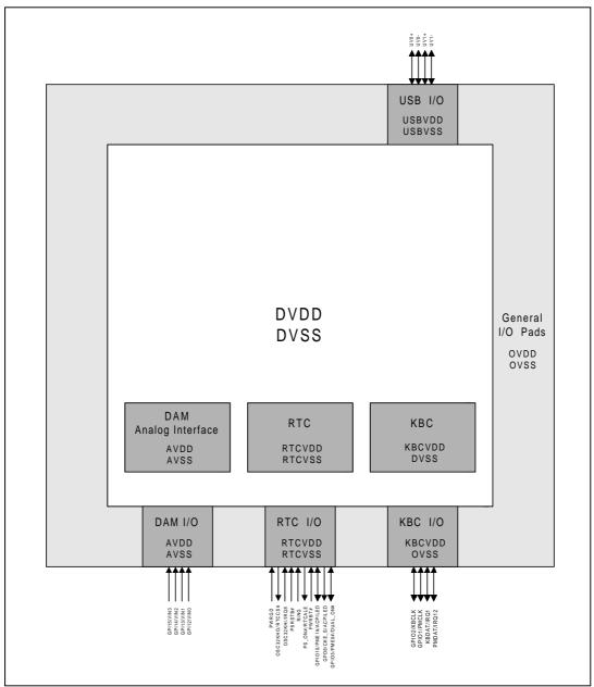
Figure 8.1-1 SiS5595 Internal Power Planes
