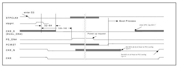
Figure 3.2-4 NB/5595's Timing Diagram in S3 State
