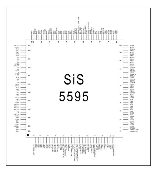
Figure 2.1-1 Pin Assignment (Top View)
