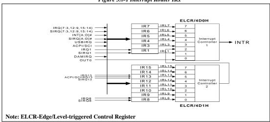
Figure 3.8-1 Interrupt Router IRx
