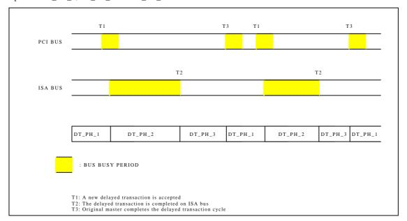
Figure 3.1-1 PCI ISA Delay Transaction
