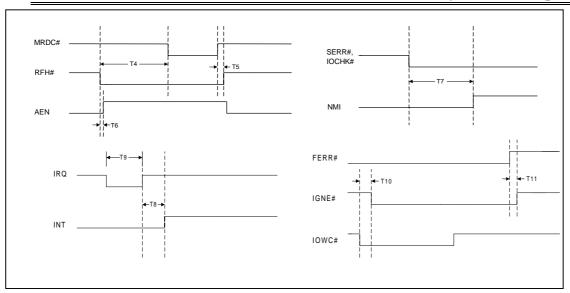
Figure 8.5-3 Miscellaneous Timing
