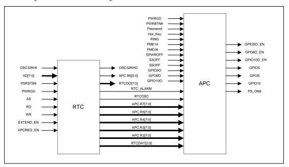
Figure 3.5-1 RTC Module Block Diagram
