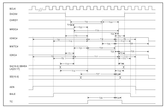
Figure 8.5-1 DMA Cycles
