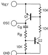
3. Another way of providing greater deadband is just to limit the maximum pulse width. This can be done by using a clamp to limit the output voltage of the error amplifier. A simple way of achieving this clamp is with the circuit below:
