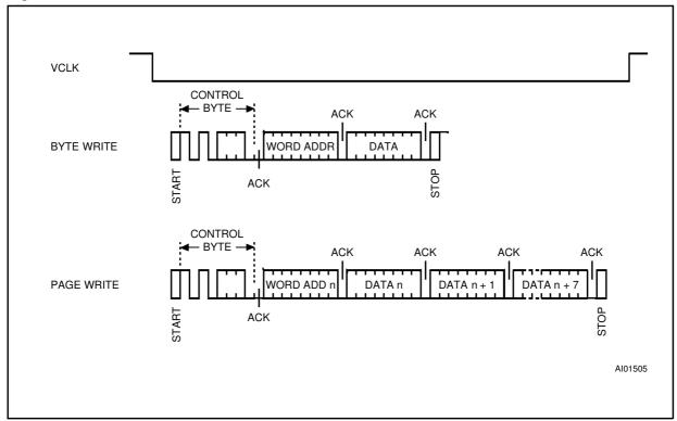
Figure 7. Inhibited Write when VCLK = 0
