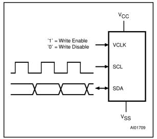
nized by the serial clock SCL. Read and write operations are initiated by a START condition generated by the bus master (Table 2). The START condition is followed by a stream of 7 bits (Table 1), plus one read/write control bit and is terminated by an acknowledge bit.
