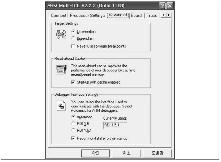
Figure 2-12. Debugger Configuration: Advanced Page
