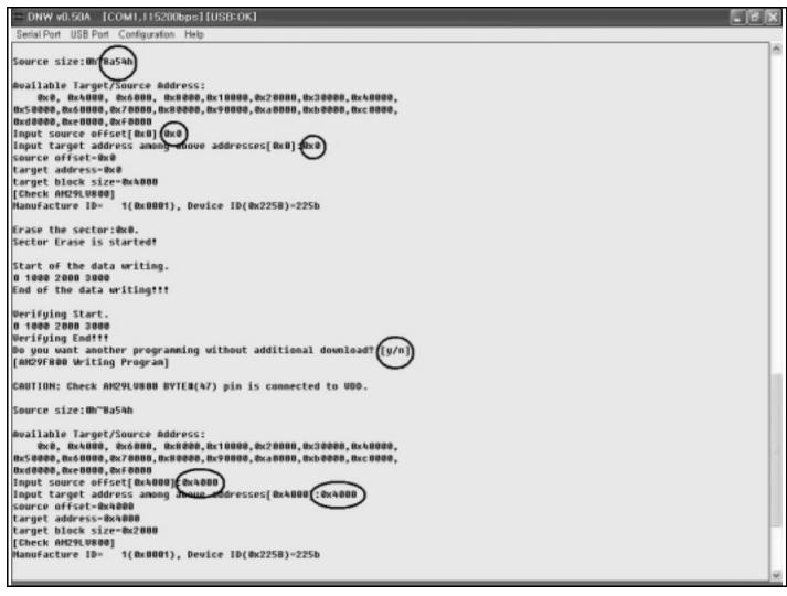
Write source offset '0x4000' and write target address '0x4000', and then type 'y'.
