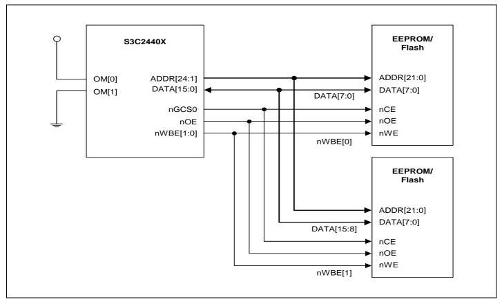
Figure 4-2. Half-word Boot ROM Design with Byte EEPROM/Flash
