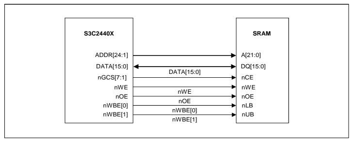
Figure 4-8. Halfword SRAM Bank Design with Halfword SRAM
