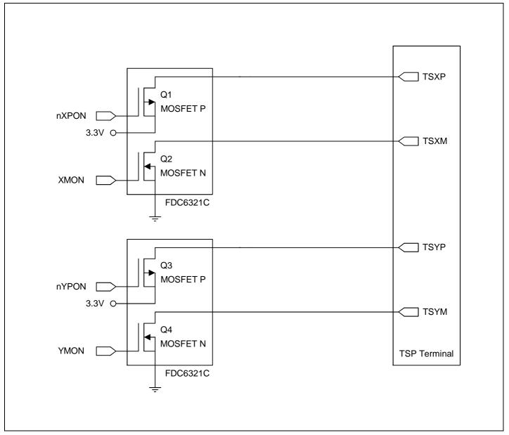
Figure 4-20. TSP Interface Circuit with S3C2440X
