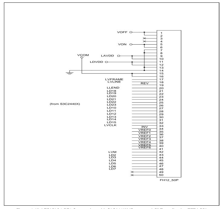
Figure 4-17. LTS350Q1-PE1 Connection with S3C2440X (Samsung 3.5" Transflective TFT LCD)
