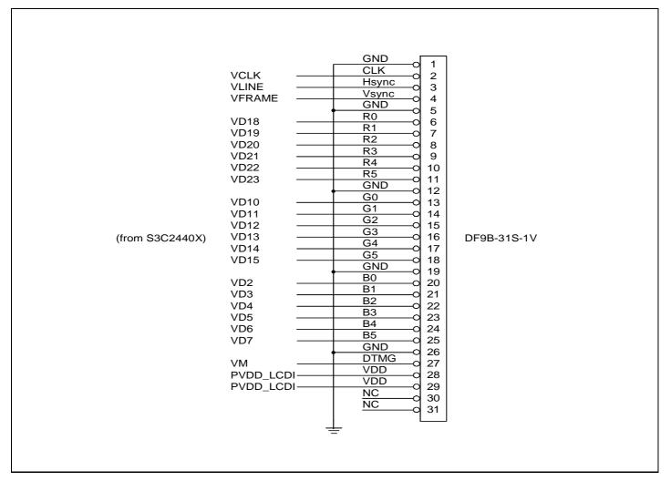
Figure 4-18. LP104V2-W Connection with S3C2440X (LG Philips 10.4" TFT LCD)
