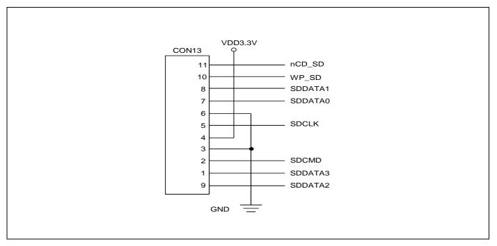
Figure 1-7. SD Card Socket on SMDK2440
