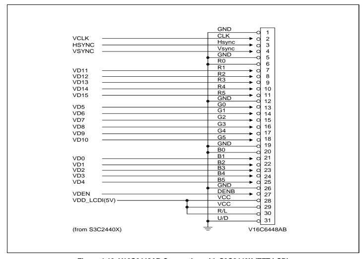
Figure 4-19. V16C6448AB Connection with S3C2440X (TFT LCD)
