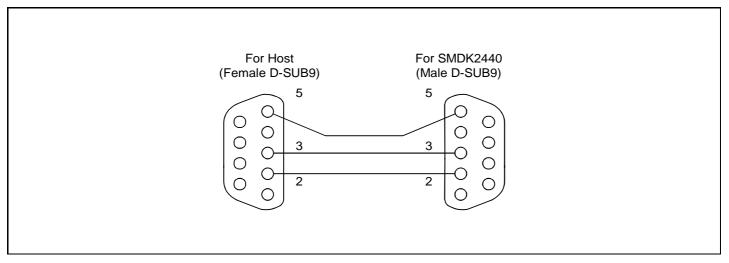
Figure 2-2. Serial Cable Connections for SMDK2440 Board
