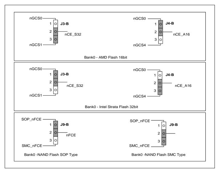
Figure 1-4. SMDK2440 Board Memory Configurations
