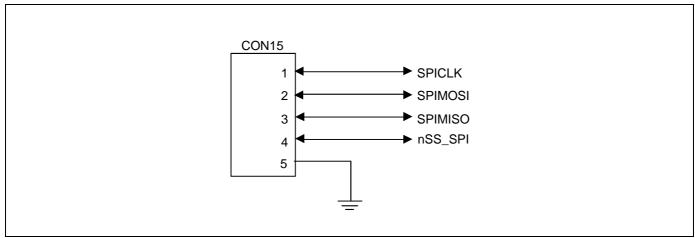
Figure 1-6. SPI Connector on SMDK2440
