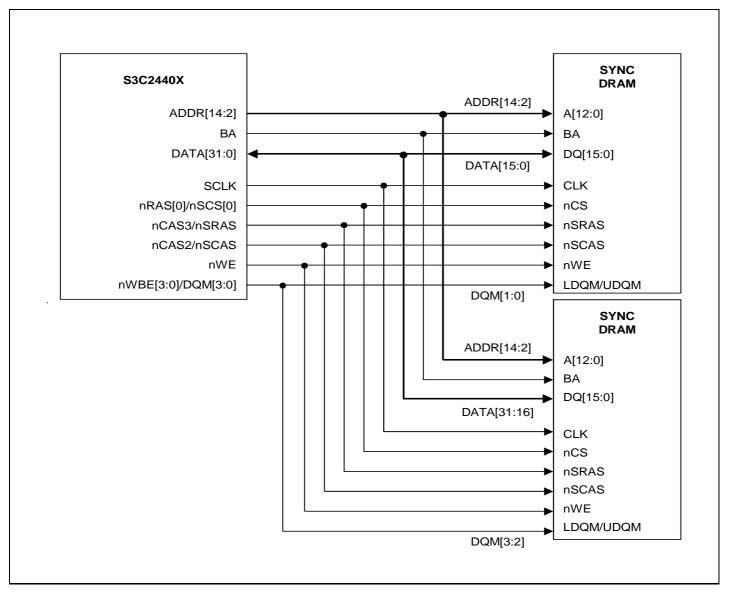
Figure 4-11. Word SDRAM Design with Half-word Component
