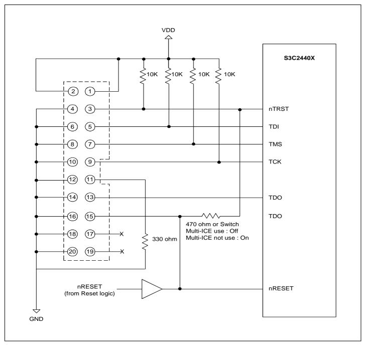
Figure 4-22. MULTI-ICE Interface Design Example
