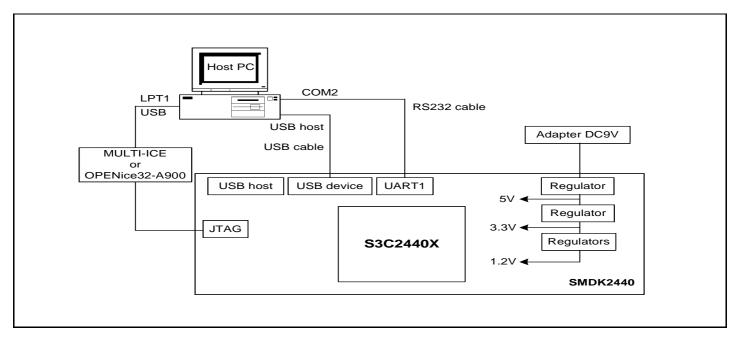
Figure 2-1. Setup Environment for SMDK2440 Board
