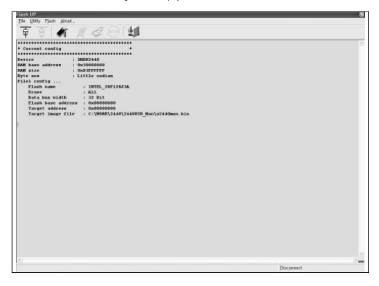
7. Select Write from the Flash Menu. Then it starts to erase the specified area of Intel Strata Flash and write the image to the Flash memory. It takes about 10 second.
