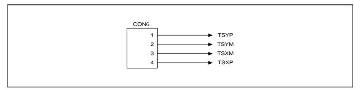
Figure 1-5. Touch Panel Film Connector on SMDK2440
