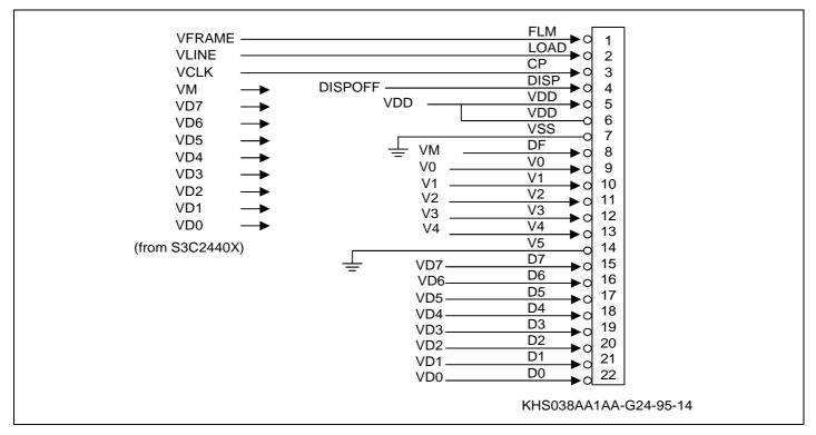
Figure 4-16. KHS038AA1AA-G24 Connection with S3C2440X (256 Color STN LCD)
