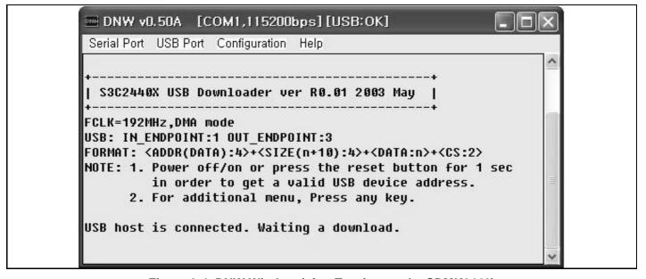
Figure 3-4. DNW Window (after Turning on the SDMK2440)
