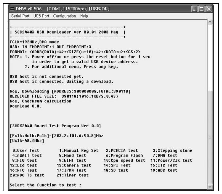
Figure 2-7. 2440TEST Execution After its Downloading through USB
