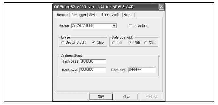
Figure 2-18. OPENice32-A900 Configuration: Flash Configuration Setting Page
