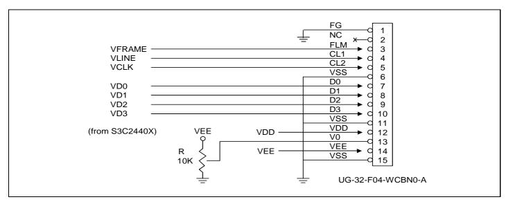
Figure 4-14. UG-32F04 Connection with S3C2440X (320x240 Mono STN LCD)
