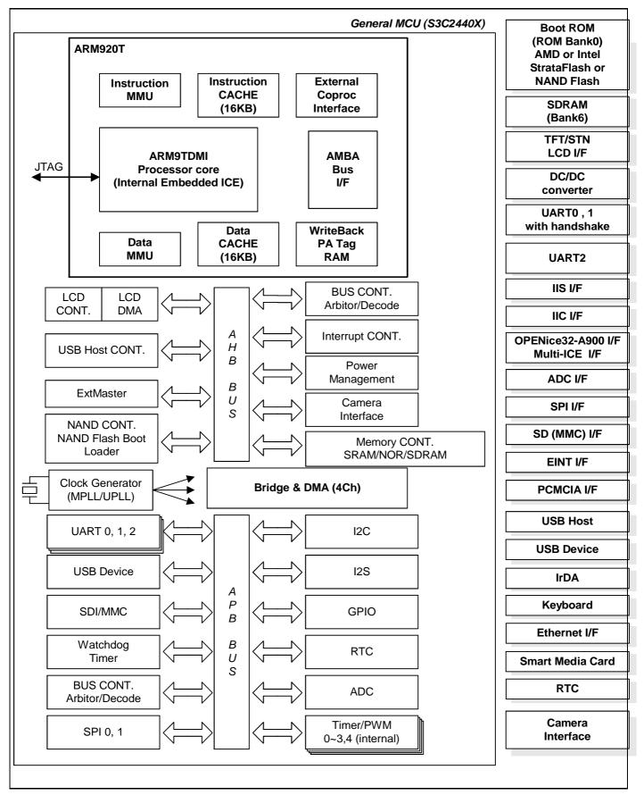
Figure 1-1. SMDK2440 Function Block Diagram
