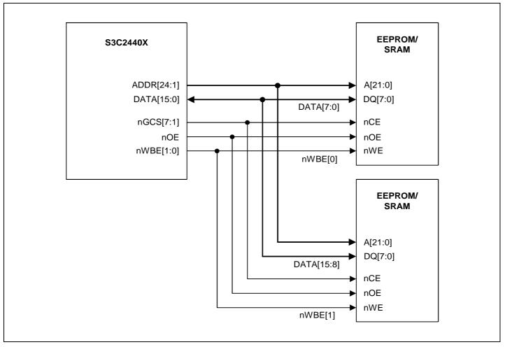
Figure 4-7. Halfword EEPROM/SRAM Bank Design
