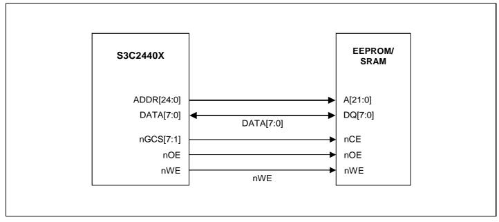
Figure 4-6. One-byte EEPROM/SRAM Bank Design
