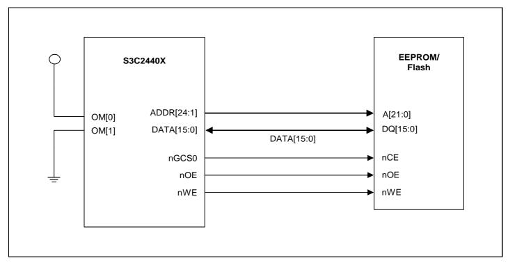
Figure 4-3. The Halfword Boot ROM Design with Halfword EEPROM/Flash
