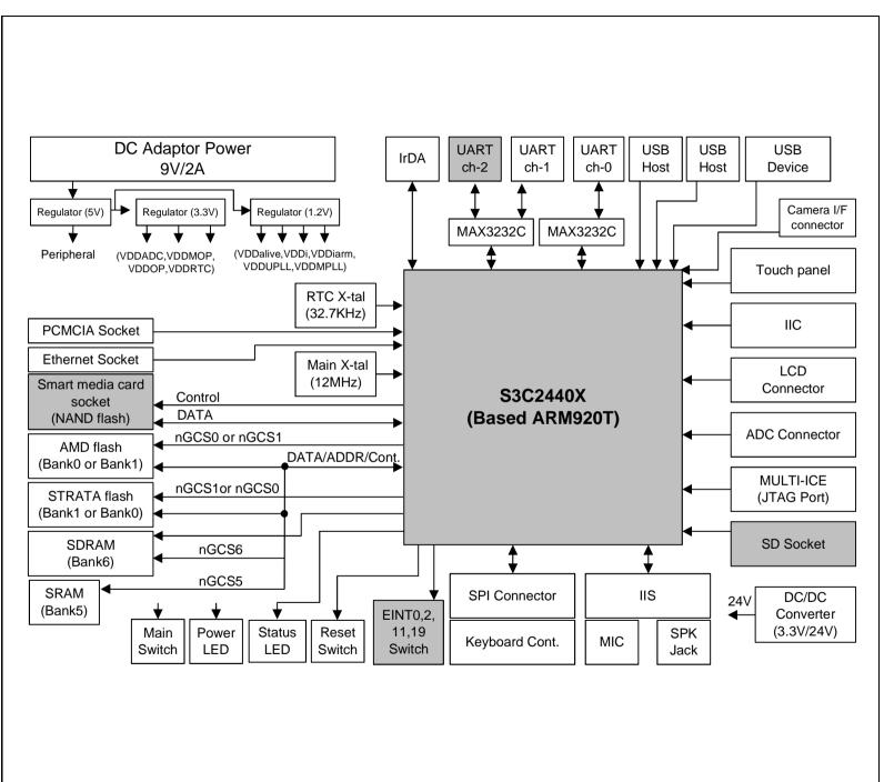
Figure 1-3. Detailed SMDK2440 Board Diagram
