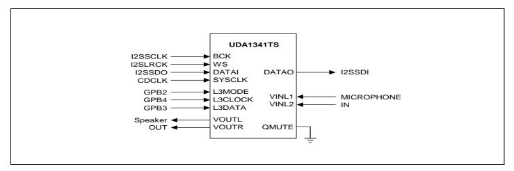
Figure 4-13. UDA1341TS Connection with S3C2440X
