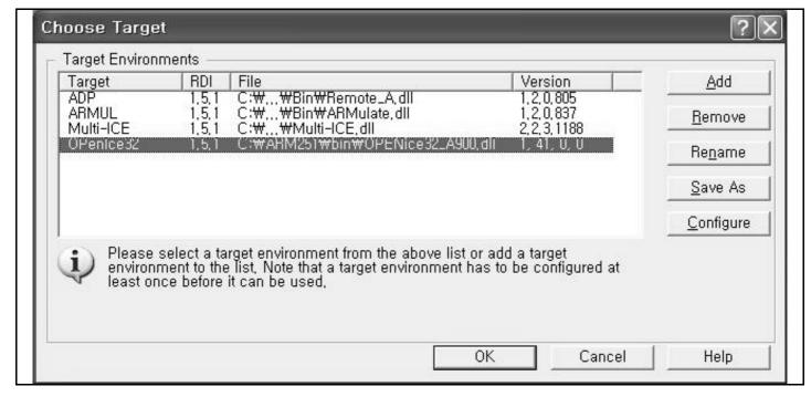
Figure 2-19. Debugger Configuration: Choose Target
