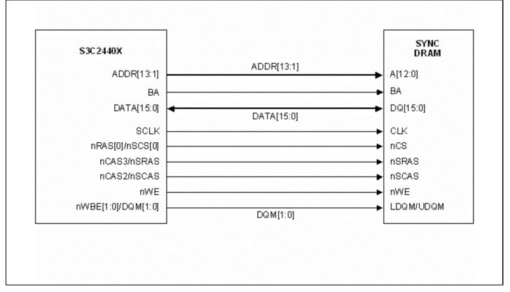
Figure 4-10. Halfword SDRAM Design with Halfword Component
