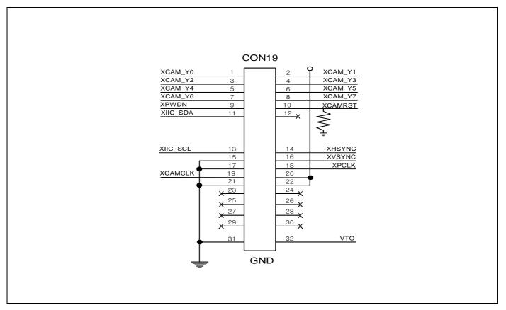
Figure 1-12. CAMERA Interface Connector on SMDK2440
