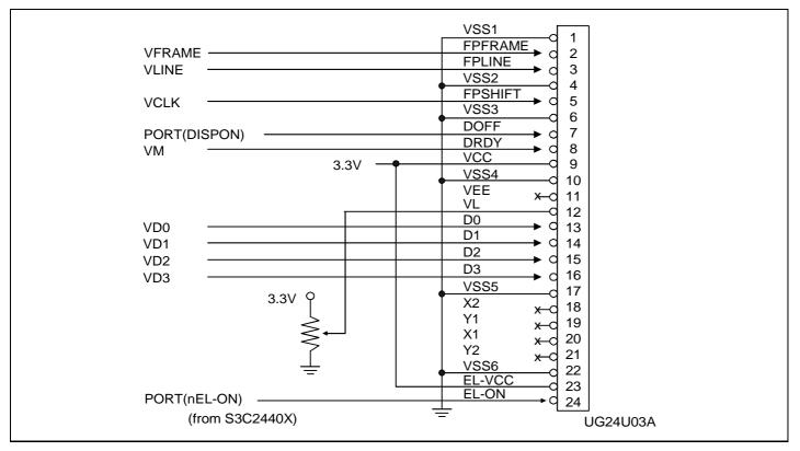
Figure 4-15. UG24U03A Connection with S3C2440X (320x240 Mono STN LCD)
