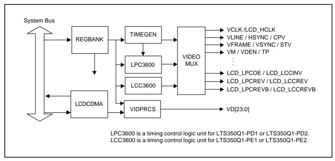
Figure 15-1. LCD Controller Block Diagram
