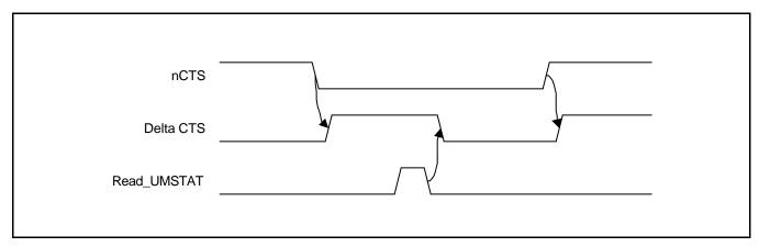
Figure 11-8. nCTS and Delta CTS Timing Diagram
