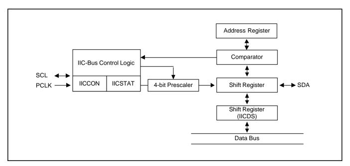
Figure 20-1. IIC-Bus Block Diagram
