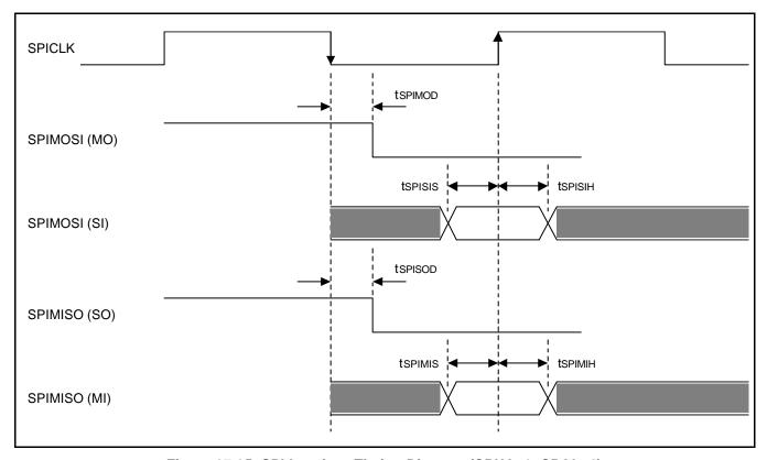
Figure 27-35. SPI Interface Timing Diagram (CPHA=1, CPOL=1)
