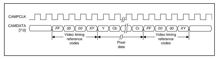
Figure 23-3. ITU-R BT 656 Input Timing Diagram
