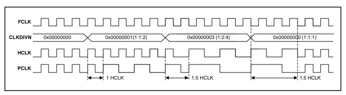
Figure 7-6. Example of Internal Clock Change
