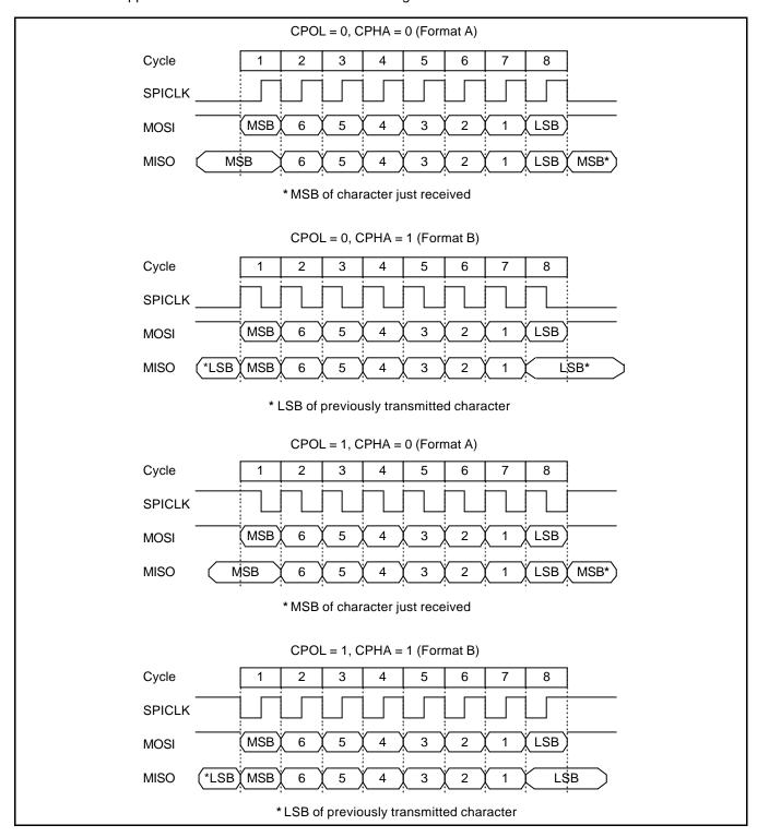
Figure 22-2. SPI Transfer Format
