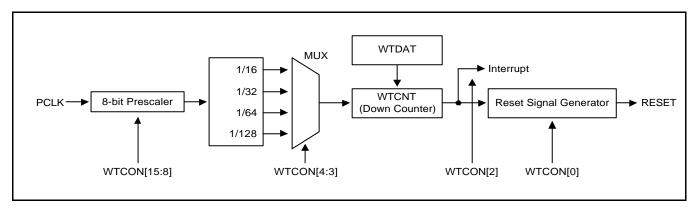
Figure 18-1. Watchdog Timer Block Diagram
