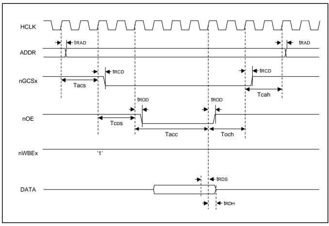
Figure 27-12. ROM/SRAM READ Timing Diagram (I) (Tacs=2, Tcos=2, Tacc=4, Toch=2, Tcah=2, PMC=0, ST=0)
