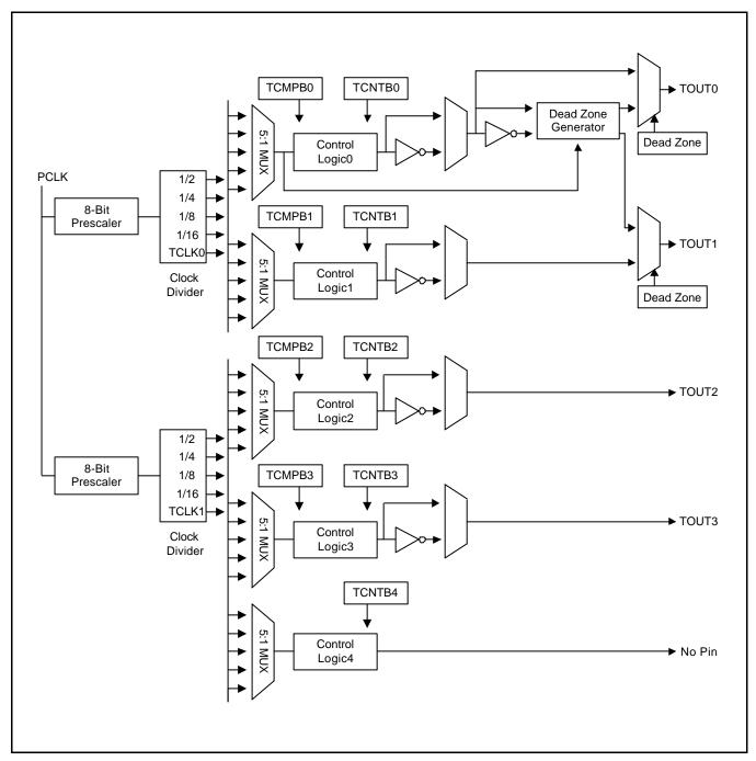
Figure 10-1. 16-bit PWM Timer Block Diagram
