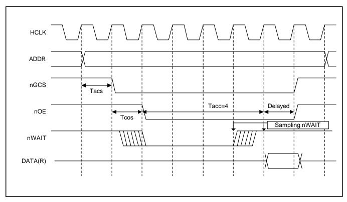
Figure 5-2. S3C2440A External nWAIT Timing Diagram (Tacc=4)
