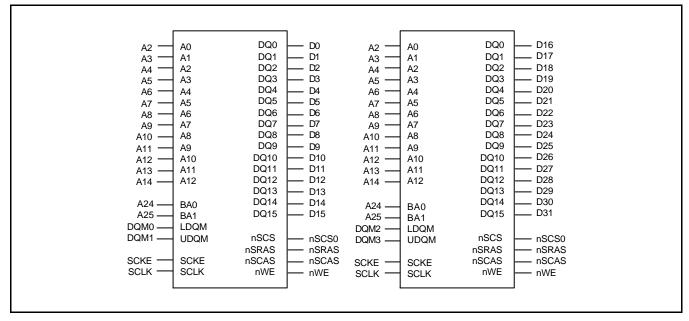
Figure 5-11. Memory Interface with 16-bit SDRAM (4Mx16x4Bank \* 2ea)
