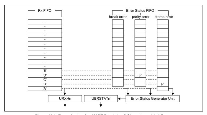
Figure 11-3. Example showing UART Receiving 5 Characters with 2 Errors
