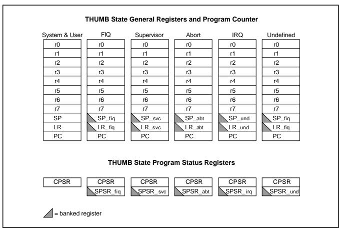
Figure 2-4. Register Organization in THUMB state
