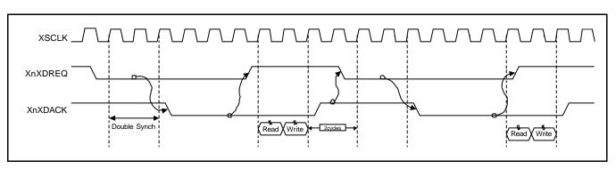
Figure 8-5. Single service in Handshake Mode with Unit Transfer Size
