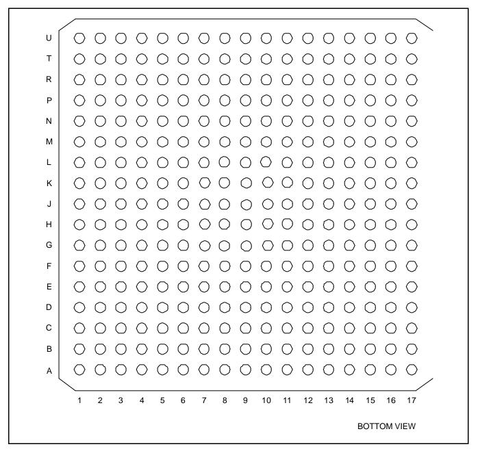
Figure 1-2. S3C2440A Pin Assignments (289-FBGA)
