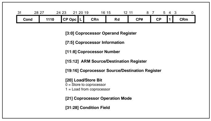
Figure 3-27. Coprocessor Register Transfer Instructions
