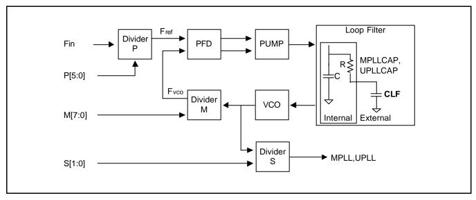
Figure 7-2. PLL (Phase-Locked Loop) Block Diagram
