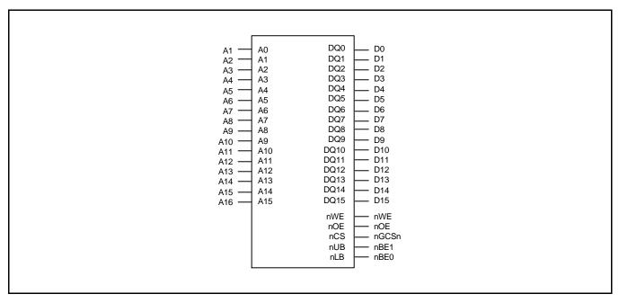
Figure 5-8. Memory Interface with 16-bit SRAM
