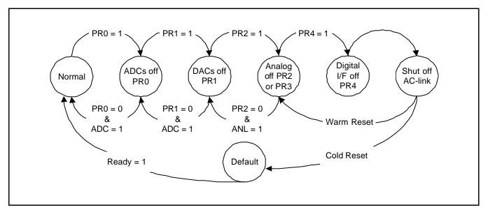
Figure 24-8. AC97 Power down/Power up Flow
