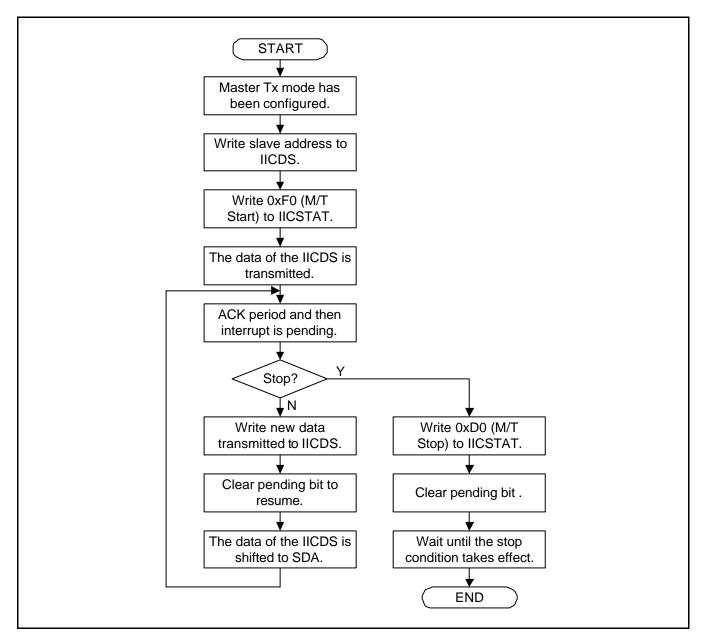
Figure 20-6. Operations for Master/Transmitter Mode
