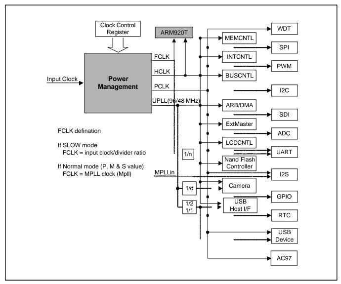
Figure 7-7. The Clock Distribution Block Diagram
