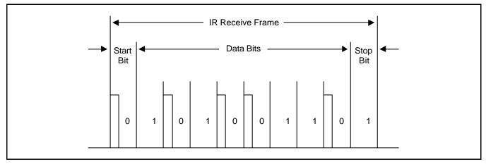
Figure 11-7. Infrared Receive Mode Frame Timing Diagram
