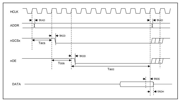
Figure 27-18. Masked-ROM Single READ Timing Diagram (Tacs=2, Tcos=2, Tacc=8, PMC=01/10/11)
