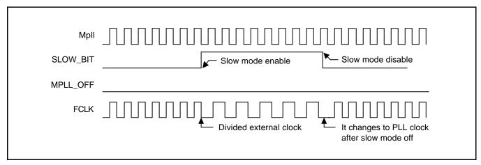
Figure 7-9. Issuing Exit\_from\_Slow\_mode Command in PLL on State
