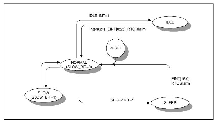
Figure 7-8. Power Management State Diagram
