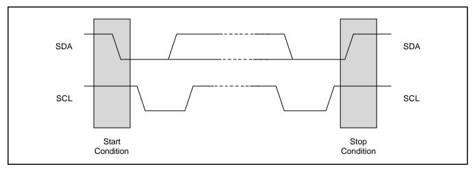
Figure 20-2. Start and Stop Condition
