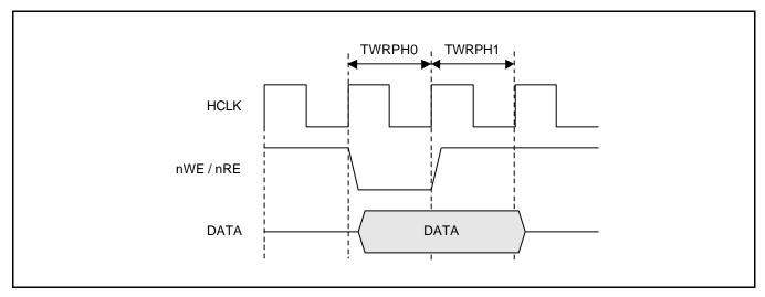
Figure 6-4. nWE & nRE Timing (TWRPH0=0, TWRPH1=0)
