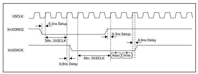
Figure 8-1. Basic DMA Timing Diagram
