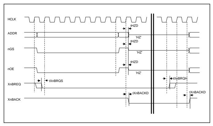
Figure 27-11. External Bus Request in ROM/SRAM Cycle (Tacs=0, Tcos=0, Tacc=8, Toch=0, Tcah=0, PMC=0, ST=0)
