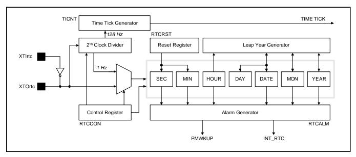
Figure 17-1. Real Time Clock Block Diagram
