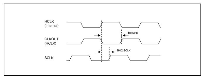
Figure 27-5. HCLK/CLKOUT/SCLK in case when EXTCLK is used
