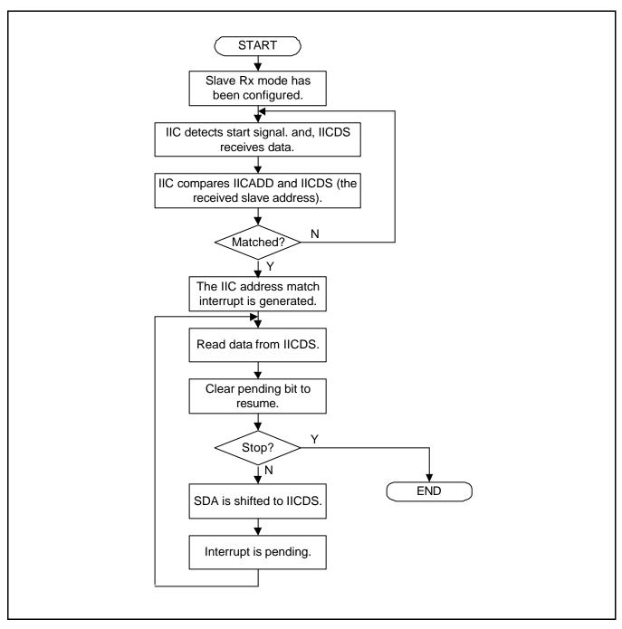
Figure 20-9. Operations for Slave/Receiver Mode
