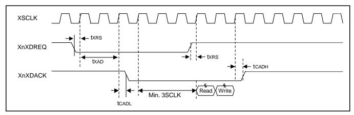
Figure 27-30. External DMA Timing Diagram (Handshake, Single transfer)
