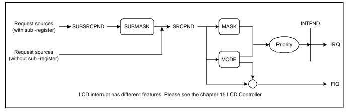
Figure 14-1. Interrupt Process Diagram
