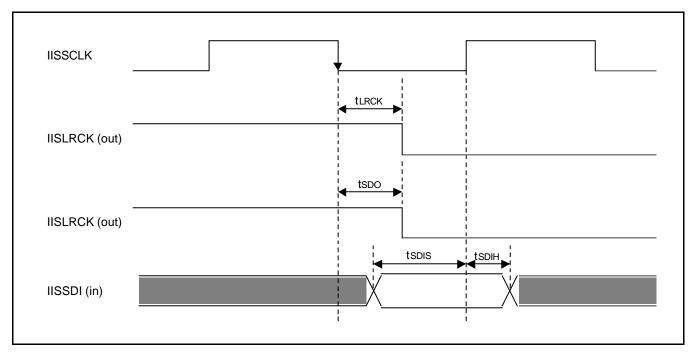
Figure 27-32. IIS Interface Timing Diagram
