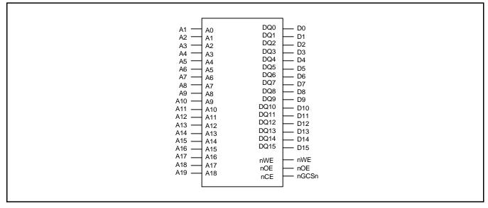
Figure 5-7. Memory Interface with 16-bit ROM
