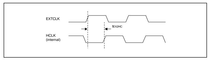
Figure 27-4. EXTCLK/HCLK in case when EXTCLK is used Without the PLL
