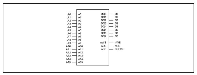
Figure 5-4. Memory Interface with 8-bit ROM
