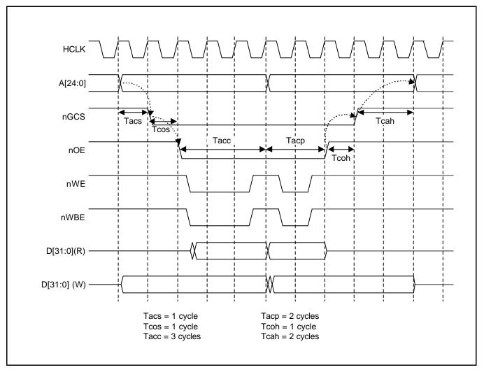
Figure 5-12. S3C2440A nGCS Timing Diagram
