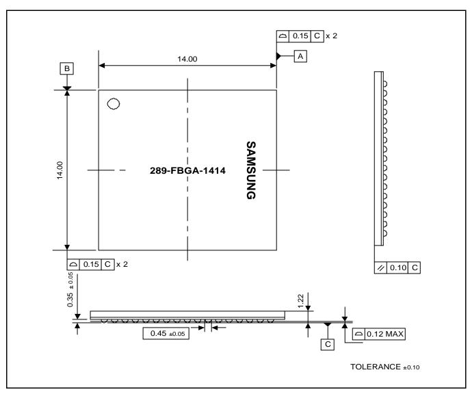
Figure 26-1. 289-FBGA-1414 Package Dimension 1 (Top View)
