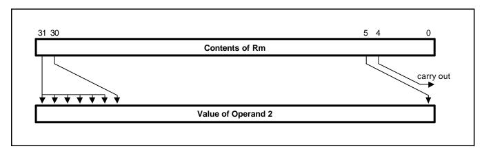
Figure 3-8. Arithmetic Shift Right
