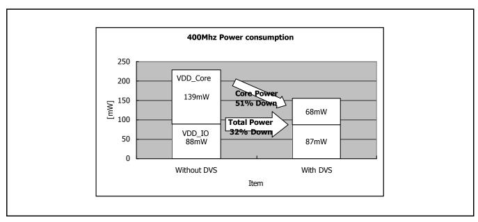
Figure 27-1. Power Consumption Example Comparison when Applied DVS Scheme
