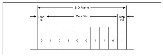
Figure 11-5. Serial I/O Frame Timing Diagram (Normal UART)
