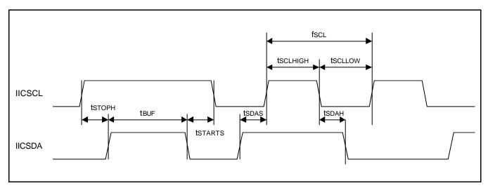
Figure 27-33. IIC Interface Timing Diagram
