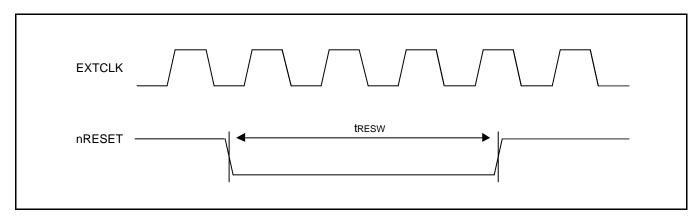
Figure 27-6. Manual Reset Input Timing Diagram
