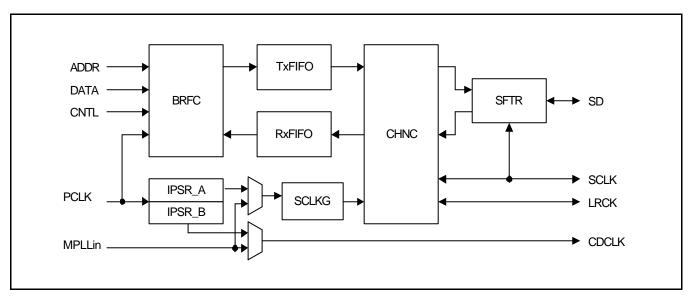
Figure 21-1. IIS-Bus Block Diagram
