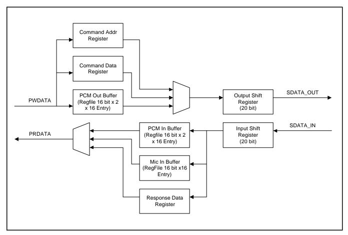
Figure 24-2. Internal Data Path
