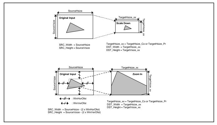
Figure 23-12. Scaling Scheme
