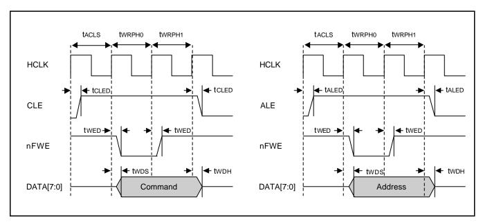
Figure 27-36. NAND Flash Address/Command Timing Diagram
