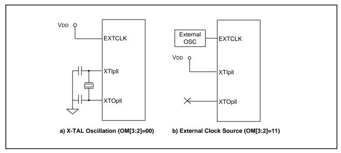
Figure 7-3. Main Oscillator Circuit Examples
