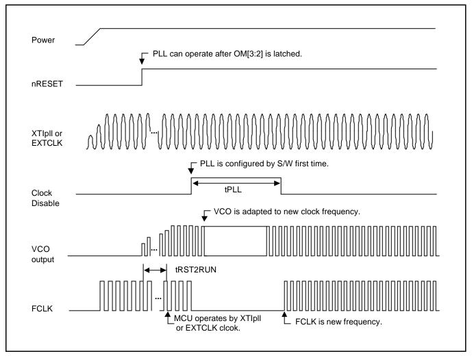
Figure 27-7. Power-On Oscillation Setting Timing Diagram
