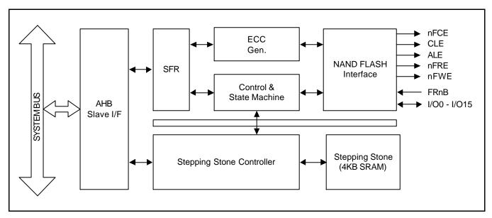
Figure 6-1. NAND Flash Controller Block Diagram
