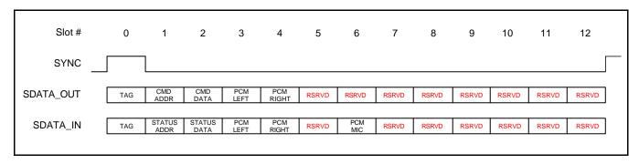
Figure 24-4. Bi-directional AC-link Frame with Slot Assignments
