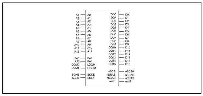
Figure 5-10. Memory Interface with 16-bit SDRAM (4Mx16, 4banks)
