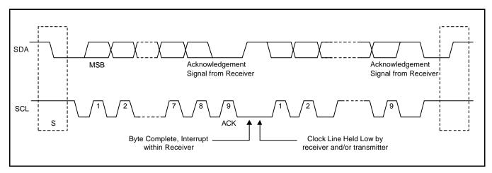
Figure 20-4. Data Transfer on the IIC-Bus
