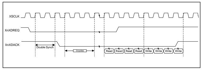
Figure 8-3. Burst 4 Transfer Size
