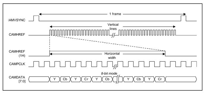
Figure 23-2. ITU-R BT 601 Input Timing Diagram
