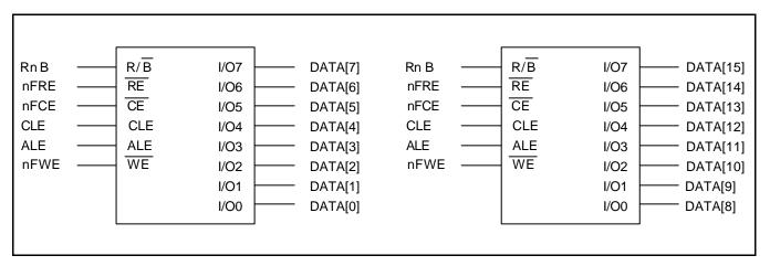
Figure 6-7. Two 8-bit NAND Flash Memory Interface
