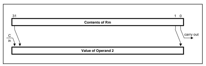
Figure 3-10. Rotate Right Extended
