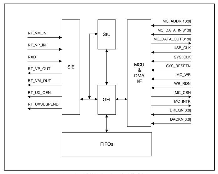
Figure 13-1. USB Device Controller Block Diagram
