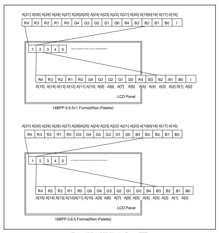
Figure 15-5. 16BPP Display Types (TFT)
