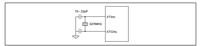
Figure 17-2. Main Oscillator Circuit Example
