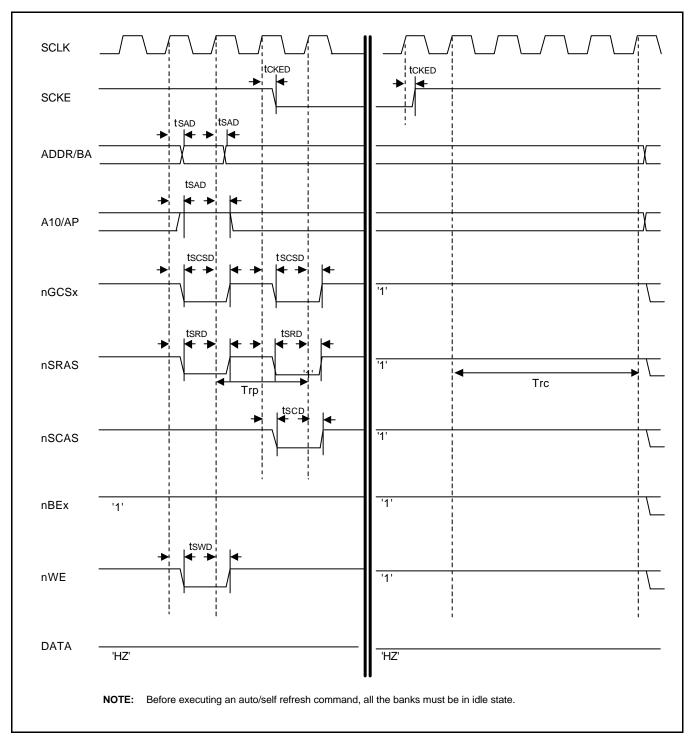
Figure 27-27. SDRAM Self Refresh Timing Diagram (Trp=2, Trc=4)
