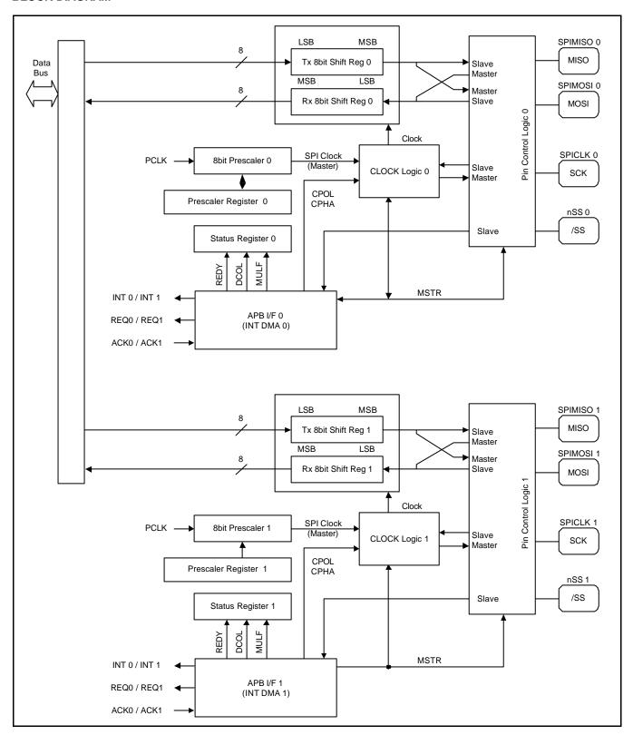
Figure 22-1. SPI Block Diagram
