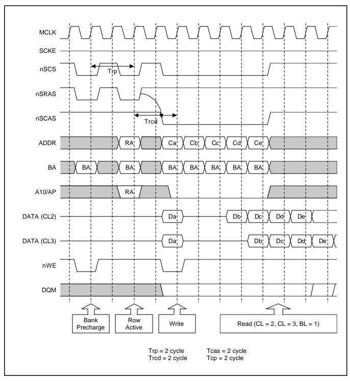
Figure 5-13. S3C2440A SDRAM Timing Diagram
