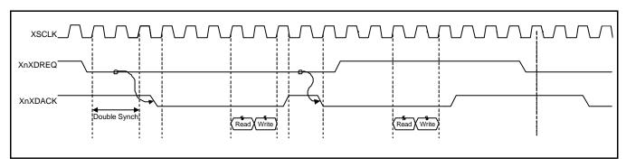
Figure 8-4. Single service in Demand Mode with Unit Transfer Size
