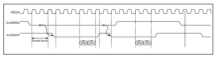
Figure 8-6. Whole service in Handshake Mode with Unit Transfer Size
