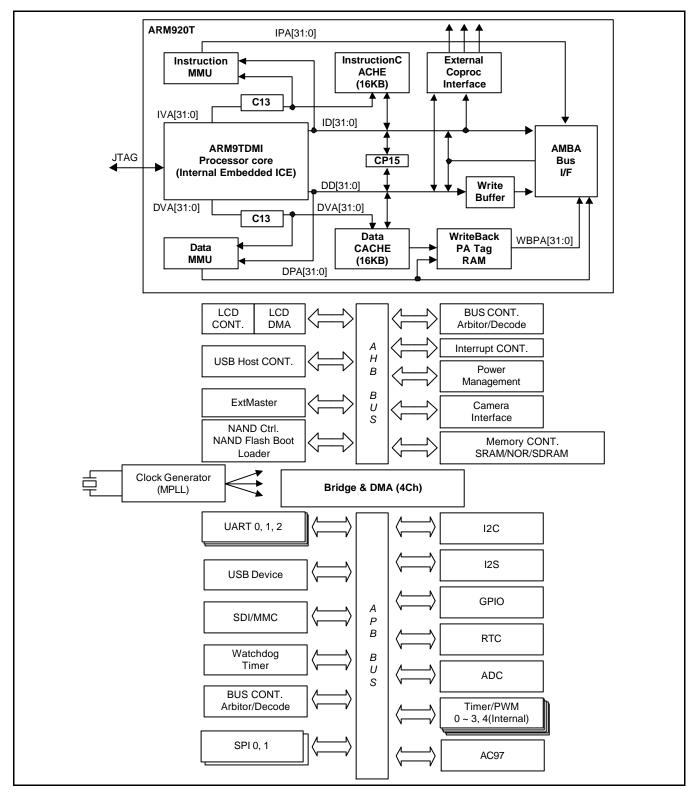
Figure 1-1. S3C2440A Block Diagram
