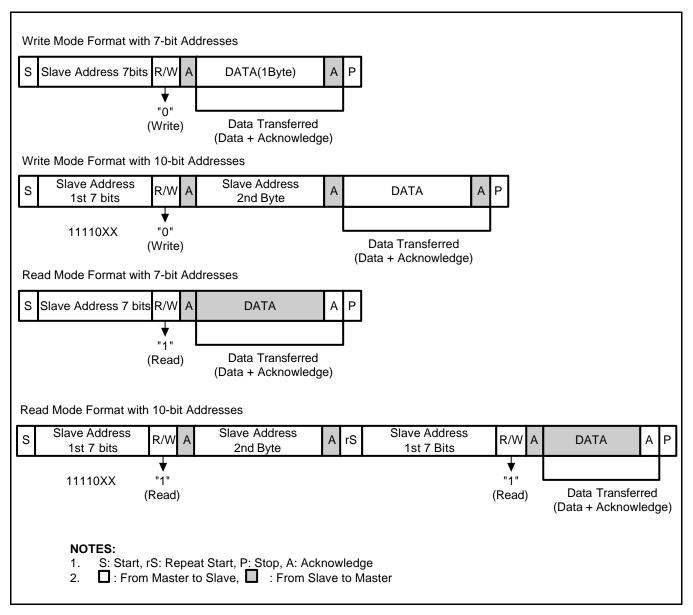
Figure 20-3. IIC-Bus Interface Data Format
