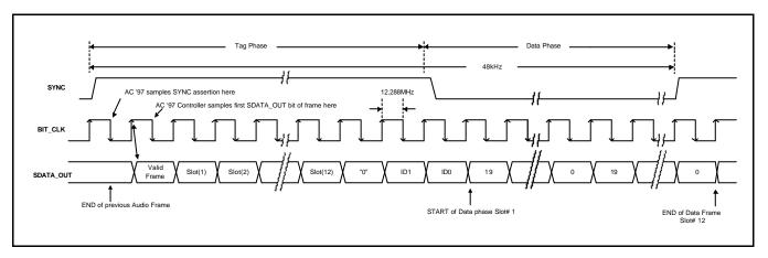
Figure 24-5. AC-link Output Frame
