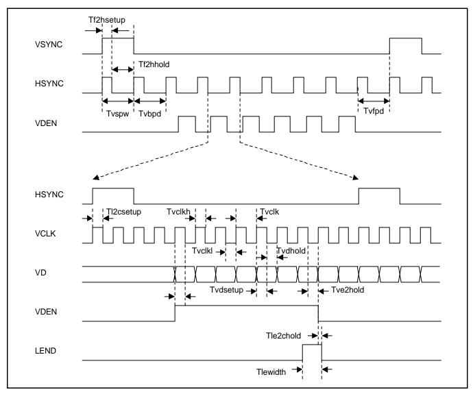
Figure 27-31. TFT LCD Controller Timing Diagram
