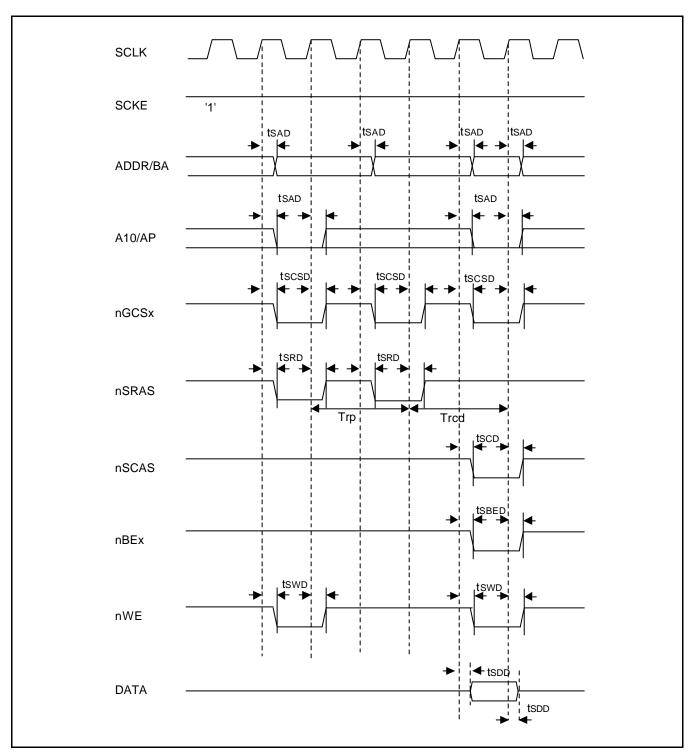
Figure 27-28. SDRAM Single Write Timing Diagram (Trp=2, Trcd=2)
