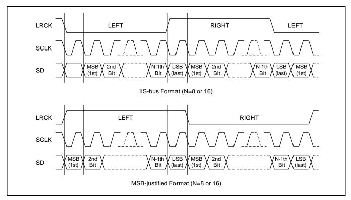
Figure 21-2. IIS-Bus and MSB (Left)-justified Data Interface Formats
