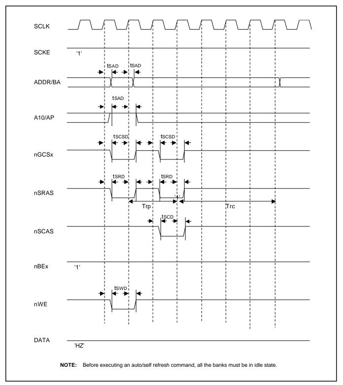
Figure 27-25. SDRAM Auto Refresh Timing Diagram (Trp=2, Trc=4)
