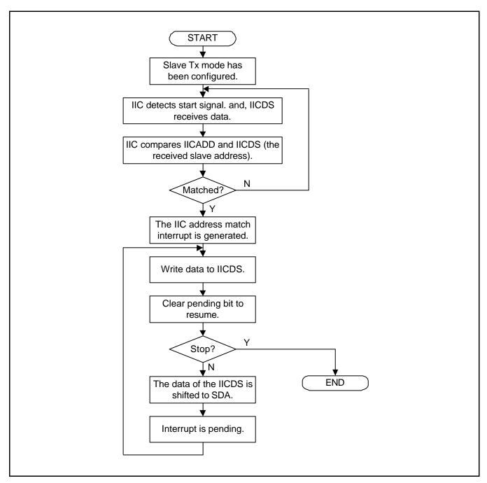
Figure 20-8. Operations for Slave/Transmitter Mode
