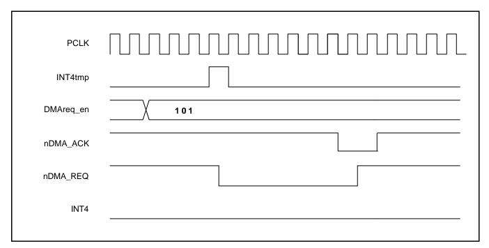
Figure 10-8. Timer4 DMA Mode Operation
