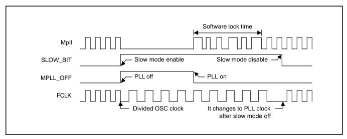
Figure 7-10. Issuing Exit\_from\_Slow\_mode Command After Lock Time
