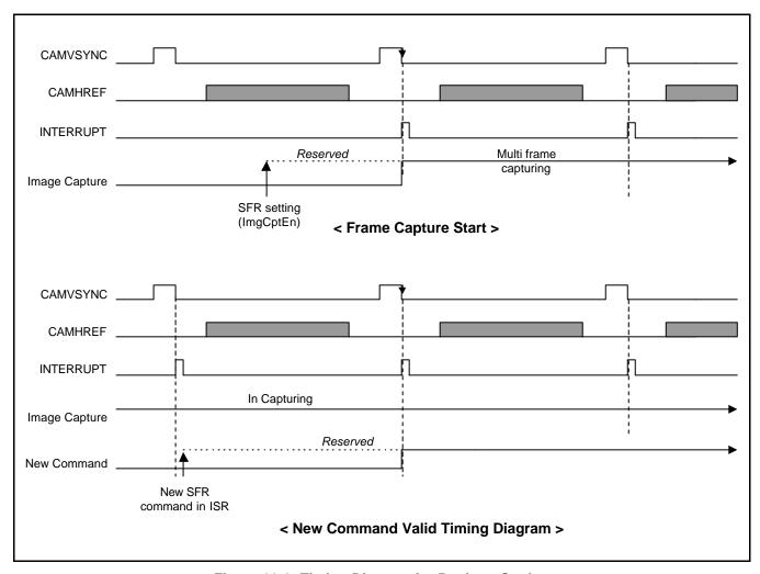
Figure 23-8. Timing Diagram for Register Setting
