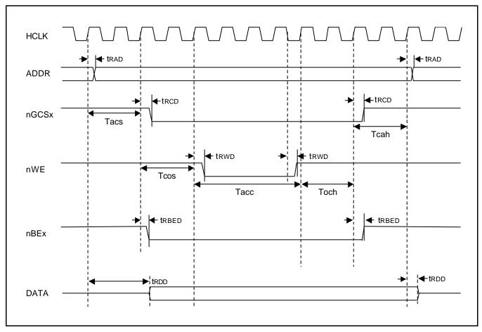
Figure 27-15. ROM/SRAM WRITE Timing Diagram (II) (Tacs=2, Tcos=2, Tacc=4, Toch=2, Tcah=2, PMC=0, ST=1)
