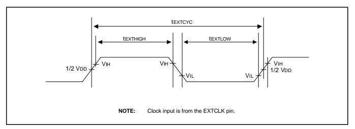
Figure 27-3. EXTCLK Clock Input Timing Diagram
