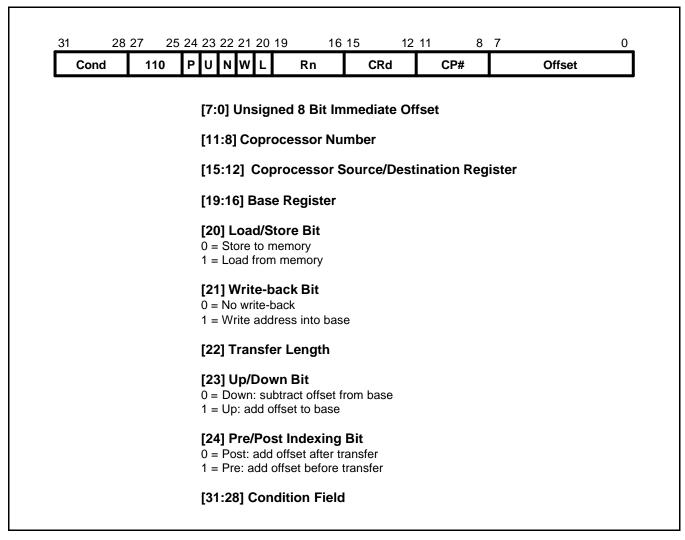
Figure 3-26. Coprocessor Data Transfer Instructions
