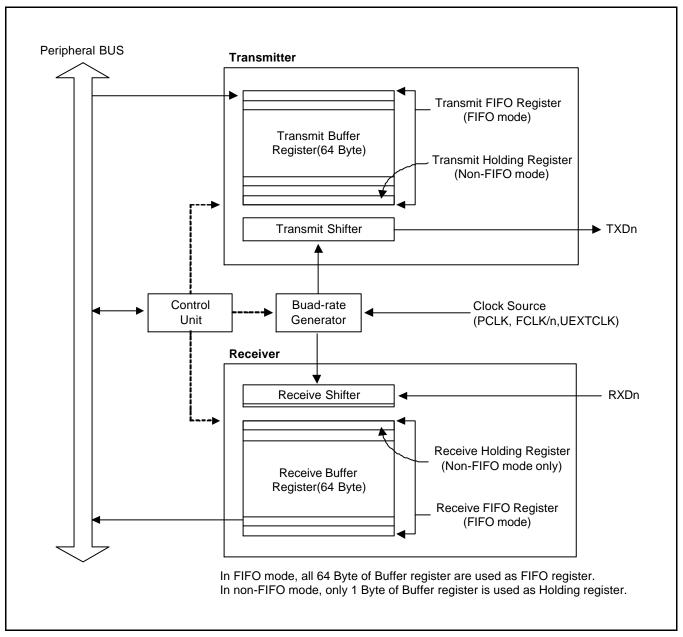
Figure 11-1. UART Block Diagram (with FIFO)
