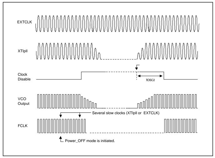
Figure 27-8. Sleep Mode Return Oscillation Setting Timing Diagram
