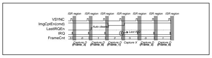
Figure 23-9. Timing diagram for last IRQ
