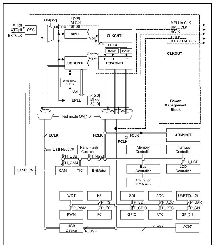
Figure 7-1. Clock Generator Block Diagram
