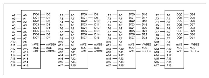
Figure 5-6. Memory Interface with 8-bit ROM x 4
