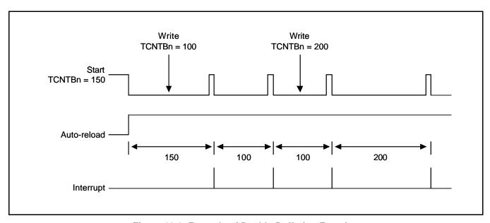
Figure 10-3. Example of Double Buffering Function
