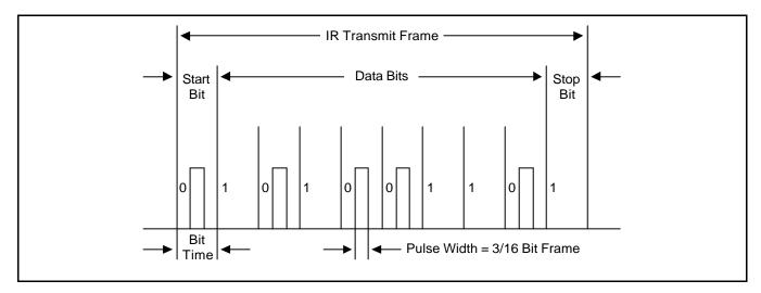
Figure 11-6. Infrared Transmit Mode Frame Timing Diagram
