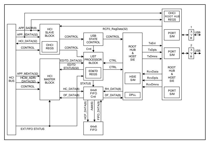
Figure 12-1. USB Host Controller Block Diagram
