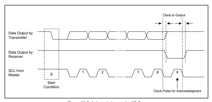
Figure 20-5. Acknowledge on the IIC-Bus
