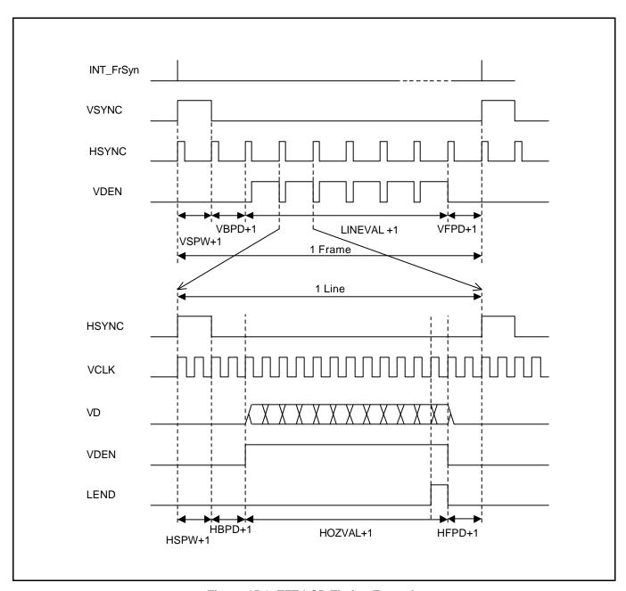
Figure 15-6. TFT LCD Timing Example
