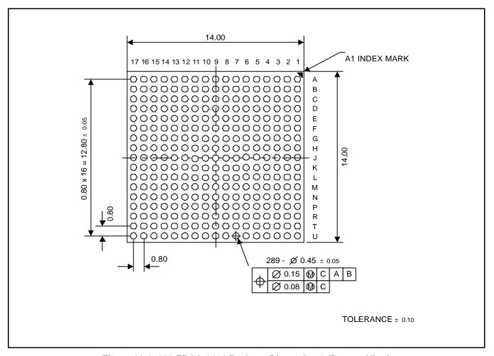
Figure 26-2. 289-FBGA-1414 Package Dimension 2 (Bottom View)
