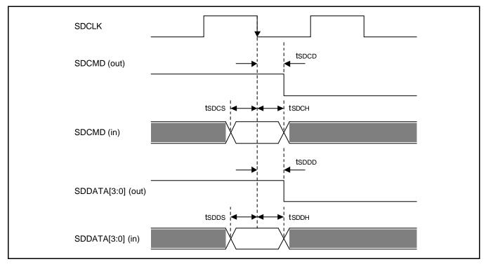
Figure 27-34. SD/MMC Interface Timing Diagram
