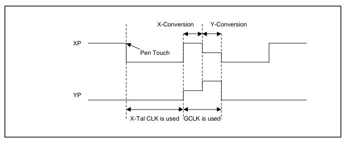
Figure 16-2. ADC and Touch Screen Operation signal
