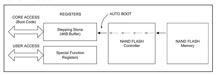
Figure 6-2. NAND Flash Controller Boot Loader Block Diagram
