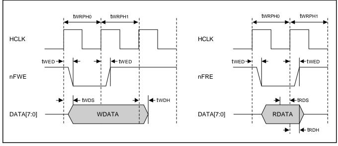
Figure 27-37. NAND Flash Timing Diagram
