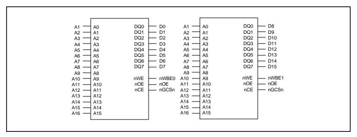
Figure 5-5. Memory Interface with 8-bit ROM x 2
