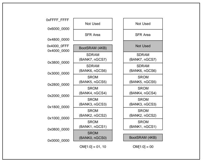
Figure 6-5. NAND Flash Memory Mapping
