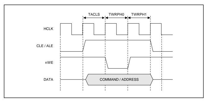
Figure 6-3. CLE & ALE Timing (TACLS=1, TWRPH0=0, TWRPH1=0)
