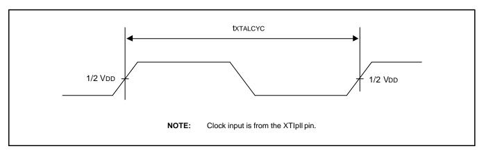
Figure 27-2. XTIpII Clock Timing Diagram
