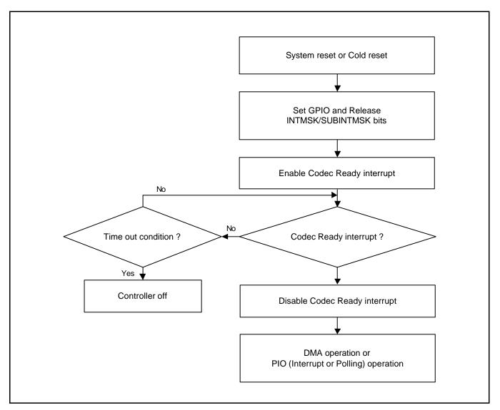
Figure 24-3. AC97 Operation Flow Chart
