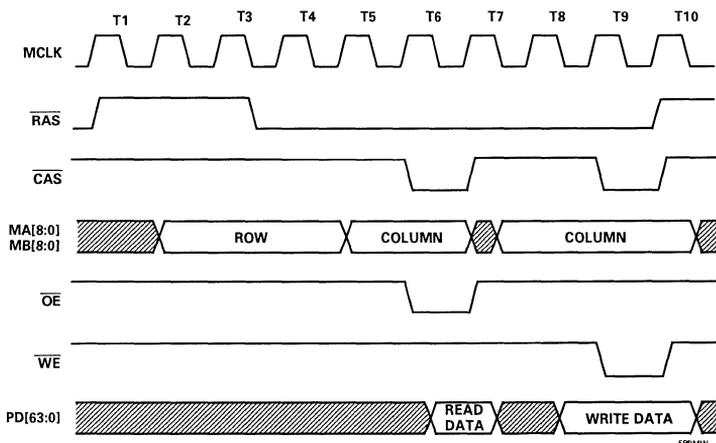
Figure 3-3. Fast Page Mode Read/Modify Write Timing
