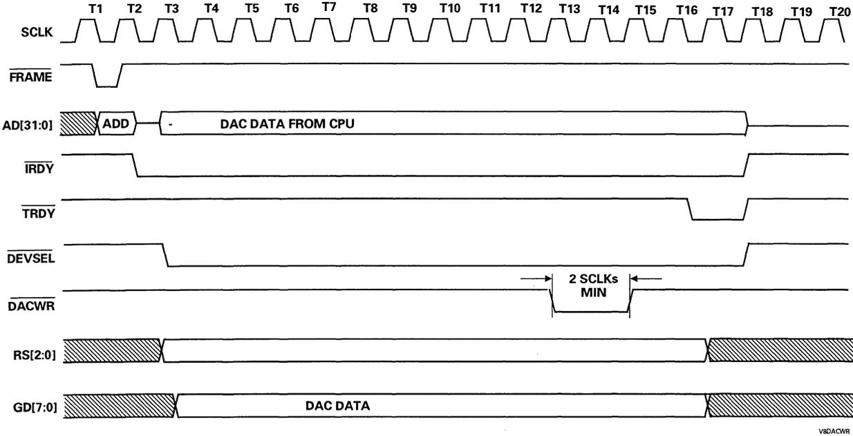
Figure 3-2. RAMDAC PCI Write Timing
