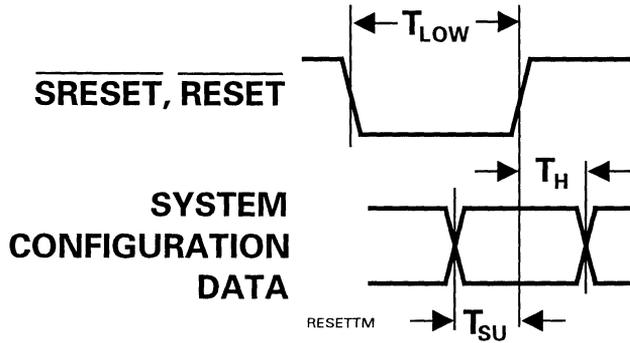
Figure 4-4. Reset Timing
