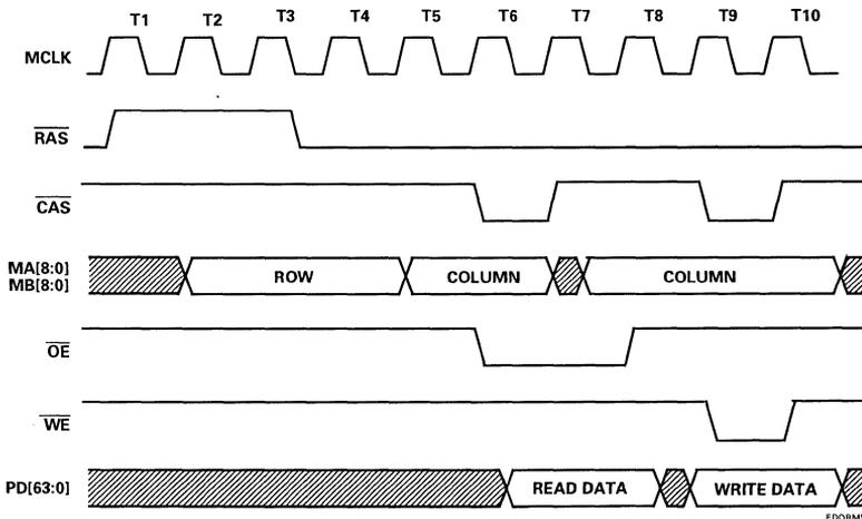
Figure 3-4. EDO Mode Read/Modify Write Timing
