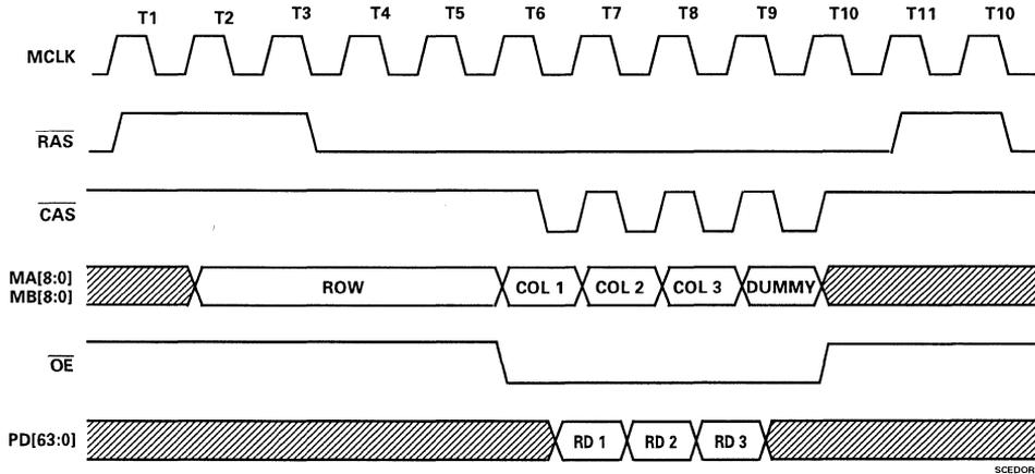
Figure 3-5. 1 Cycle EDO Read Timing
