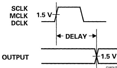
**Figure 4-3. Output Timing**
