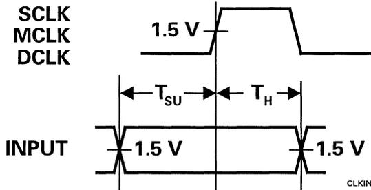
Figure 4-2. Input Timing
