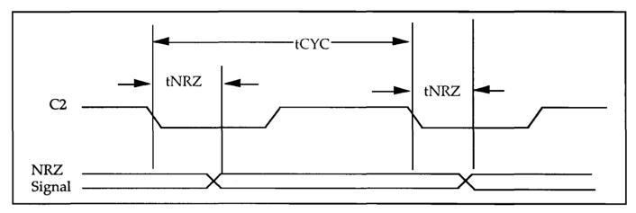
Figure 5-7. RESP, NMIP, and TSTP Input Waveforms
