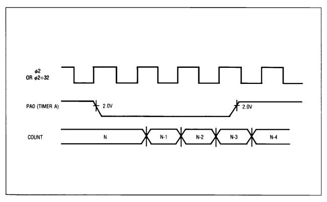
Figure 3-13. Pulse Width Measurement (Mode 3) Waveforms
