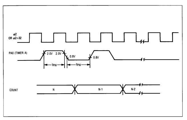
Figure 3-12. Event Counter (Mode 2) Waveforms
