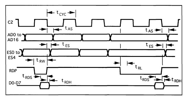
Figure 5-5. Expansion Bus Read Waveforms
