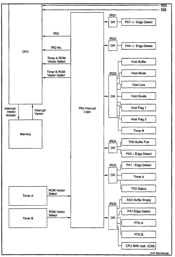
Figure 3-5. IRQ Interrupt Logic Interface
