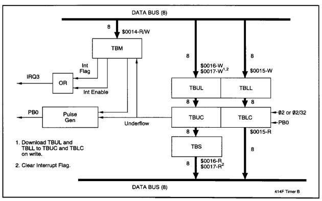
Figure 3-9 . Counter/Timer B Block Diagram
