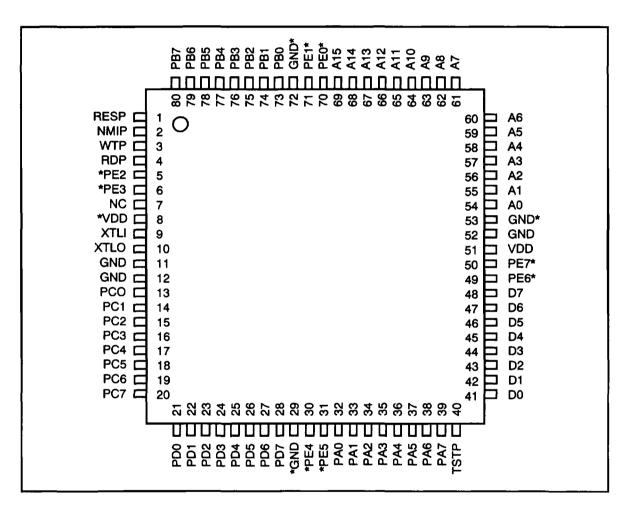
NOTE: \* Indicates pins not bonded in the 68 pin PLCC package.
