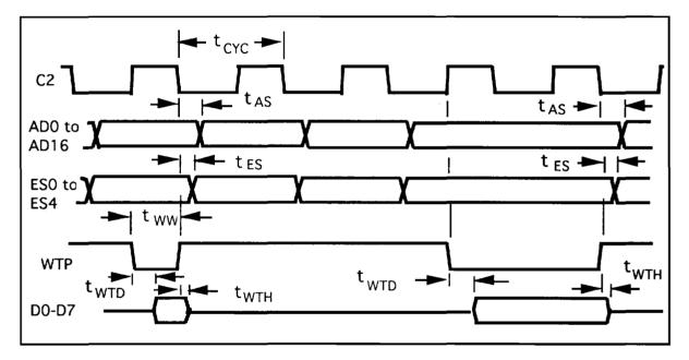
Figure 5-6. Expansion Bus Write Waveforms
