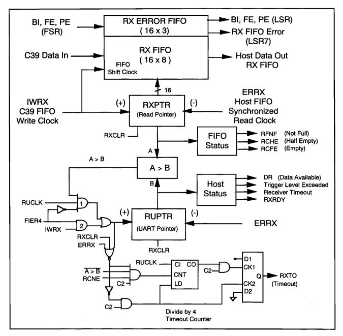
Figure 3-21. RX FIFO Block Diagram
