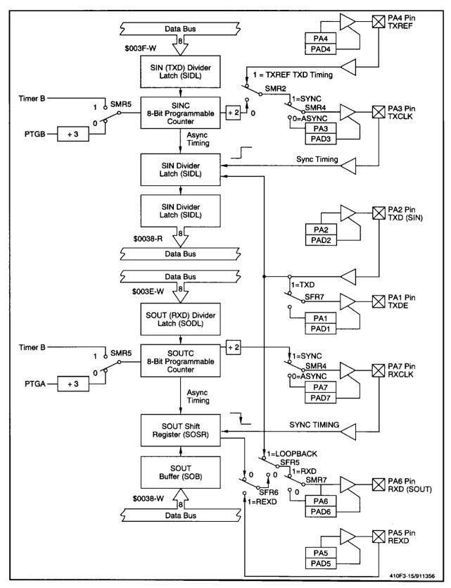
Figure 3-16. USART Block Diagram
