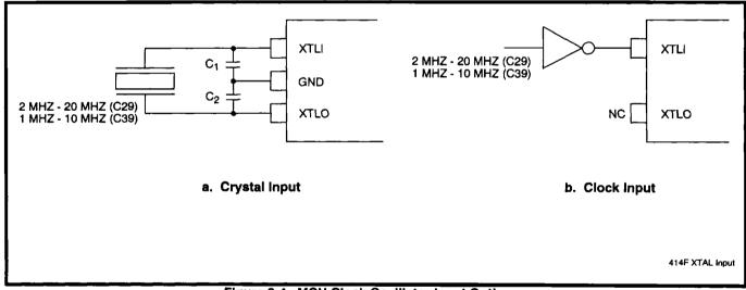
Figure 3-4. MCU Clock Oscillator Input Options
