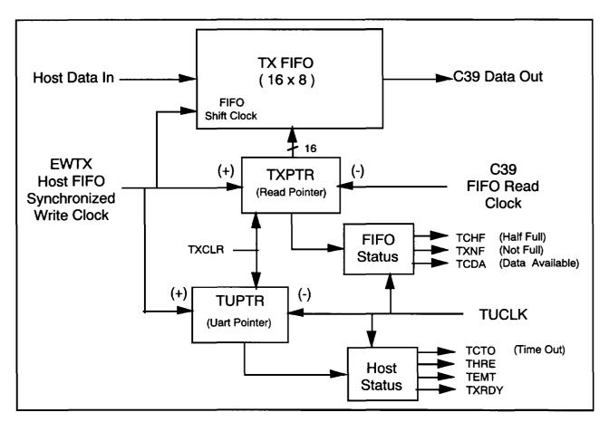
Figure 3-19. TX FIFO Block Diagram
