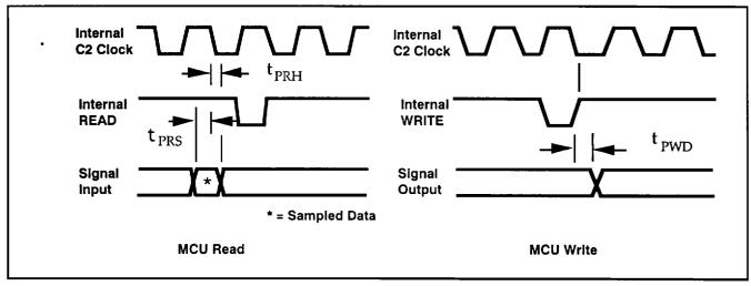
Figure 5-1. Port A, B, C, D, and E Read/Write Waveforms
