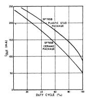
Fig. 8 SP765 operating characteristics ( $T_A = +70^{\circ}C$  max.)
