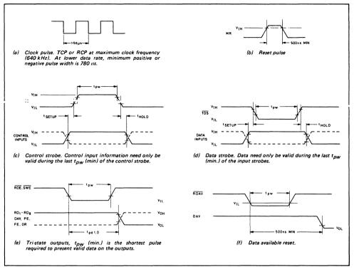
Fig.3 Timing diagrams
