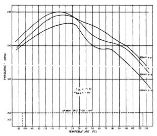
Fig. 5 Maximum input frequency v. temperature
