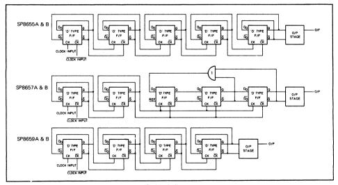
Fig.1 Logic diagrams
