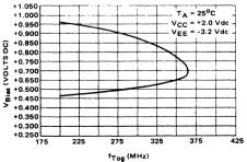
Figure 6 illustrates the variation in toggle frequency with the dc offset voltage (V<sub>Bias</sub>) of the input clock signal. V<sub>Bias</sub> is defined by the test circuit in Figure 4, and waveform Figure 5.
