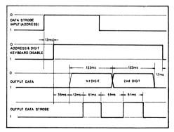
Fig. 4 Output timing Note: times specified are minimum.
