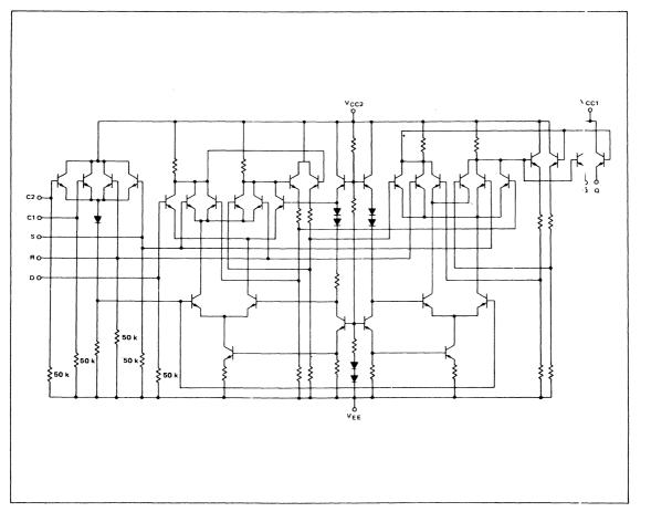
FIGURE 10 - SP1670 CIRCUIT SCHEMATIC
