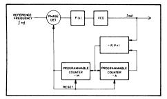
Fig. 9 Synthesiser block diagram (simplified)
