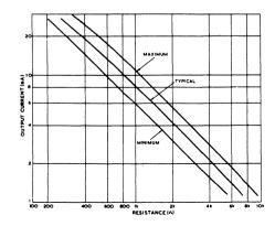
Fig. 2 Output current v. resistance between pin 2 and OV, assuming 5% tolerance on resistance
