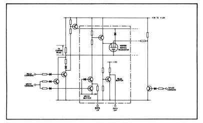
Fig.9 TTL - compatible memory application
