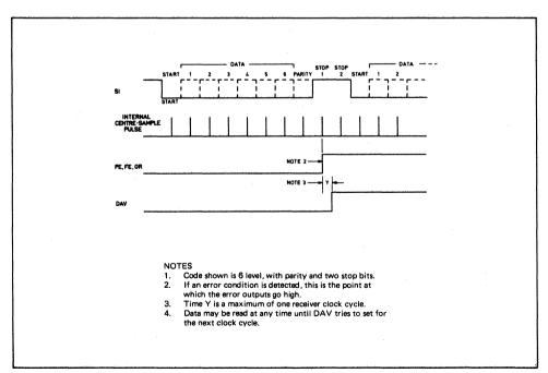
Fig.5 Receiver timing
