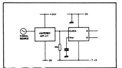
Fig. 7 The SP8616 driven by a commercially available nyorid amplifier. The Amperex ATF417 output is internally capacitively coupled.
