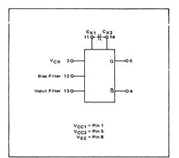
The SP1658 is a voltage-controlled multivibrator which provides appropriate level shifting to produce an output compatible with PSOL U and PSOL 10,000 logic levels. Frequency control is accomplished through the use of voltage-variable current sources which control the slew rate of a single external capacitor.
