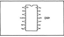
Fig. 1 Pin connections
