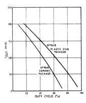
Fig. 7 SP764 operating characteristics ( $T_A = +70^{\circ}C max$ .)
