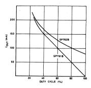
Fig. 6 Operating characteristics at +70°C
