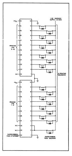
Fig.14 Typical printing calculator application
