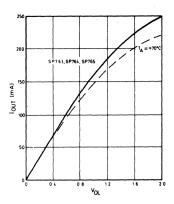
Fig. 5 Output characteristics ( $T_A = +25^{\circ}C$ )
