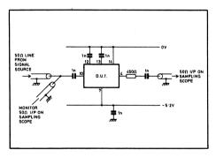
Fig.3 Test circuit.
