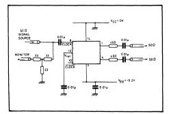
Fig. 3 Toggle frequency test circuit
