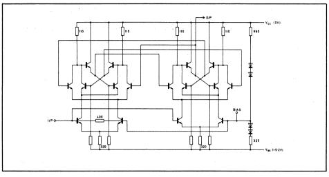
Fig.2 Circuit diagram of 1st element (÷2) showing input biassing arrangement.
