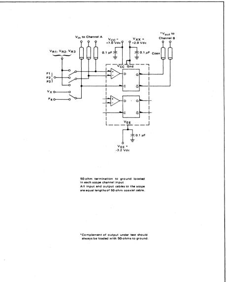
FIGURE 1 - SWITCHING TIME TEST CIRCUIT @ 25°C
