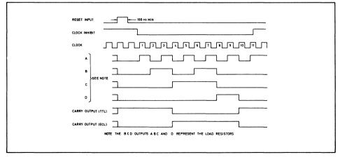
Fig. 5 Decade counter timing diagram
