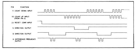
Fig. 4 Frequency comparator and filter timing
