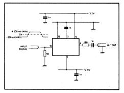
Fig. 4 Directly connecting the input signal (a useful technique at low frequencies)
