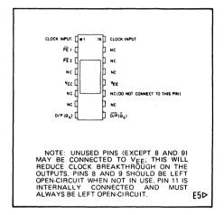
Fig. 1 Pin connections (top)
