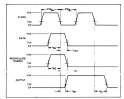
Fig. 3 Timing diagram and voltage wave forms
