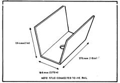
Fig. 13 Heatsink details for stud package
