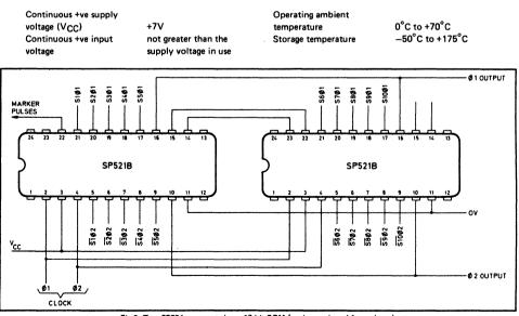
Fig.2 Two SP521s connected as a 10-bit BRM (packages viewed from above)
