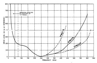
Fig.4 Minimum drive level v. I/P frequency at +25°C.
