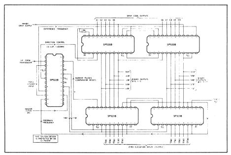
Fig. 5 Frequency-to-digital encoder
