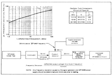
FIGURE 5 - NOISE DEVIATION TEST CIRCUIT AND WAVEFORM
