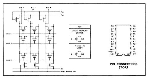
Fig.1 NOM401C circuit and pin connections
