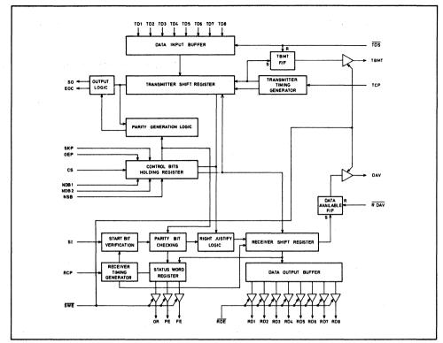
Fig.2 Functional block diagram
