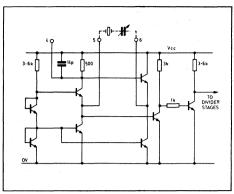
Fig. 3 Circuit diagram of SP705B oscillator
