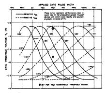
Fig.7 Write/Erase switching speed characteristics
