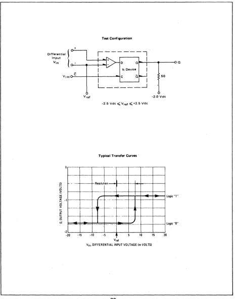
FIGURE 5 -- TRANSFER CHARACTERISTICS (Q versus V in)
