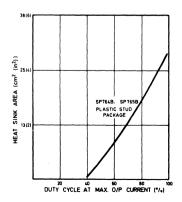
Fig. 9 Operating characteristics, stud package with heatsink (T\_A =  $+70^{\circ}$ C max.)
