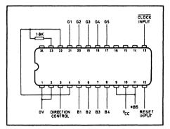
Fig.2 SP520 connected as a 5-bit counter
