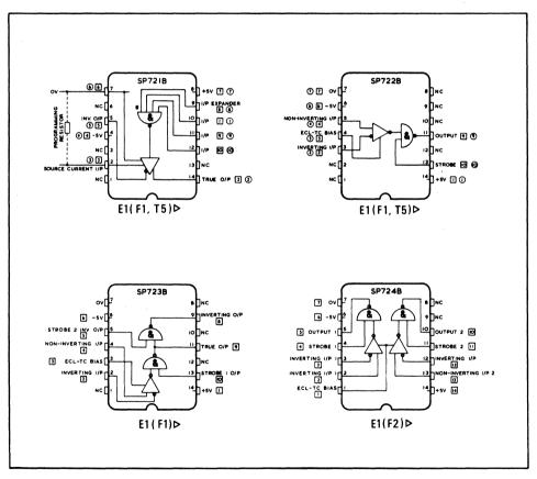
Fig. 1 Logic and dual-in-line peckage connection diagrams. Connections for peckage options shown thus: 🗆 = Flatpeck, O = TO-5.
