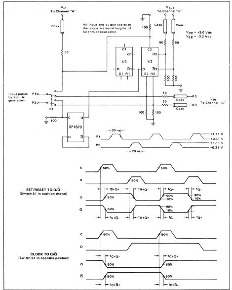
SWITCHING TIMES TEST CIRCUIT AND WAVEFORMS @ 25°C
