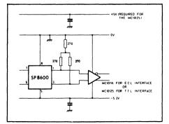
Fig. 7 ECL and Schottky TTL interfacing
