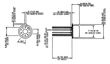
IO LEAD TO-IOO(5-84mm P.C.D.) WITH STANDOFF
