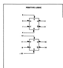
This device is a Dual Clocked Latch/R-S Flip-Flop. Whenever the Clock is low, the R-S inputs control the output state. Whenever the Clock is high, the output follows the data (D) input.
