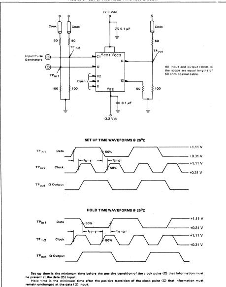
FIGURE 3 - SET UP AND HOLD TIME TEST CIRCUIT
