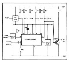
Fig. 4 Typical application configuration
