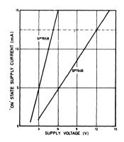
Fig. 10 Current drain per element ( $T_A = +70^{\circ}C$  max.)
