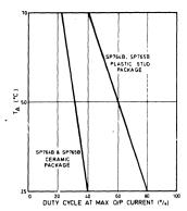
Fig. 6 Operating characteristics ( $T_A = +25^{\circ}C$  to  $+70^{\circ}C$ )
