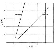
Fig. 3 Input characteristic (including strobe)  $T_{amb} = +25^{\circ}C$
