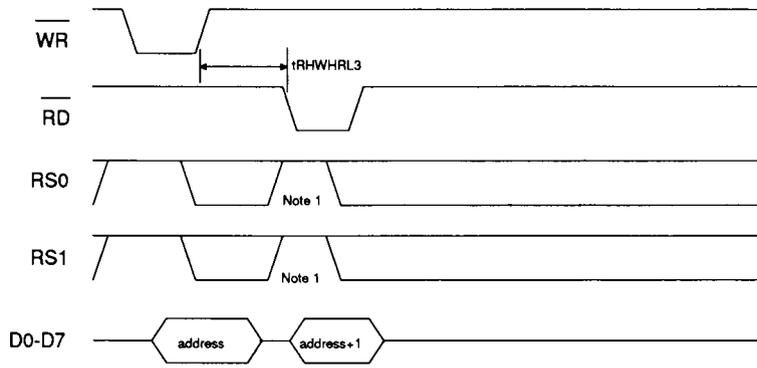
Note 1: The timing for reading from address 0.0 is identical to that for reading from address 1.1.
