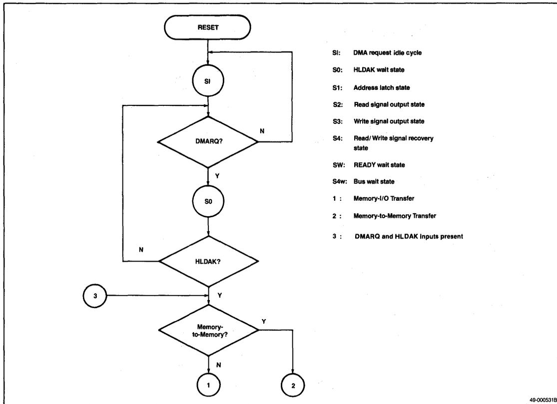
Figure 23. DMA Cycle, Cascade Mode
