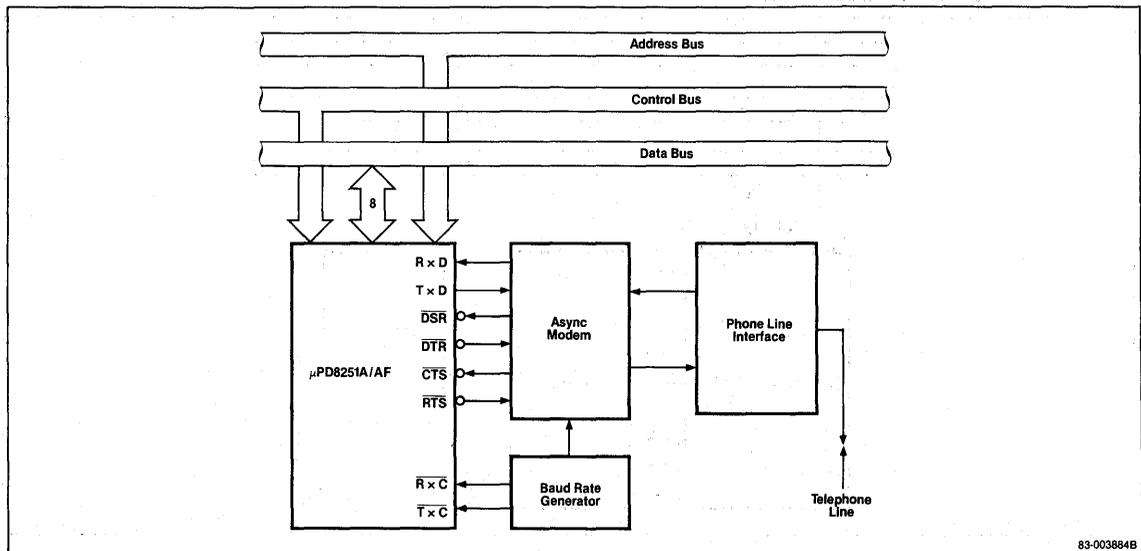
**Synchronous Interface to Terminal or Peripheral Device**
