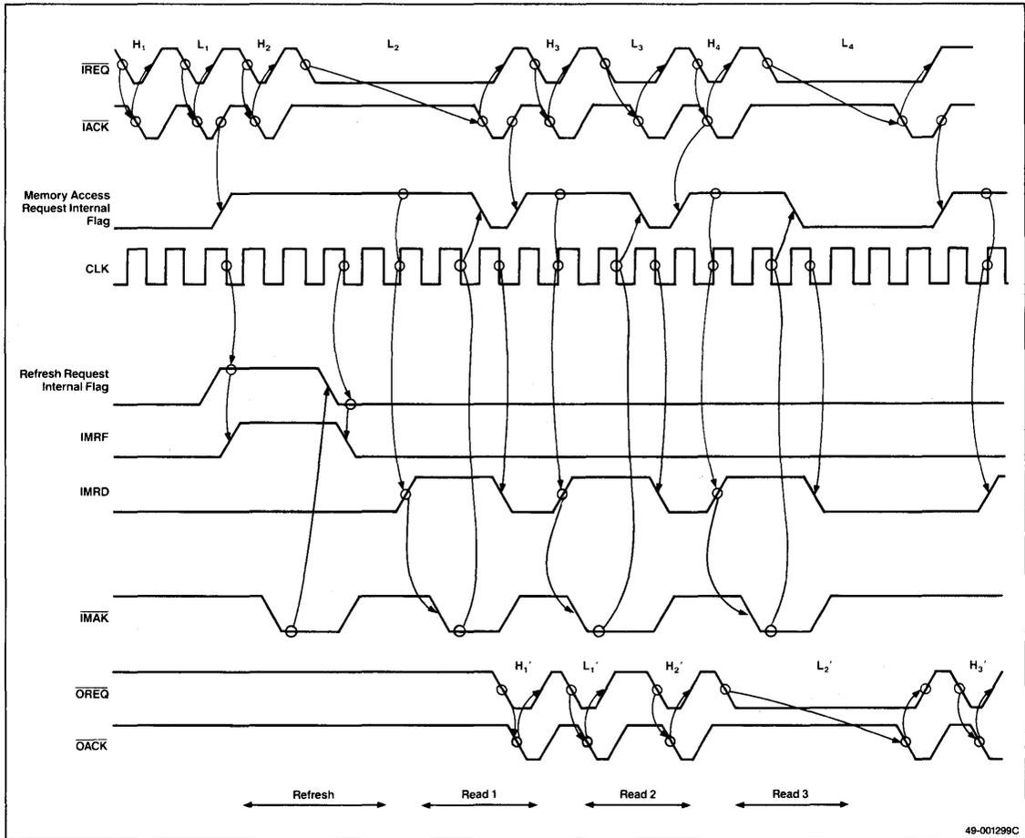
**Figure 18. Self Object Load Timing**
