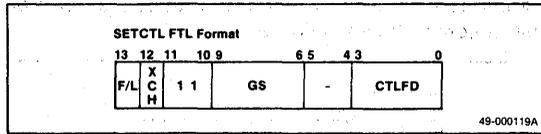
SETCTL is used to read and rewrite the contents of the Link Table and the Function Table. Since it can change the contents of the Link Table and the Function Table, this instruction can be used to write a self-modifying code. The type of operation to be performed is further specified by the contents of CTLFD field, as shown in table 22.
