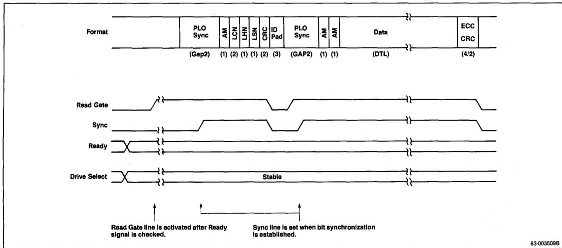
Figure 22. "Data Write" Timing (Soft Sector)
