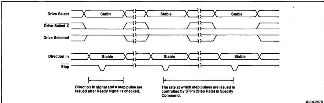
**Figure 20. "Buffered Seek" Timing (Soft Sector)**
