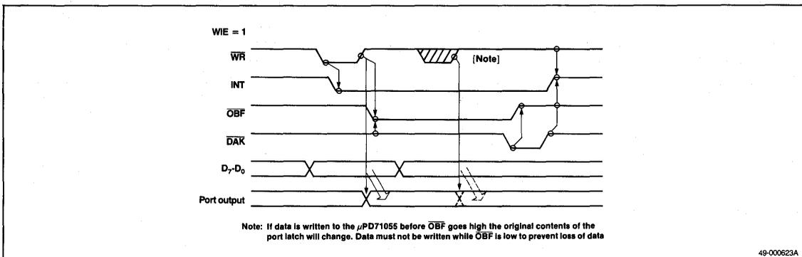
**DAK** [Data Acknowledge]. When this input is low, it signals the μPD71055 that output port data has been taken from the 71055.
