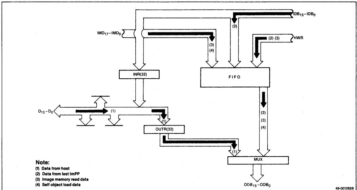
Figure 12. μPD7281, Input Control Data Flow
