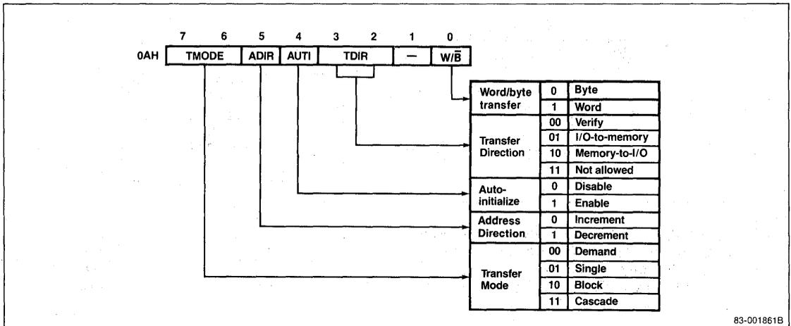
Figure 43. DMA Mask Register
