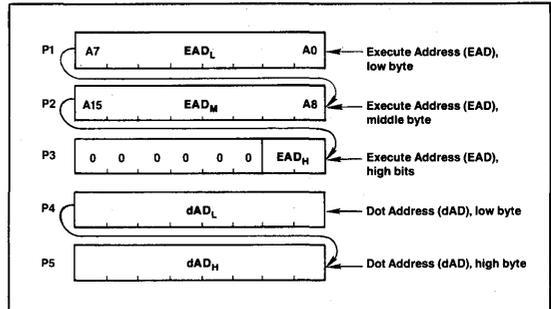
The execute address, EAD, points to the display memory word containing the pixel to be addressed.
