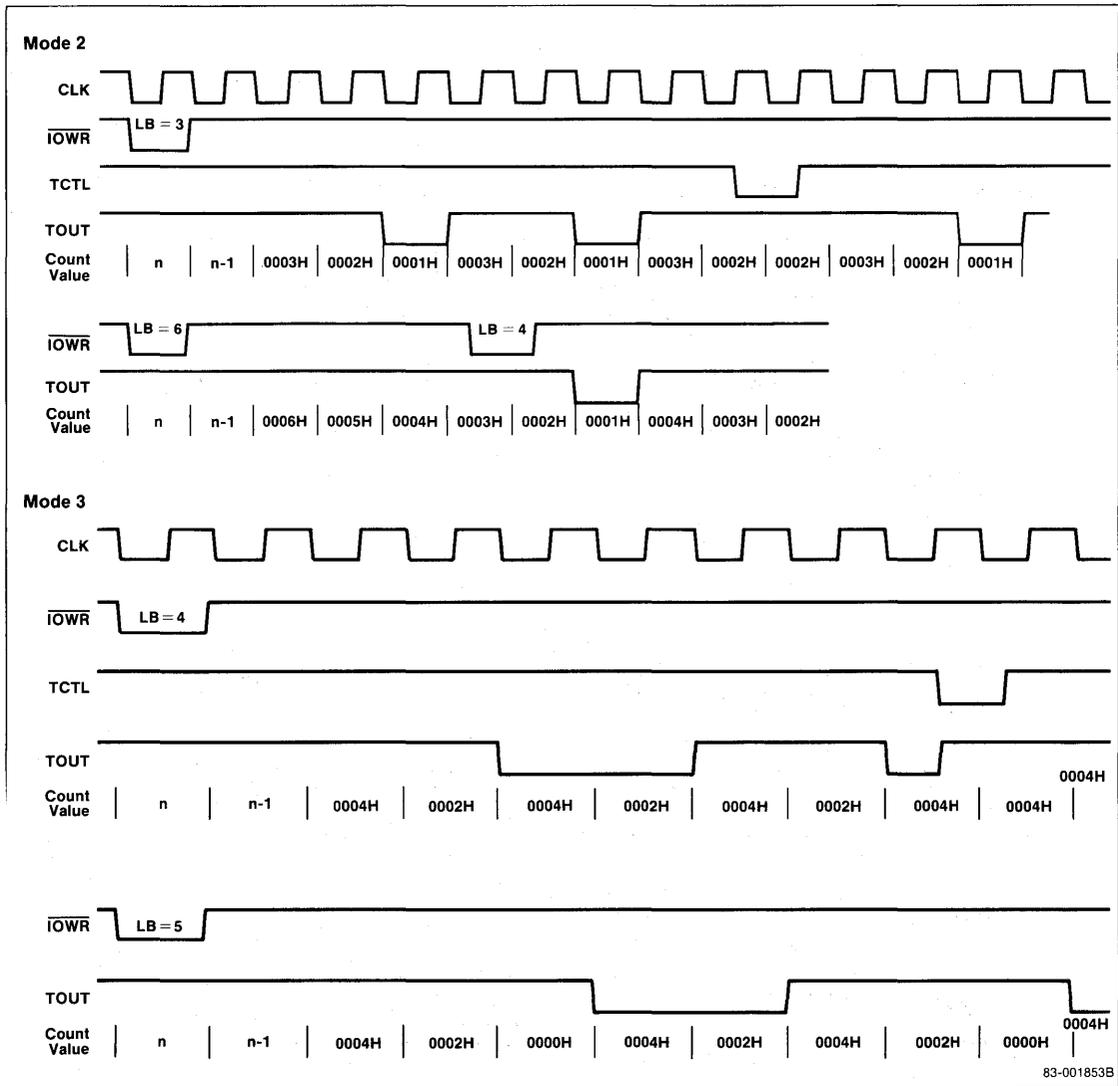
Figure 22. TCU Waveforms (Sheet 3 of 3)
