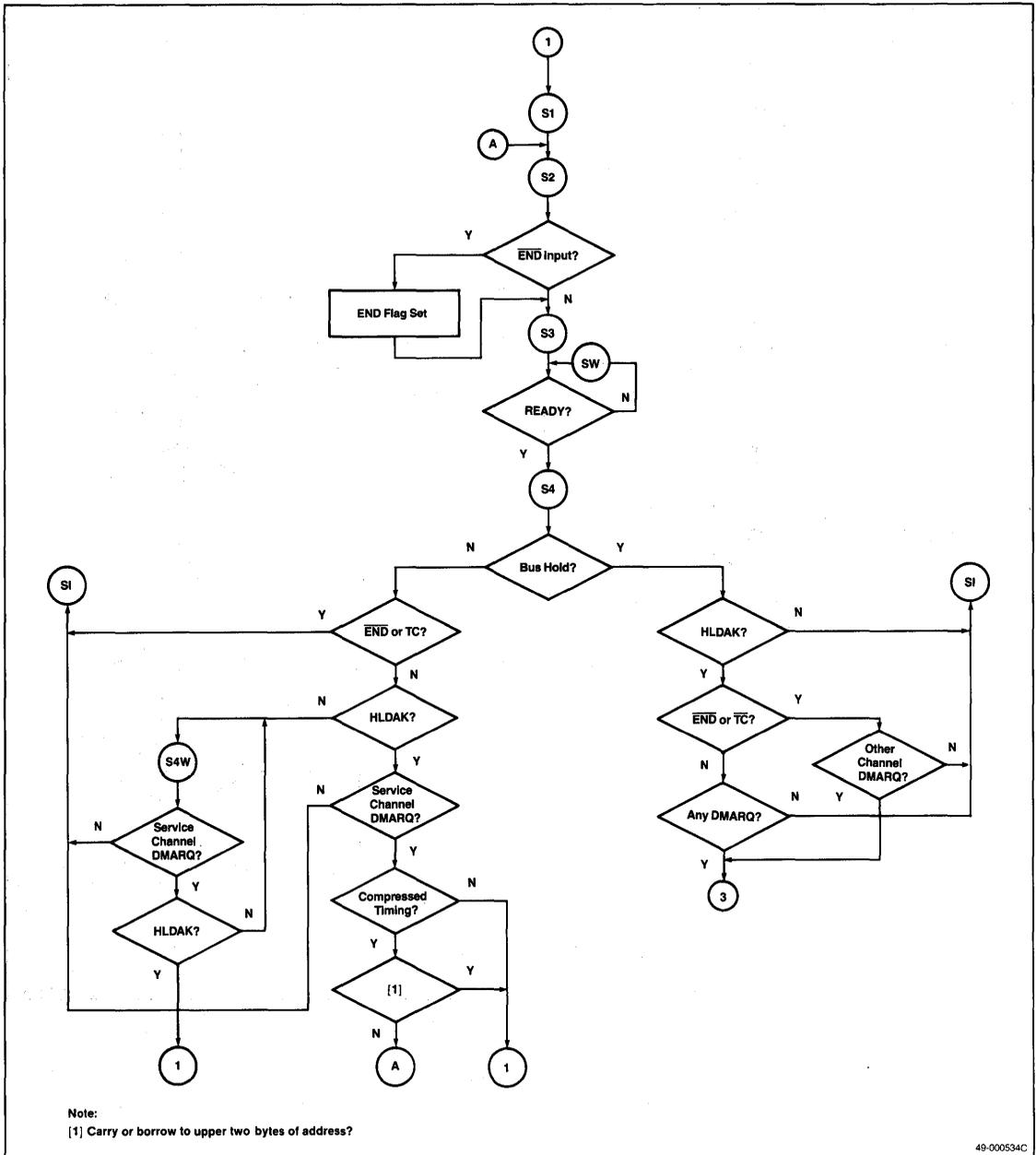
Figure 26. DMA Cycle, Block Mode
