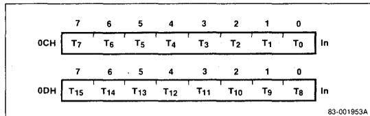
**Figure 20. Request Register Read/Write Format**
