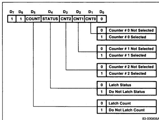
If the data that was latched is not read before a second multiple latch command is executed, the second command is ignored for those latches whose contents have not been read. This is because the data latched by the first command is held until it is read or until a new mode is set. When the data in the latch is read, the latch is released. See figure 7.
