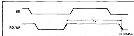
**AC Waveform Measurement Points (except CLK)**
