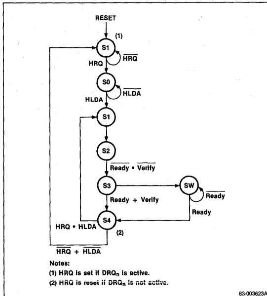
The DMA cycle consists of four internal states; S1, S2, S3, and S4. If the access time of the memory or I/O device is not fast enough to return a ready command to the μPD8257 after it reaches state S3, then a wait state is initiated (SW). One or more than one wait state occurs until a ready signal is received, and the μPD8257 is allowed to go into state S4. Either the extended write option or the DMA verify mode may eliminate any wait state.
