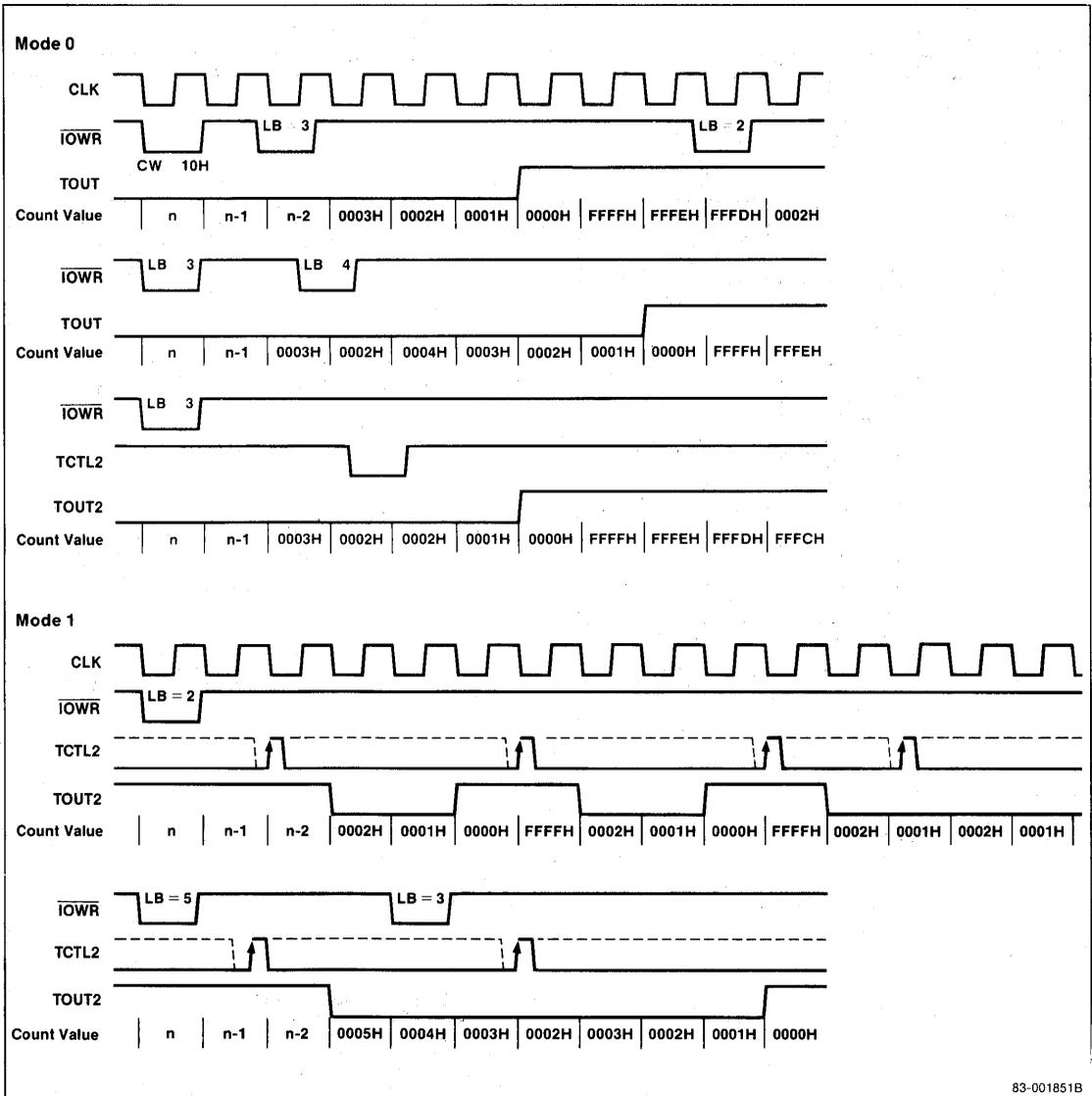
Figure 22. TCU Waveforms (Sheet 2 of 3)
