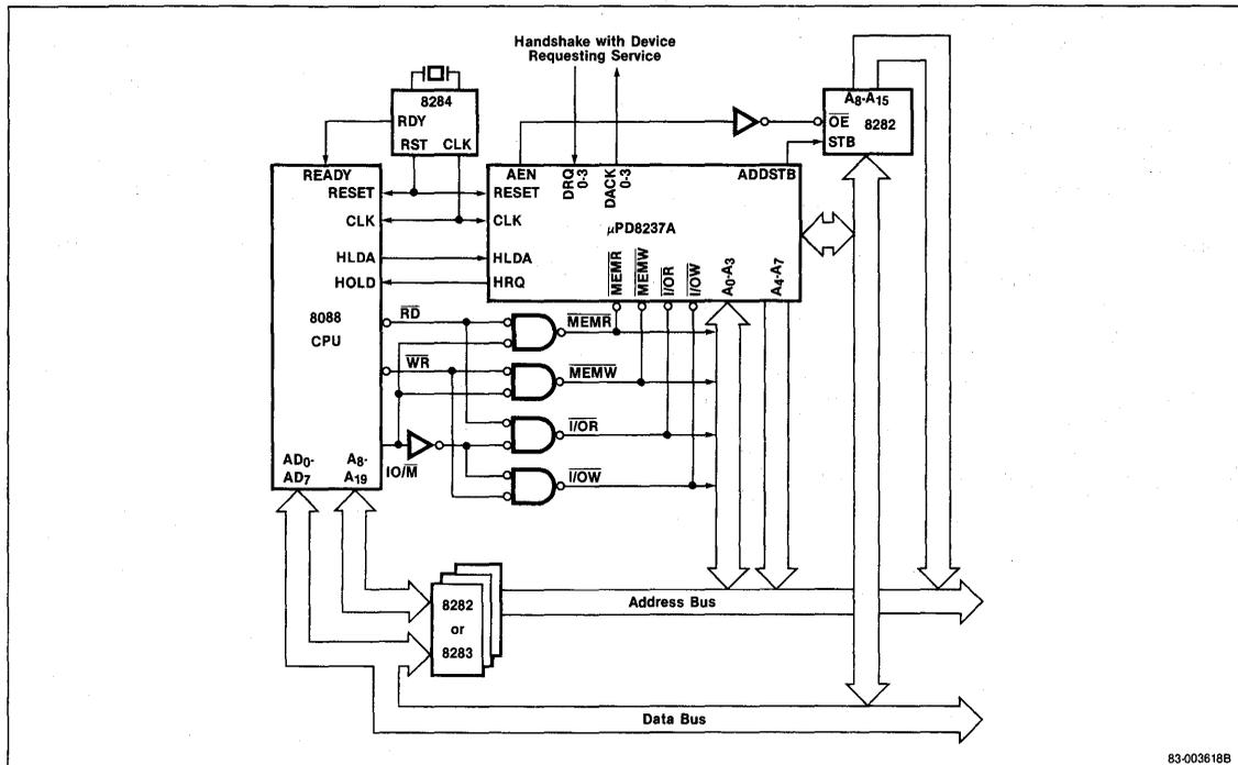
replies with an HLDA signal. The address for the first transfer appears in two bytes: the eight LSBs are output on A<sub>0</sub>-A<sub>7</sub> and the eight MSBs are output on the data bus pins. The contents of the data bus pins are latched to the 8282 to make up the 16 bits of the address bus. Once the address is latched, the data bus transfers data to or from a memory location or I/O device, using the control bus signals generated by the μPD8237A.
