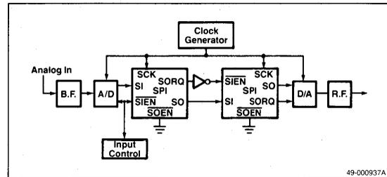
Figure 26. A Signal Processing System Using SPIs as a Complex Computer Peripheral
