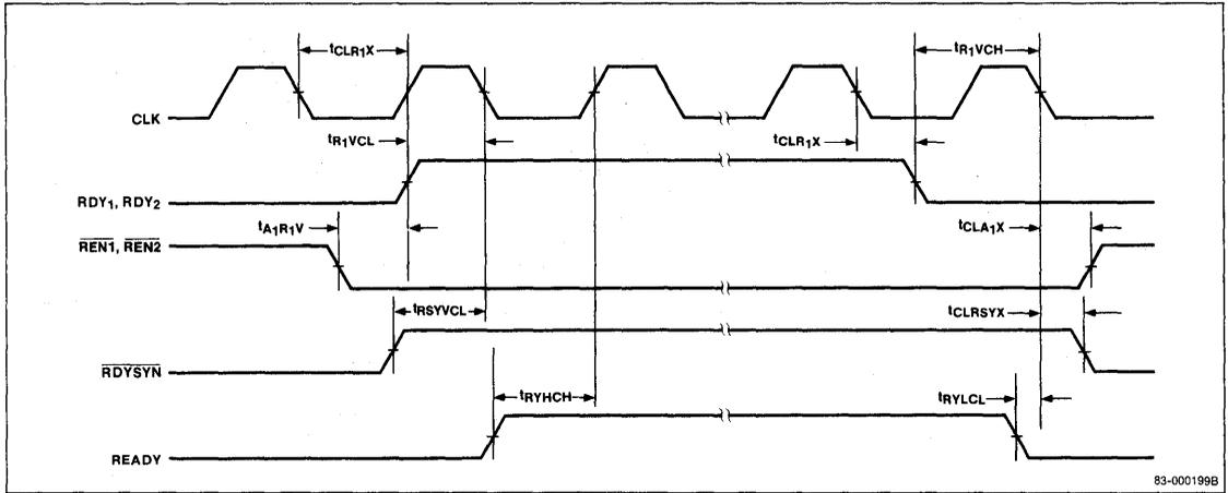
**Input/Output Waveform for AC Test**
