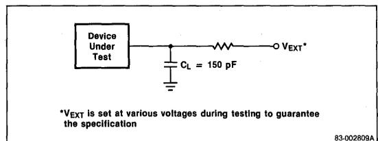
\*V<sub>EXT</sub> is set at various voltages during testing to guarantee the specification
