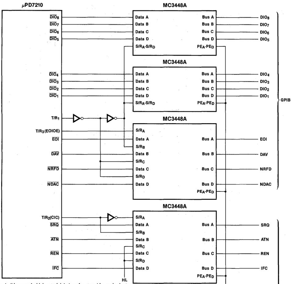
Note: In this example, high speed data transfer cannot be made since the bus transceiver is an open-collector type (set B<sub>2</sub> = 0).
