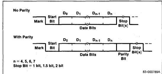
**Figure 11. Asynchronous Transmitter Example**
