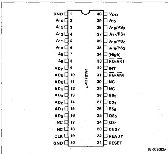
**Figure 3. Pin Configuration for V40 Mode (μPD70208 Microprocessor)**
