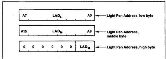
The light pen address, LAD, corresponds to the display word address, DAD, at which the light pen input signal is detected and deglitched.
