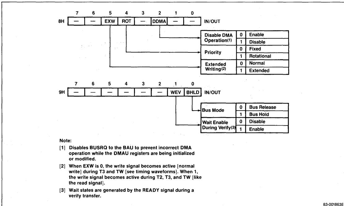
**Figure 41. DMA Status Register**
