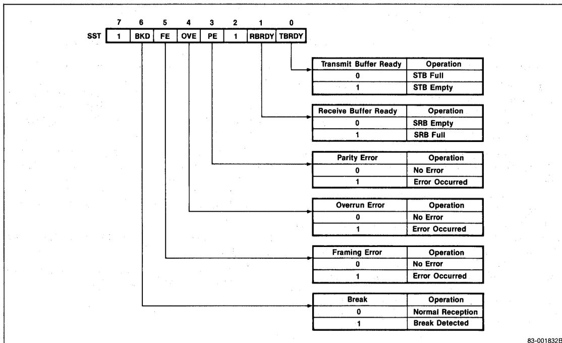
The SST register (figure 24) contains the status of the transmit and receive data buffers and the error flags. Error flags are persistent. Once an error flag is set, it remains set until a clear error flags command is issued.
