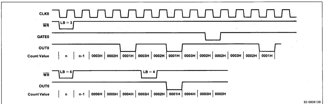
**Mode 2 Program Example.** This subroutine generates an interrupt to the CPU each time 10000 (decimal) clock pulses elapse. Counter 0 is in 2-byte mode and binary counting. See figure 13.
