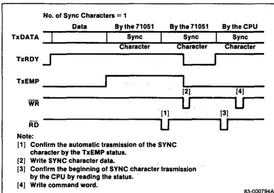
Automatic transmission of SYNC characters begins after the CPU sends new data. SYNC characters are not automatically sent by enabling the transmitter. Figure 16 shows these timing sequences.
