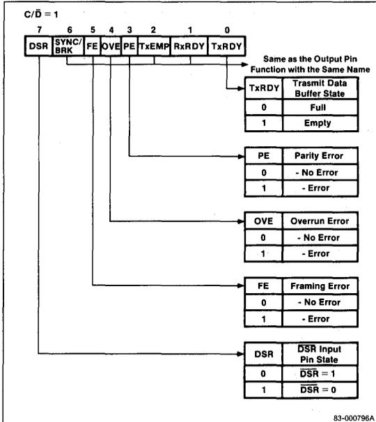
Framing, overrun, and parity errors do not disable the μPD71051's operations. All three error flags are cleared to 0 by a command byte that sets the ECL bit to 1.
