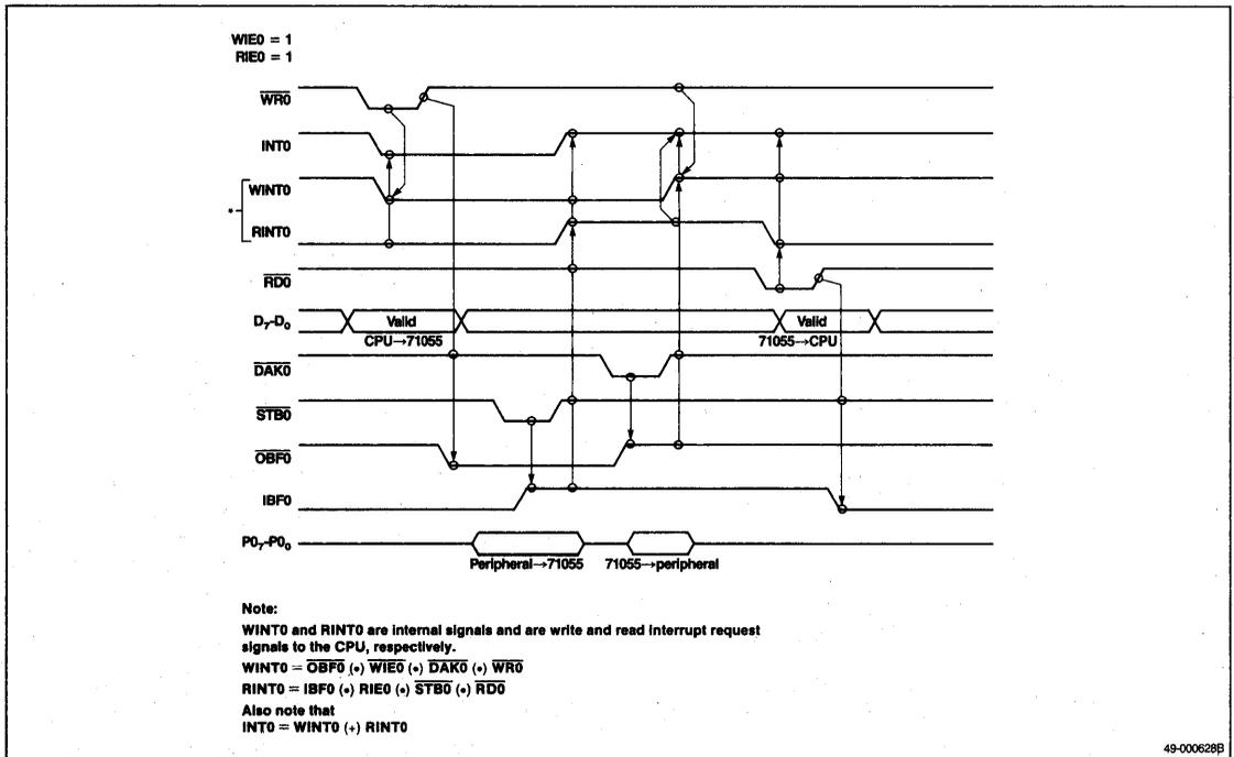
**RIE0 [Read Interrupt Enable Flag].** RIE0 controls the read interrupt request output. Interrupts are enabled by using the bit manipulation command to set this bit to 1 and disabled by setting it to 0. The state of RIE0 does not affect the  $\overline{\text{STB0}}$  function of this pin.
