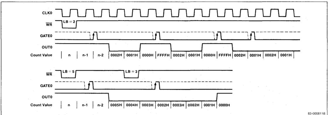
**Mode 1 Program Example.** This subroutine waits until no trigger is generated for an interval of 200 or more CLK pulses after the first gate trigger and returns to the main program. Counter 1 is set to low-byte read/write mode and binary count. See figure 11.
