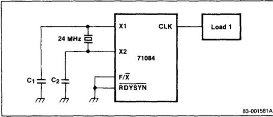
**Test Circuit for CLK High or Low Time
