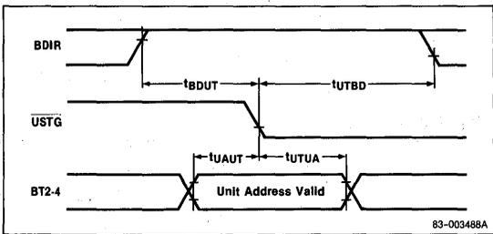
**Bit Bus Timing, Servo Offset/Data Strobe**
