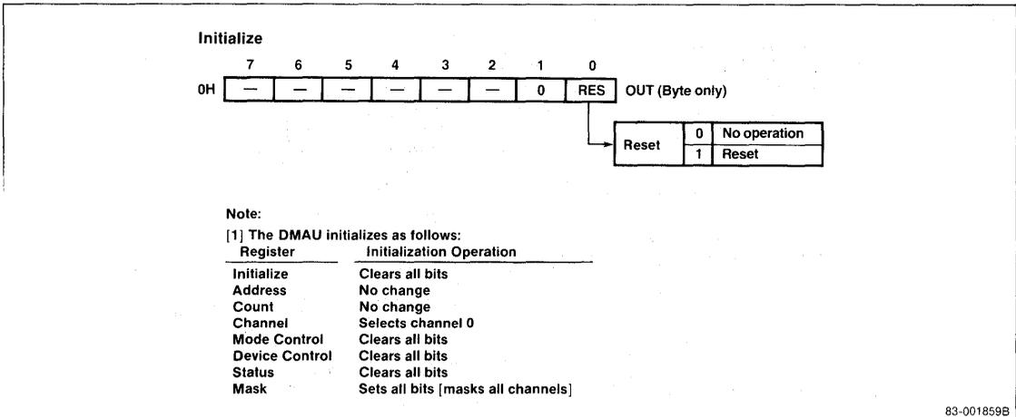
Figure 39. DMA Channel Register
