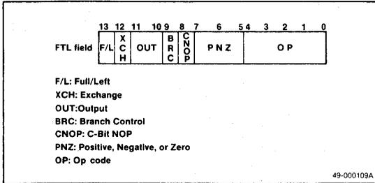
PU instructions (see table 20) are stored in the Function Table Left field of the Function Table memory. The bits 0 through 11 are used as control information for the Processing Unit. The bits 12 and 13 are deleted before the token arrives at the Processing Unit. Two operands from the A and B sides are operated on by the Processing Unit and the result is output to the X and Y sides (see figure 19).
