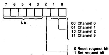
**Mask Register.** There is a mask bit for each channel which can disable an incoming DRQ. If the channel is not set for autoinitialize, each mask bit is set when its channel produces an  $\overline{EOP}$ . Each bit can be set or cleared under software control. Reset clears the register. This disallows DMA requests until they are permitted by a clear mask register instruction.
