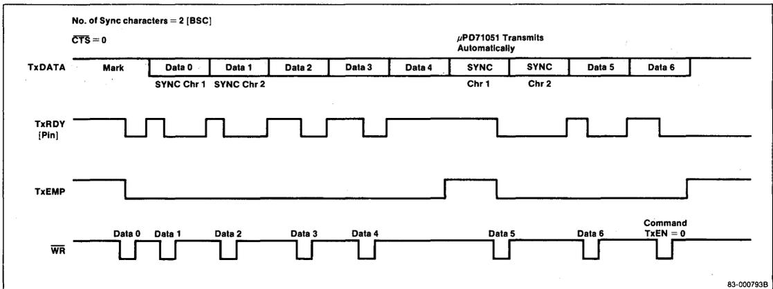
**Figure 17. Issuing a Command During SYNC Character Transmission**
