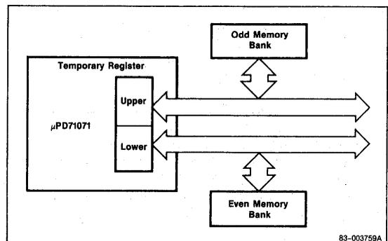
range of memory can be initialized with the same value since the contents of the source address never change. During memory-to-memory transfer, the DMAAK signal and channel 0's terminal count (TC) pulse are not output. (See figure 3.)
