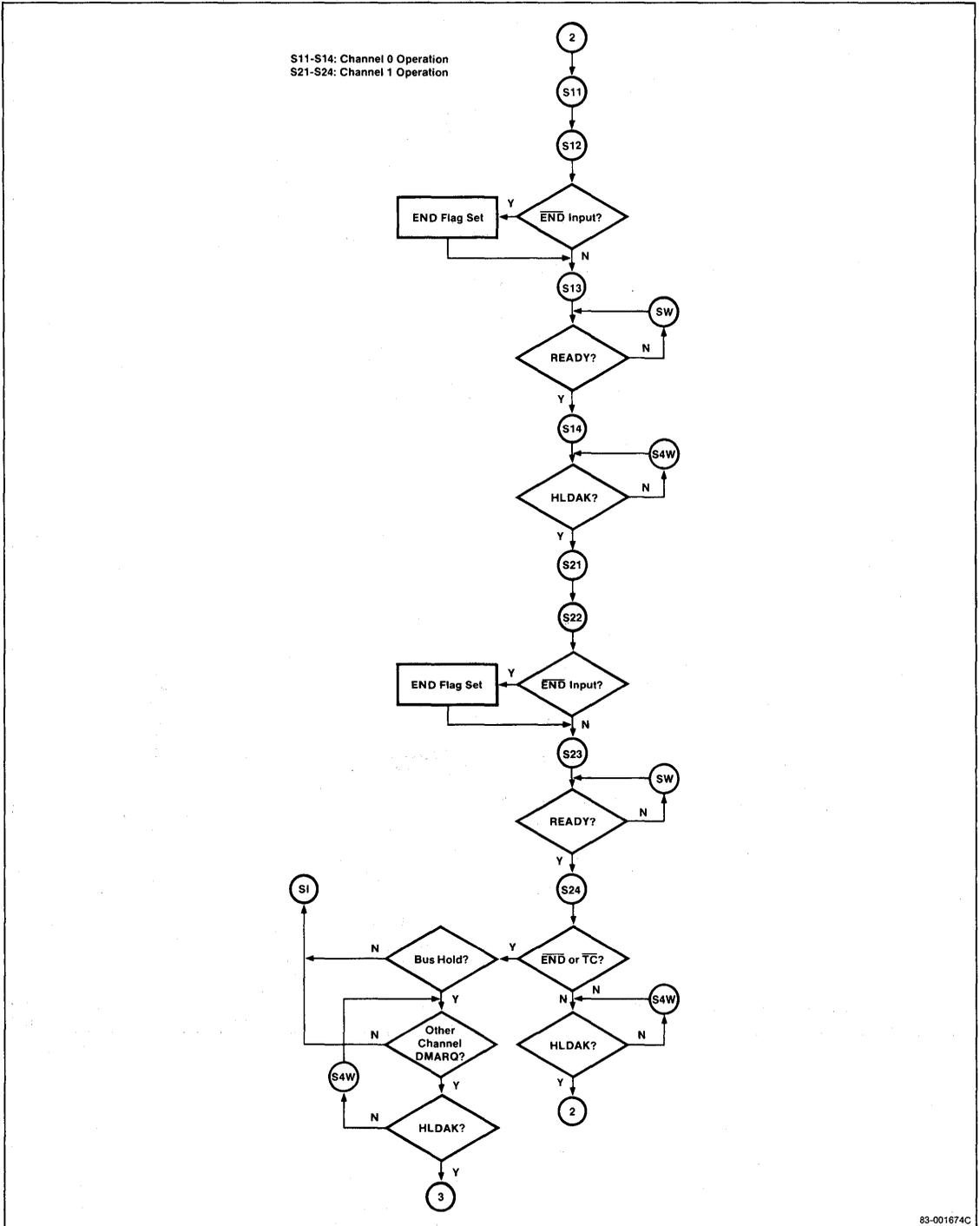
**Figure 28. Memory-I/O Transfer, Normal Timing**
