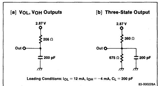
Loading Conditions:  $I_{OL} = 12\text{ mA}$ ,  $I_{OH} = -4\text{ mA}$ ,  $C_L = 200\text{ pF}$
