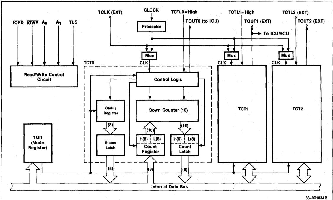
Because **RESET** leaves the TCU in an uninitialized state, each timer/counter must be initialized by specifying an operating mode and a count. Once programmed, a timer/counter will continue to operate in that mode until another mode is selected. When the count has been written to the counter and transferred to the down counter, a new count operation starts. Both the current count and the counter status can be read while count operations are in progress.
