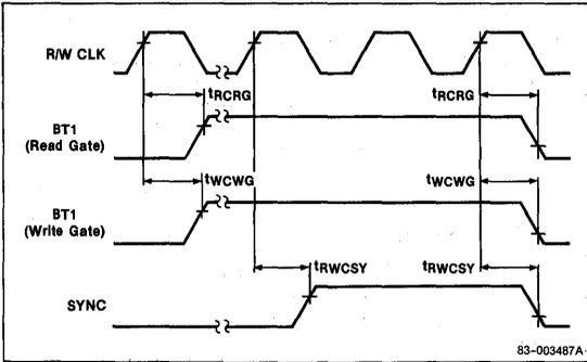
**Bit Bus Timing, Fault Clear/Return-to-Zero**
