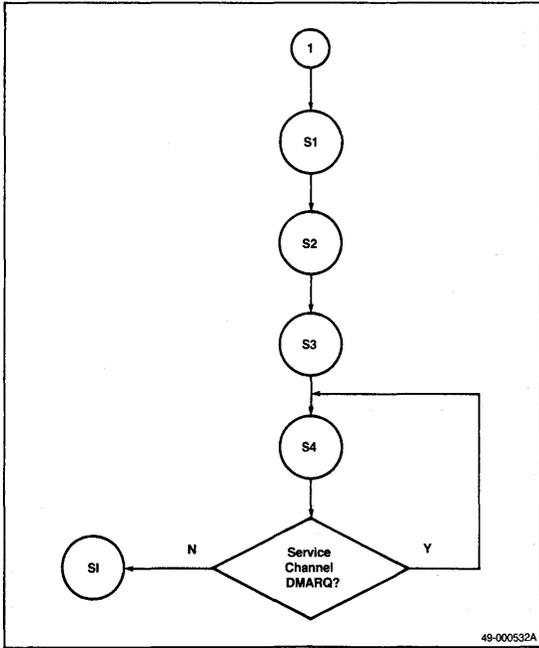
Figure 24. DMA Cycle, Single Mode
