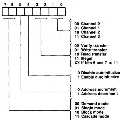
**Request Register.** This register allows the μPD8237A to respond to DMA requests from software as well as hardware. There is a bit pattern for each channel in the request register. These bits can be prioritized by the priority resolving circuitry and are not maskable. Each bit is set or reset under software control or cleared when TC or an external EOP is generated. A reset clears the entire register. The correct data word is loaded by software to set or reset a bit.
