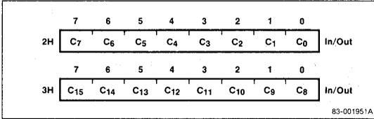
**Figure 15. Address Register Read/Write Format**
