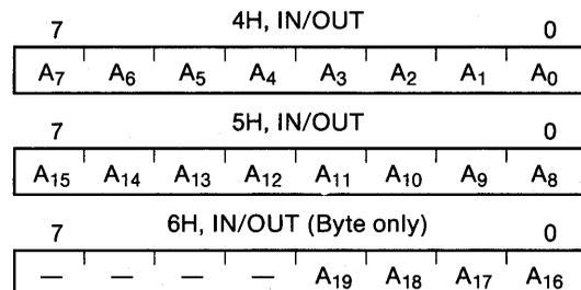
The DBA register holds the starting address value until a new address is specified. This value is transferred to the DCA register automatically if autoinitialization is selected. For each DMA transfer, the current address register is incremented/decremented by one.
