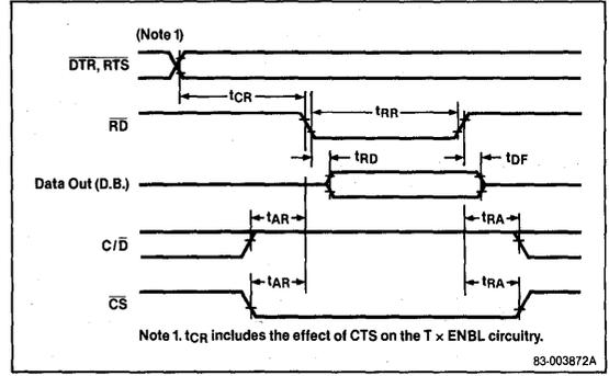
**Transmitter Control and Flag Timing (Async Mode)**
