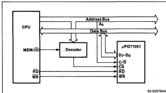
**Figure 3. μPD71051 Operating Procedure**
