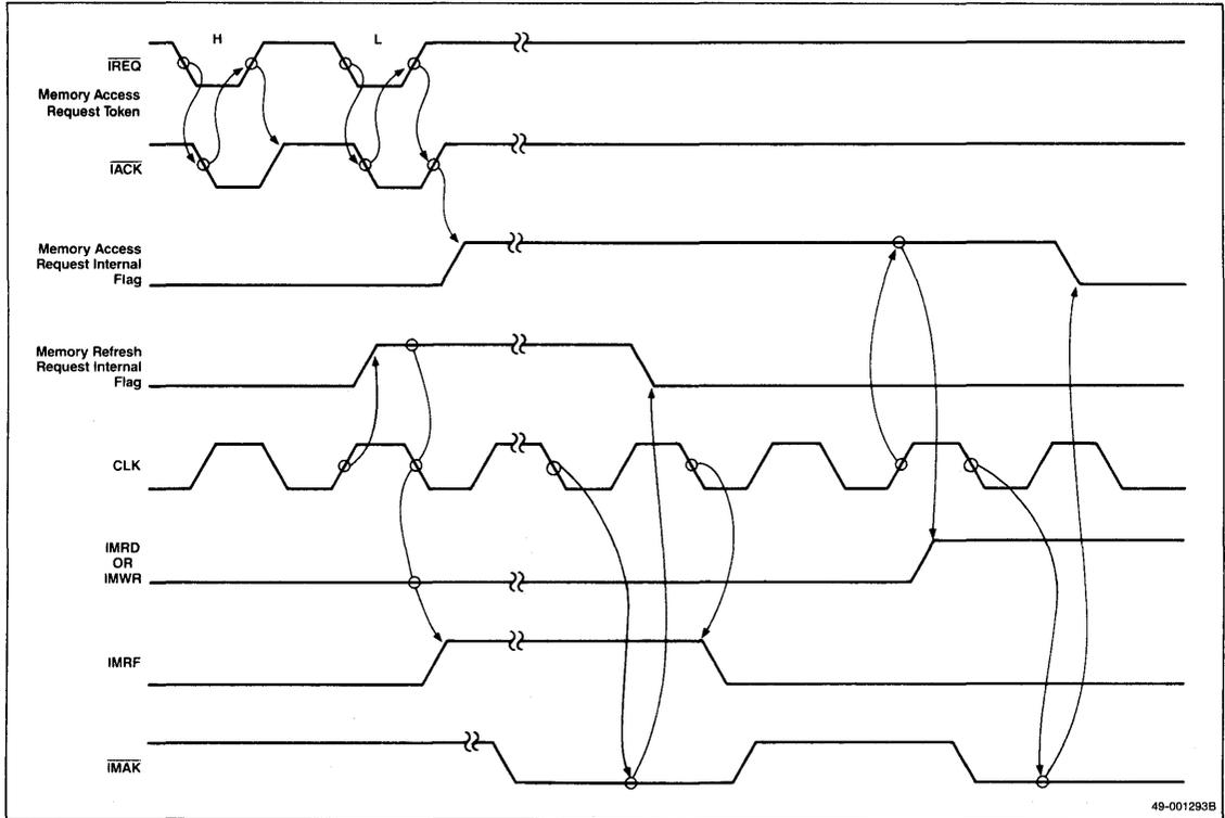
Figure 16. Read Data → μPD7281 Output Timing (Single Output)
