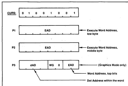
When the WG bit is set to one, any data following the WDAT command is written as is. When the WG bit is set to zero, the 7220A performs as the 7220 does: The pattern written is determined by the least significant bit of each parameter byte following the WDAT command. This bit is expanded into 16 identical bits which form the pattern.
