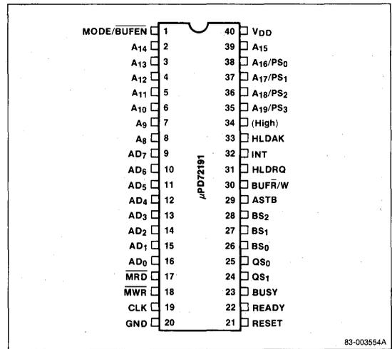
**Figure 2. Pin Configuration for V30 Mode (μPD70116 Microprocessor)**
