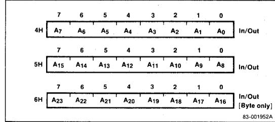
**Figure 16. Device Control Register Read/Write Format**
