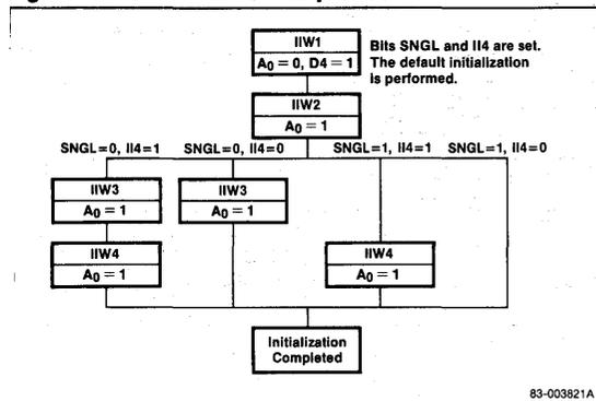
slave μPD71059 INT output is routed to one of the μPD70208 INTP inputs. During the second interrupt acknowledge bus cycle, the ICU places the slave address on address lines A<sub>10</sub>-A<sub>8</sub>. Each slave compares this address with the slave address programmed using interrupt initialization word 3 (IIW3). If the same, the slave will place the interrupt vector on pins AD<sub>7</sub>-AD<sub>0</sub> during the second interrupt acknowledge bus cycle.
