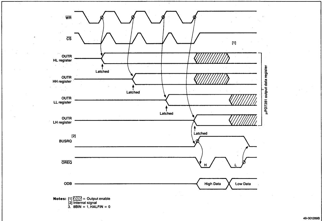
**Figure 10. Output Timing (μPD7281 to μPD9305 to Host)**
