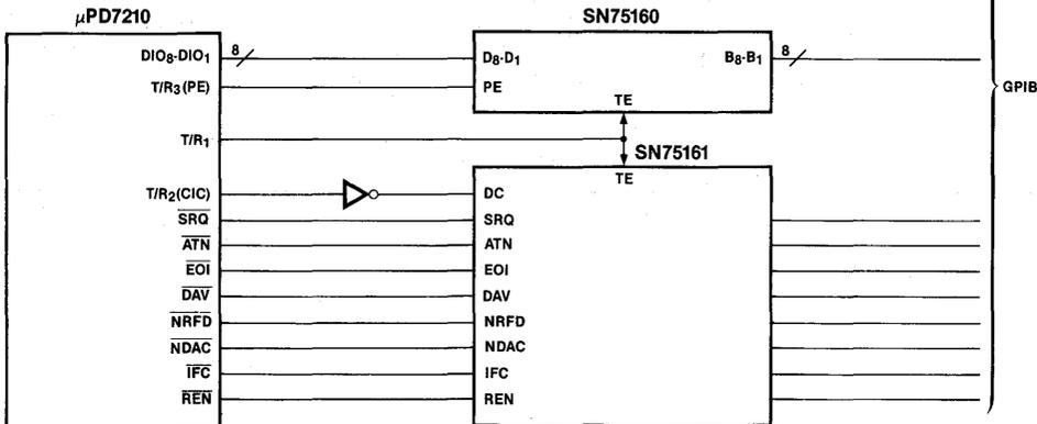
Note: In the case of low-speed data transfer (B<sub>2</sub> = 0), the T/R<sub>3</sub> pin can be used as a TRIG output. The PE input of SN75160 should be cleared to 0.
