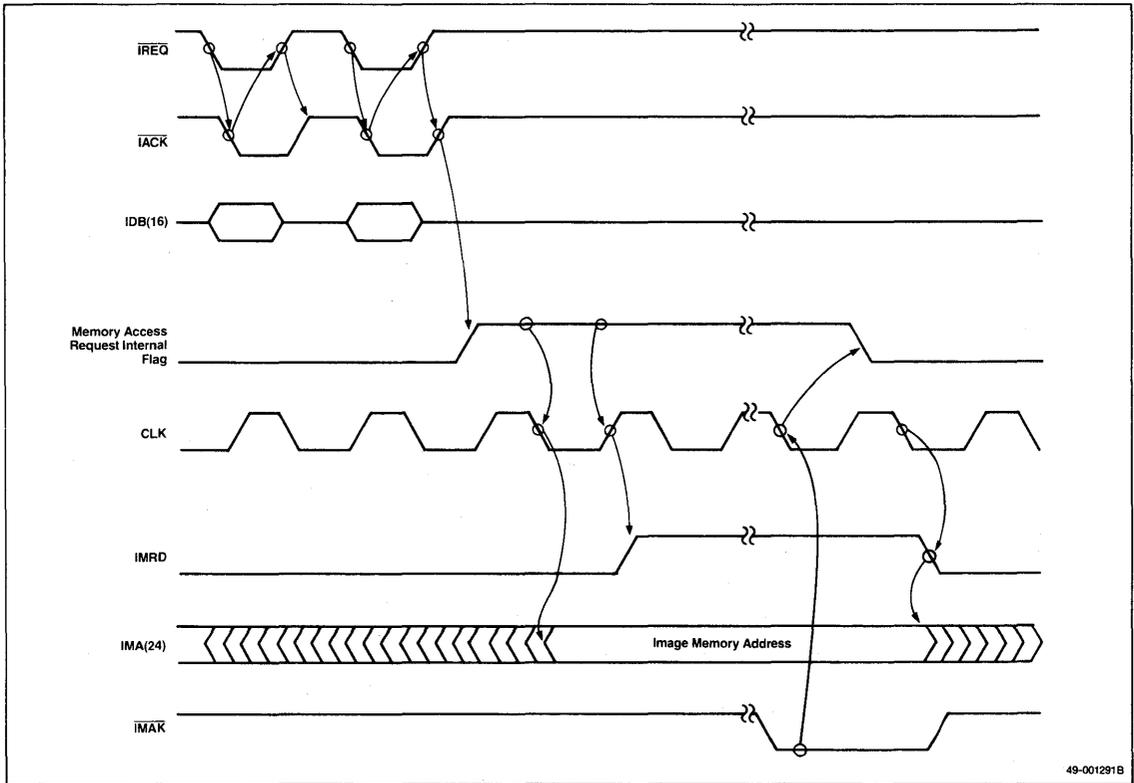
Figure 14. Image Memory Write Timing (Without Refresh Request)
