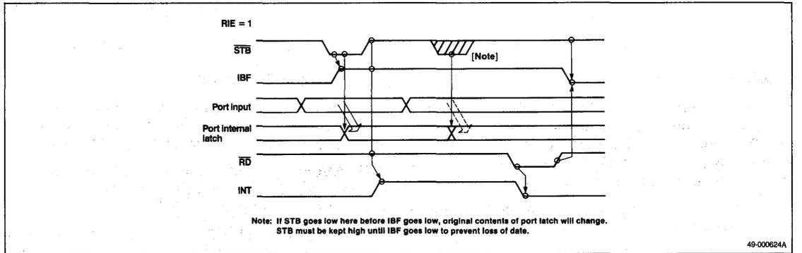
**RIE [Read Interrupt Enable Flag].** RIE controls the interrupt output. Interrupts can be enabled by using the bit manipulation command to set this bit to 1, and disabled by resetting it to 0. This signal is internal to the μPD71055 and is not an output. The state of RIE does not affect the function of  $\overline{STB0}$  or  $\overline{STB1}$ , which are inputs to the same bits (P2<sub>4</sub> and P2<sub>2</sub>) of port 2.
