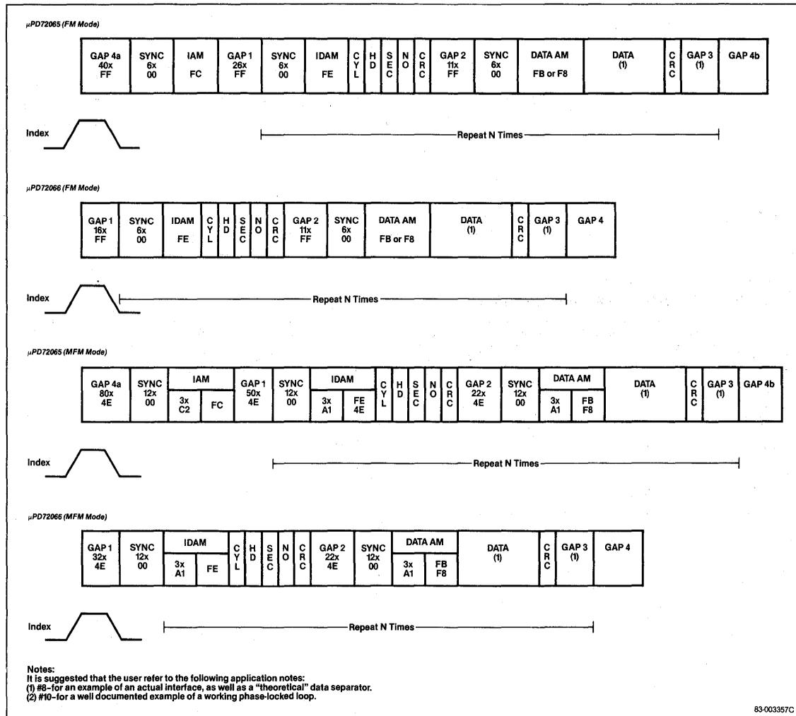
Figure 5. Data Format (Sheet 2 of 2)
