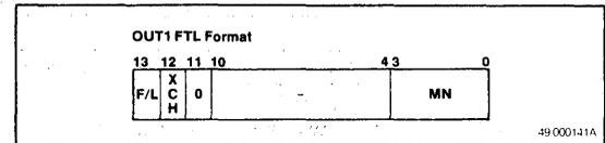
This instruction outputs a 32-bit data token via the Output Data Bus (ODB). Since the size of the ODB is 16 bits, a 32-bit output data token is divided into two 16-bit words and output one 16-bit word at a time. The format of an output data token is shown in figure 24.
