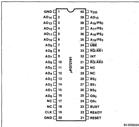
**Figure 4. Pin Configuration for V50 Mode (μPD70216 Microprocessor)**
