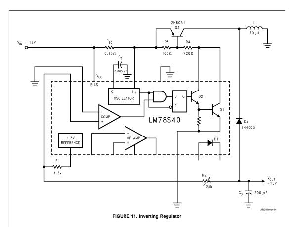
The sampling network, R1 and R2, can easily be calculated. Assuming the sampling network current  $\rm I_S$  is 1 mA:
