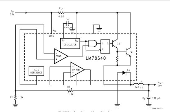
FIGURE 9. Step-Down Voltage Regulator
