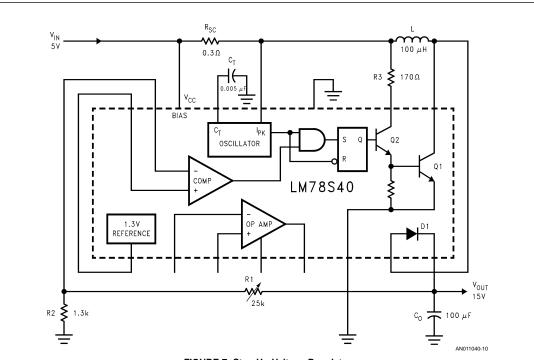
FIGURE 7. Step-Up Voltage Regulator
