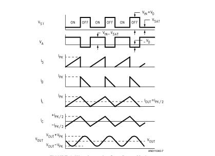
FIGURE 4. Waveforms for Step-Down Mode
