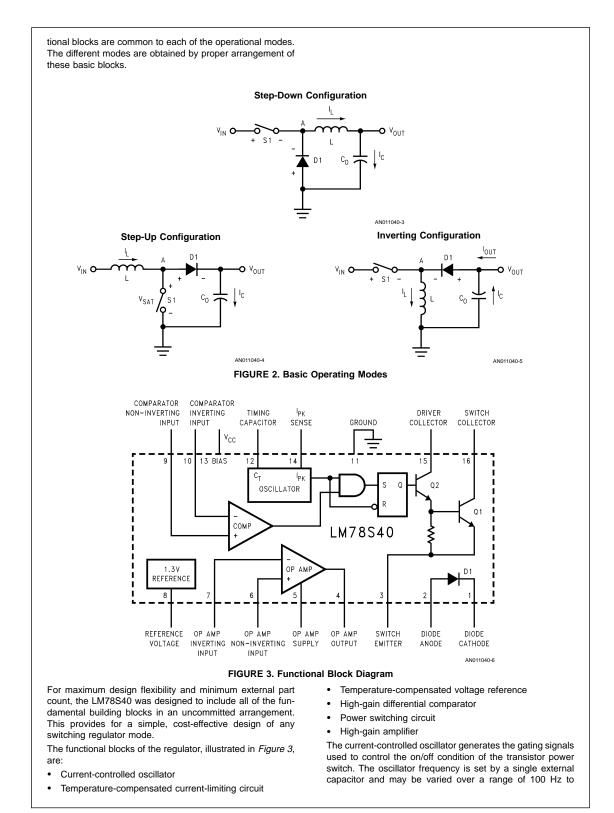
100 kHz. Most applications require an oscillator frequency from 20 kHz to 30 kHz. The oscillator duty cycle ( $t_{on}/t_{off}$ ) is internally fixed at 6:1, but may be modified by the current-limiting circuit.
