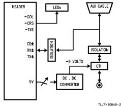
FIGURE 2. Connector Card Block Diagram
