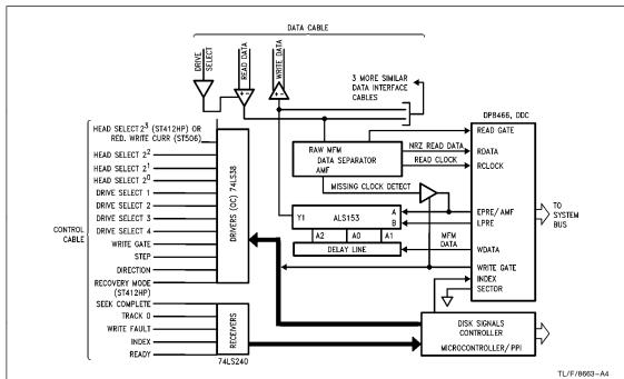
FIGURE 6.14. Disk Data and Control Paths (ST506/ST412HP)
