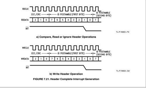
operations, the interrupt is generated when first byte of ID Postamble is being read by the DDC whereas in Write Header operation, interrupt is generated when first byte of ID Postamble is being written to the disk by the DDC.
