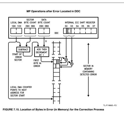
the DDC ignores any drive command loaded into the Drive Command Register. On initiation of the Correction Cycle, the Correction Cycle Active flag, (bit 6 of the Status register), will go high.
