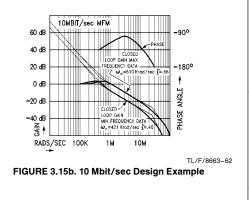
The impact of a 2,7 code on the data separator is significant. Loop bandwidth is dependent upon the sample rate into the phase detector. With MFM it has been seen that the bandwidth in minimum frequency data is  $1/\sqrt{2}$  times the bandwidth in maximum frequency data. This is a ratio of 1:0.707. In a 2,7 code the ratio is  $\sqrt{378}$  or 1:0.612. The damping factor follows the bandwidth so a 2,7 code system must be more carefully designed to avoid underdamped or overdamped response.
