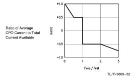
Ensures unlimited capture range. The digital phase detector ensures fre-quency acquisition by forcing the charge pump to always pump in the direction needed to make FVCO equal to FREF
