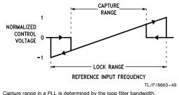
FIGURE 3.4. Capture and Lock Range
