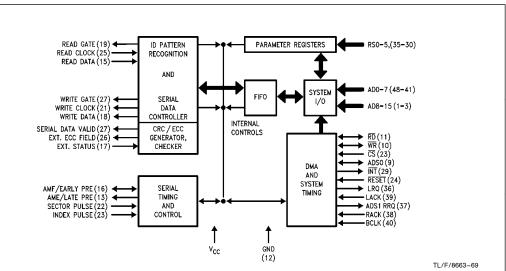
FIGURE 4.2(b). The DDC Block Diagram with Pin Assignment
