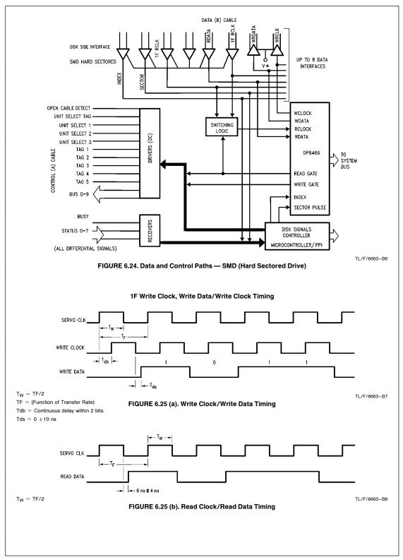
Preamble length: The synchronization time required to allow the PLL to synchronize is 11 bytes before the sync pattern of address and data fields.
