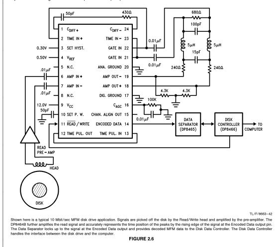
The output of the DP8464B drives a data separator (such as the DP8465) which extracts the digital data from the encoded data supplied by the DP8464B. The data separator utilizes a phase-locked loop that locks onto the leading edge of the encoded data signal from the DP8464B.
