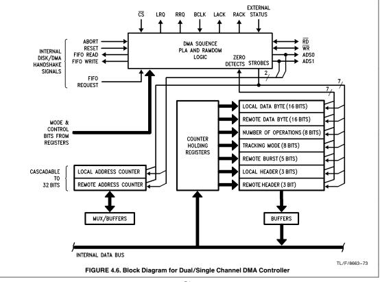
then transfer the data from the port to system memory. Refer to Figure 4.7(b). The local request and remote request are issued when the DDC requires a transfer, the microprocessor and bus arbiter respond by acknowledging the requests. If both channels are requesting, the system should arbitrate the acknowledge, however the local DMA has a higher priority if both requests are acknowledged.
