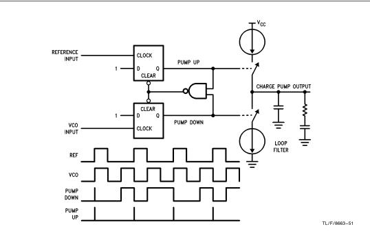
FIGURE 3.6. Digital Phase Detector
