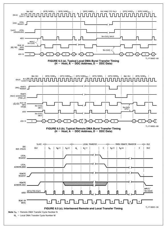
At 20 MHz bus clock (i.e. clock period of 50 ns and memory cycle of 200 ns) and assuming word-wide DMA transfers, the DDC will take  $16 \times 200$  ns =  $3.2 \ \mu$ s to empty the FIFO. This essentially shows that microprocessor bus is free for  $17 - 3.2 = 13.8 \ \mu$ s (81.2% of the time). In other words, the DDC will need bus control after every 17  $\mu$ s.
