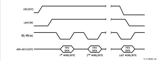
FIGURE 6.7 (b). DDC FIFO Read/Write by External DMA
