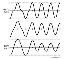
Typical MFM waveforms on oxide media with ferrite heads. Since there is only slight shouldering on the outer track, the traditional self gating (de-snaker) pulse detector can be used. FIGURE 2.1
