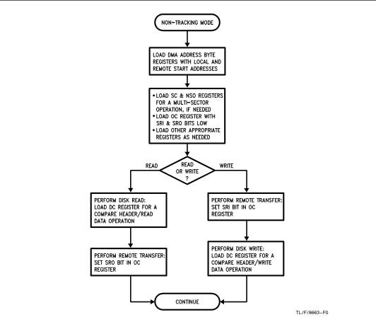
FIGURE 7.13. Dual DMA Non-tracking Mode µP Programming Flow Chart
