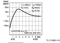
Controller must keep SET PLL LOCK deasserted for 8 bytes after READ GATE is asserted.
