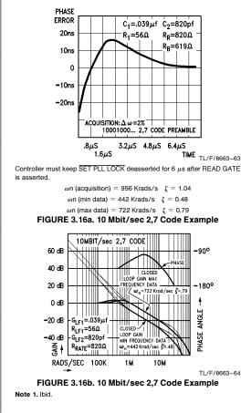
In conclusion, loop filter design for 2,7 codes is more difficult than for MFM. In hard sectored drives, or pseudo hard sectored drives with dc erased gaps, the problem is simply the wide range of damping factors and can be easily solved.
