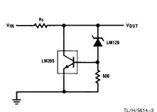
FIGURE 8. Power Shunt Regulator
