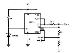
FIGURE 7. External Reference For IC
