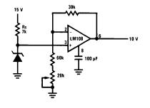
FIGURE 3. Bridge Compensation for Line Changes
