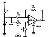
FIGURE 5. Bipolar Output Reference
