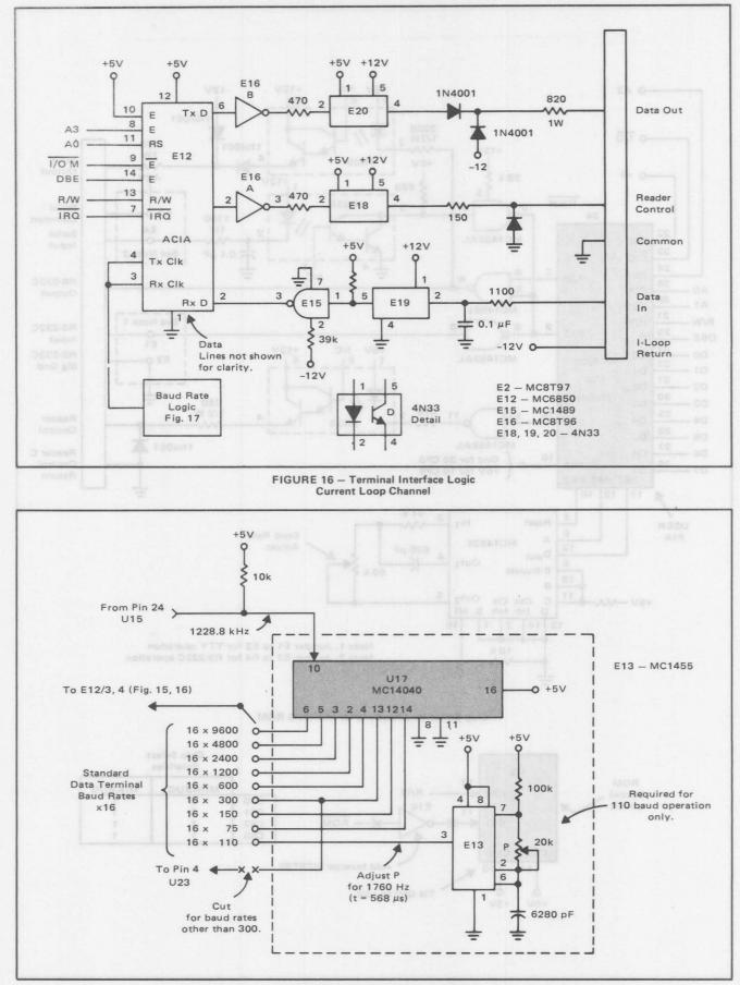
FIGURE 17 – Baud Rate Logic
