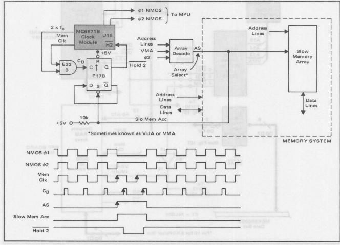
FIGURE 6 – Slow Memory Handshake Logic and Waveforms
