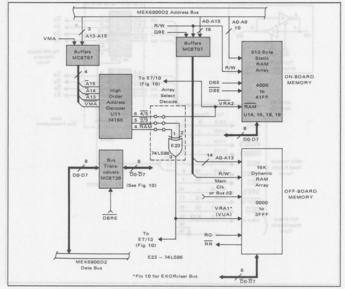
FIGURE 9 - Addressing for 16.5K Memory Configuration
