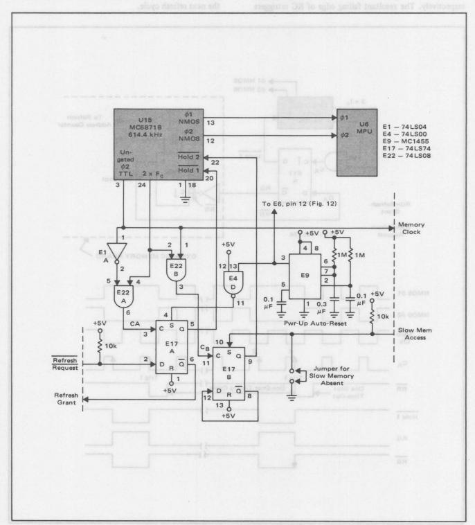
FIGURE 4 – Memory Control Handshake Logic
