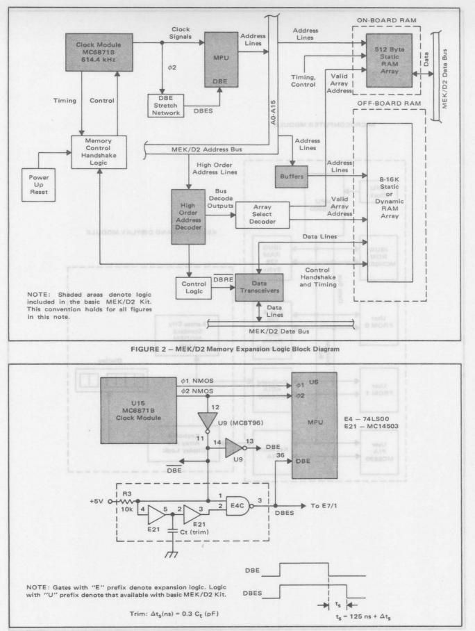
FIGURE 3 – DBE Stretch Network for Memories with Non-Zero Data Hold Time Requirement
