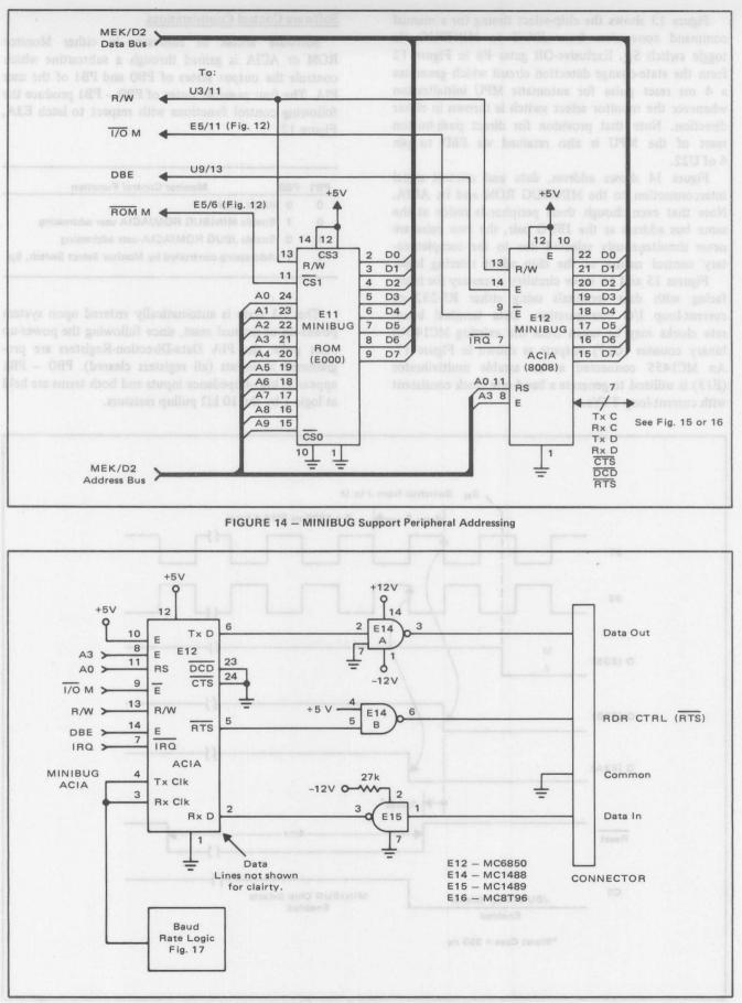
FIGURE 15 – Terminal Interface Logic RS-232 Channel
