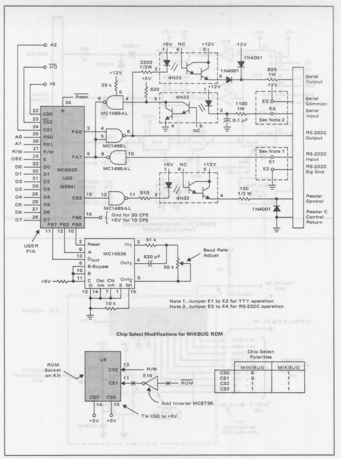
FIGURE 18 - Terminal Interface Logic for MIKBUG
