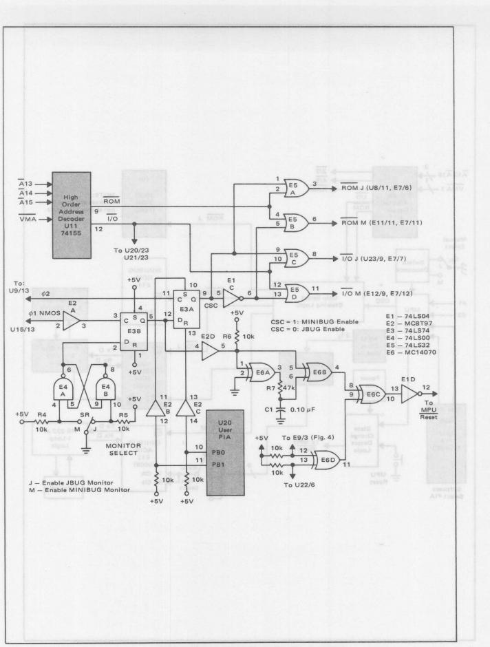
FIGURE 12 – Dual-Monitor Switching Logic
