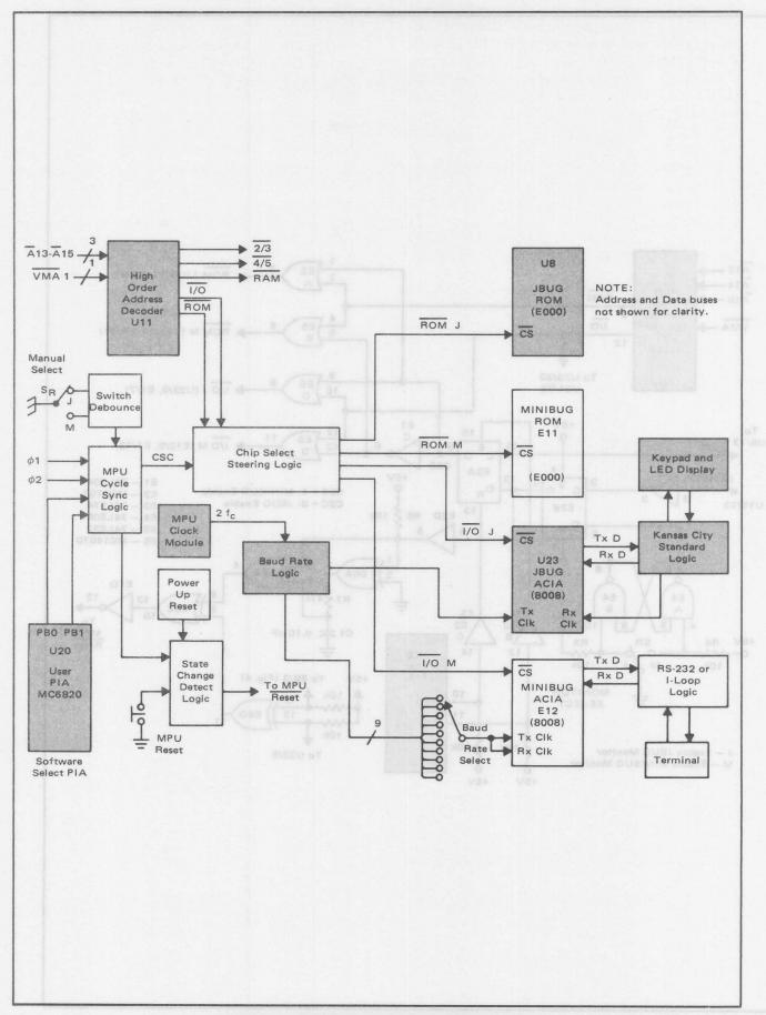
FIGURE 11 - Dual-Monitor Switching Logic Block Diagram
