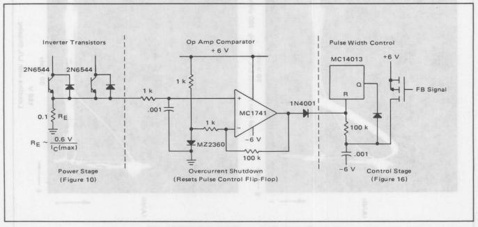
FIGURE 13 - Suggested Overcurrent Shutdown Circuit
