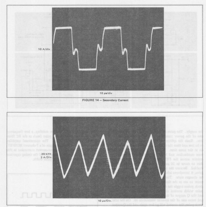
FIGURE 15 - Filter Inductor Current
