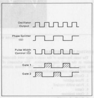
Figure 17 — Timing Diagram
