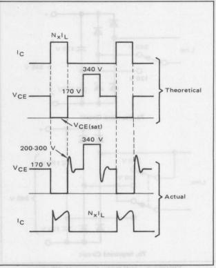
FIGURE 6 - Waveforms of Inverter Transistors
