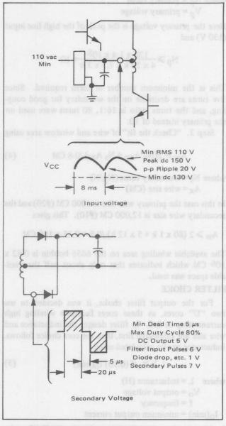
FIGURE 9 – Transformer Waveforms at Low Line
