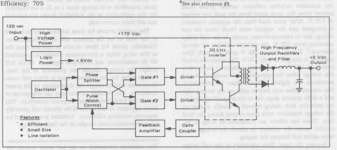
FIGURE 8 - Block Diagram 5-V, 50-A Line Operated Switched Mode Power Supply
