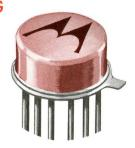
The addition of a welded cap, providing a hermetic seal for each Motorola integrated circuit, completes the fabrication process. Each unit then undergoes a 3-foot drop test on a maple block, stabilization baking, and 20,000 g centrifuge testing in accordance with military specifications to assure ruggedness and reliability.
