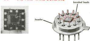
After separation into individual circuits, each chip is mounted on a ceramic wafer, then to a header by means of a very high temperature eutectic solder. Short wires, .001" in diameter, are bonded from the circuit to the proper header leads. This rugged mounting method and the advanced wire bonding techniques used make it possible for Motorola circuits to withstand severe centrifuge, shock and vibration conditions.
