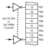
CMOS or TTL Driving Port B Directly.
