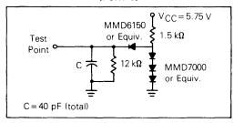
FIGURE 2 — CMOS EQUIVALENT TEST LOAD (PORT A)
