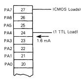
Port A, Bit 7 Programmed as Output, Driving CMOS Loads and Bit 4 Driving one TTL Load Directly (using CMOS output option).
