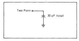
FIGURE 3 — TTL EQUIVALENT TEST LOAD (PORTS A AND C)
