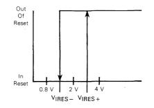
Figure 7-1. Typical Reset Schmitt Trigger Hysteresis
