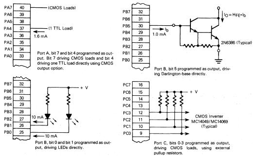
Figure 8-2a. Typical Port Connections—Output Modes
