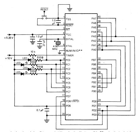
\* This connection depends on clock oscillator user selectable mask option. Use jumper if the RC mask option is selected.
