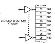
CMOS or TTL driving port B directly.
