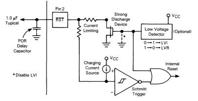
Figure 7-3. RESET Configuration
