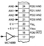
Port D used as 4-channel A/D input with bit 7 used as CMOS digital input. MC6805R2, MC6805R3, MC6805R3, and MC68705R5 only.
