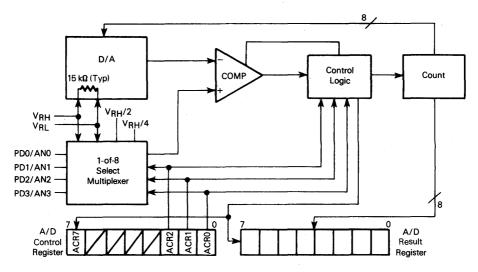
Figure 8-3. A/D Block Diagram
