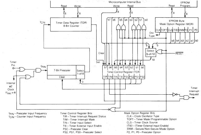
NOTES: The TOPT bit in the mask option register selects whether the timer is software programmable via the timer control register or emulates the mask programmable parts via the MOR PROM byte.
