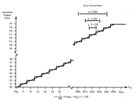
Figure 8-5. Ideal Converter Transfer Characteristic
