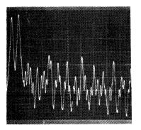
Figure 7 - SPECTRAL ANALYSIS OF WAVEFORM IN FIG. 6 (Vert-10 dB/Div, Horizontal-1 KHz/Div)
