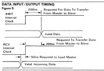
this event, the set-up and hold times for the first clock pulse should be measured from the positive edge of RCV. SYNC.
