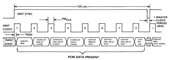
NOTE: All rise and fall times are measured from 0.4V and 2.4V. All delay times are measured from 1.4V.
