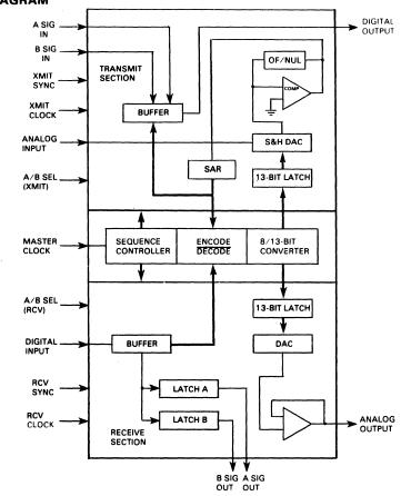
components helps reduce system operating power which was the overriding consideration in chip design. Using the CMOS process, the digital portions dissipate power only during transitions. The linear sections consume power continuously.
