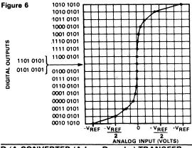
D/A CONVERTER (A-Law Decoder) TRANSFER CHARACTERISTIC
