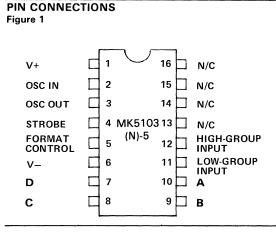
over a longer period. When a minimum of 30 milliseconds of a valid DTMF digit is detected, the proper data is latched into the outputs and the output strobe goes high. When a valid digit is no longer detected, the strobe will return low and the data will remain latched into the outputs. Minimum interdigit time is 35 milliseconds.
