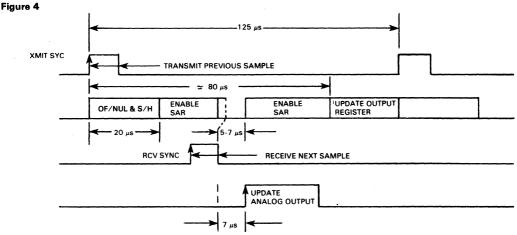
process is completed, the output of the SAR is loaded into the output buffer. The data is transmitted serially at the output clock rate during the period the XMIT SYNC is high. During the signalling frame, signalling information (SigA/SigB) is inserted into the output bit stream in place of the 8th data bit as selected by the A/B select (SMIT) input.
