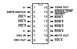
The MK5387 was designed specifically for integratedtone-dialer applications that require the following: wide-supply operation with regulated output, scanned keyboard inputs which recognize either negative-true or Class A closures, and auxiliary switching functions. Keyboard entries to the MK5387 integrated tone-dialer cause the selection of the proper divide ratio to obtain the required two audio frequencies from the 3.579545 MHz reference oscillator.
