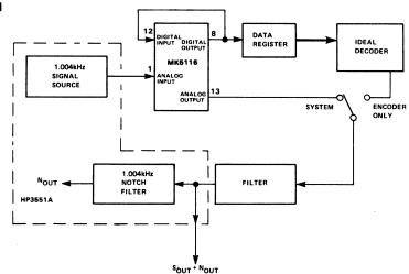
NOTE: The ideal decoder consists of a digital decompander and a 13-bit precision DAC.
