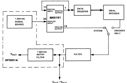
S<sub>OUT</sub> + N<sub>OUT</sub> NOTE: The ideal decoder consists of a digital decompander and a 13-bit precision DAC.
