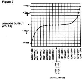
transfer characteristic of the D/A converter (A-law Decoder) is shown in Figure 7.
