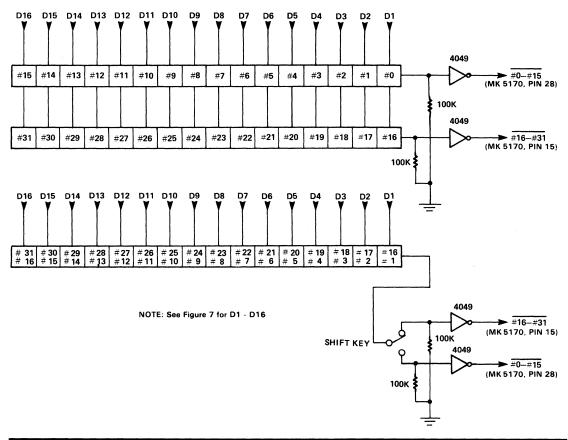
Four types of functions are used to control the dialer: (1) ENTER/DIAL allows entry and dialing of telephone numbers, (2) STORE enables storage of entered numbers, (3) CLEAR clears erroneous entries or begins a data entry sequence and (4) PAUSE provides for intergroup pauses while dialing. Note that one of three lengths of pause may be selected:
