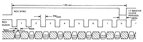
NOTE: All rise and fall times are measured from 0.4V and 2.4V. All delay times are measured from 1.4V.
