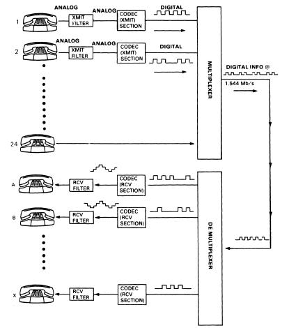
For T1 carrier systems, the digital PCM information might be transmitted between central offices. For PBX applications, the PCM technique is used to allow the switching to be done digitally. The accuracy of the subsequent D-A conversion preserves the voice quality so that insertion loss is not a problem.
