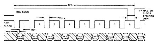
NOTE: All rise and fall times are measured from 0.4V and 2.4V. All delay times are measured from 1.4V.
