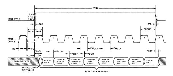
NOTE: All rise and fall times are measured from 0.4V and 2.4V All delay times are measured from 1.4V.
