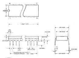
NOTES: 1. The true-position pin spacing is 0,100 between centerlines. Each pin centerline is located within ± 0.010 of its true longitudinal position relative to pins 1 and 40,
