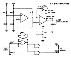
\* CE1 & CE2 must be inverted to enable memory. NOTE: ALL ACTIVE DEVICES POWERED FROM +5M
