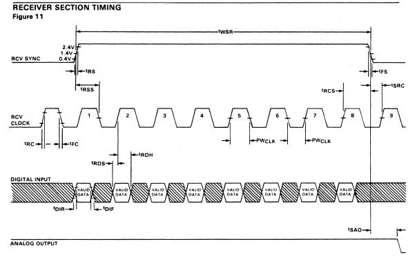
NOTE: All rise and fall times are measured from 0.4V and 2.4V. All delay times are measured from 1.4V.
