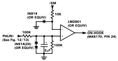
NOTE: Comparator is powered from +5M
