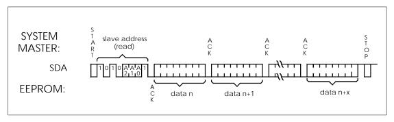
Figure 10: EEPROM Sequential Read Operation
