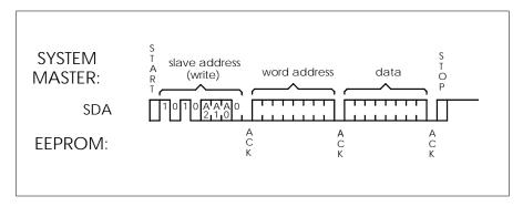
Figure 6: EEPROM Byte Write Operation
