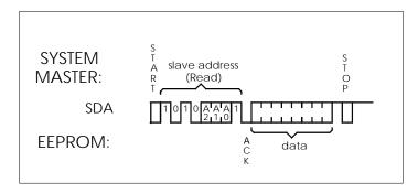
Figure 8: EEPROM Current Address Read Operation
