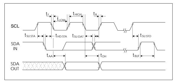
Figure 2: EEPROM Component A.C. Timing Parameters
