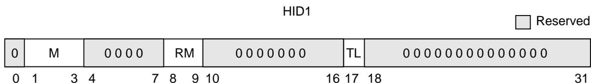
**Figure 2-26. PowerPC 601 Microprocessor Debug Modes Register**
