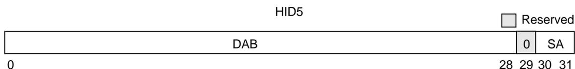
**Figure 2-28. Data Address Breakpoint Register (DABR)**
