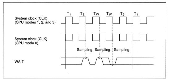
Figure 8-4 Wait State Insertion Timing Using the WAIT Line
