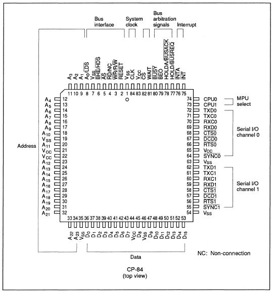
Figure 2-1 Pin Arrangement
