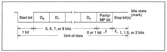
Figure 5-9 Character Format for Asynchronous Mode
