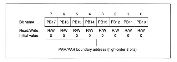
This register can specify only the high-order eight bits  $(A_{23}-A_{16})$  of the boundary address; the remaining low-order 16 bits  $(A_{15}-A_0)$  are fixed to 0000H. Thus, each area is specified in 64-kbyte units.
