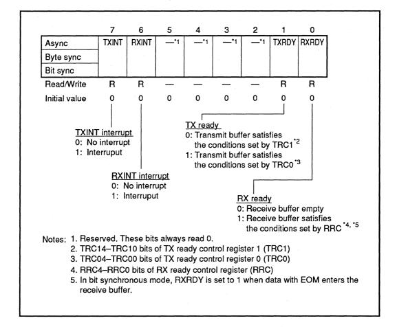
**Bit 7 (TXINT: TXINT Interrupt):** Indicates whether or not the TXINT interrupt has occurred. A TXINT interrupt request is issued to the MPU when this bit and the TXINTE bit of interrupt enable register 0 (IE0) are both 1.
