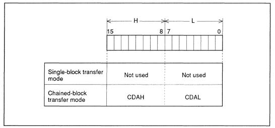
Figure 6-3 Current Descriptor Address Register
