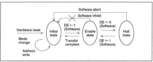
Figure 6-7 Software Abort and DMAC Operation
