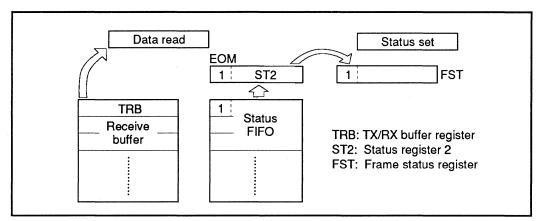
Figure 5-5 Frame Status Register (FST)
