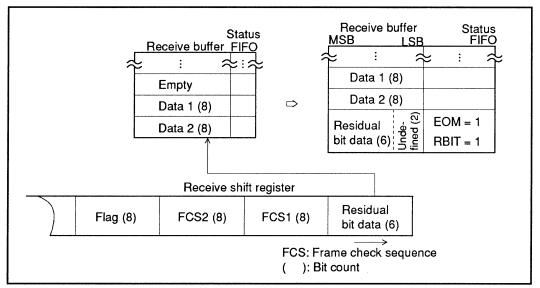
Figure 5-3 Residual Bit Frame Reception Operation (CRCCC = 1)
