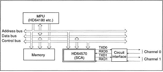
Figure 9-7 System Configuration Incorporating the SCA
