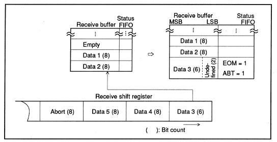
**Figure 5-4** Abort End Frame Reception Operation (CRCCC = 1)
