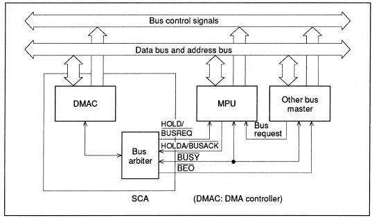
Figure 3-4 Bus Arbiter and Bus Masters
