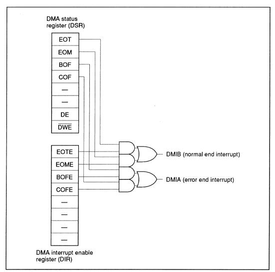
Figure 1-26 Logic Flow for Interrupt Requests, Status, and Enable Bits in DMAC Module
