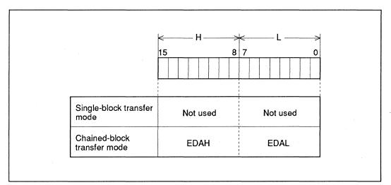
Figure 6-4 Error Descriptor Address Register
