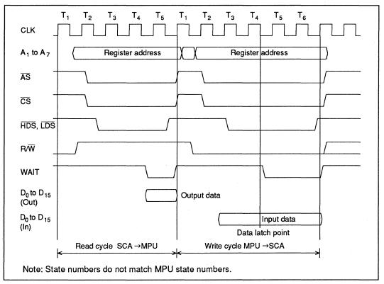
Figure 3-10 Slave Mode Bus Timing Sequence in CPU Mode 2
