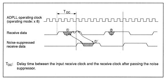
Figure 5-42 Noise Suppression in the Receive Clock Noise Suppressor
