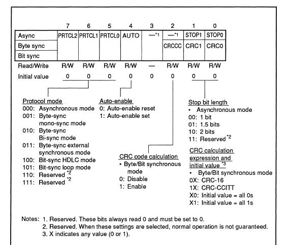
**Bits 7–5 (PRTCL2-PRTCL0: Protocol Mode):** Specify the transmission protocol (transmission control procedure). These bits must be initialized with a channel reset command before the bit setting is changed. Otherwise, normal operation is not guaranteed.
