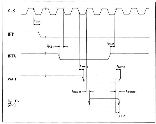
Figure 10-11 CPU Mode 1, 2, 3 Interrupt Timing
