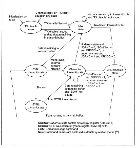
Figure 5-23 State Transition Diagram for Transmission in Byte Synchronous Mode
