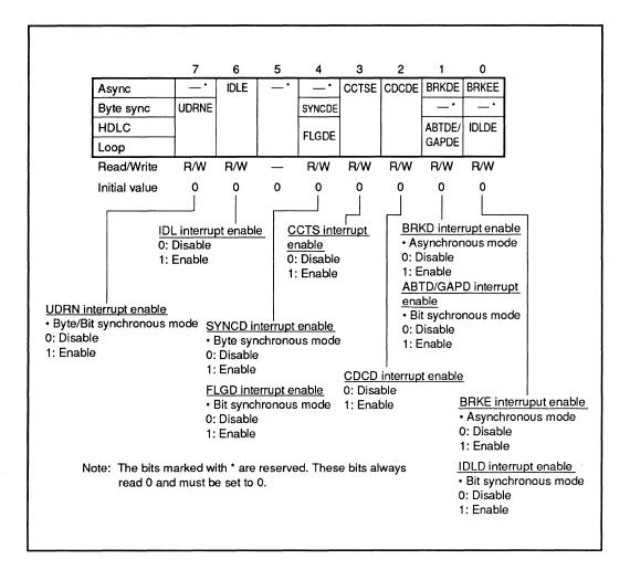
Bit 7 (UDRNE: UDRN Interrupt Enable): The function of this bit is described below.
