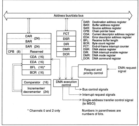
Figure 1-3 DMAC Block Diagram (one channel)
