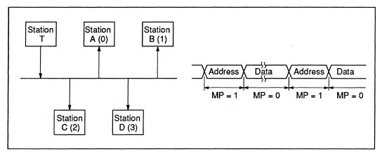
Figure 5-21 MP Bit Operation Example
