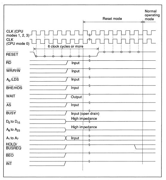
Figure 3-2 Reset Mode Timing
