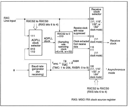
Figure 1-10 Receive Clock Source
