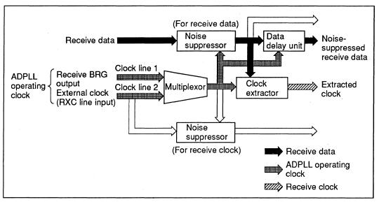
Figure 5-37 Data and Clock Signal Flow for Clock Extraction from Receive Data
