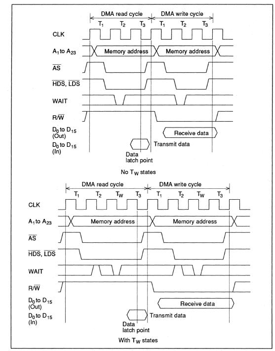
Figure 3-16 Master Mode Bus Timing Sequence in CPU Modes 2 and 3
