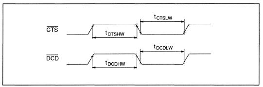
Figure 10-21  $\overline{\text{CTS}}$  and  $\overline{\text{DCD}}$  Timing
