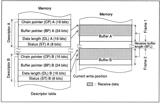
Figure 6-9 Descriptors and Buffers in MSCI-to-Memory Chained-Block Transfer Mode
