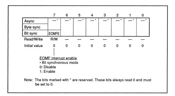
Bit 7 (EOMFE; EOMF Interrupt Enable): The function of this bit is described below.
