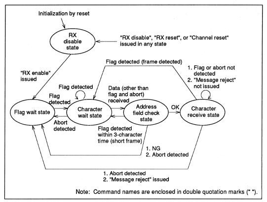
Figure 5-27 State Transition Diagram for Reception in Bit Synchronous Mode
