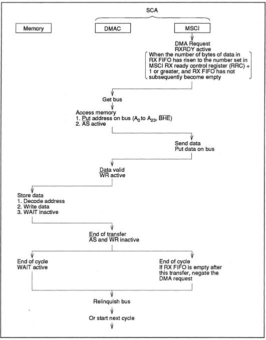
Figure 1-16 Receive DMA Operation (CPU mode 0)
