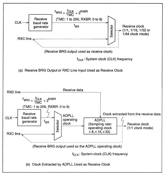
Figure 5-35 Receive Clock Sources
