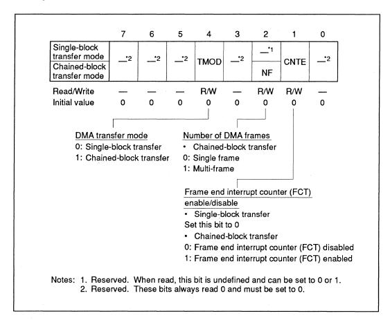
This register must be set in DMA initial state.
