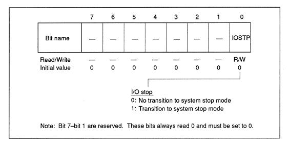
The low-power register controls transition to system stop mode.
