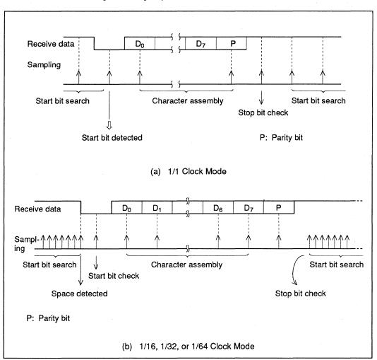
The timing of sampling receive data is shown in figures 5-15 (a) and (b). This example uses an 8-bit character and one stop bit, with parity.
