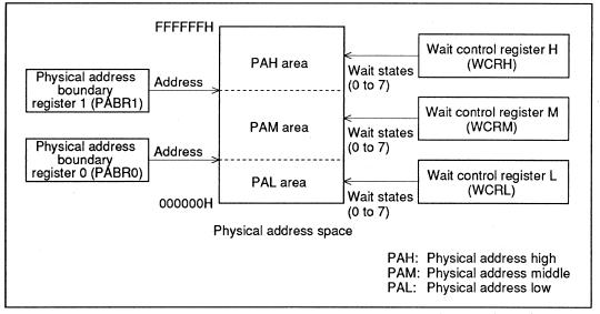
Figure 1-28 Subdivision of Address Space by Wait Controller and Insertion of Wait States
