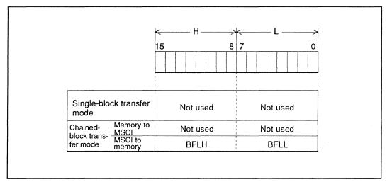
Figure 6-5 Receive Buffer Length Register
