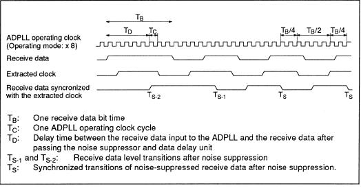
Figure 5-39 FM0 Receive Data Phase Compensation in Operating Mode ×8
