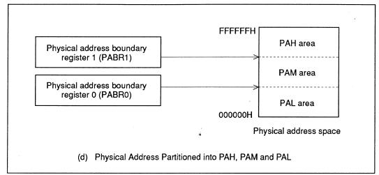
Figure 8-2 Boundary Address Setting Examples (cont)
