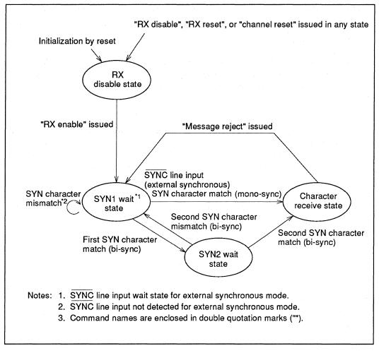
Figure 5-24 State Transition Diagram for Byte Synchronous Mode Reception
