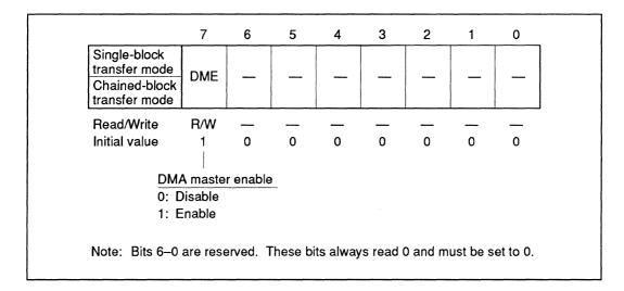
**Bit 7 (DME: DMA Master Enable):** Enables or disables channels 0, 1, 2, or 3 in either singleblock transfer mode or chained-block transfer mode as follows.
