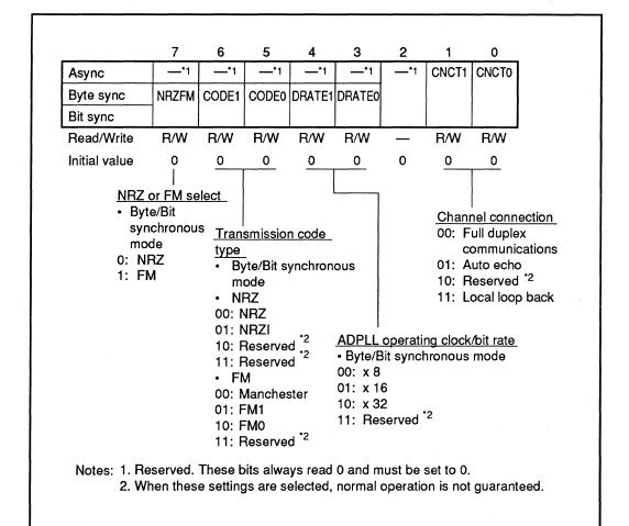
Bit 7 (NRZFM: NRZ/FM Select): Used in conjunction with the CODE1–CODE0 bits (below) to specify the transmission code type (NRZ or FM). This bit specifies MSCI decoding and encoding types. Only the NRZ type is available in asynchronous mode.
