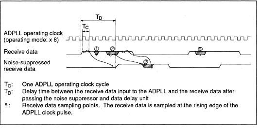
Figure 5-40 Noise Suppression in the Receive Data Noise Suppressor in Operating Mode ×8
