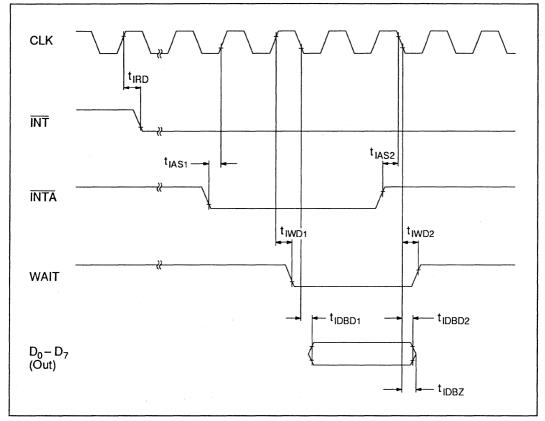
Figure 10-10 CPU Mode 0 Interrupt Timing
