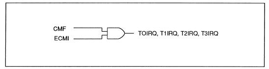
Figure 1-27 Logic Flow for Interrupt Requests, Status, and Enable Bits in Timer Module
