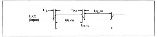
Figure 10-18 ADPLL Operating Clock Timing
