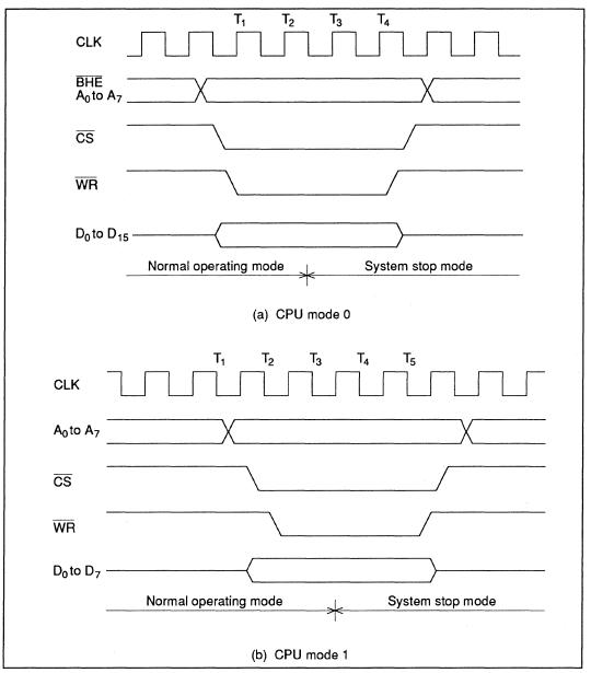
Figure 3-3 Timing of Transition to System Stop Mode
