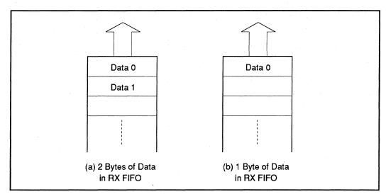
Figure 5-7 Data Arrangement in Receive Buffer
