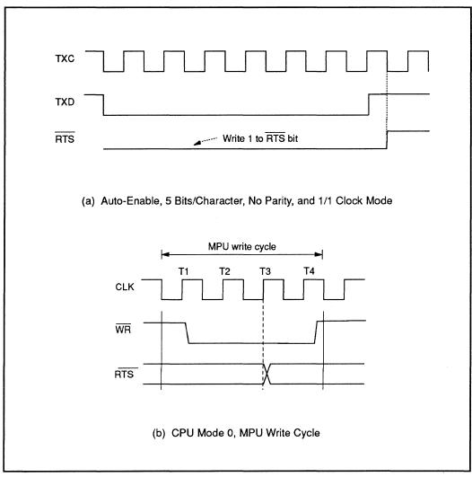
Figure 5-1 Modem Control Signal Timing
