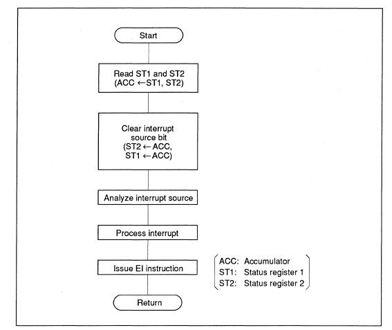
Figure 9-4 RXINT Interrupt Processing Routine (using HD64180)
