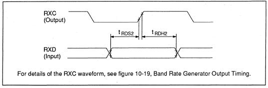
Figure 10-17 Receive Timing (RXC output)
