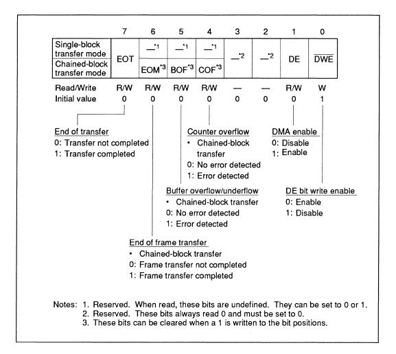
**Bit 7 (EOT: End of Transfer):** A 1 indicates that the transfer operation by the DMAC has been completed normally, in either single-block transfer or chained-block transfer mode. See section 6.4.1, Overview, for the conditions governing DMA normal completion.
