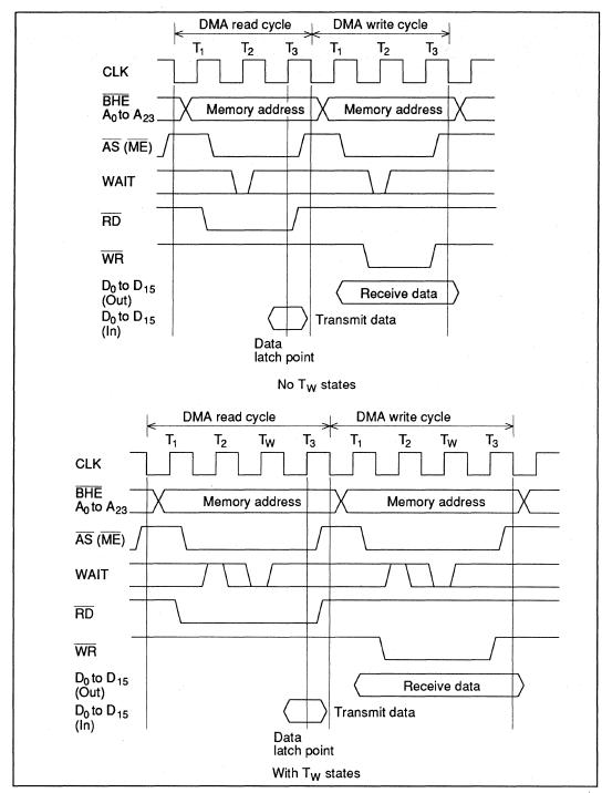
Figure 3-14 Master Mode Bus Timing Sequence in CPU Mode 0
