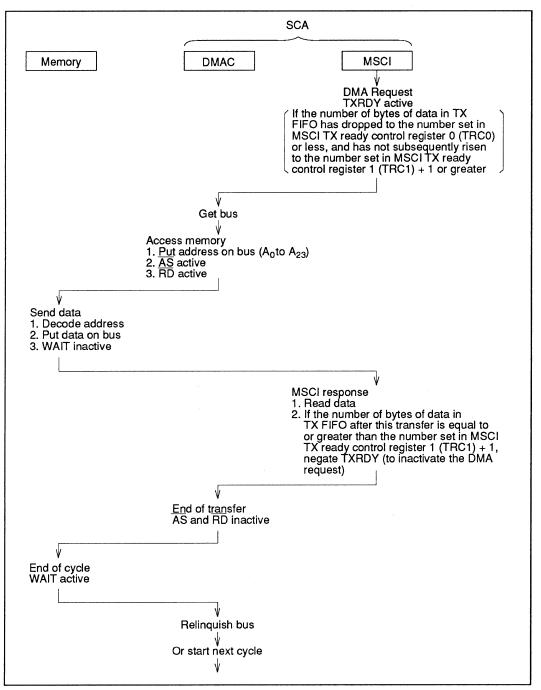
Figure 1-17 Transmit DMA Operation (CPU mode 1)
