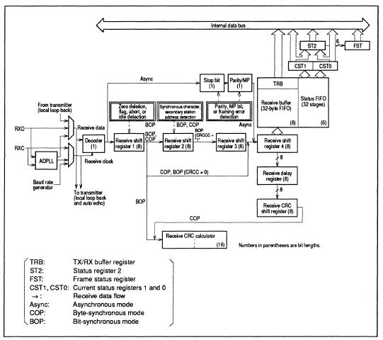
Figure 1-13 Block Diagram of the MSCI Receiver
