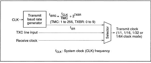
Figure 5-34 Transmit Clock Sources
