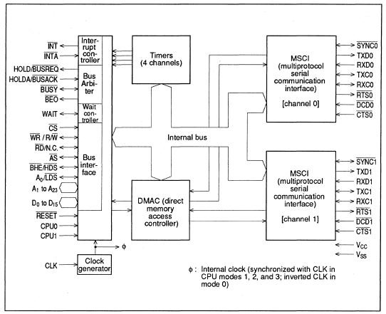
Figure 1-1 Block Diagram of SCA
