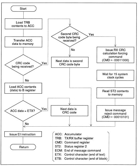
Figure 9-3 RXRDY Interrupt Processing Routine (using HD64180)
