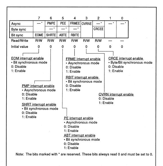
Bit 7 (EOME: EOM Interrupt Enable): The function of this bit is described below.
