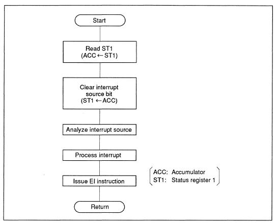
Figure 9-2 TXINT Interrupt Processing Routine (using HD64180)
