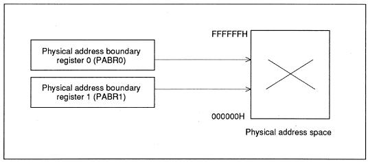
Figure 8-3 Incorrect Boundary Address Setting Example
