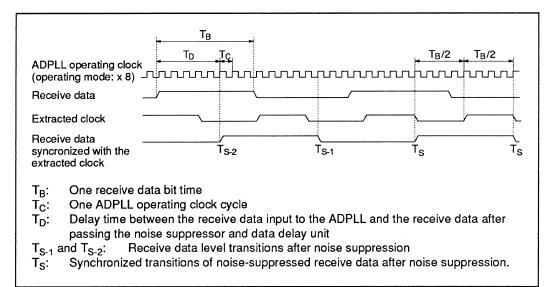
Figure 5-38 NRZ Receive Data Phase Compensation in Operating Mode ×8
