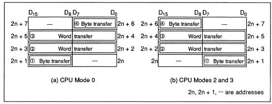
Figure 3-13 Data Transfer from Odd Address (example)
