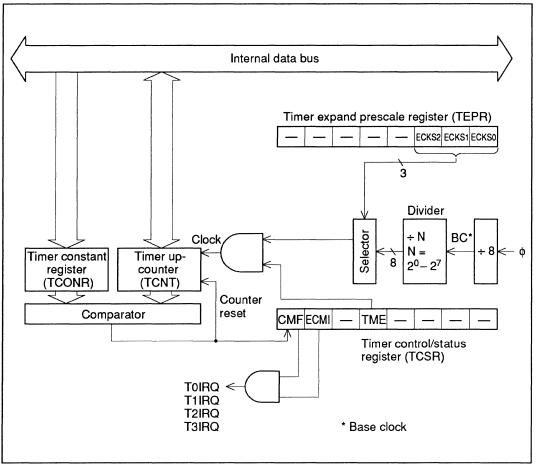
Figure 1-4 Timer Block Diagram
