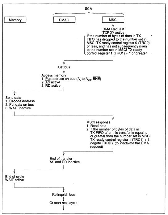
Figure 1-15 Transmit DMA Operation (CPU mode 0)
