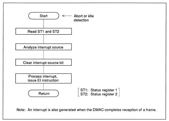
Figure 9-6 RXINT Interrupt Processing Routine (using HD64180)
