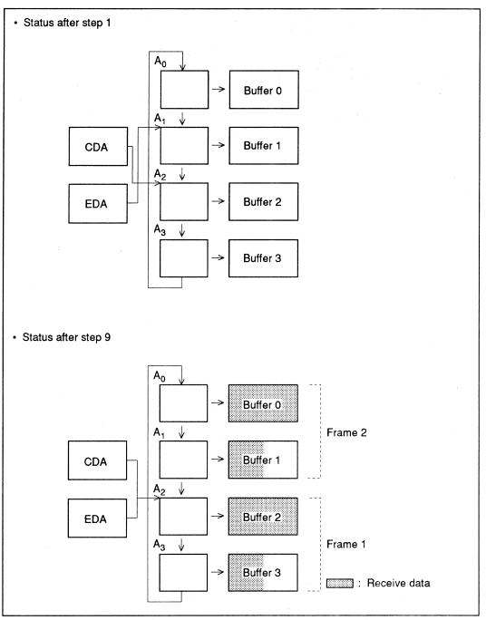
Figure 6-20 MSCI-to-Memory Chained-Block Multi-Frame Transfer (normal reception operation)
