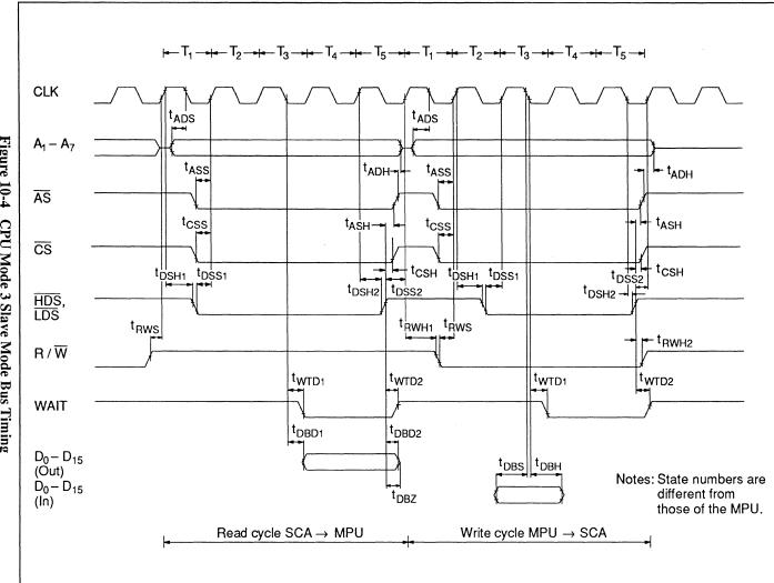
Figure 10-4 **CPU Mode 3 Slave Mode Bus Timing**
