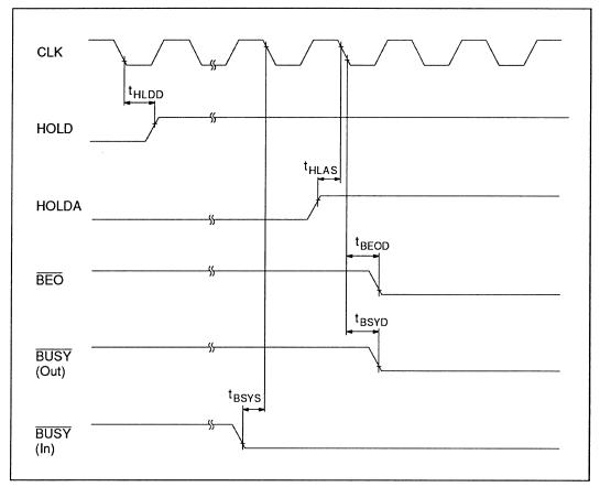
Figure 10-12 CPU Mode 0 Bus Arbitration Timing
