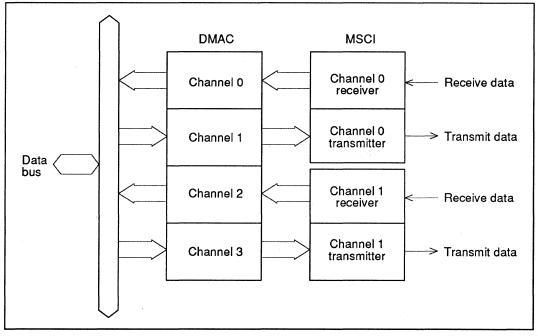
Figure 1-14 Interconnections between DMA Channels and MSCI Channels (concept)
