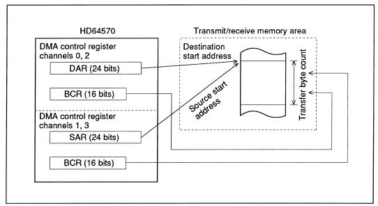
Figure 6-10 Memory-to/from-MSCI Single-Block Transfer Mode
