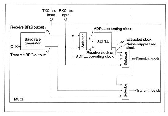
Figure 5-33 Selecting Transmit and Receive Clock Sources
