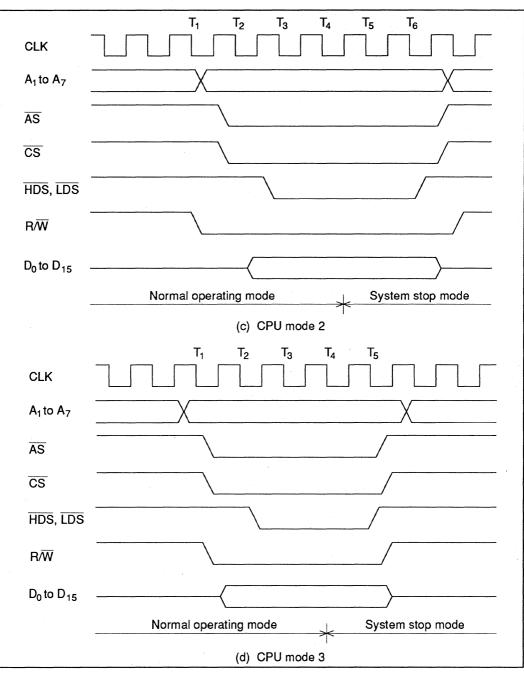
Figure 3-3 Timing of Transition to System Stop Mode (cont)
