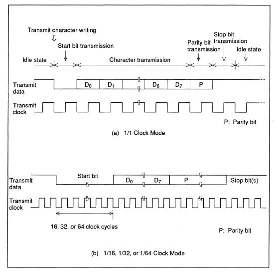
Figure 5-13 Transmission Operation
