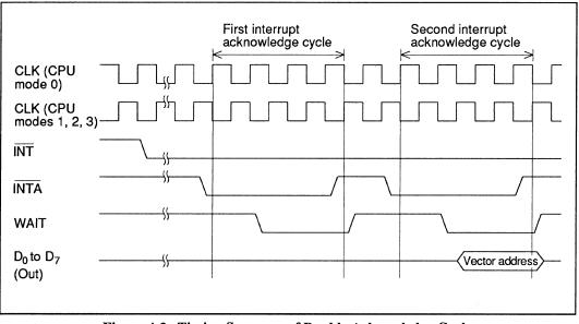
Figure 4-3 Timing Sequence of Double Acknowledge Cycle
