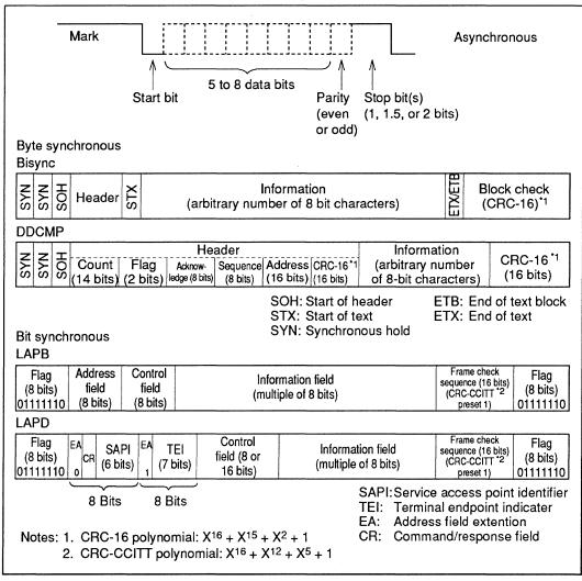
Figure 1-7 Examples of Transmission Formats
