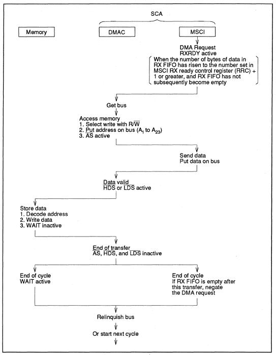
Figure 1-20 Receive DMA Operation (CPU modes 2 and 3)
