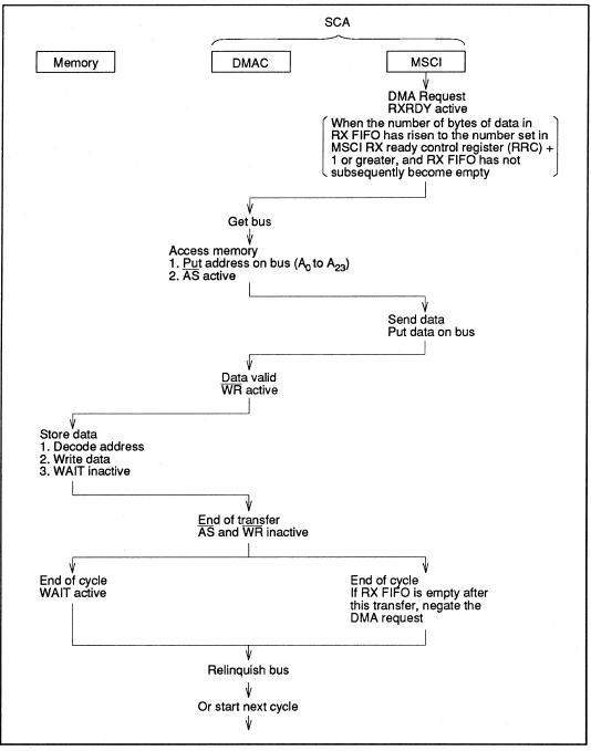
Figure 1-18 Receive DMA Operation (CPU mode 1)
