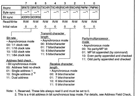
I his is a 4-bit address in bit synchronous loop mode. For details, see Address Field Check in sections 5.3.3, Bit Synchronous Mode and 5.3.4, Bit Synchronous Loop Mode. Bits 7–6 (BRATE1–BRATE0/ADDRS1-ADDRS0: Bit Rate/Address Field Check): Specify the relationship between the bit rate and the transmit/receive clock in asynchronous mode, and the checking method for the address field in bit synchronous mode. These bits are used for both transmission and reception.
