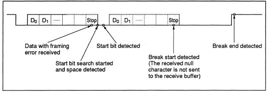
Figure 5-20 Break Detection by the Receiver
