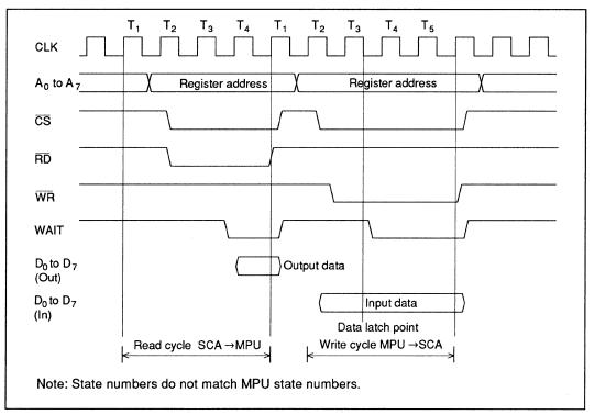
Figure 3-9 Slave Mode Bus Timing Sequence in CPU Mode 1
