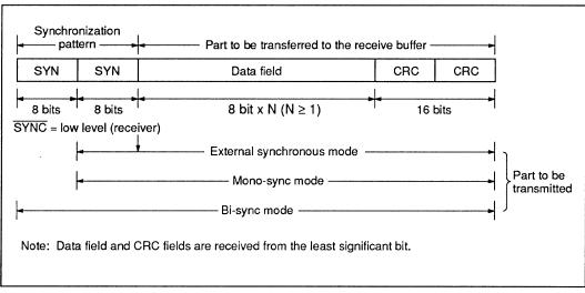
The character format for byte synchronous mode is shown in figure 5-22.
