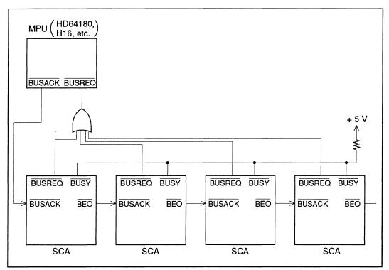
Figure 1-23 Daisy-Chained Multi-Channel System (example)
