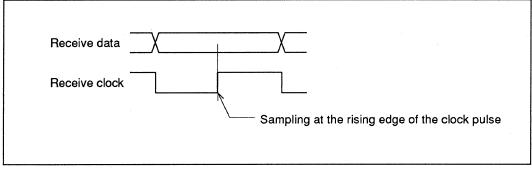
Figure 5-11 Data Sampling Timing (1/1 clock mode)
