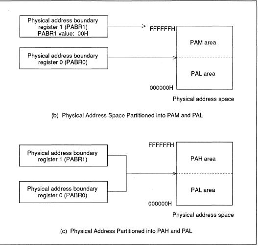
Figure 8-2 Boundary Address Setting Examples (cont)
