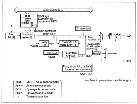
Figure 1-11 Block Diagram of the MSCI Transmitter
