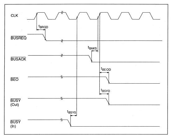
Figure 10-13 CPU Mode 1, 2, 3 Bus Arbitration Timing
