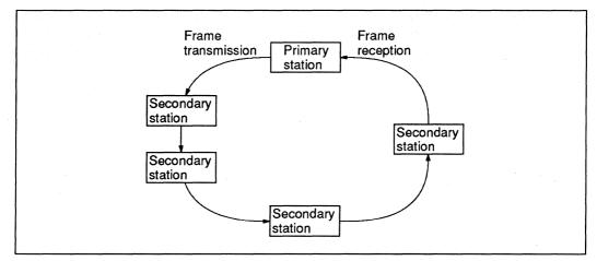
Figure 5-28 Relationship between Primary and Secondary Stations in Bit Synchronous Loop Mode
