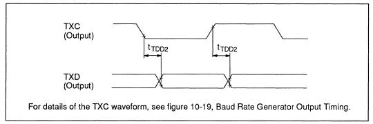
Figure 10-15 Transmit Timing (TXC output)
