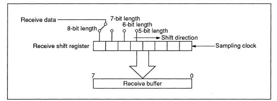
Figure 5-16 Character Assembly in the Receive Shift Register
