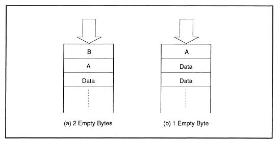
Figure 5-8 Empty Data Byte Arrangement in Transmit Buffer
