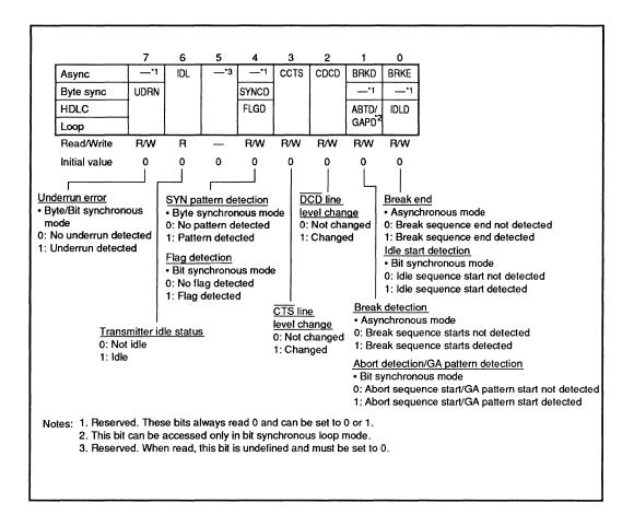
Bit 7 (UDRN: Underrun Error): Indicates whether or not an underrun error has occurred in byte or bit synchronous mode. (In asynchronous mode, underrun errors do not occur.) This bit is cleared when 1 is written to this bit position.
