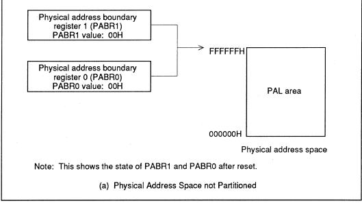
Figure 8-2 Boundary Address Setting Examples
