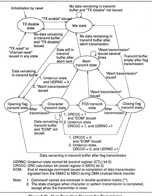
Figure 5-26 State Transition Diagram for Transmission in Bit Synchronous HDLC Mode
