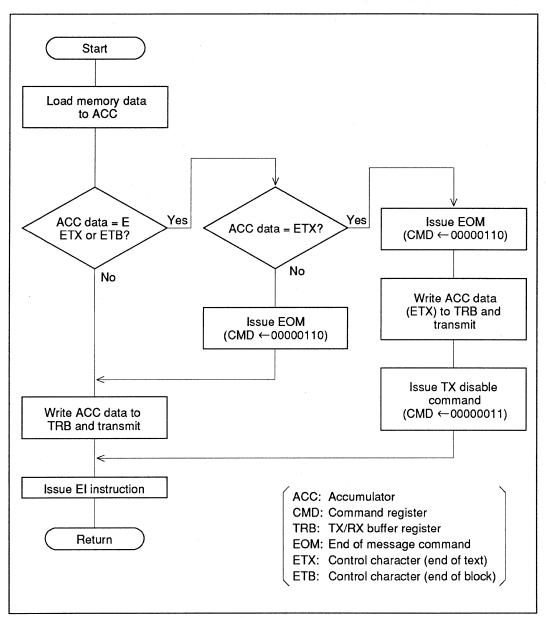
Figure 9-1 TXRDY Interrupt Processing Routine (using HD64180)
