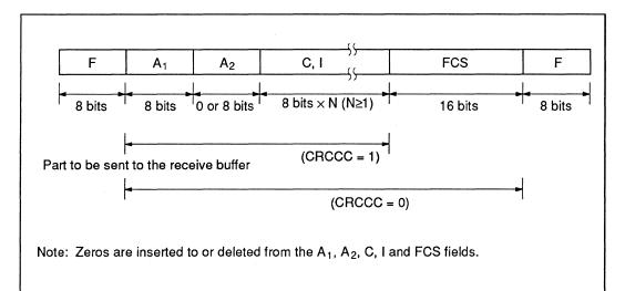
Figure 5-25 Message Format for Bit Synchronous Mode
