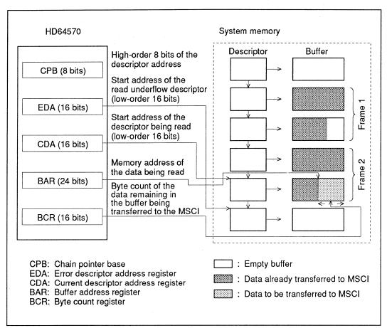
Memory-to-MSCI chained-block transfer mode is shown in figure 6-13.
