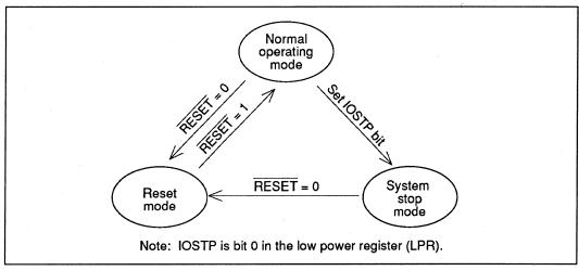
Figure 3-1 Chip Operating Mode Transitions
