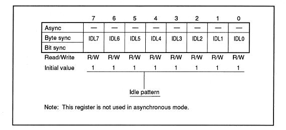
Bits 7–0 (IDL7–IDL0: Idle Pattern): The function of these bits is described below.
