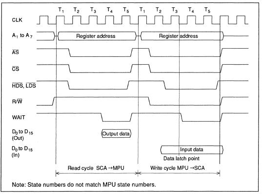
Figure 3-11 Slave Mode Bus Timing Sequence in CPU Mode 3
