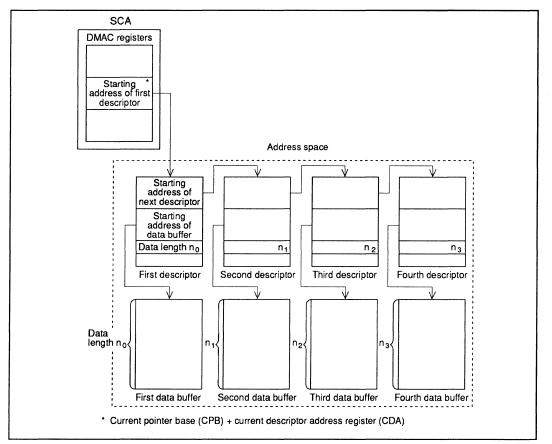
Figure 1-21 DMA Buffer Chaining
