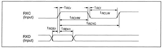
Figure 10-16 Receive Timing (RXC input)
