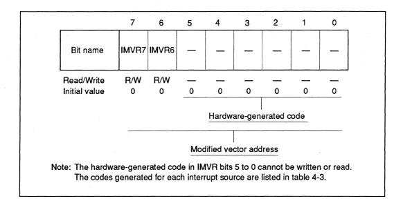
Bits 7 and 6 are cleared to 0 by a reset. Bits 5 to 0 always read 0. When writing to IMVR, write 0 in bits 5 to 0.
