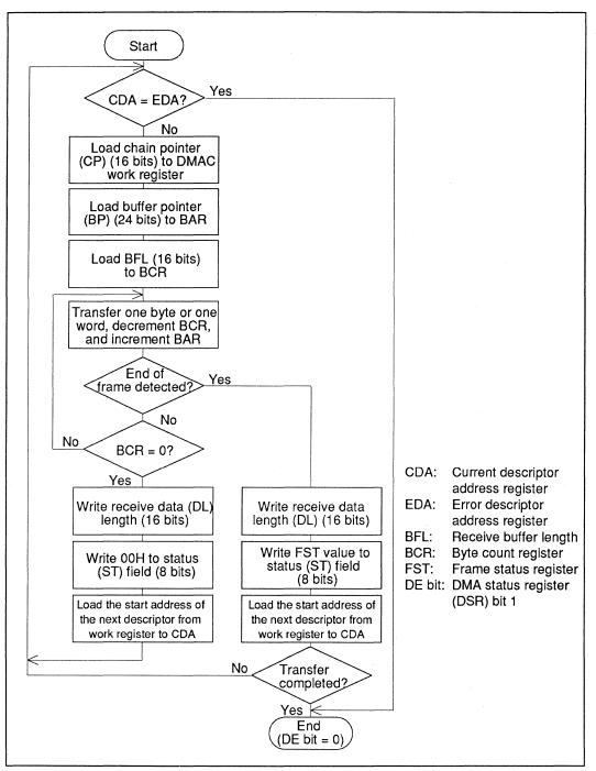
Figure 6-19 Operation Flow in MSCI-to-Memory Chained-Block Transfer Mode
