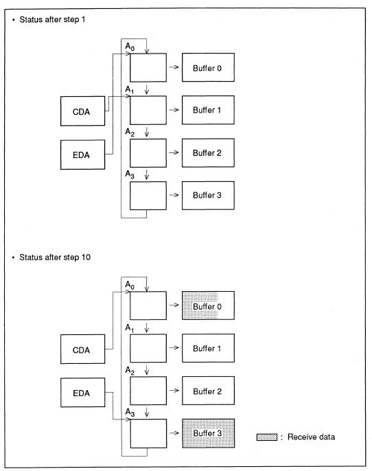
Figure 6-21 MSCI-to-Memory Chained-Block Multi-Frame Transfer (part of a buffer released during reception operation)
