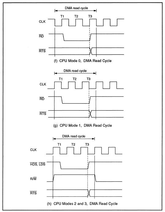
Figure 5-1 Modem Control Signal Timing (cont)
