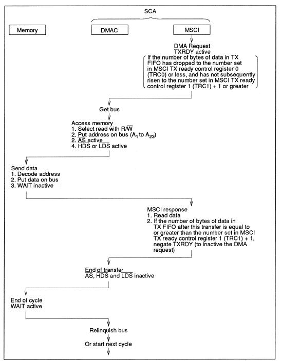
Figure 1-19 Transmit DMA Operation (CPU modes 2 and 3)
