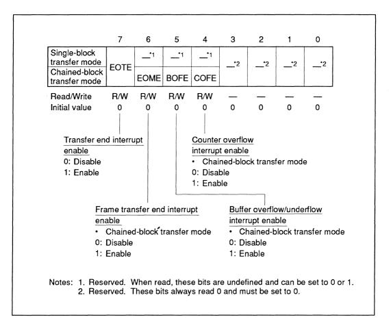
Bit 7 (EOTE: Transfer End Interrupt Enable): Enables or disables a DMA normal end interrupt (DMIB) caused by the EOT bit of DSR in either single-block transfer mode or chained-block transfer mode as follows.
