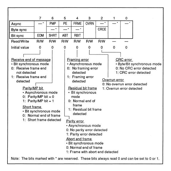
Bit 7 (EOM: Receive End of Message): Indicates whether or not a receive frame has ended in bit synchronous mode. This bit is cleared when 1 is written to this bit position.
