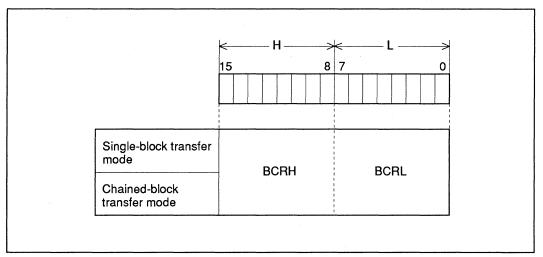
Figure 6-6 Byte Count Register
