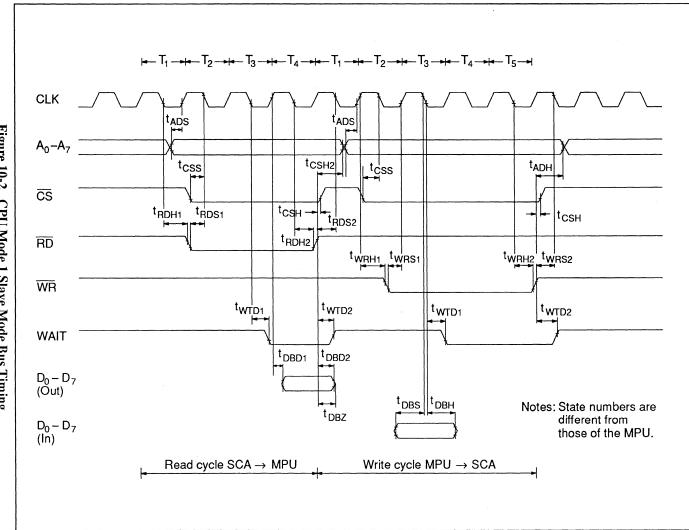
Figure 10-2 **CPU Mode 1 Slave Mode Bus Timing**
