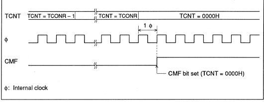
Figure 7-3 Timer Output Timing
