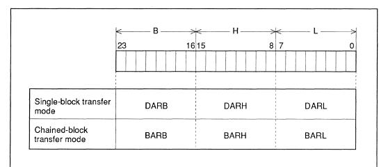
Figure 6-1 Destination Address Register/Buffer Address Register
