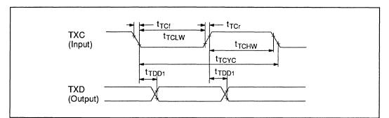
Figure 10-14 Transmit Timing (TXC input)
