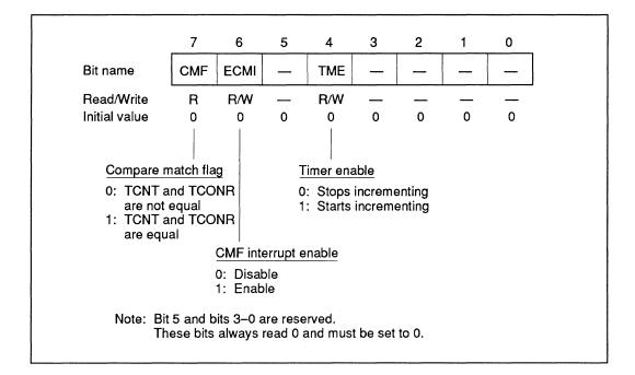
**Bit 7 (CMF: Compare Match Flag):** Indicates whether or not the TCNT value matches the timer constant register (TCONR) value. This bit is cleared when TCNT is read after TCSR. Other instructions can be inserted between the TCSR and TCNT read instructions. This bit is also cleared at reset or in system stop mode.
