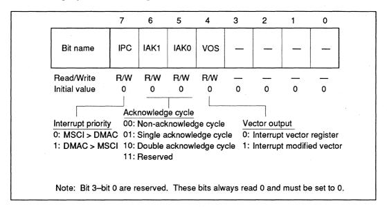
Bit 7 (IPC: Interrupt Priority Control): Controls the priority order of interrupt sources. This bit is cleared to 0 at a reset.
