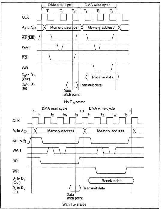
Figure 3-15 Master Mode Bus Timing Sequence in CPU Mode 1
