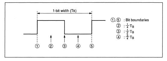
Note: An enter search mode command is automatically issued; the ADPLL automatically enters search mode and attempts to reestablish synchronization at the next transition point if the ADPLL detects no level transition in FM-code receive data in the successive two bit cycles  $(-1/4T_B \text{ to } 1/4T_B \text{ for FM0} \text{ and FM1}, \text{ and } 1/4T_B \text{ to } 3/4T_B \text{ for Manchester}).$
