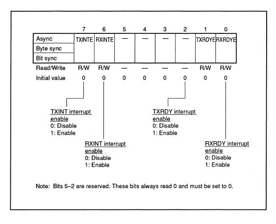
Bit 7 (TXINTE: TXINT Interrupt Enable): The function of this bit is described below.
