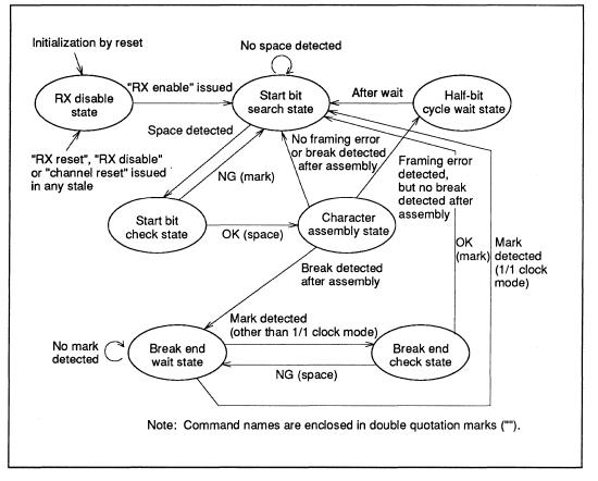
Figure 5-14 State Transition Diagram for Reception in Asynchronous Mode
