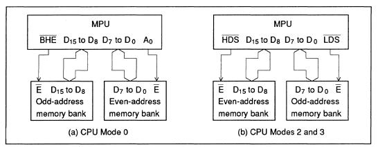
Figure 3-7 Data Bus Mapping onto Memory Banks in CPU Modes 0, 2, and 3
