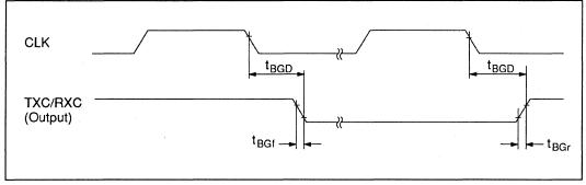
Figure 10-19 Baud Rate Generator Output Timing ( $f_{BRG} \neq f_{CLK}$ )
