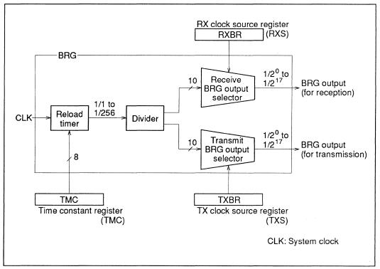
Figure 5-43 Baud Rate Generator Block Diagram
