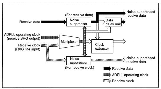
Figure 5-41 Data and Clock Signal Flow for Receive Clock Noise Suppression
