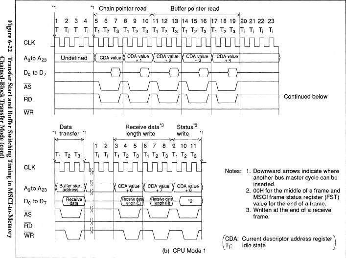
Transfer Start and Buffer Switching Timing in MSCI-to-Memory Chained-Block Transfer Mode (cont)
