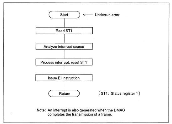
Figure 9-5 TXINT Interrupt Processing Routine (using HD64180)
