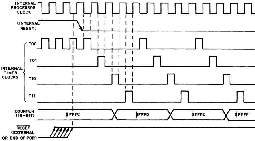
Fig. 16 - Timer State Timing Diagram For Reset
