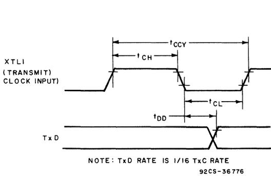
Fig. 23 - Transmit timing waveforms with external clock.
