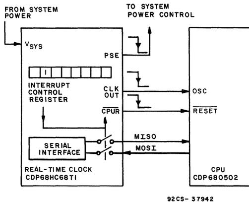
Fig. 4 - Power-down functional diagram.
