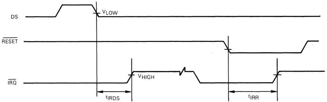
NOTE:  $V_{\text{HIGH}} = V_{DD} - 2.0 \text{ V}$ ,  $V_{\text{LOW}} = 0.8 \text{ V}$ , for  $V_{DD} = 5.0 \text{ V} \pm 10\%$
