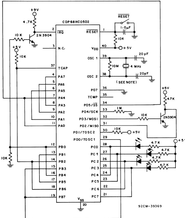
NOTE: THE RC OSCILLATOR OPTION MAY ALSO BE USED IN THIS CIRCUIT
