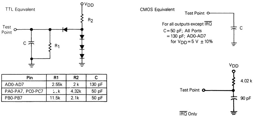
Fig. 2 - Equivalent test loads.
