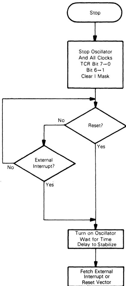
Fig. 16 - Stop function flowchart.
