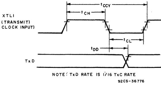
**Fig. 26 - Transmit-timing waveforms with external clock.**
