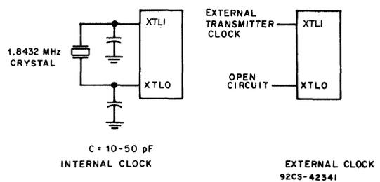
Fig. 26 - Transmitter clock generation.
