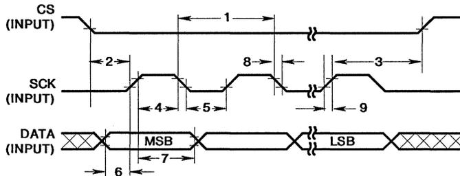
**Timing Characteristics**  $V_{DD} = 5.0 V_{DC} \pm 10\%$ ,  $V_{SS} = 0 V_{DC}$ ,  $T_A = -40^\circ\text{C}$  to  $+85^\circ\text{C}$
