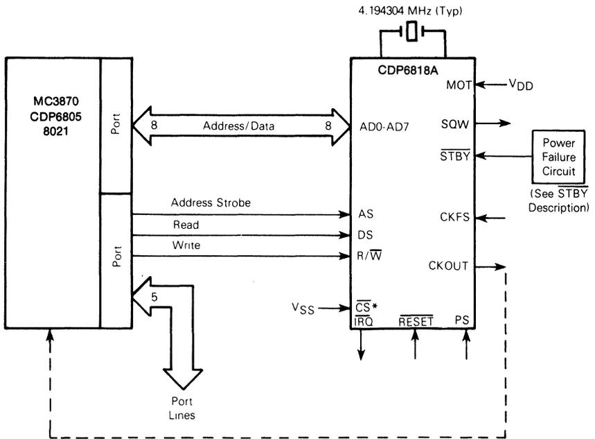
\* NOTE:  $\overline{CS}$  can be controlled by a port pin (if available).
