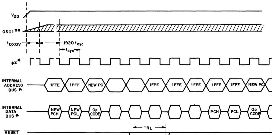
\* INTERNAL TIMING SIGNAL AND BUS INFORMATION NOT AVAILABLE EXTERNALLY
