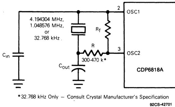
Fig. 10 - Crystal oscillator connection.
