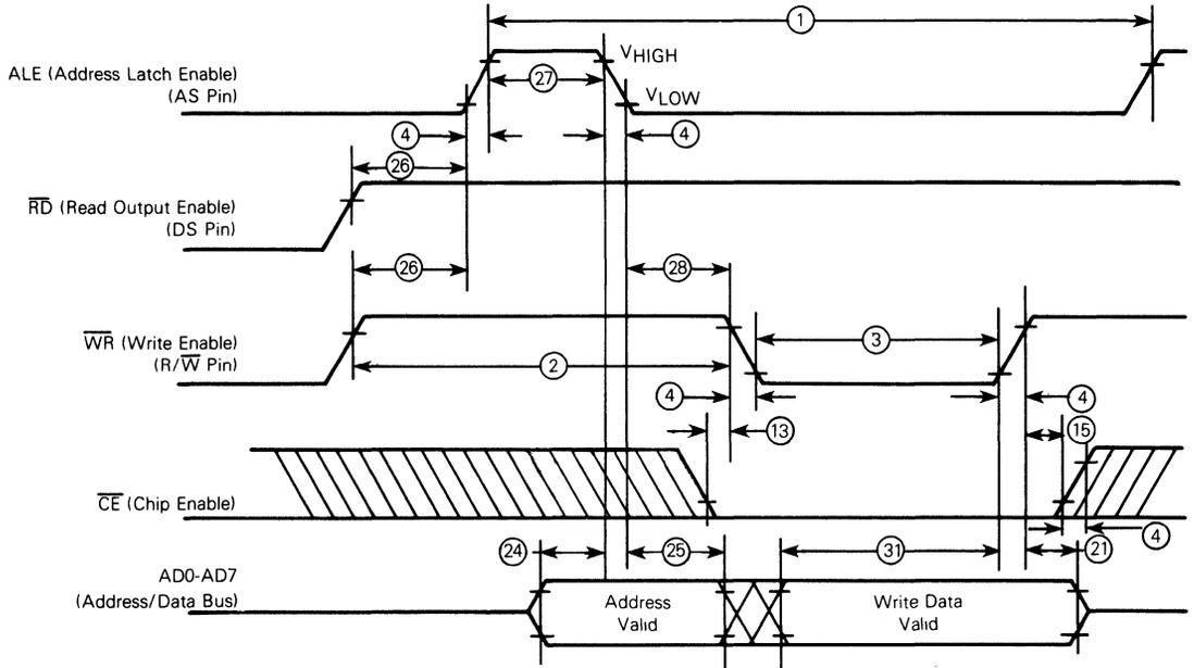
NOTE:  $V_{HIGH} = V_{DD} - 2V$ ,  $V_{LOW} = 0.8V$ , for  $V_{DD} = 5V \pm 10\%$
