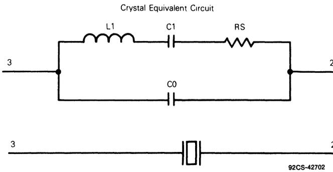
Fig. 11 - Crystal parameters.
