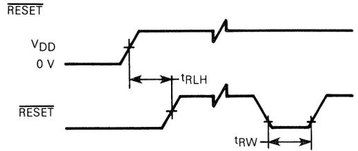
Fig. 6 - Control timing diagrams.
