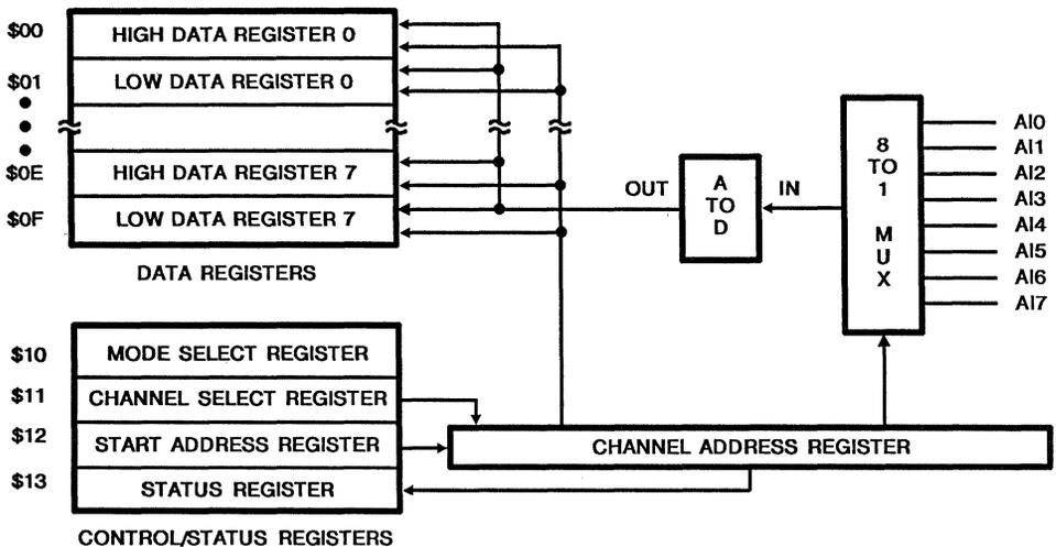
FIGURE 2. A PROGRAMMER'S MODEL OF THE CDP68HC68A2
