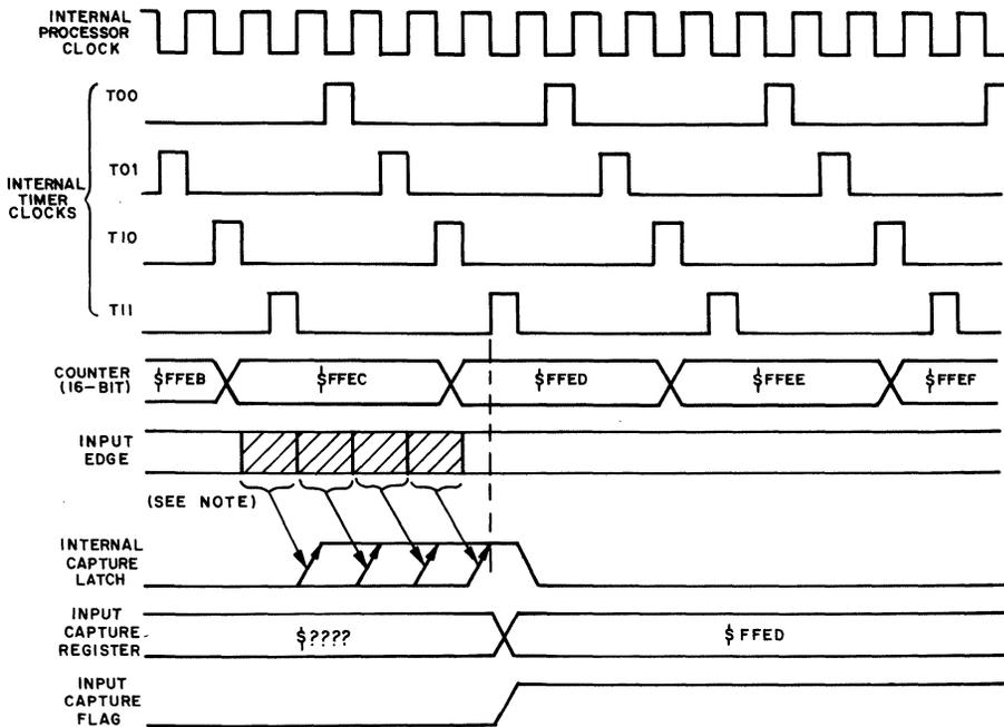
Fig. 17 - Timer State Timing Diagram For Input Capture
