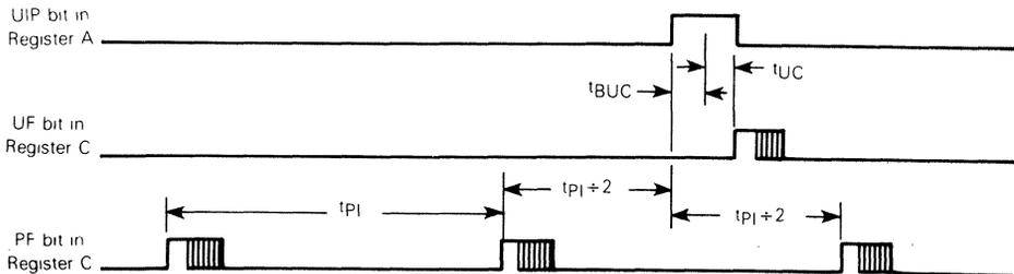
t<sub>PI</sub> = Periodic Interrupt Time Interval (500 ms, 250 ms, 125 ms, 62.5 ms, etc. per Table 5)
