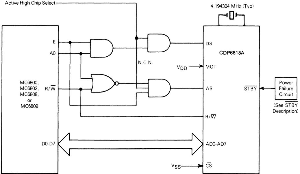
Fig. 20 - CDP6818A interfaced with Motorola Processors.
