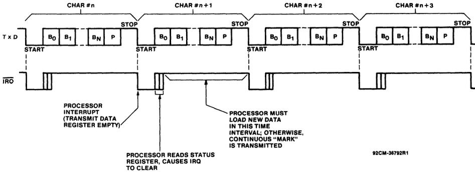
Fig. 8 - Continuous data transmit.
