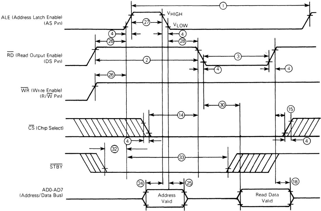
Fig. 3 - Bus read timing competitor multiplexed bus.
