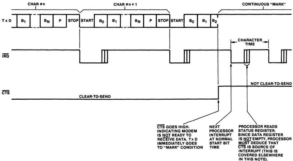
Fig. 11 - Effect of CTS on transmitter.
