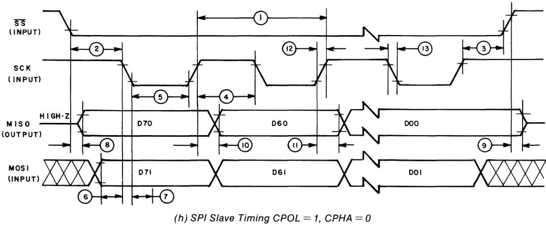
NOTE: MEASUREMENT POINTS ARE  $V_{OL}$ ,  $V_{OH}$ ,  $V_{IL}$  AND  $V_{IH}$
