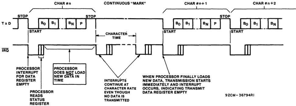
Fig. 10 - Transmit data register not loaded by processor.
