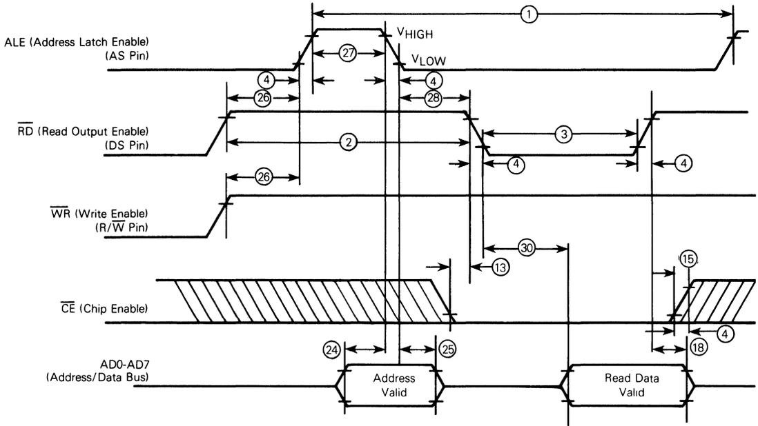
Fig. 4 - Bus READ timing competitor multiplexed bus.
