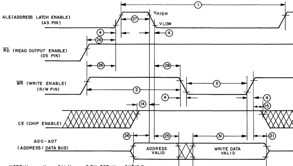
NOTE:  $V_{HIGH} = V_{DD} - 2.V$ ,  $V_{LOW} = 0.8V$ , FOR  $V_{DD} = 5V \pm 10\%$
