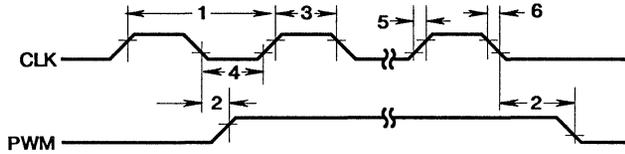
Timing Characteristics  $V_{DD} = 5.0 V_{DC} \pm 10\%$ ,  $V_{SS} = 0 V_{DC}$ ,  $T_A = -40^\circ C$  to  $+85^\circ C$
