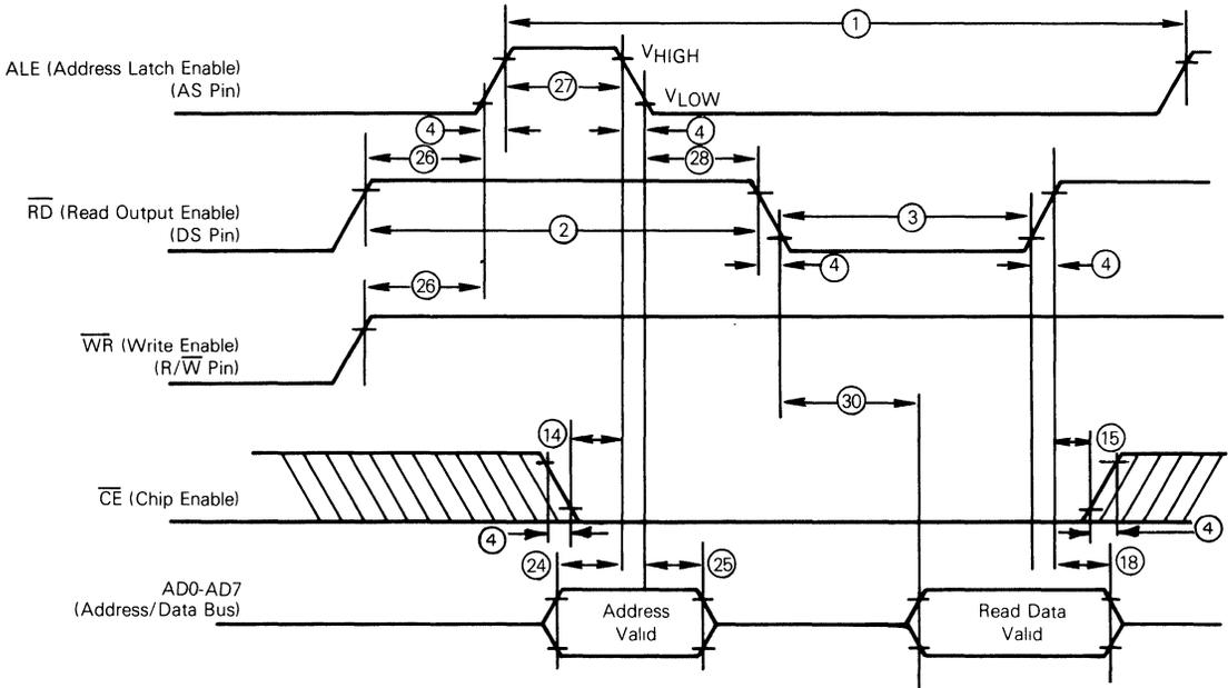
Fig. 3 — Bus-read timing competitor multiplexed bus.
