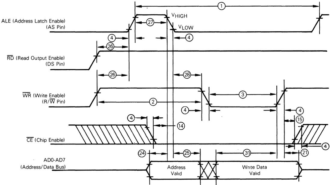
NOTE:  $V_{HIGH} = V_{DD} - 2.0\text{ V}$ ,  $V_{LOW} = 0.8\text{ V}$ , for  $V_{DD} = 5.0\text{ V} \pm 10\%$
