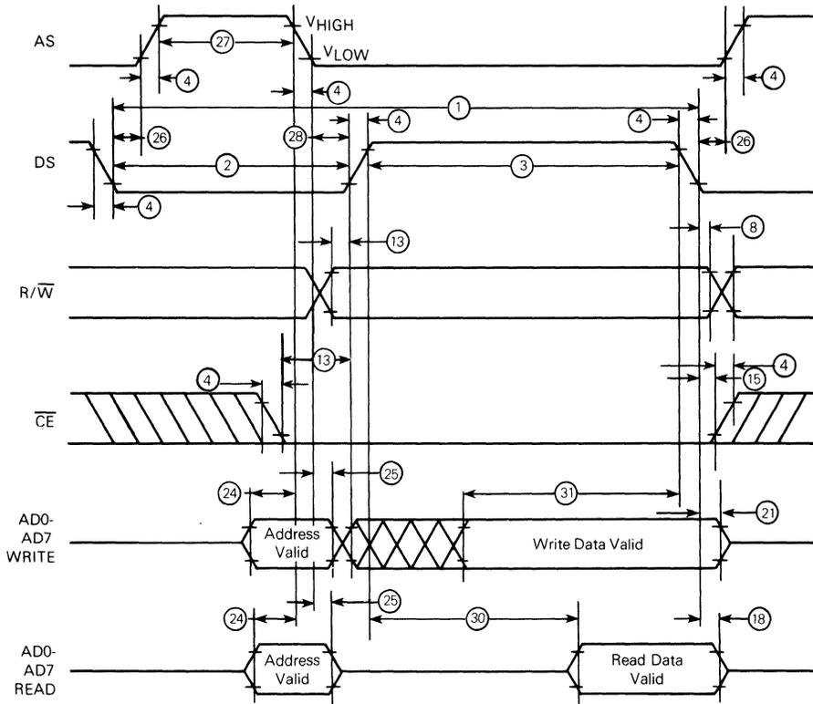
NOTE:  $V_{HIGH}=V_{DD}-2\text{ V}$ ,  $V_{LOW}=0.8\text{ V}$ , for  $V_{DD}=5\text{ V} \pm 10\%$
