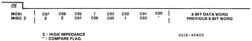
At the time the eighth data bit is strobed into the data pins (D0-D7) will change as indicated in Fig. 7.
