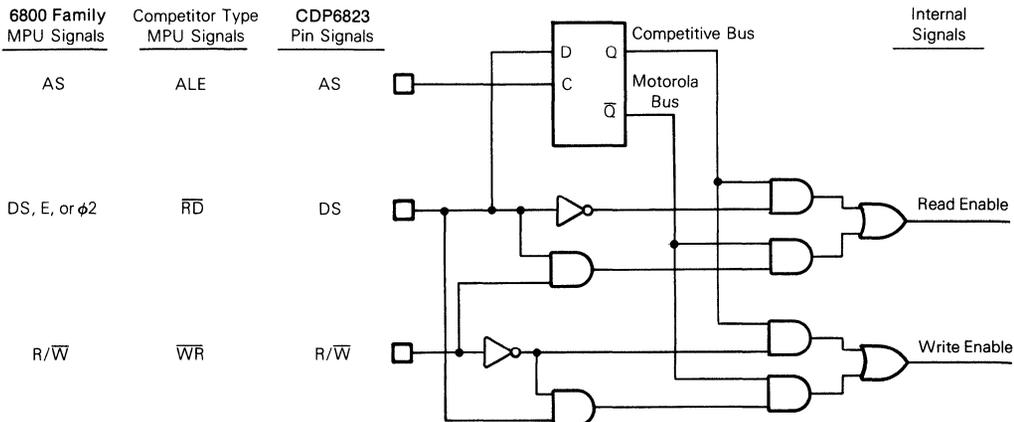
Fig. 7 - Functional diagram of MOTEL circuit.
