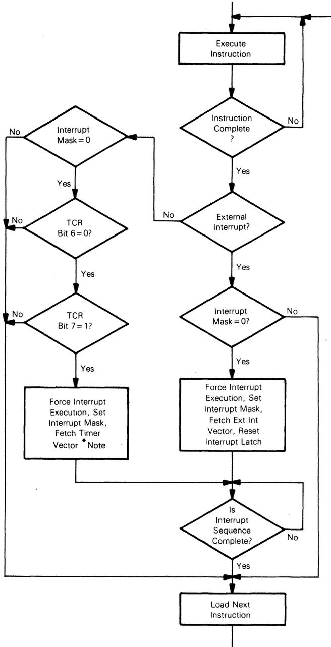
\* NOTE: The clear of TCR bit 7 must be accomplished with software.
