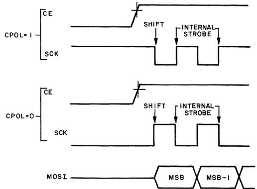
NOTE: "CPOL" IS A BIT THAT IS SET IN THE MICROCOMPUTER'S CONTROL REGISTER
