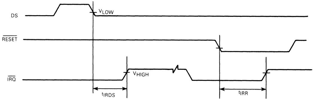
NOTE:  $V_{HIGH} = V_{DD} - 2.0$  V,  $V_{LOW} = 0.8$  V, for  $V_{DD} = 5.0$  V  $\pm 10\%$
