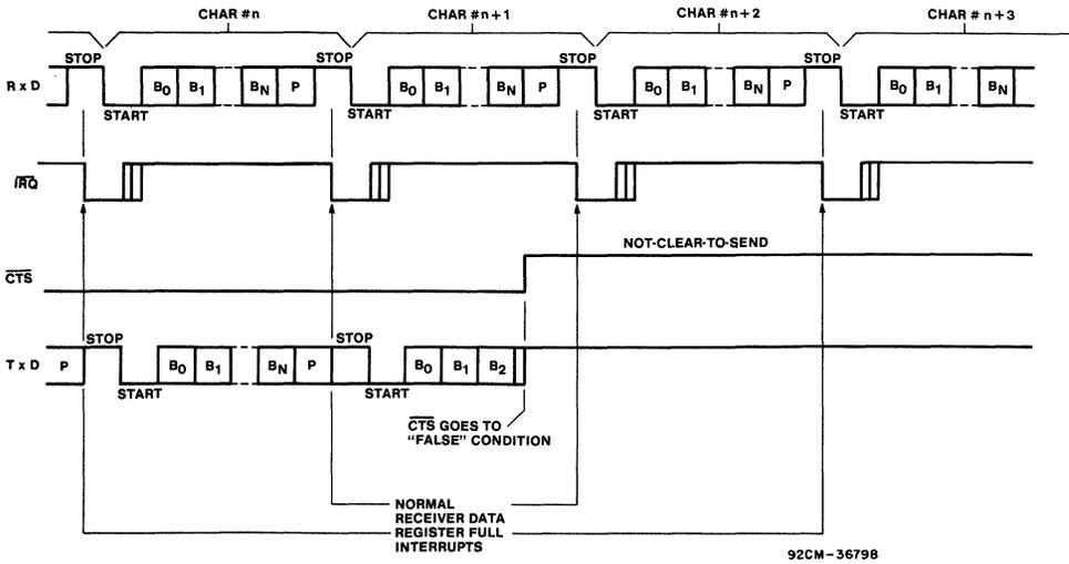
Fig. 14 - Effect of  $\overline{\text{CTS}}$  on echo mode.
