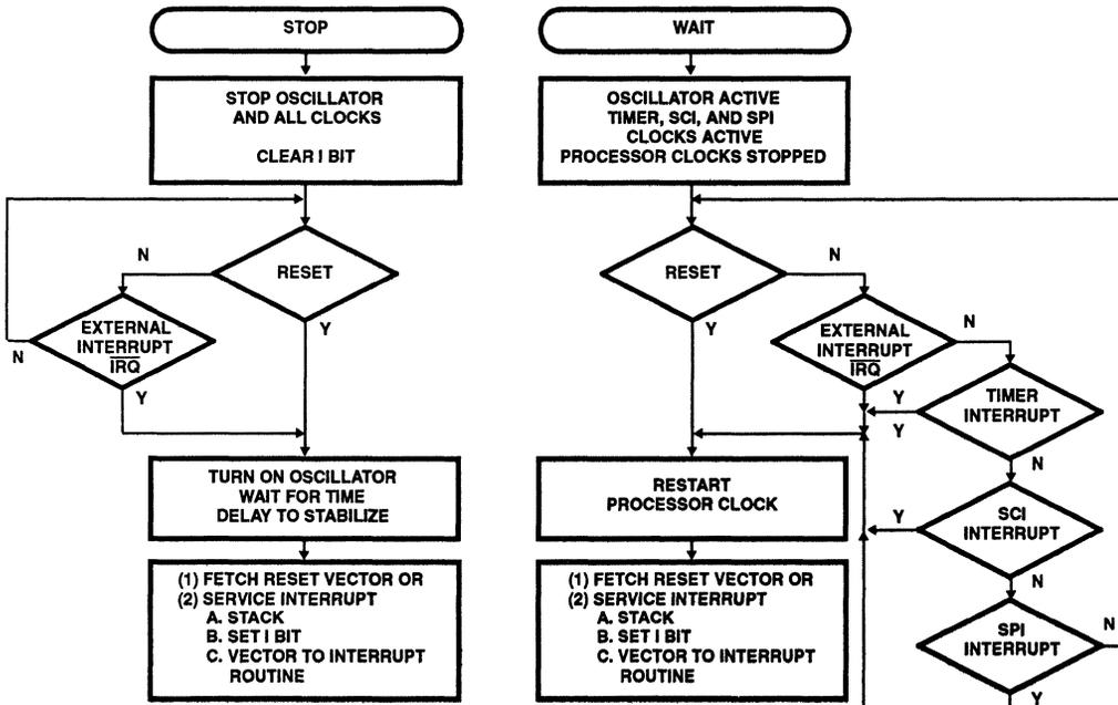
FIGURE 13. STOP/WAIT FLOW DIAGRAM
