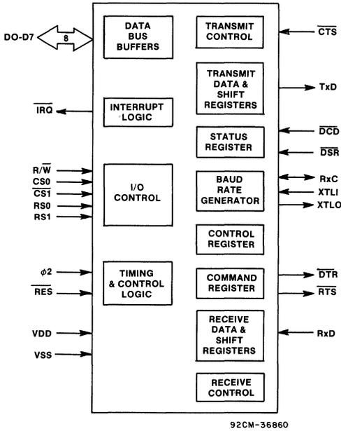
Fig. 1 - CDP65C51/51A interface diagram
