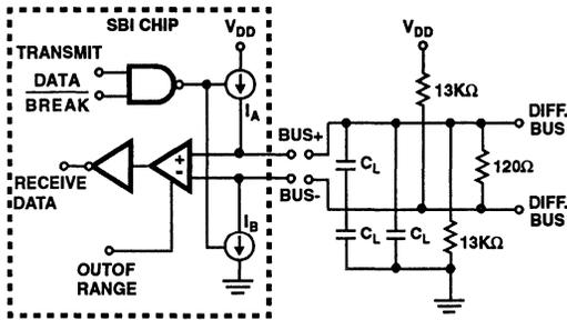
FIGURE 4. DIFFERENTIAL DRIVER/RECEIVER
