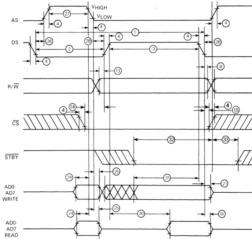
Note: V<sub>HIGH</sub> = V<sub>DD</sub> - 2.0 V, V<sub>LOW</sub> = 0.8 V, for V<sub>DD</sub> = 5.0 V ± 10% for outputs only.
