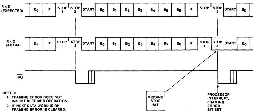
Fig. 15 - Framing error.
