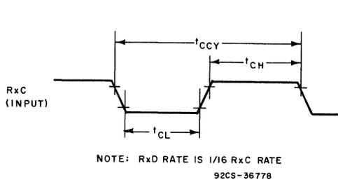
Fig. 25 - Receive external clock timing waveforms.
