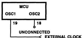
FIGURE 3F. EXTERNAL CLOCK SOURCE CONNECTIONS
