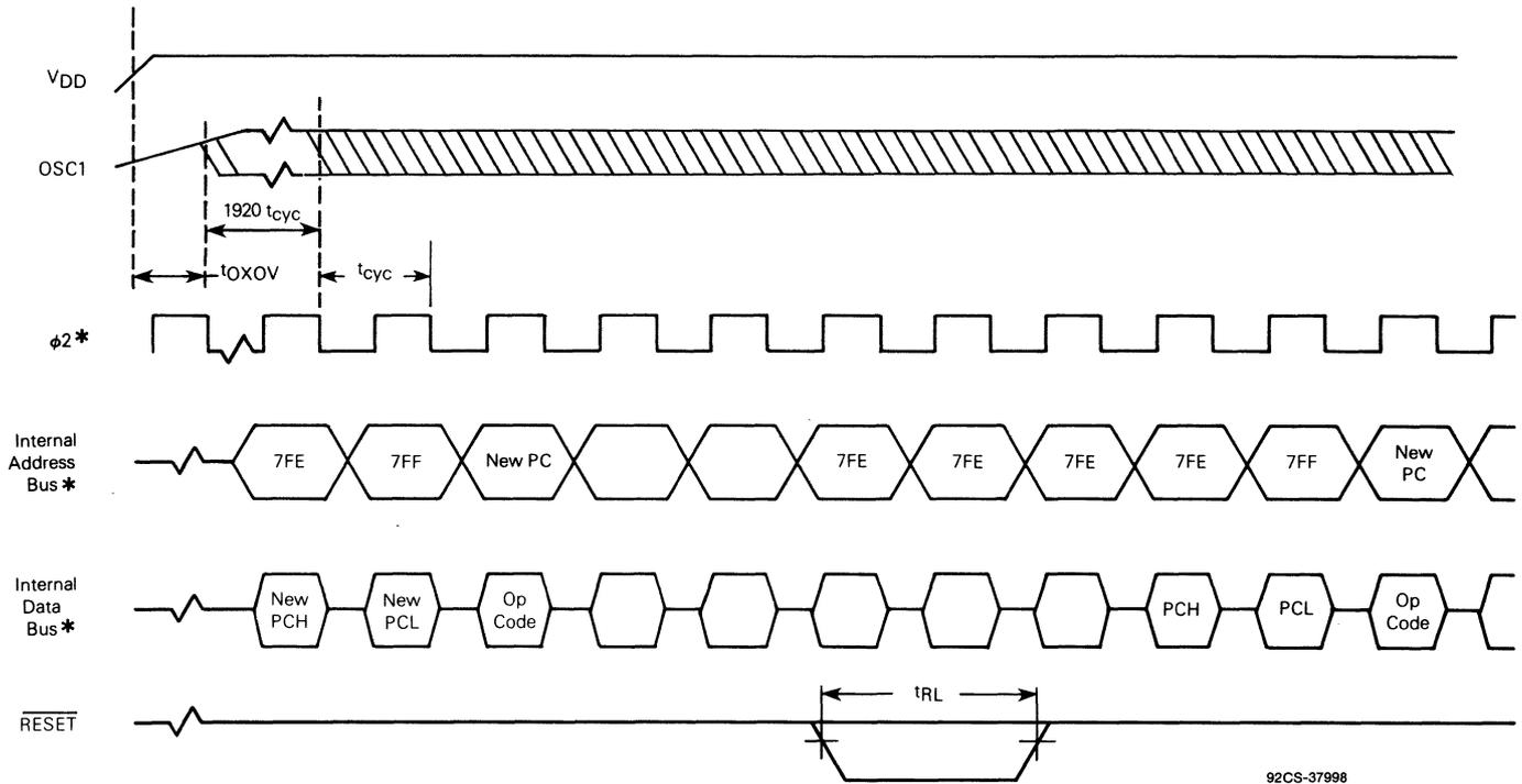
\* Internal timing signal not available externally.
