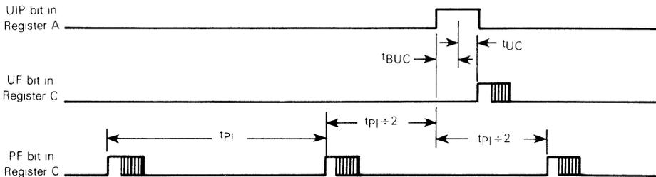
$t_{PI}$  = Periodic Interrupt Time Interval (500 ms, 250 ms, 125 ms, 62.5 ms, etc. per Table 5)
