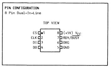
separate lines are used the DO output pin is valid only in the read mode and is in the high impedance state in all other modes, thus eliminating bus contention. Seven instructions may be executed and the instruction length will be thirteen bits when using the 256 x 8 organization and twelve bits when the 128 x 16 organization is used. The instruction format has a logical 1 as a start bit, four bits as an opcode and either seven or eight address bits.
