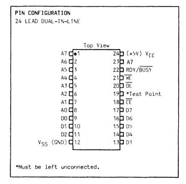
RAM. Since the address and data are internally latched and the RDY/ $\overline{BUSY}$  signal is available, the ER5902I frees the system for other tasks during the programming cycle. The read/write logic is designed such that bus contention will be minimized by use of  $\overline{OE}$  and  $\overline{CE}$  inputs.
