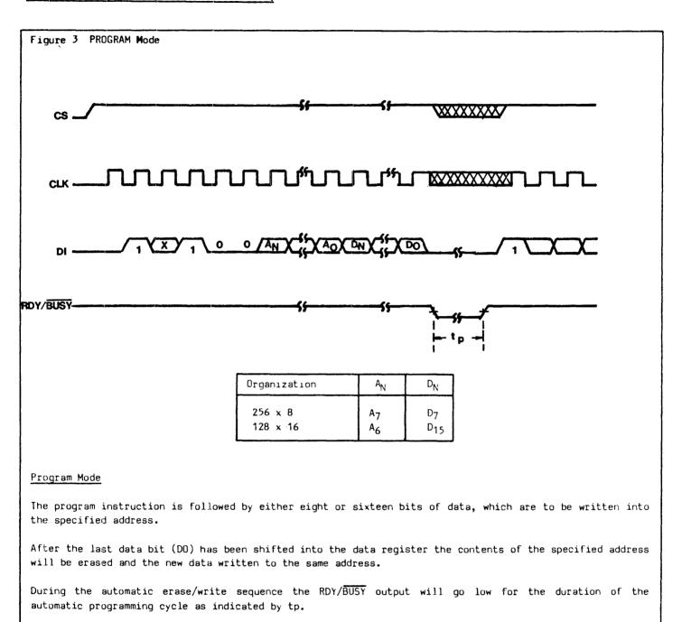
During a program cycle the internal erase and write operations occur automatically and are self-timed on the device. A single memory location may also be erased by programming that address with all "1's".
