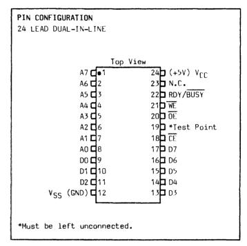
RAM. Since the address and data are internally latched and the RDY/BUSY signal is available, the ER5902 frees the system for other tasks during the programming cycle. The read/write logic is designed such that bus contention will be minimized by use of  $\overline{\text{OE}}$  and  $\overline{\text{CE}}$  inputs.
