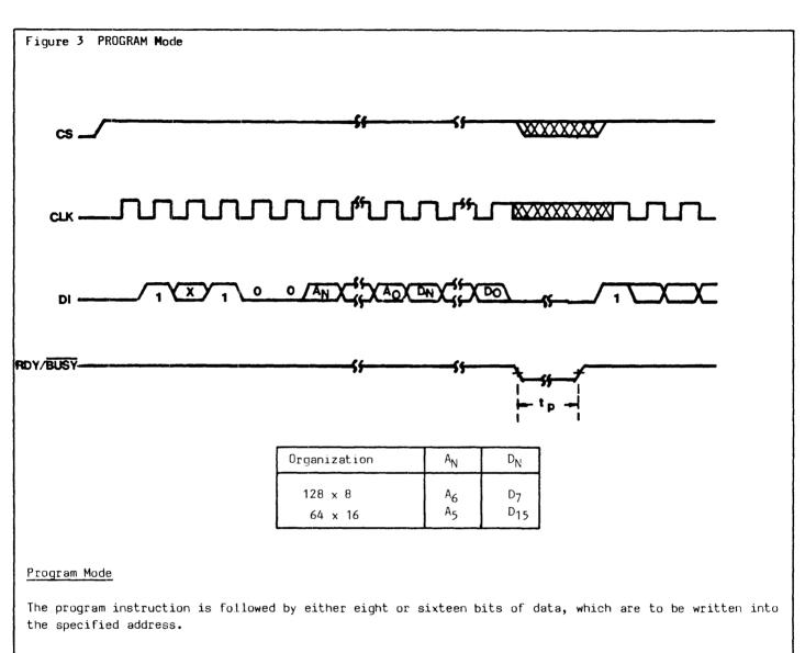
After the last data bit (DD) has been shifted into the data register the contents of the specified address will be erased and the new data written to the same address.
