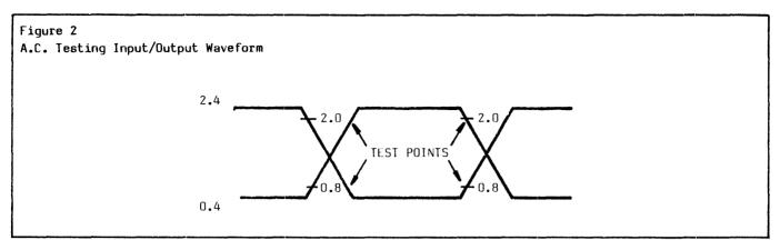
AC Testing inputs are driven at 2.4V for a logic 1 and 0.4V for a logic 0 timing measurements are made at 2.0V for a logic 1 and 0.8V for a logic 0.
