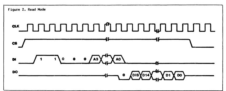
The READ instruction is the only instruction which outputs serial data on the DO pin. Only during the READ mode is the output pin (DO) valid. During all other modes the DO pin is in tri-state, eliminating bus contention. A dummy bit (logical "O") precedes the 16-bit output string. The output data changes during the high state of the system clock.
