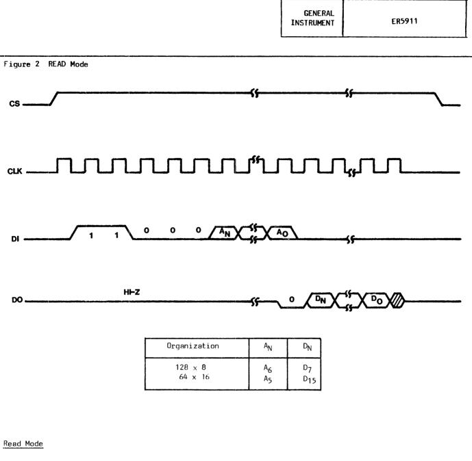
The READ instruction is the only instruction which outputs serial data on the DO pin. After a READ instruction is received, the instruction and address are decoded, followed by data transfer from the memory register into a serial-out shift register. A dummy bit (logical "O") precedes the data output string. The output data changes during the high states of the system clock.
