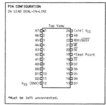
RAM. Since the address and data are internally latched and the RDY/BUSY signal is available, the ER5904I frees the system for other tasks during the programming cycle. The read/write logic is designed such that bus contention will be minimized by use of  $\overline{\text{OE}}$  and  $\overline{\text{CE}}$  inputs.
