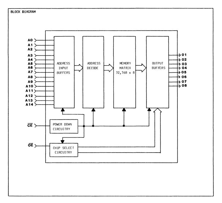
III) "ORED" chip select requirement (chip selects at pins 20 ( $\overline{CE}$ ) and 22 ( $\overline{OE}$ ) function as a logical "OR"). \*This is ideally suited for applications that have limited chip select decoding capabilities.
