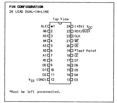
RAM. Since the address and data are internally latched and the RDY/BUSY signal is available, the ER5901 frees the system for other tasks during the programming cycle. The READ/write logic is designed such that bus contention will be minimized by use of  $\overline{OE}$  and  $\overline{CE}$  inputs.
