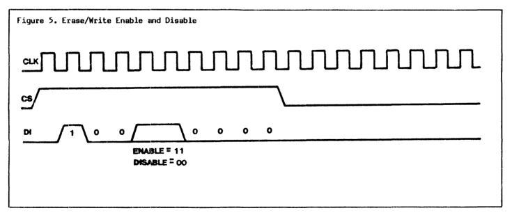
Programming must be preceded once by an Erase/Write Enable (EWEN) instruction. Programming remains enabled until an Erase/Write Disable (EWDS) instruction is executed. The programming disable instruction is provided to protect against accidental data disturb. Execution of a READ instruction is independent of both EWEN and EWDS instructions. The device powers up in the Erase/Write Disable (EWDS) mode.
