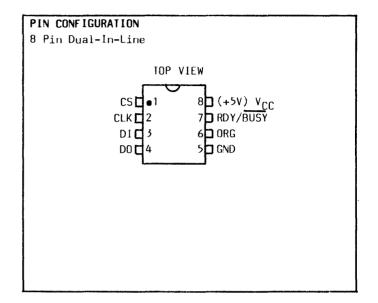
used the DO output pin is valid only in the read mode and is in the high impedance state in all other modes, thus eliminating bus contention. Five instructions may be executed and the instruction length will be twelve bits when using the 128 x 8 organization and eleven bits when the 64 x 16 organization is used. The instruction format has a logical 1 as a start bit, four bits as an opcode and either six or seven address bits.
