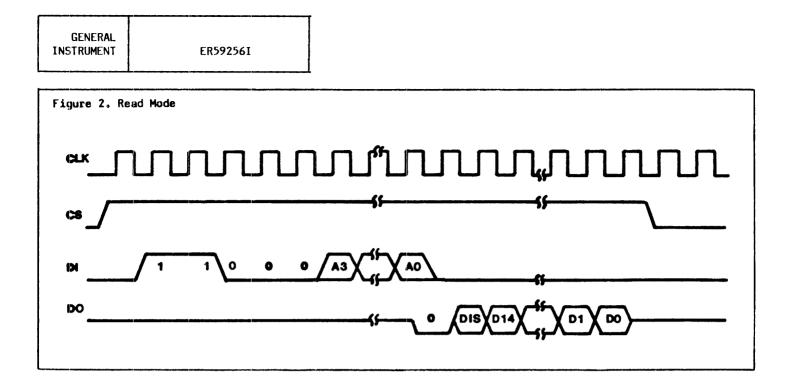
The READ instruction is the only instruction which outputs serial data on the DO pin. Only during the READ mode is the output pin (DO) valid. During all other modes the DO pin is in tri-state, eliminating bus contention. A dummy bit (logical "O") precedes the 16-bit output string. The output data changes during the high state of the system clock.
