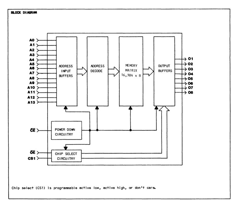
III) \*\*"ORED" chip select requirement (chip selects at pins 20 (CE) and 22 (OE) function as a logical "OR").
