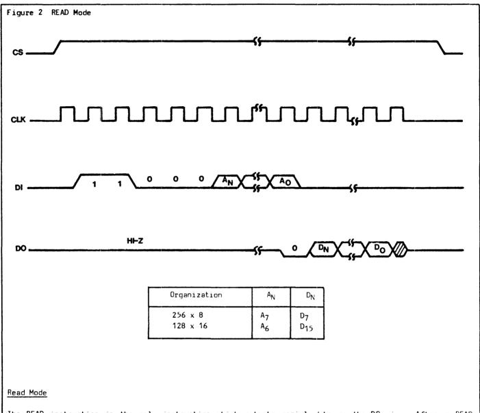
The READ instruction is the only instruction which outputs serial data on the DO pin. After a READ instruction is received, the instruction and address are decoded, followed by data transfer from the memory register into a serial-out shift register. A dummy bit (logical "O") precedes the data output string.
