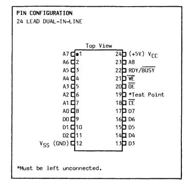
RAM. Since the address and data are internally latched and the RDY/BUSY signal is available, the ER5904 frees the system for other tasks during the programming cycle. The read/write logic is designed such that bus contention will be minimized by use of  $\overline{\text{OE}}$  and  $\overline{\text{CE}}$  inputs.
