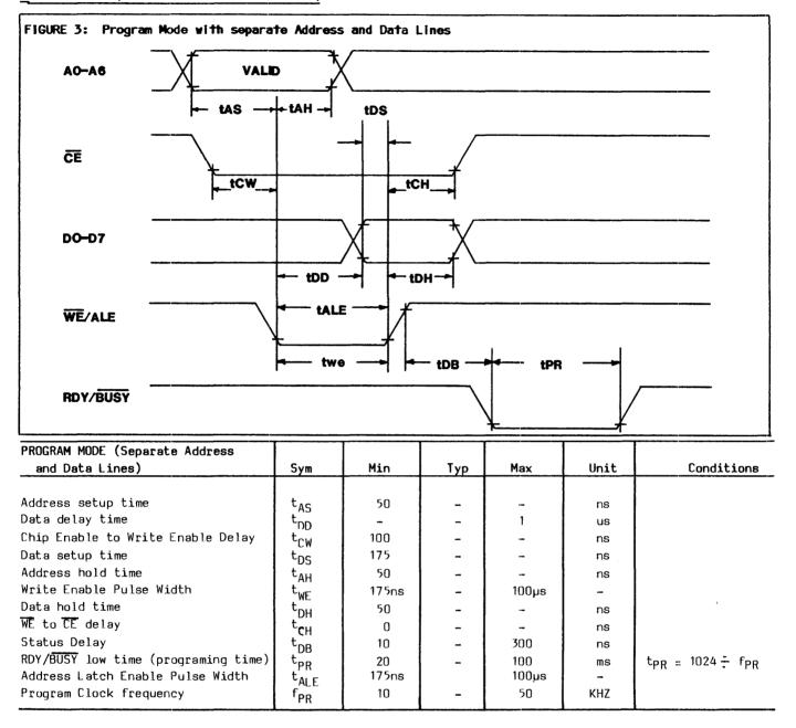
low for the duration of the programming cycle. All inputs to the ER5901I are disabled during a programming cycle.
