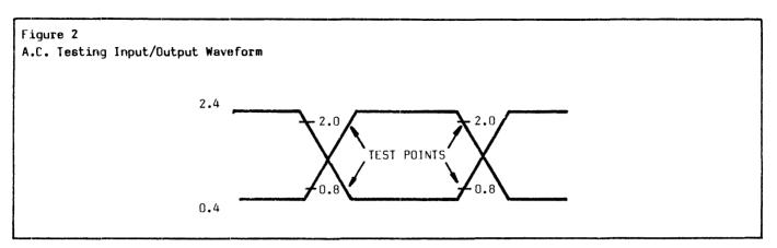
AC Testing inputs are driven at 2.4V for a logic 1 and 0.4V for a logic 0. Timing measurements are madet at 2.0V for a logic 1 and 0.8V for a logic 0.
