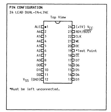
RAM. Since the address and data are internally latched and the RDY/ $\overline{\text{BUSY}}$  signal is available, the ER5901I frees the system for other tasks during the programming cycle. The READ/write logic is designed such that bus contention will be minimized by use of  $\overline{\text{OE}}$  and  $\overline{\text{CE}}$  inputs.
