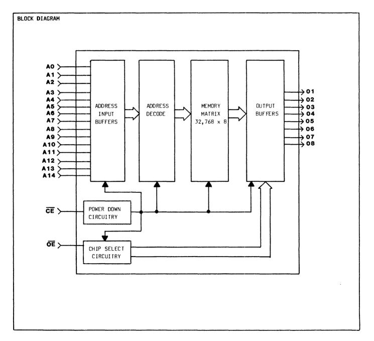
III) "ORED" chip select requirement (chip selects at pins 20 ( $\overline{CE}$ ) and 22 ( $\overline{OE}$ ) function as a logical "OR"). \*This is ideally suited for applications that have limited chip select decoding capabilities. Logic Function: ( $\overline{CE} + \overline{OE}$ ) = Chip Selected
