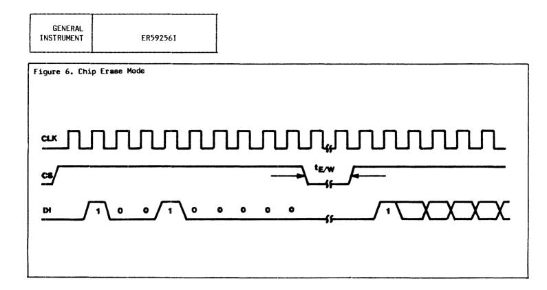
Entire chip erasing is provided for ease of programming. Erasing the chip means that all registers in the memory array have each bit set to a 1. Each register is then ready for a WRITE instruction.
