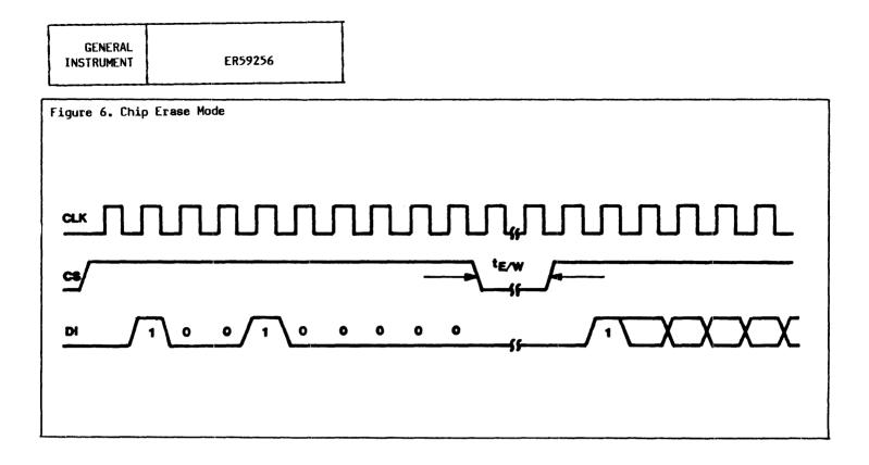
Entire chip erasing is provided for ease of programming. Erasing the chip means that all registers in the memory array have each bit set to a 1. Each register is then ready for a WRITE instruction.
