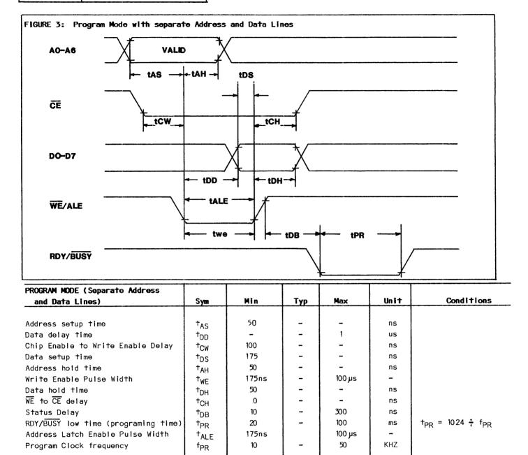
low for the duration of the programming cycle. All inputs to the ER5901 are disabled during a programming cycle.
