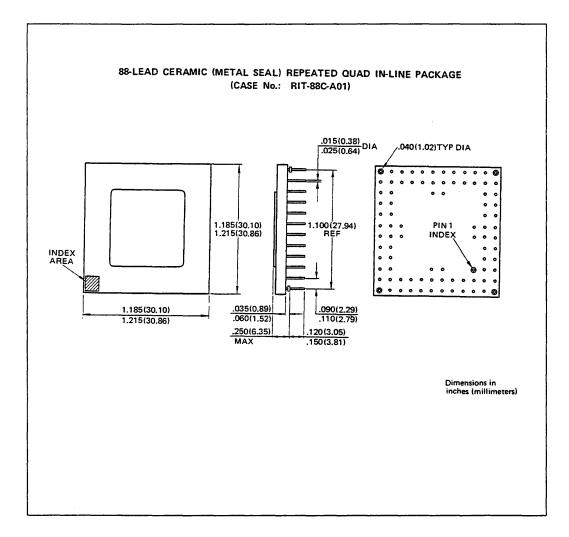
Figure 1.4.1 Dimensions of Package
