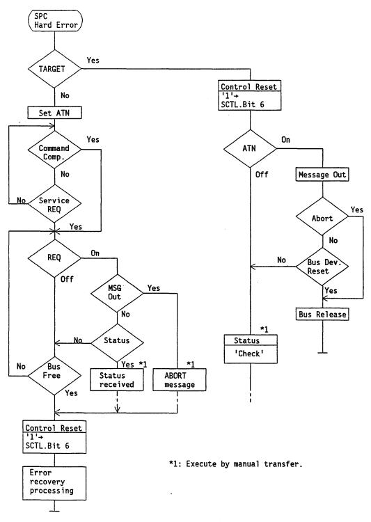
Fig. 4.11.5 Example of control processing for SPC-detected error (3)
