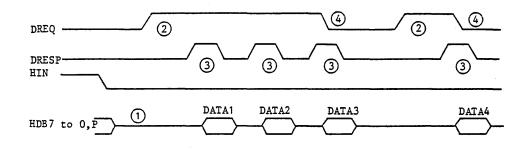
Fig. 5.2.2 Transfer to external data buffer (output operation)
