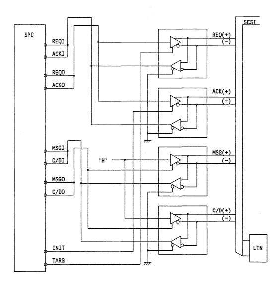
Fig. 5.1.3 Example of differential type SCSI driver/receiver circuit (continued)
