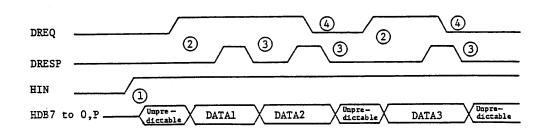
Fig. 5.2.1 Transfer with external data buffer (input operation)
