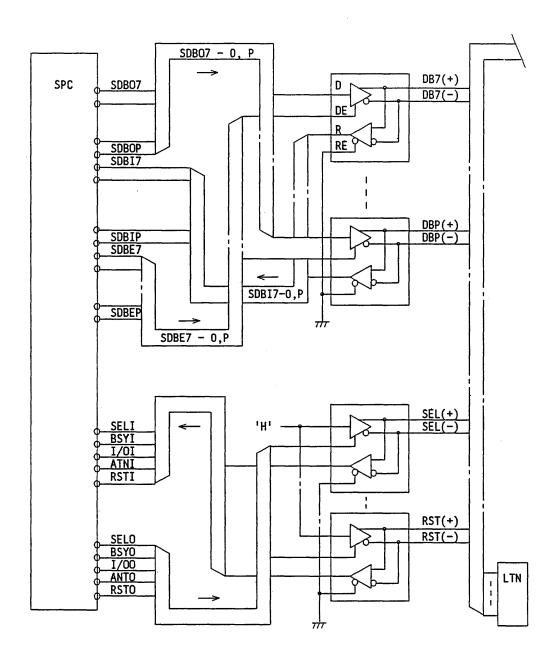
Fig. 5.1.3 Example of differential type SCSI driver/receiver circuit (continued on next sheet)
