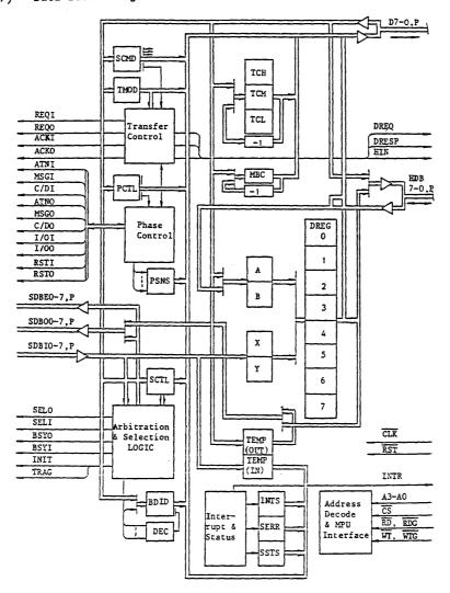
Figure 3.1.1 SPC functional block diagram
