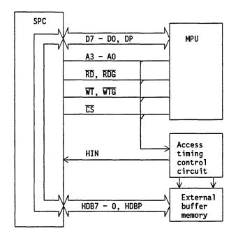
Fig. 4.14.1 Access from MPU to external buffer memory
