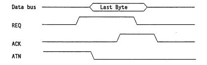
Fig. 4.3.3 ATN signal resetting in MESSAGE OUT phase
