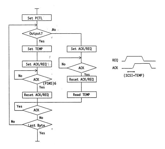
Fig. 4.3.4 Manual transfer procedure (SPC serving as a TARGET)
