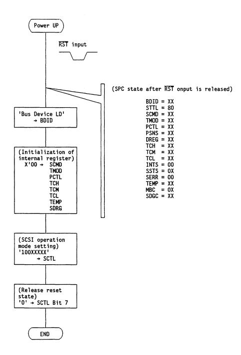
Fig. 4.16.1 SPC initialization (at power-on)
