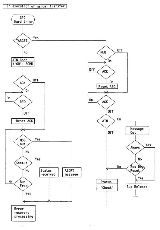
Fig. 4.11.4 Example of control processing for SPC-detected error (2)
