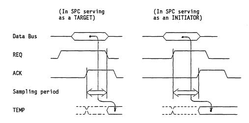
Fir. 4.7.1 Data bus save in manual transfer input operation
