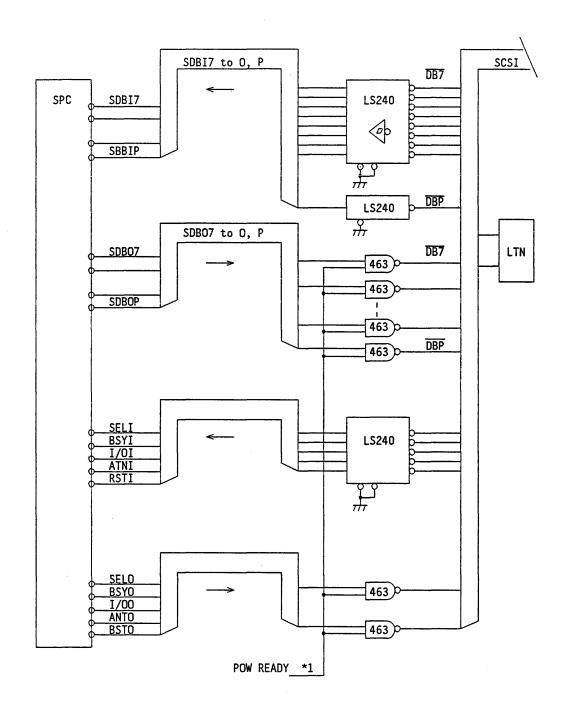
Fig. 5.1.2 Example of single ended type SCSI driver/receiver circuit (continued on next sheet)
