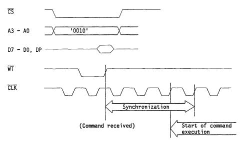
Fig. 4.3.6 Command execution timing
