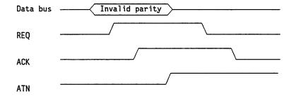
Fig. 4.3.2 ATN signal generation in data transfer
