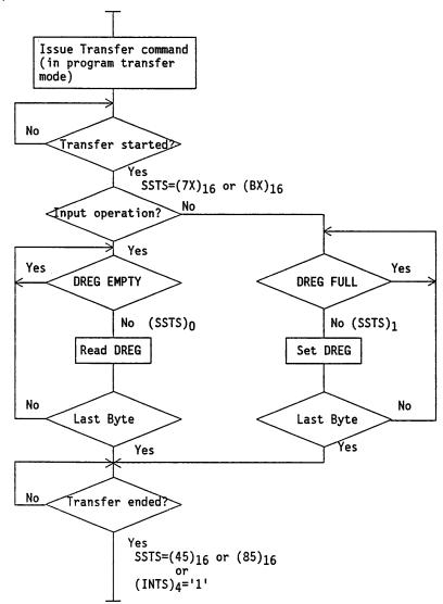
Fig. 4.6.1 DREG access procedure in program transfer mode
