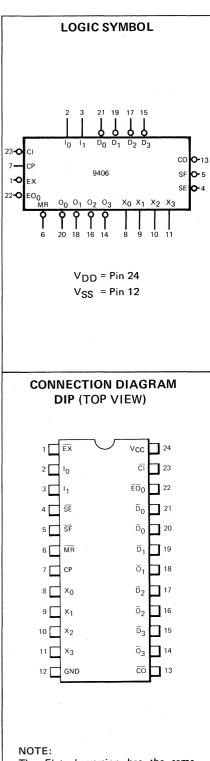
The Flatpak version has the same pinouts (Connection Diagram) as the Dual In-Line Package.
