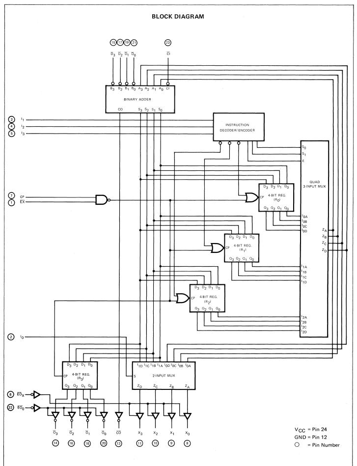
**FUNCTIONAL DESCRIPTION** – The 9407 contains a 4-bit slice of three Registers  $(R_0-R_2)$ , a 4-Bit Adder, a 3-state Address Output Buffer  $(X_0-X_3)$ , and a separate Output Register with 3-state buffers  $(\overline{O}_0-\overline{O}_3)$ , allowing output of the register contents on the data bus (refer to the Block Diagram). The DAR performs 16 instructions, selected by  $I_0-I_3$ , as listed in Table 1.
