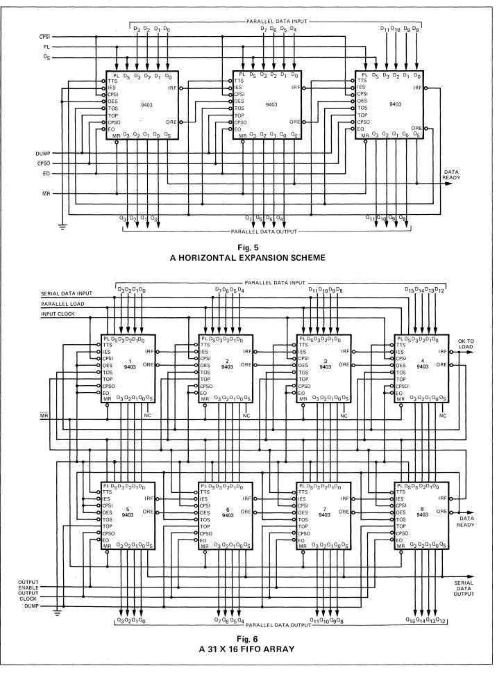
Horizontal and Vertical Expansion – The 9403 can be expanded in both the horizontal and vertical direction without any external parts and without sacrificing any of the FIFO's flexibility for serial/parallel input and output. The interconnections necessary to form a 31-word by 16-bit FIFO are shown in Figure 6. Using the same technique, any FIFO of  $15n_1 + 1$  words by 4 X n<sub>2</sub> bits can be constructed.
