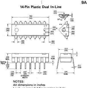
Leads are intended for insertion in hole rows on .300" centers They are purposely shipped with "positive" misalignment to facilitate insertion Board-drilling dimensions should equal your practice for .020" diameter lead Leads are tin-plated kovar Package weight is 0.9 gram Package material is silicone 24-Pin Plastic Dual In-Line
