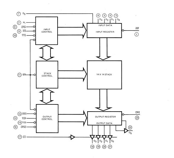
**FUNCTIONAL DESCRIPTION** – As shown in the Block Diagram the 9403 consists of three parts:
