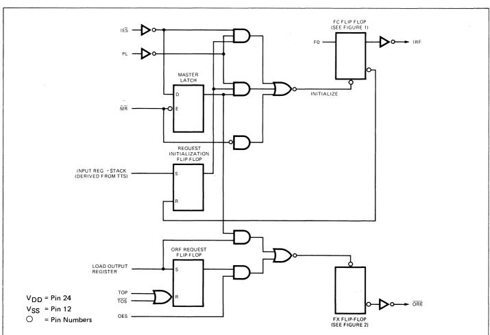
Fig. 10 CONCEPTUAL DIAGRAM, INTERLOCKING CIRCUITRY
