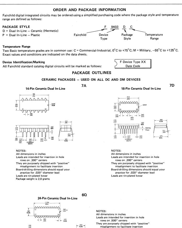
Board-drilling dimensions should equal your practice for .020" diameter lead Leads are tin-plated kovar
