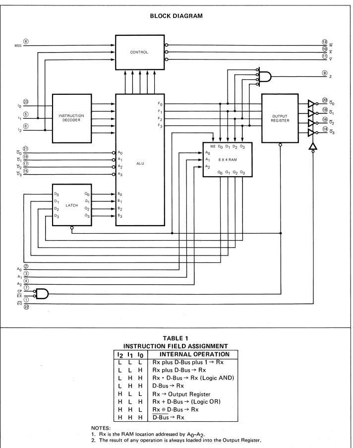
**FUNCTIONAL DESCRIPTION** – As shown in the Block Diagram the 9405 Arithmetic Logic Register Stack (ALRS) consists of a 4-bit ALU, an 8-word by 4-bit RAM with output latches, an instruction decode network, control logic and a 4-bit Output Register.
